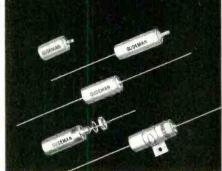
The development of the Gudeman "XC" capacitors results in a new line of high temperature capacitors that has exceptionally high insulation resistance, low power factor and low dielectric absorption. The case sizes were selected whereby no voltage derating is required when the capacitors are used within a temperature range from  $-65^{\circ}$  C. to  $+165^{\circ}$  C.
