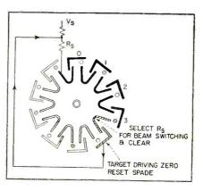
FIG. 8—Tube interconnection for fourposition indication
