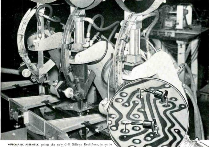
possible by the Axial Lead design. There is no heat sink required, no troublesome screw terminals. Leads slip easily into the board, and dip-soldering quickly completes the assembly.
