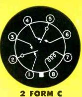
These relays contain 2, 3, or 4 magnetic switches. Each switch is hermetically sealed in a high pressure hydrogen atmosphere in a glass capsule. Platinum contact surfaces are continuously wetted with mercury by capillary connection to mercury reservoir.
