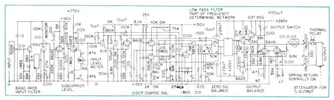
FIG. 22—Circuit diagram of linear multivibrator type of subcarrier discriminator. Plug-in filters permit use on any of the standad channels. Output limiting circuit protects the load (such as recording galvanometer) if output becomes unbalanced in excess of  $\pm$  150 percent full scale
