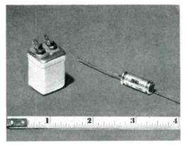
125 C TANTALYTIC\* CAPACITORS—for high speed aircraft and missile systems where quality, long life, and small size are main requirements. In plain or etched foil, and rectangular or tubular designs. Ratings: .25 to 180 uf, 10 to 100 volts. Tolerance: +20% (plain foil), -15 to +75%(etched). Temp. range: -55 C to +125 C. Write for GEA-6258. \*Reg. trade-mark of General Electric Co.
