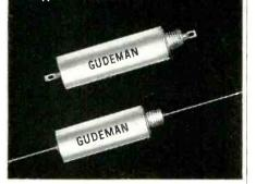
The Gudeman Feed-Thru Capacitor, Types 271 and 272, is a three-terminal component designed to be used for R.F. Interference suppression in a manner similar to a low pass filter. The typical insertion loss characteristics for these Feed-Thru Capacitors when measured in a 50 ohm line are in accordance with MIL-Standard 220.
