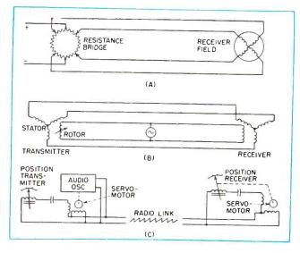
FIG. 15—Remote dial reading systems. So-called d-c synchro (A), conventional a-c synchro (B), and tuned audio system (C)
