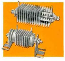
**POWER RECTIFIERS** with solid stack assembly range in size from  $1" \ge 1"$  to  $5" \ge 6"$  and with convection cooling are rated from .80 to 10.0 amperes per cell on a single-phase full-wave bridge basis.
