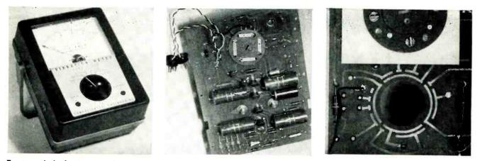
Front panel of vibration meter having six-position frequency range switch, one side of double-etched circuit board and front and rear closeup views of etched range switch
