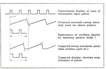
Comparison of triggered or driven sweep with synchronized free-running sweep
