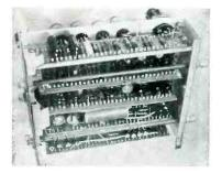
BUT THIS—Neat, compact vertical "planes of circuitry" result from construction based on Alden Terminal Card Mounting System.
