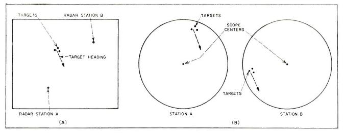
FIG. 1—Configuration of targets and radar stations (A) and simulated ppi presentations (B)
