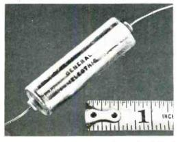
METAL-CLAD TUBULAR CAPACITORS for all d-c uses where utmost reliability is required. Ratings: .001 to 1.0 uf, 100-600 v. d-c. Tol:  $\pm 5\%$ ,  $\pm 10\%$ , or  $\pm 20\%$ . Temp. range: -55 C to +125 C with solid impregnant: -55 C to +85 C with mineral oil. Write for GEC-987.
