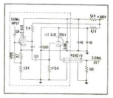
Tandem cathcde-follower probe has attenuation of only 2 to 1 with input capacitance of less than 3  $\mu\mu t$
