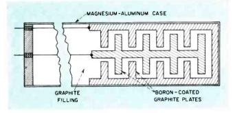
FIG. 11—Parallel circular-plate ionization chamber has boron-coated electrodes for detection of slow neutrons. Wire leads are of lead and are coated with quartz
