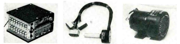
Electronic commutator (left) uses 20 tube sections and 50 semiconductor diodes. Sampling switch built by General Devices (center) has three poles with 60 shorting channels for each pole. Unit at right, operating at 1,800 rpm, is used in ground tests
