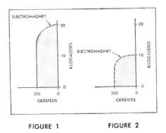
Therefore, to make the comparison valid, the residual induction of the electromagnet must be reduced to 10,000 gausses (Figure 2).
