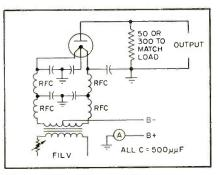
FIG. 2-Noise diode and its circuit
