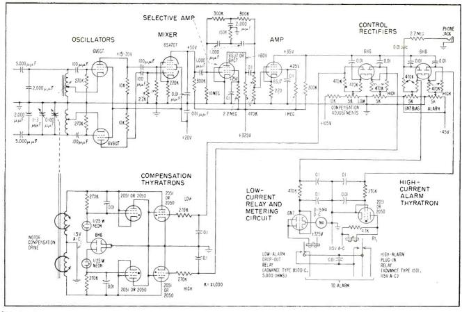
FIG. 3—Complete control circuits of Browning model BL-300 alarm signal system. Power supply is conventional
