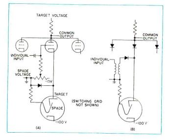
FIG. 26—Typical beam-gated sampling circuits using the Burroughs magnetron beam switching tube built by Haydu.
