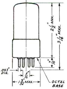
This precision sealed-inglass crystal unit provides exceptional stability with minimum ageing when used as a reference source secondary frequency in standards.
