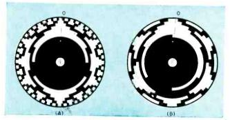
FIG. 23—Binary code disks used to sense fluid level and convert it to pulse code. Disk (A) measures inches and (B) measures feet
