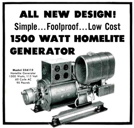
• New Money-Saving features... No DC brushes; just two easy-to-get-at collector ring brushes... No commutator or DC windings... No intermediate couplings; armature keys directly to shaft. Fewer parts to wear out — longer trouble-free generator service.
