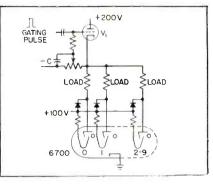
FIG. 9-Single-triode gating circuit
