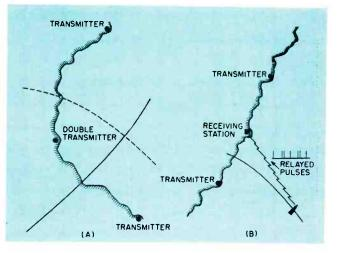
FIG. 5—Data transmission in position-finding system often depends upon time of propagation. A standard hyberbolic fix from two pairs of transmitters is shown at (A). A relayed line of position comes from the lifeboat at (B)
