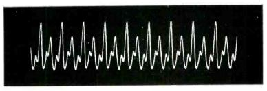
Vibrations of the sound "or" in the word "four." Pattern represents nine of the "pitch periods" which originate in puffs of air from the larynx when a word is spoken.
