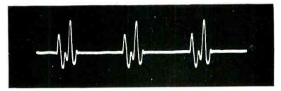
An electronic sampling of the "or" sound. One "pitch period" in three has been selected for transmission. This permits great naturalness when voice is rebuilt. Intelligible speech could be sent through a 1 in 6 sampling.
