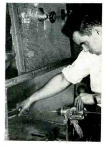
Spraying resistance card with molten metal to form end connections, using combination mask and holding fixture
