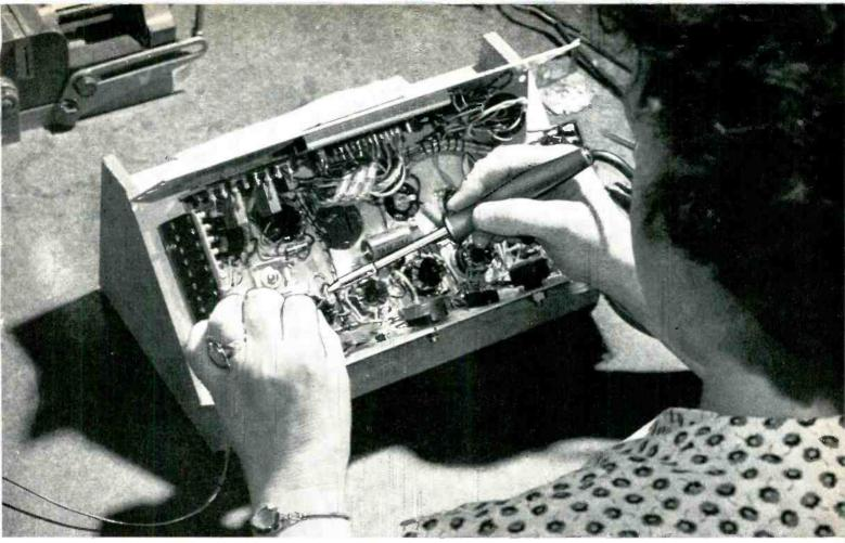
**HARD-TO-REACH JOINTS** in Sauborn Co.'s electro-cardiographs are soldered quickly with the fine-point G-E Midget iron—with no damage to adjacent parts. Weight of iron—less than 2 cunces—helped increase output by reducing operator fatigue. The Midget's ironclad-copper tip saves Sanborn  $\frac{1}{2}$  hour cleaning and tinning time daily, per operator station.
