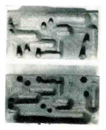
Aluminum mold (top) and sponge rubber pressure pad made from it for use in holding components down on wiring board while cutting and clinching leads
