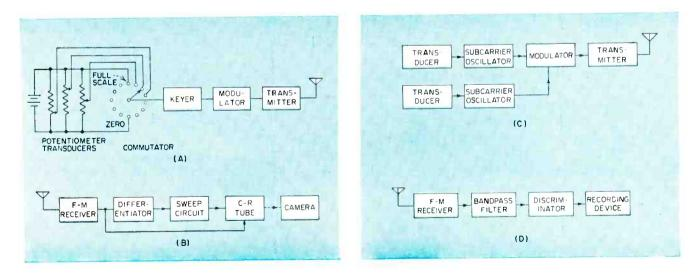
FIG. 19—Basis of pulse-width modulation of a frequency modulated carrier (pwm/f-m) transmitter (A) and receiver (B). Two-channel f-m/f-m transmitter (C) and receiver (D)
