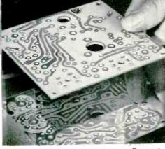
G-E "Thru-Con" Printed Circuit Boards offer positive connection through the holes, without staking pins, patterns on both sides if needed. Printed circuitry cuts assembly time, eliminates product bulk and weight, reduces inspection time and parts inventory.
