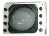
DIRECT DISPLAY OF IMPEDANCE can be obtained by using the Type 1025 Hybrid in conjunction with the AMCI type 1028 Polar Display Unit (frequency range 120 mc to 240 mc) together with a standard d-c oscilloscope and suitable swept oscillator. A typical display is shown in the unretouched photograph at the left.
