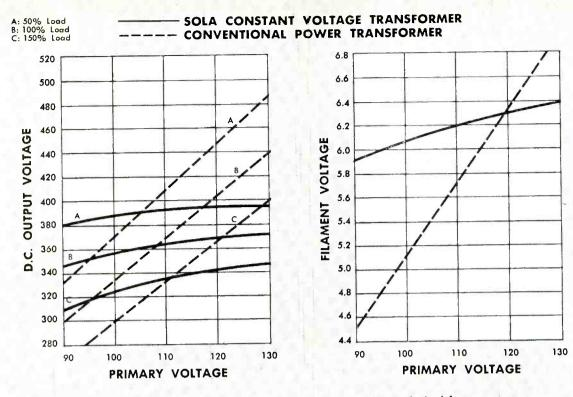
These curves contrast the plate and filament supply voltages obtained from a Sola and a conventional power transformer when line voltage is varied from 100v to 130v.
