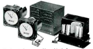
The Transicoil servo assembly used in the Lorac receiver. Components include a 400 cycle oscillator supply for two indicators and two servo amplifiers. System is built on separate chassis to permit the indicators and amplifiers to be located in separate parts of the ship.
