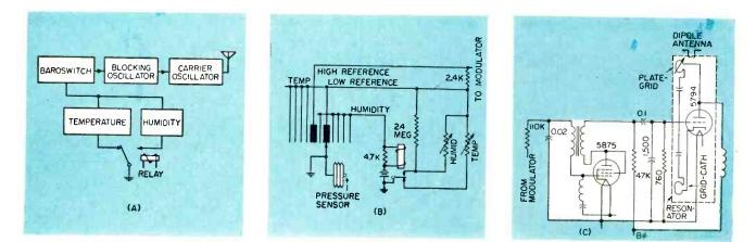
FIG. 27—Elements of a modern weather radiosonde (A) that show dependence upon the commutating system (B). Modulator and r-f transmitter shown at (C) transmit tones representing weather measurements
