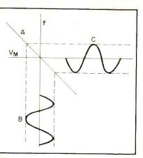
FIG. 3—Transfer characteristic of reactance-tube circuit
