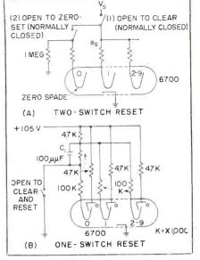
FIG. 4-Resetting circuit arrangements
