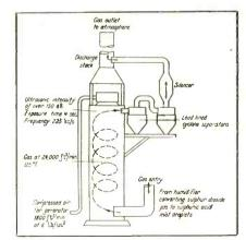
Schematic arrangement of acid fog precipitation using sonic agglomeration
