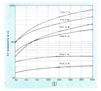
FIG. 21—Pulse-code signaling systems compared with other types on the basis of signal-noise ratio and bandwidth
