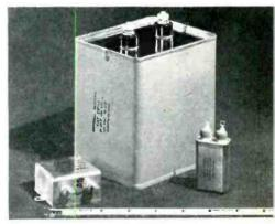
MIL-C-25A CAPACITORS—for filter, by-pass, and blocking in military equipment. Built to MIL-C-25A specifications. Ratings: .05 to 15 uf at 100 to 12,500 v. d-c in case styles CP50, CP60, CP70 series. Temp. range: -55 C to +85 C, and -55 C to +125 C. Write for GEC-810.
