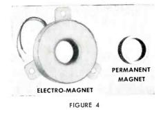
*First*, no power source is required with permanent magnets, because no energy is consumed. Once magnetized, the field is permanently retained.
