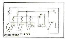
FIG. 6—Automatic zero reset circuit
