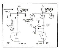
FIG. 11—Beam-gated sampling circuits
