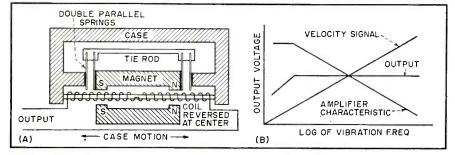
FIG. 1—Electromagnetic vibration transducer used as pickup (A) and voltage-frequency transfer characteristics of system (B) (B)
