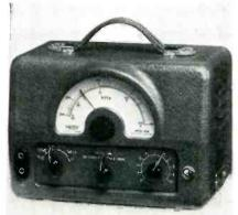
from 30 cps to 30 kc which largely covers the acoustic frequency range. It is intended for adjustments of a-f amplifiers and measurements at audio and acoustic frequencies. Output level is adjustable from 10  $\mu v$  to 10 v by an accurate attenuator system. An automatic regulation circuit keeps the output level constant with changes in frequencies.
