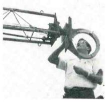
FIG. 2—Panning head and driver shafts. Ring mounted on plate holds transmitter and dish antenna
