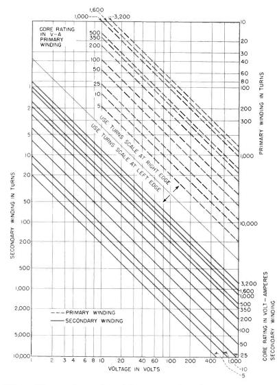
**D**<sup>ESIGN</sup> of simple, low-voltage transformers creates a problem for most transformer design groups. These design charts eliminate or minimize the amount of calculation necessary.
