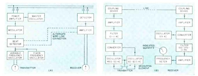
FIG. 16—Frequency telemetering system depends upon transmission of audio tone (A). Variation of the system uses two oscillators whose frequencies are varied in opposite directions (B)
