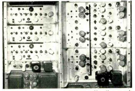
Complete three-channel gamma correction amplifier
