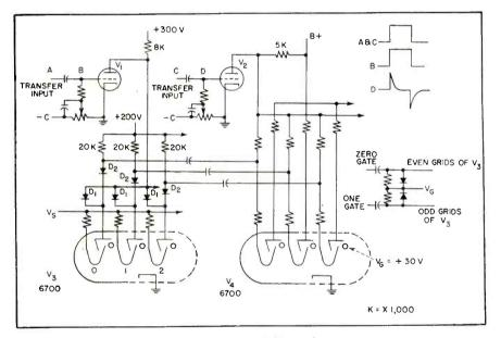
FIG. 10-Transfer-storage circuit using two switching tubes
