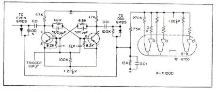
FIG. 13—Transistor driver used with low-voltage version of beam switching tube. One switching tube can do all the functions of approximately twenty transistors
