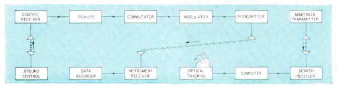
FIG. 24—Possible arrangement of tracking and telemetering equipment to observe phenomena between 200 and 300 miles above the earth from the Vanguard satellite on its orbit about the earth
