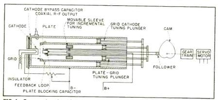
FIG. 1—Cross-section of stable L-band local oscillator
