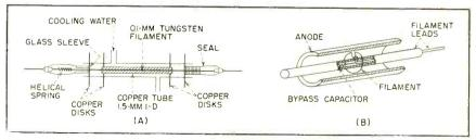
FIG. 3—Disk-seal coaxial noise diode (A) and coaxial-line noise diode (B)
