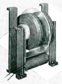
**High Voltage Plate Trans**former for use under oil with other equipment in same tank. Unit shown is 50 KV center tap grounded, 4 KVA and high impedance. Note plastic insulation shield between coils. This unit available from 100 VA to 100 KVA.
