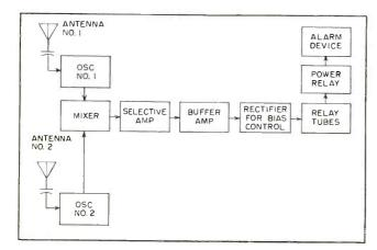
FIG. 1--Elements of complete electrostatic intrusion alarm
