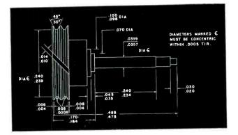
Inspection of incoming precision shafts took 10 to 15 minutes each by mechanical gaging—involved concentricity, diameters, shoulder locations, and other tough-to-measure dimensions to tolerances of .0002". Doing the work on a Kodak Contour Projector cut time to 2 to 3 minutes per shaft:
