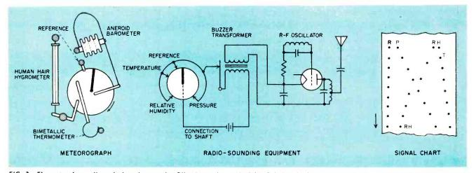
FIG. 3—Elements of a radiosonde based upon the Olland sampling principle. Relative displacement of elements is shown by a series of short dashes on moving chart paper at ground station
