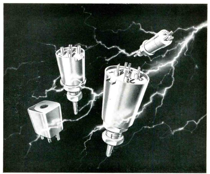
Four sizes of shielded coil forms cover a wide range of design requirements. Dimensions when mounted, including terminals, are: LS-12 (square type for printed circuits),  $\frac{1}{2}$  " x  $\frac{1}{2}$ " x  $\frac{1}{2}$ "; LS-9,  $\frac{1}{6}$ " diameter x  $\frac{1}{2}$ " high; LS-10,  $\frac{1}{6}$ " x  $\frac{1}{6}$ "; LS-11,  $\frac{1}{16}$ " x  $\frac{1}{12}$ ". Each form mounts by a single stud. Windings may be universal or wound to your specifications.
