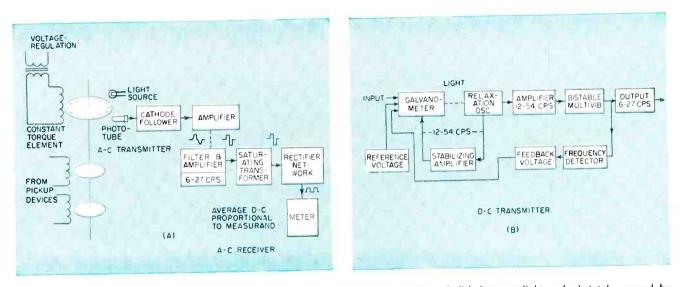
FIG. 18—Power-line telemetering system sends low-frequency pulses derived from rotation of disk between light and phototube caused by variation in a-c parameters (A). Information derived from d-c is transmitted by equipment (B)
