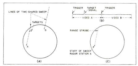
FIG. 2—Target pattern (A), video output (B) and method of writing targets on storage tube (C)  $% \left( C\right) =0$
