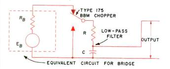
In basic modulator circuit, chopper alternately connects filter across bridge and then shorts filter
