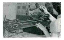
Linearity checking setup, with resistance card on fixture in front of **B** battery. Contact arm running over card is moved by stainless steel belt going over shaft of master potentiometer in front of operator
