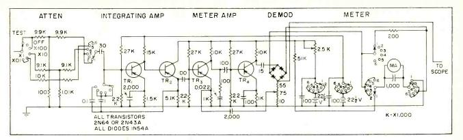
FIG. 2—Integrating amplifier uses one grounded-emitter and one grounded-collector stage. Meter amplifier uses two groundedemitter stages. Range switch controls input attenuator
