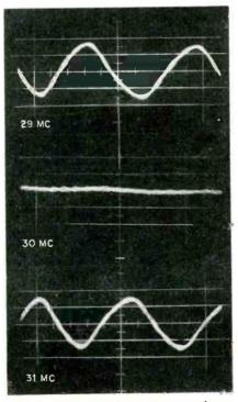
FIG. 6-Servo amplifier output waveforms at null and at either side of null
