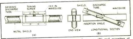
FIG. 4-Glow-discharge noise source for microwave frequency (A) and mounting of small-bore tube to generate shi noise (B)
