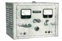
bench cabinet with all controls and gages conveniently located on the front panel. The portable, versatile instrument is suited for altitude test chambers, evacuation of tubes, and leak detection of mechanical aud electrical components.
