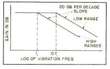
FIG. 3—Frequency response of meter on low and high frequency ranges
