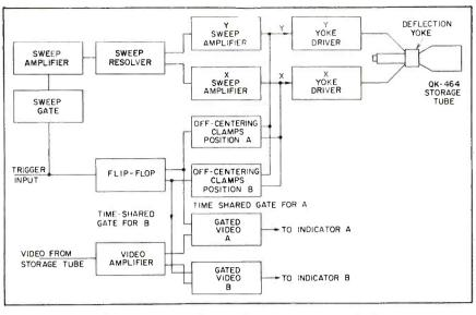
FIG. 3—Time-shared sweep permits alternate display on two radar indicators
