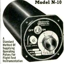
The Model N-10 Intervalometer is a lightweight, compact instrument for controlling the cycle rate of camera recording devices and other electrically or electronically operated apparatus. Pulse rates per second are 1. 2. 4. 5. 8, and 10, and the pulse length is variable from 25 milliseconds to 70 milliseconds. Special pulse intervals and pulse duration may be supplied on order. The Model N-10 Intervalometer is built to meet all environmental conditions encountered in aircraft use.
