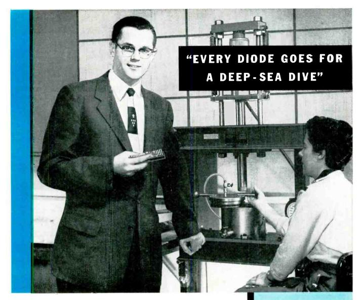
Morgan McMahon, Head of Engineering Services, is in charge of PSI's product applications and manufacturing engineering. Here he holds diodes prior to subjecting them to 1000 p.s.i. hermetic seal test.
