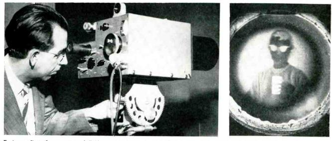
Engineer adjusts the evaporograph (left) to pick up image of girl holding a glass of ice water. The picture (right) was taken in a completely darkened room at a distance of 30 feet
