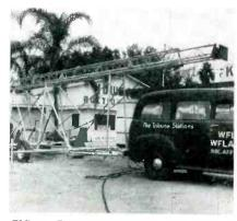
FIG. 1—Trailer carrying tower is located at desired spot. Outriggers keep unit steady while tower is raised in about three minutes
