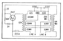
FIG. 1—Transistor negative-impedance telephone line repeater
