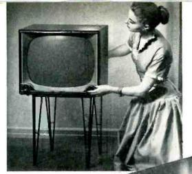
ALSO ..... no more bothersome "both-hands" tuning of the set! The distance switch can be eliminated-another 6BU8 plus and cost-saver. When choosing programs, viewers no longer need manipulate two controls: tuning knob and distance switch. One control knob will tune in all stations, near and far.
