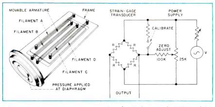
FIG. 7—Unbonded strain-gage pressure transducer has diaphragm mechanically coupled to movable armature. Pressure variations cause armature to move and change tension of wire filaments. Typical circuit is shown at right; source voltage can be a-c or d-c
