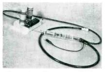
Video probe with power-supply filter chassis. Cable terminating resistor is located in cable connector
