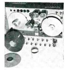
New take-apart spool, at left, being disassembled from airborne tape recorder. Extra sleeve appears in center foreground. Spool at right is older solid type that cannot be taken apart
