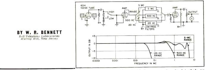
FIG. 1-Circuit (A) and spectral density (B) of noise generator using hot-cathode arc
