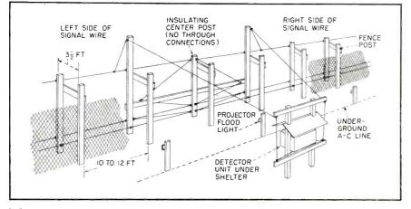
FIG. 4-Example of antenna system and lead-in for woven-wire fence
