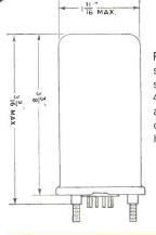
Photo and dimensional drawing of steel can in which 4 Form C switches are enclosed with coil. Plug-in header shown.
