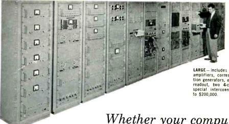
LARGE – includes two control units with 200 pots, 80 amplifiers, corresponding number of multipliers, function generators, etc., plus digital voltmeter with printed readout, two 4-channel recorders, timing matrix and special interconnecting panel. Price range, \$100,000 to \$200,000.
