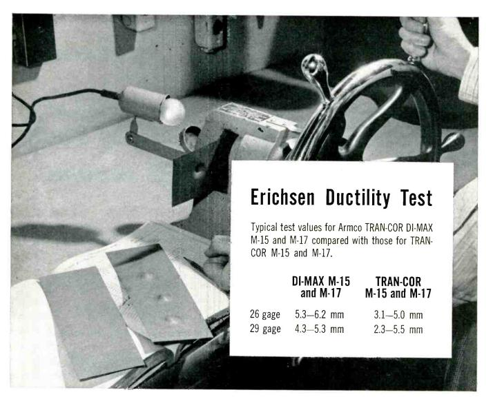
Armco's DI-MAX process now offers a new design advantage in the low core loss M-15 and M-17 electrical steels. Better, more uniform ductility now makes it possible for designers to use punched laminations where they need the low core losses of these grades.
