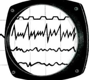
The Beamplexer is actually a fast electronic switch. Its heart is the Burroughs Beam Switching Tube which acts as a gate, picking the ten parallel input signals off in sequence, at adjustable speeds ranging from push button to 100 kc, and putting them out on one line. Each signal can be located on the scope as desired, and even superimposed on another, through individual position and amplitude controls for each channel. Other controls include separate amplification for each channel.
