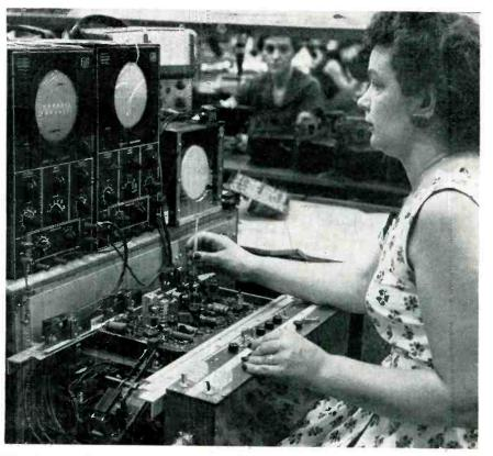
Adjusting transformer on sync board. All connections are made automatically by solenoids after operator slides board into position on test stand
