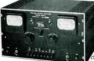
Models 5-2V and 5-4V Variable Voltage Regulated Power Supplies provide extremely well filtered and regulated direct current output which may be varied continuously without switching from zero to 500 volts. Maximum current output of the instruments may be drawn at any voltage setting. **REGULATION:** against load .15%
