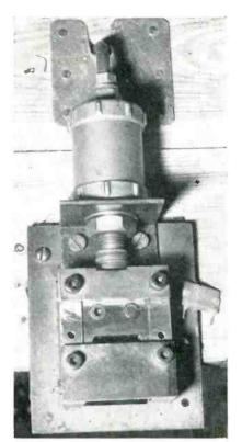
Air-actuated lead chopper for ceramic components
