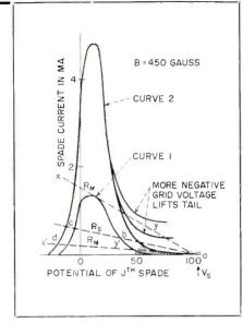
FIG. 2-Spade characteristic curves
