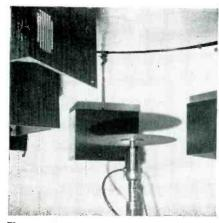
Electrostatic spray room, showing disk
