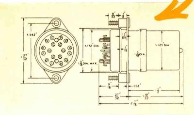
THIS NEW UNION 10,000 ohm, current-sensitive relay picks up at a nominal value of 8 milliamperes throughout the entire temperature range of  $-65^{\circ}$ C to  $+125^{\circ}$ C, while maintaining the excellent shock and vibration characteristics inherent in our standard design. It can withstand 200 volts across the coil continuously.
