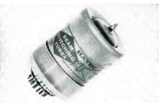
Beam switching tube of a type being used in telemetering equipment
