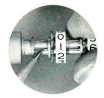
The problem was to check many small calculating machine parts averaging about 13 critical dimensions for each with shapes mostly complex. With carefully engineered mechanical gages, inspection time averaged 50 seconds each. Optical gaging on a Kodak Contour Projector brought the average down to 12 seconds.
