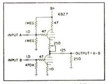
FIG. 6-Simplified diagram of difference amplifier used in each masking amplifier channel
