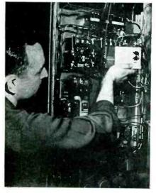
Exploring trouble sources in electrical equipment is a new use for pocket-sized transistor radios, according to Raytheon
