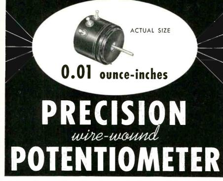
Jewel bearings for lowest torque, and superior seal against surroundings that contain abrasive dust, make this new, Model LLT 7/8 Waters pot the ideal unit for high-reliability service where minimum torque is essential. With torque low enough to permit actuation by a Bourdon tube or a bimetallic thermal element, this potentiometer offers new advantages in sensitive-instrument applications as well as in computer, servo, and selsyn uses. Check your needs with these specifications:
