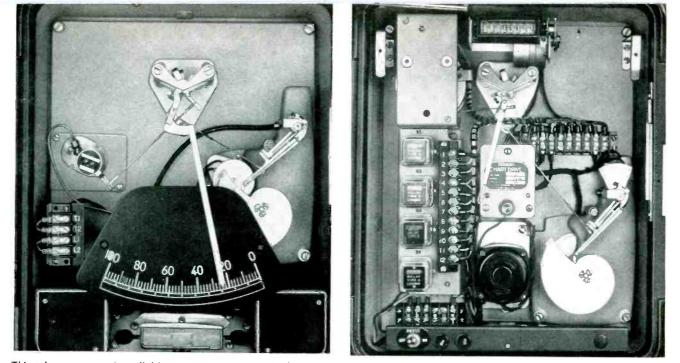
This telemeter transmitter (left) uses a cam to transmit the temperature pickup reading. The receiver (right) has a reversible motor that moves in either direction or remains motionless. A pen is attached to the drive
