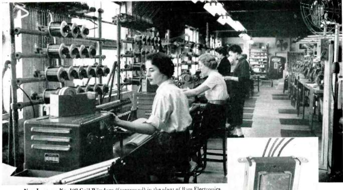
New Leesona No. 108 Coil Winders (foreground) in the plant of Ram Electronics, Inc., L.vington, N. Y., where Leesona Winders have become "standard equipment." These were added as best winders for producing short runs of stick-wound coils of varying specifications. (Inset) Ram has built an excellent reputation for winding quality coils and transformers used in radio and TV equipment.
