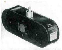
The MA-200 is a pulsed-type fixed-tuned magnetron generating approximately 40 kw peak power at 35 kmc. Its r-f spectrum is unchanged when subjected to vibration conditions of 15 g at 1,000 cycles.
