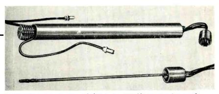
Traveling-wave tube with helix and electron gun assembly shown in foreground
