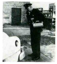
Among the growing list of transistorized firsts is the Motorola two-way portable communications set that employs transistors in i-f amplifiers and audio stages of the receiver. Battery drain is thereby reduced more than 70 percent
