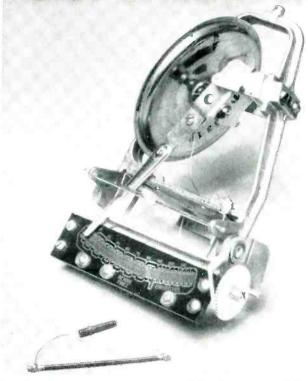
Transducer elements of radiosonde include, from top to bottom, barometer for altitude, thermistor for temperature and lithiumchloride coated plastic sheet for humidity measurements
