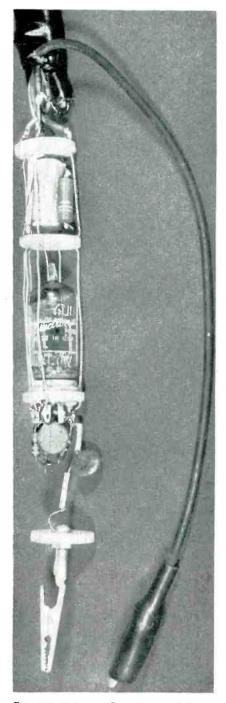
Components mounted on tube socket are connected to power supply and output wiring by bus wires running up sides of tube as shown in the photograph
