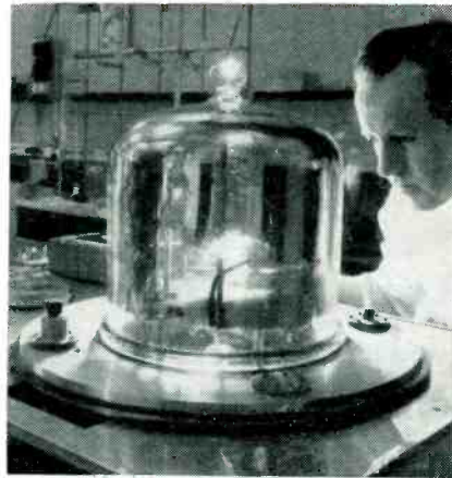
Fabricating diffusion transistors: left, adjusting temperature of vacuum oven in which solid-state diffusion occurs; center, evaporating metal contacts to transistor prior to attaching wire leads. Silicon double-diffusion transistor is shown at right
