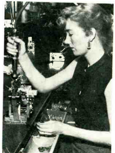
Inserting mounting bolts in tuner with air gun while clamp on welded support holds end plate in position
