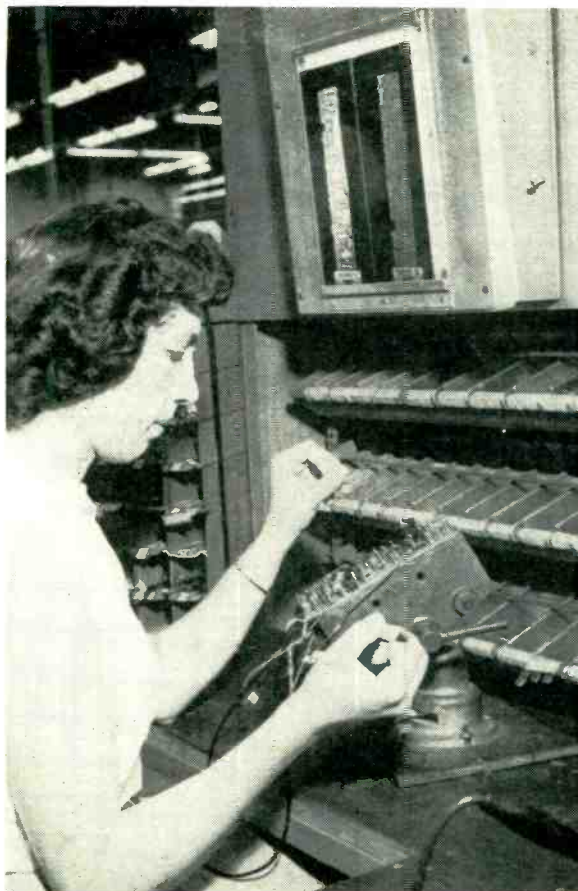
Single-station portable ferris-wheel bin setup, with color transparencies of finished wiring board mounted in light box overhead to guide operator
