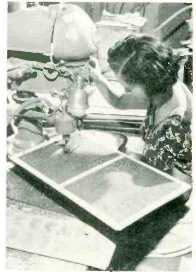
Method of drilling tape sandwich while air-operated foot presses boards firmly down on table of drill press
