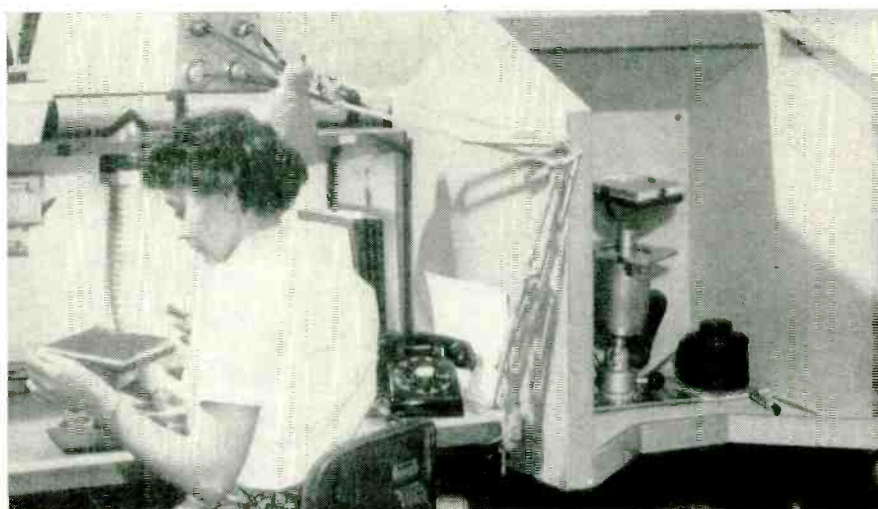
Wiring station, showing operator threading wire through cores held by frame of work fixture on bench. Core-positioning station at right is acoustically treated to reduce noise from vibrating jig
