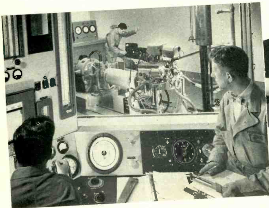
Engineer checks action of automatic transmission, with water simulating the flow of oil. His hand rests on a Standard timing instrument in the foreground.
