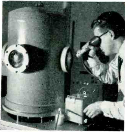
Fabricating diffusion transistors: left, adjusting temperature of vacuum oven in which solid-state diffusion occurs; center, evaporating metal contacts to transistor prior to attaching wire leads. Silicon double-diffusion transistor is shown at right
