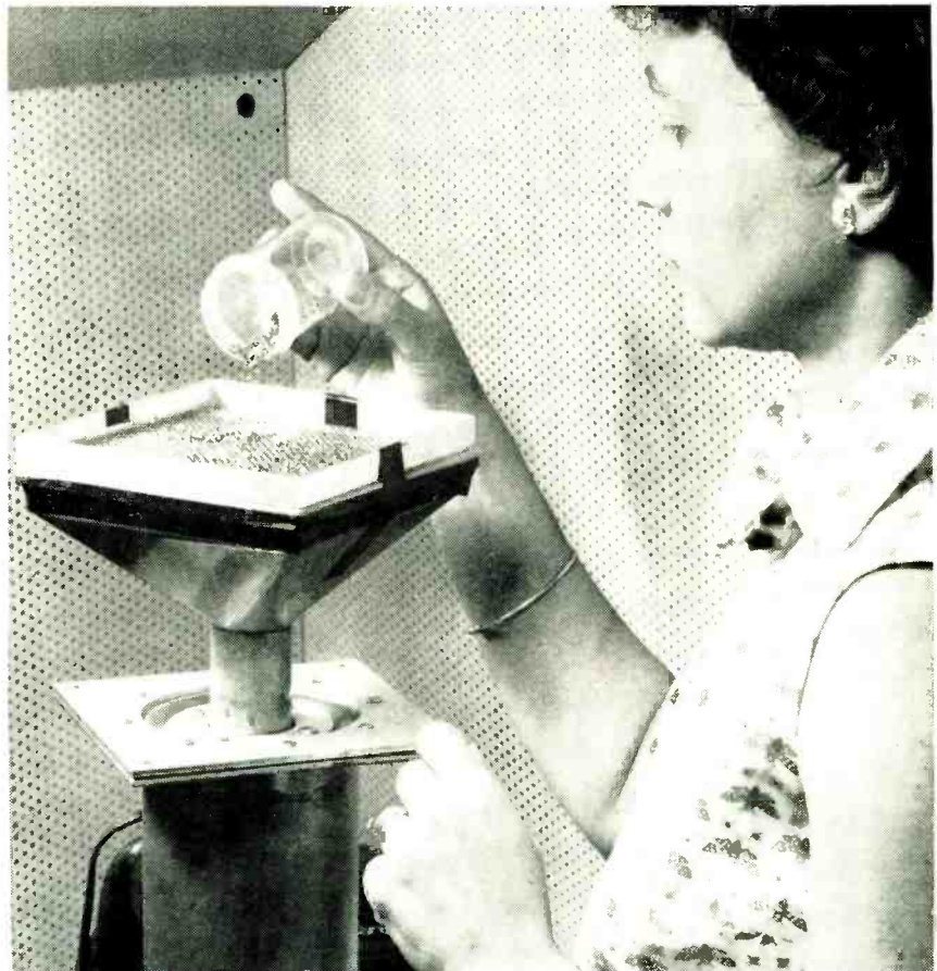
Pouring ferrite cores on to fenced-in area of vibrating form while vacuum cleaners are pulling air at full speed down through flexible hose at lower left. During pouring, form may be tilted and rotated to get one core into each of the 4,096 pockets
