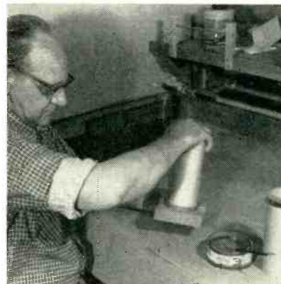
Quick turn of cylinder inside block-type applicator applies compound neatly in uniform band on outside
