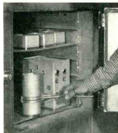
Removing cylindrical housing from 500 F oven after tinning compound has fused
