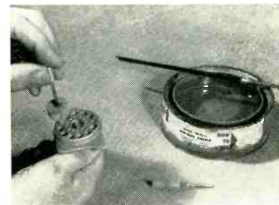
Applying tinning compound inside a hole with a small applicator. The compound is here applied to the felt with a small brush
