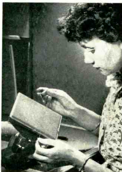
Method of using long 26-gage hypodermic needle to pull wires through 50-mil inside diameter of cores. An X wire and the Z winding are being pulled simultaneously
