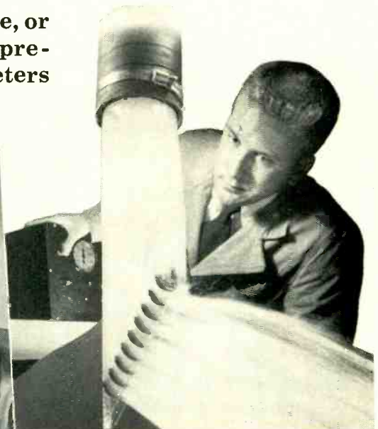
Engineer checks action of automatic transmission, with water simulating the flow of oil. His hand rests on a Standard timing instrument in the foreground.
