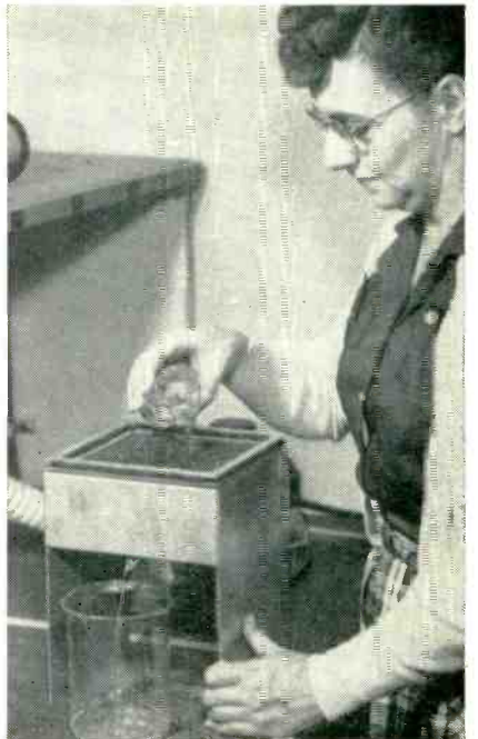
Pouring diluted Amphencil Polyweld over dip-soldered mat to cement each core at its four-wire junction below for later use
