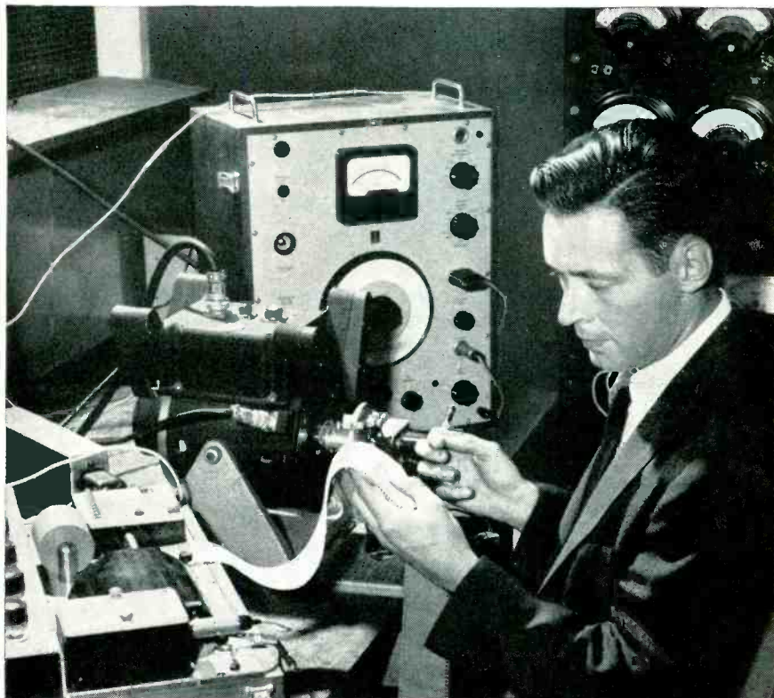
Engineer locating tube resonances from a record of noise output by a tube which has been subjected to sinusoidal vibrations over a range of frequencies at 15 times the force of gravity.
