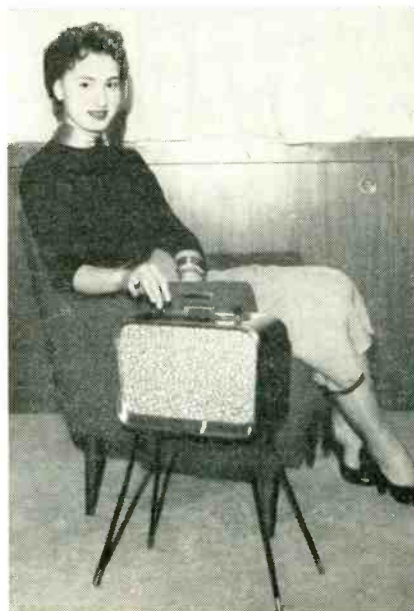
Cordless, all transistor home radio that operates on six transistors and a self-contained battery is CBS-Columbia chairside model
