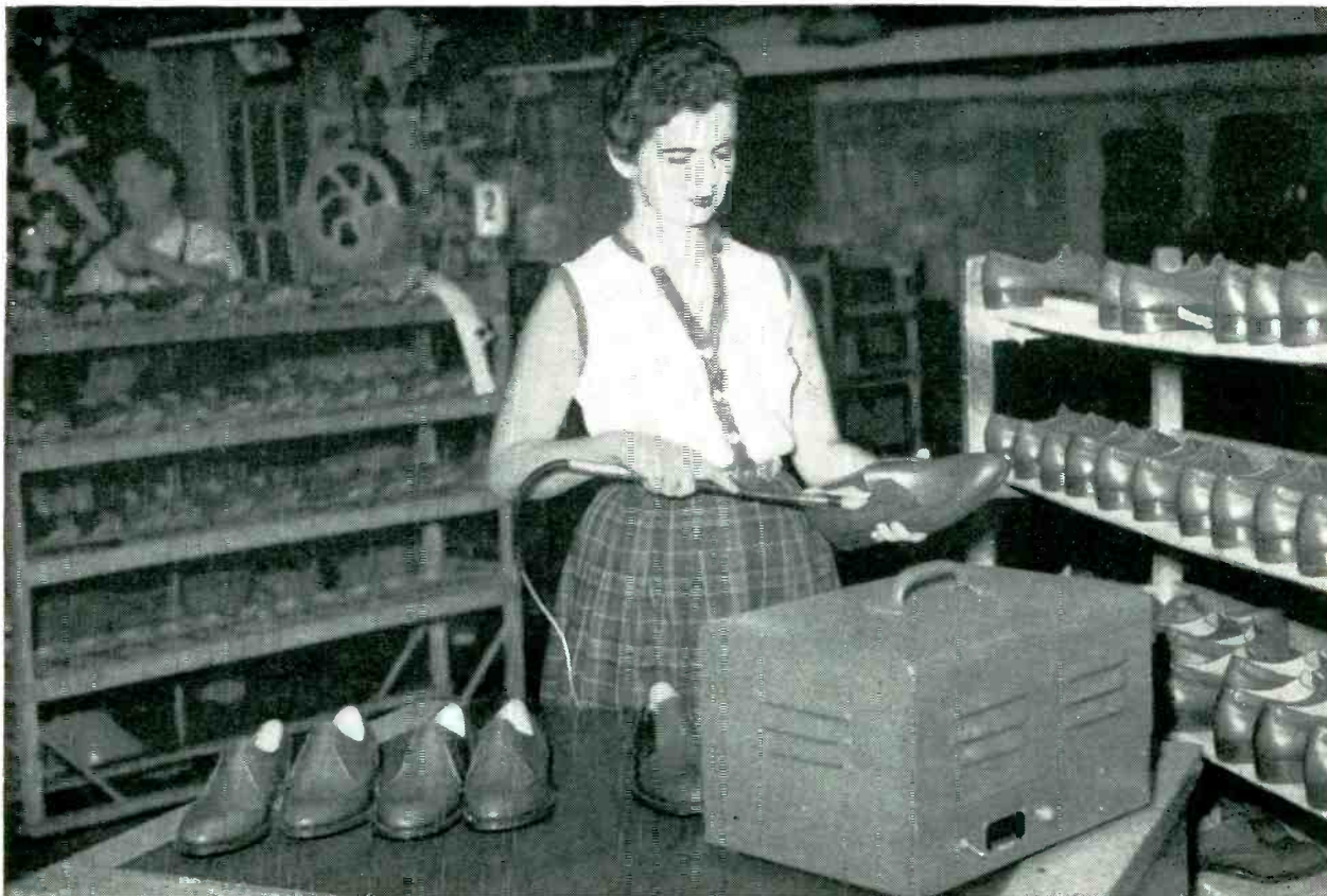
Checking shoe insoles for projecting tacks is speeded by r-f detector using oscillator loading to signal presence of metal
