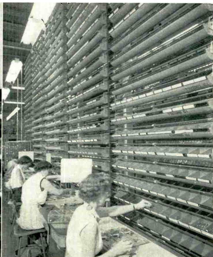
Large five-station permanent ferris-wheel bin setup, with bins independently controlled by the five operators. All bins are clearly labeled for quick identification when bins are run up or down for new job setup
