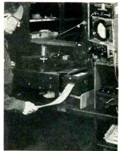
Linearity checker in operation
