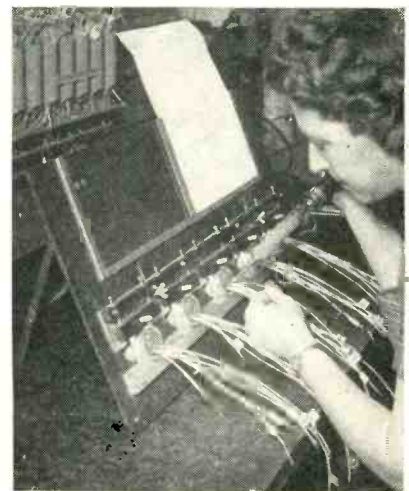
Assembling plugs with aid of universal holding fixture
