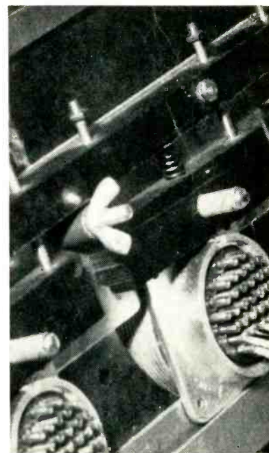
Details of holding fixture. Wing nut can be loosened to slide under strip up or down to accommodate different sizes
