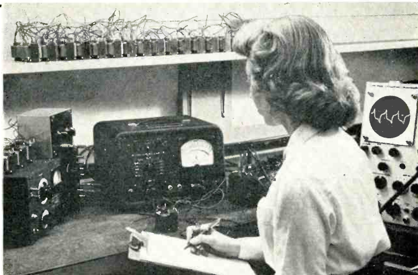
Voltmeter allows 100- \mu v signal to be detected with a noise level of 12 \mu v's
