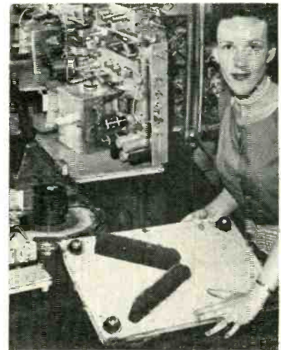
Method of mounting table-sweeping brooms under one of dollies on color-tv test line. Wood handles of broom project up above top of dolly through cut-out slots, hence the sweeping dolly does not normally carry a chassis
