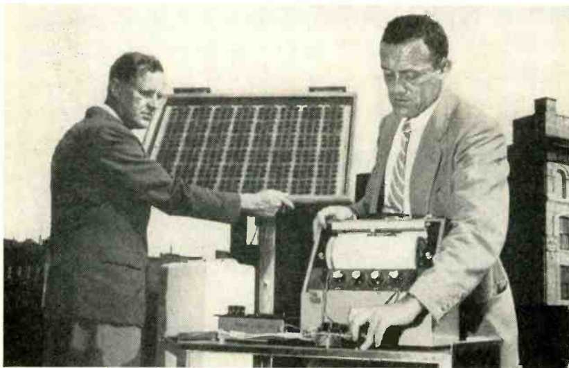
SOLAR battery developed by Bell Laboratories gets final tests before shipment.
