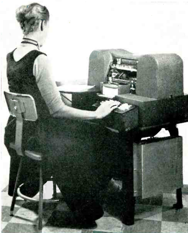
CARD PUNCHER —Keyboard of commercial model has been modified to punch binary members for programming the various machines of the Automatic Component Assembly System
