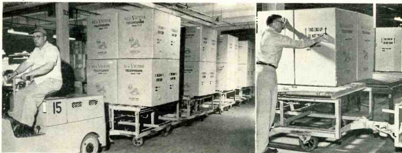
Pulling train-load of cabinets for 21-inch television receivers up to the ends of roller conveyor lines. Cars have double-layer loads of eight cabinets each
