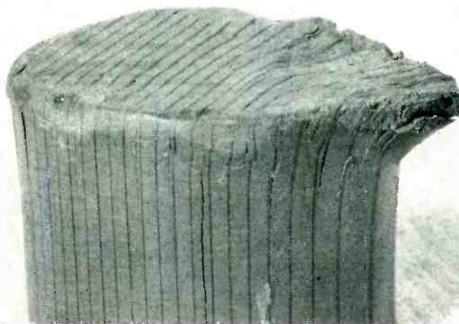
Tip of 2" diameter Taylor Built-Up Vulcanized Fibre Rod used as drift pin for driving out stuck roll-up shafts in paper mill. Heavy sledge hammer blows on end of rod could not split apart the laminations at bond joints.
