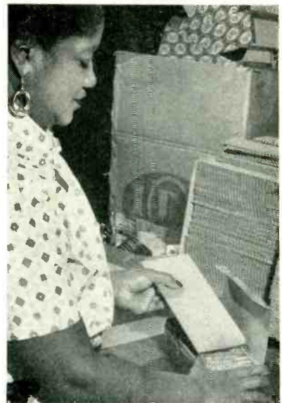
Placing corrugated cardboard over resistors in carton, after having first inserted vertically ribbed strips against ends of resistor leads to achieve pack that will not shift during shipping
