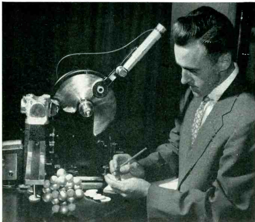
Scientist using X-ray diffractometer, indispensable to ceramics research. Raytheon studies include atomic structure, stress conditions, identification of solid state reaction products, crystal orientation and particle size.
