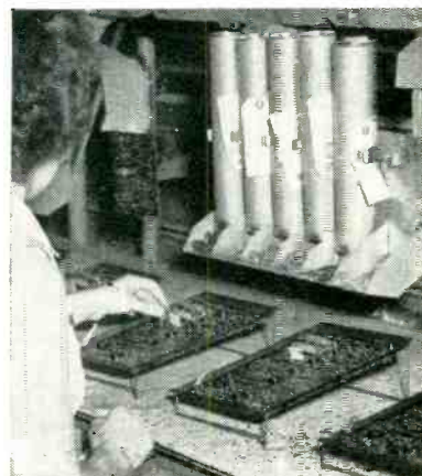
Typical work position on line, showing method of holding cardboard storage cylinders in dispenser bins. Boards are dip soldered without clinching leads
