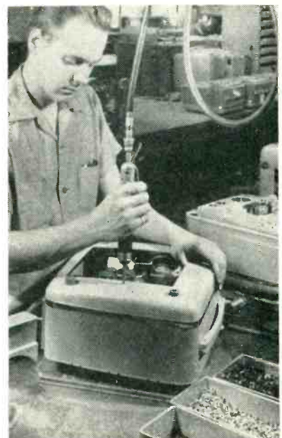
Driving assembly screws in filter units with new magnetic-clutch air tool
