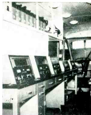
Interior of insulated van showing radio equipment. Rack of portable radiotelephone transmitter-receivers stowed at the upper left
