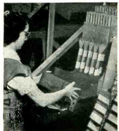
Placing baffle over separator frame
