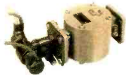
VA-1281 Stalo Cavity with VA-201 klystron
