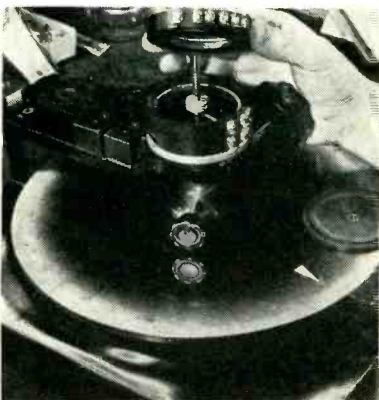
Placing third section on multigang potentiometer being assembled on phasing fixture having large calibrated dial
