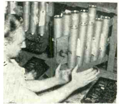
Method of swinging out dispenser frame for replacing cardboard cylinders in rear row. Hand is held over full cylinder as shown when placing in rack
