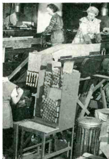
Setup used for achieving perfect alignment of resistors as they are fed into shipping carton. Operator at top distributes incoming batch of 2,500 resistors approximately equally to the five chutes of the loading machine. Operator at bottom removes loaded cartons and puts empties in position
