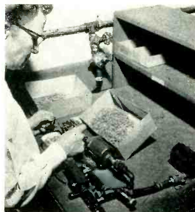
Removing capped resistor from air-operated vise used for assembly
