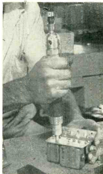
New tool drives screws to optimum tightness in plastic housing of tape recorder, avoiding distortion of housing
