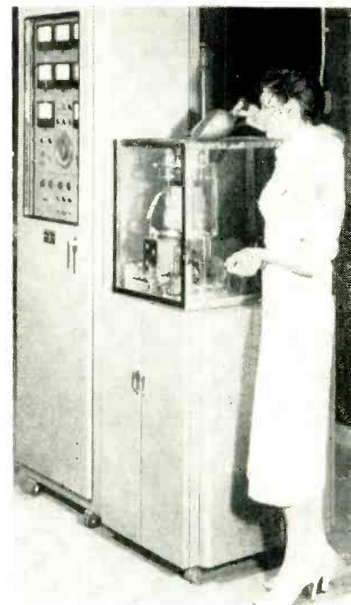
FIG. 7—Automatic inspection device tests 100 cores a minute
