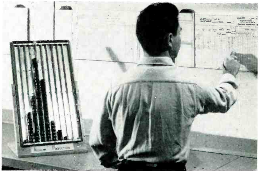
Quality control panel at left, with magnetic recording heads in channels corresponding to test readings, gives data in convenient form for quick transfer to permanent quality control chart on wall
