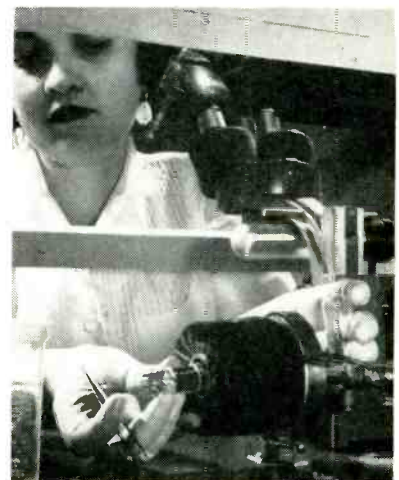
Inserting finished mount in coil for simultaneous demagnetizing and cleaning. Vacuum line is attached to other end of the coil
