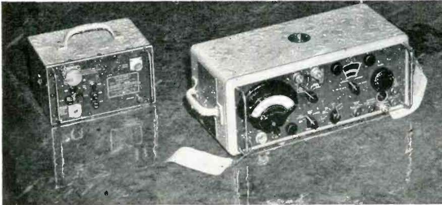
Stoddart NM-10A Radio Interference and Field Intensity Meter* covering the frequency range of 14 kc to 250 kc.
