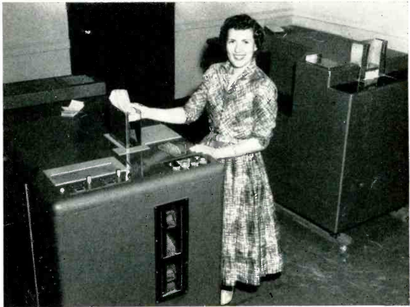
PHOTOELECTRIC reader controls card-punching operation as . . .
