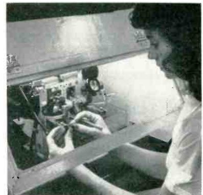
Assembling tube cages under protective hood. Rubber cots worn on fingers are changed every hour. Rubber conveyor belt under hands of operator moves mount along under hood to next operator on the assembly line
