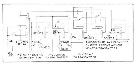
FIG. 3—Wiring d.agram of transmitter control unit. Time-delay relays provide warmup period for transmitter and determine transmission periods. Unit has two controls, one to select desired operation and other to turn equipment on
