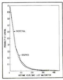
FIG. 1—Theoretical and observed reliability of airborne equipments
