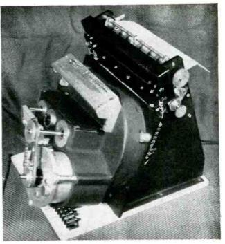
Transmitter-scanner must be solidly constructed to reduce vibration from high-speed operation. Continuous copy at upper right
