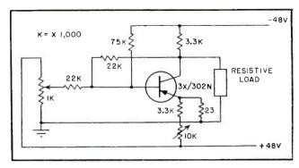
FIG. 5—Experimental high-output power amplifier uses 200-milliwatt pnp junction transistor
