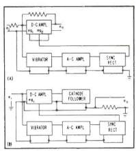
FIG. 5—Alternative stabilized d-camplifier elements
