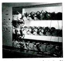
Gear-driven arrangement for testing 24 potentiometers at a time. Eight lamps combined with three-position selector switch permit quick determination of failed unit
