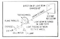
FIG. 1—Fizeau's toothed wheel for measuring speed of light
