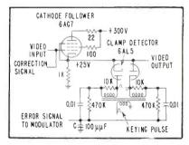
FIG. 1—Diode clamp detector operates from low-impedance source minimizing effect of unbalance between diodes
