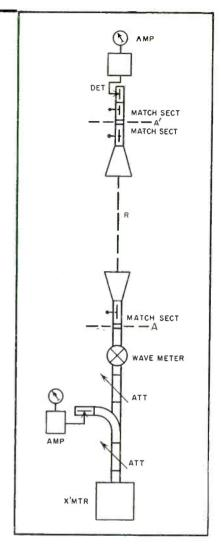
FIG. 3—Experimental setup for gain measurements
