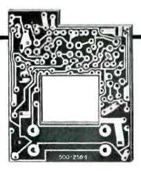
Here's the printed-circuit board used in the Regency . . made with Richardson T-725 copper-clad INSU-ROK. Engineers of I.D.E.A., Inc. of which Regency is a division, laid out the circuit. Croname, Inc.\* Chicago, took it from there ... printed the complex circuit on Richardson T-725 copper-clad INSUROK, then etched it. Results: a lightweight, compact, efficient circuit . . tedious, time-consuming wiring eliminated . . faster assembly.
