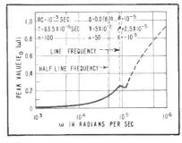
FIG. 3—Clamp circuit response to cosinusoidal signal after initial transient
