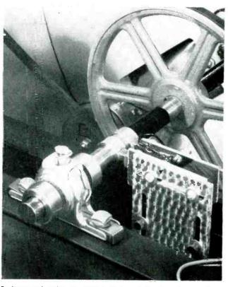
Audio signal is fed to rotating loudspeakers through coin-silver slip rings and silver graphite brushes
