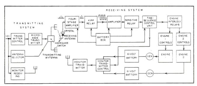
FIG. 1—Block diagram of microwave transmitting and receiving systems of remotely controlled fog alarm
