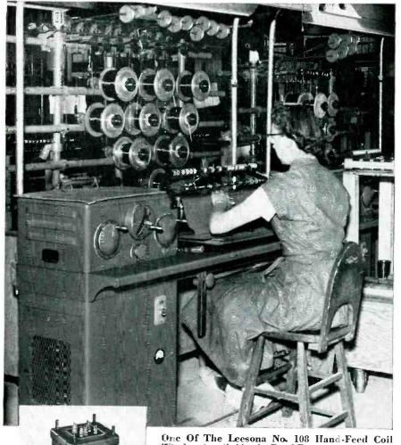
Winders installed by the Freed Transformer Company of Brooklyn, N. Y. Note the convenient location of controls for quick set-up change. Many other features make this the fastest, easiest to operate, most advanced hand-feed coil winder ever designed. Inset shows a Hi-Fidelity Transformer, a typical Freed component in which precision-wound coil structures are vital to high performance and reliability.
