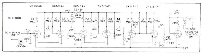
FIG. 5—Receiving unit uses CK512AX subminiature hearing-aid-type tubes to reduce battery current drain
