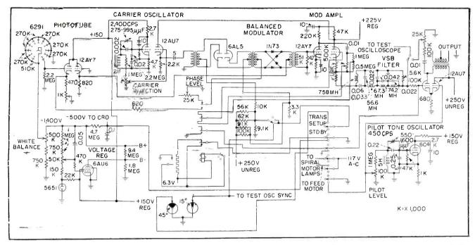
FIG. 3—Scanner amplifier used in system with common power synchronization. Additional subcarrier modulation can be added for remote locations using pilot tone oscillator like that shown to right
