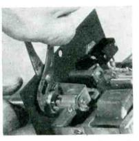
Holding ferrule thread with pliers while removing driving mandrel
