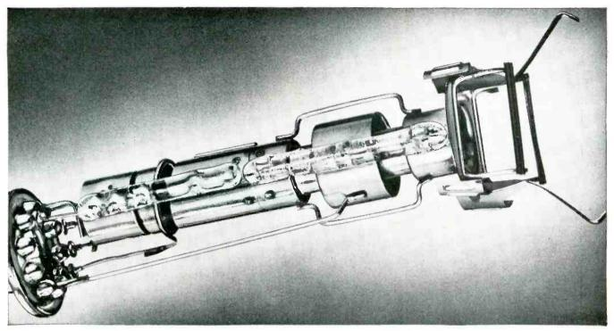
The new Westinghouse electrostatic gun improves picture tube focus, extends tube life, eliminates arcing at high voltages. That's why you can . . .
