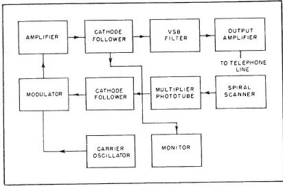
FIG. 1—Elements of the continuous-feed facsimile scanner-transmitter
