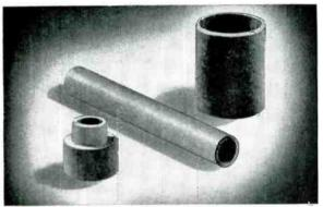
A VERY HARD TUBE is supplied in C-D-F Grade 6A. The parts shown have maximum mechanical strength, lowest water absorption rate under immersion conditions and most stable dielectric loss properties. Fine for bushings and cores.
