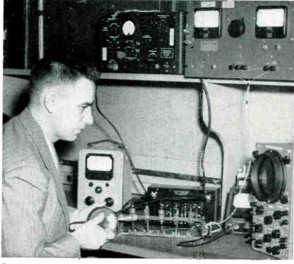
Experimental five-stage 10 to T0-mc all-pass amplifier test setup. Amplifier is shown immediately to right of author's hands
