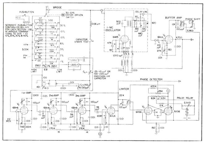
FIG. 3-Modified circuit using 1-mc signal source for sorting low-value capacitors
