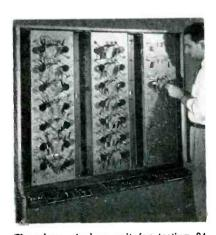
Three-bay, six-door unit for testing 84 units at a time. Metal strips locked in position by wing nuts hold potentiometers in position on doors
