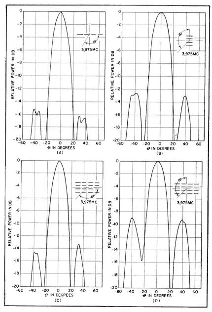
FIG. 10-Radiation patterns for H-plane array (A), E-plane array (B), E-plane pattern of composite array (C) and H-plane pattern of composite array (D)
