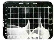
Response of an audio band stop filter with null marker showing frequency of one peak.
