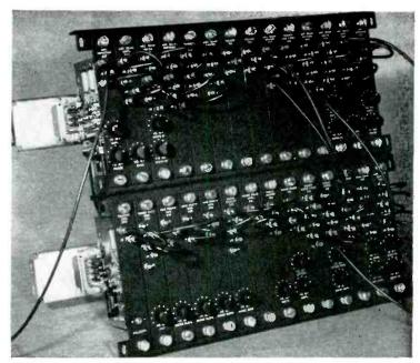
Rack-mounted group of simulator modulars. Unitized construction provides for testing wide variety of radar systems
