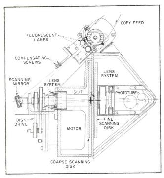
Scanning mirror picks up image from brightly lighted line of copy. Compensating screws equalize effective illumination
