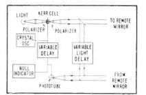
FIG. 2—Diagram shows use of the Kerr cell shutter and variable delay units
