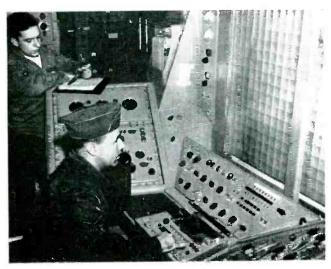
Interior of radar control station (left) from which pilotless jets are made to traverse desired target area. Alternatively, the QF-80 (right photograph) can be flown off the runway by the controller
