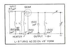
FIG. 1—Circuit of the 6AN4 amplifier stage used to drive power amplifier. Several stages are cascaded to improve bandwidth
