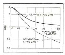
FIG. 2—Gain per stage of conventional amplifier compared with all-pass amplifier
