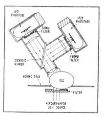
FIG. 2—Fluorescence from egg is split by dichroic mirror for transmission to two filtered phototubes
