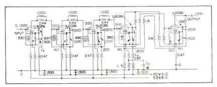
FIG. 4—Five-stage 10 to 70-mc amplifier. Heater and plate voltages are supplied to the tubes through trifilar coils. Capacitances are in  $\mu\mu$ F and inductances in  $\mu$ H
