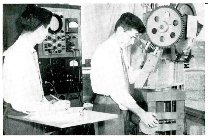
Checking radiation pattern of four-by-four slot array shown in Fig. 1
