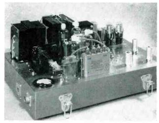
FIG. 4—Microwave transmitter and modulator. Magnetron output tube is mounted on left side of chassis
