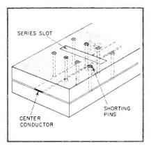
FIG. 2—Series-slot radiating element showing use of shorting pins
