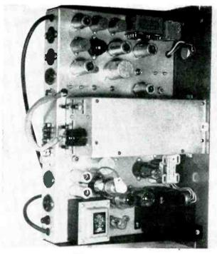
Compact scanner amplifier showing vestigial sideband filter (top) monitor oscilloscope (center) and power supply
