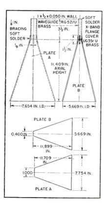
FIG. 2—Typical construction drawing for α gain-standard horn. Plates are made from 0.50 in. sheet brass
