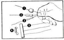
VARIETY OF HOUSINGS available for Vac-u-Sel rectifiers. 1) Metal-clad casing, 2) Textolite tube, 3) Ceramic tube, 4) Nylon tube, 5) Slotted Textolite tube.
