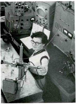
Changing frequency setting of variable oscillator in preparation for checking another point on each of the eleven frequency meters. Frequency counter, scope and other equipment are on table at rear
