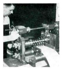
Input end of 12-inch rotary gang slitter as set up for cutting 73/4 inch wide 0.012-inch silicon steel into 5/8-inch
