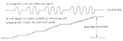
Note that each full cycle produces 2 jerks, and that 10 full cycles produce 1 revolution.
