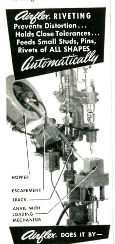
an exclusive, patented principle that combines high frequency blows with spinning action to cold-flow any type of stud, pin, rivet, etc. in any material. Peening tolerances to .002". Rivet capacities of standard automatic machines 1/16" to 1/8", larger capacities special. Also, portable and floor model riveters with capacities up to 5/8" solid steel rivets.
