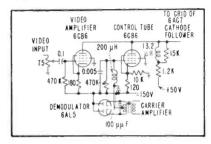
FIG. 5—Demodulator and control tube circuit
