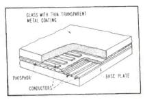
FIG. 2-Construction of phosphor screen
