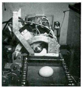
In lowered position, rubber cup on phototube housing rests on egg shell to eliminate outside light
