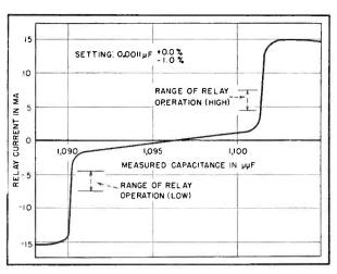
FIG. 5—Current in polar relay of 1-kc bridge when set for tolerance range of 1 percent at 0.0011  $\mu {
