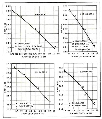
FIG. 4—Gain curves for gain-standard horns in the 8-mm, 1.25-cm, 1.8-cm and 3.2-cm bands. Comparisons of measured gain for hours scaled from one band to another show good agreement
