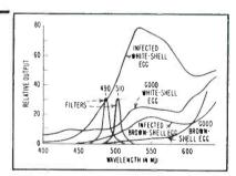
FIG. 1—Spectral response curves of good and infected eggs, with response curves of filters used on phototubes
