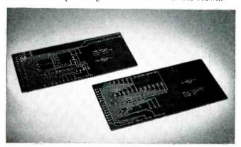
GB-181E COPPER CLAD-GLASS FABRIC WITH EPOXY RESIN The new C-D-F epoxy grade uses a glass fabric laminate with a copper foil surface on one or both sides. Epoxy resin laminates possess very high mechanical strength (tensile and flexural), along with good dielectric strength, both perpendicular and parallel to laminations. Used in
