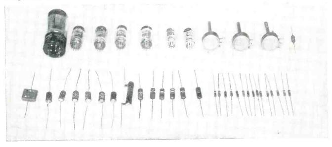
the 40 components of an electron-tube crt deflection system......
