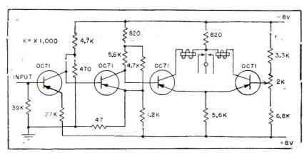
FIG. 1—Transistor servo amplifier with 0.11-watt power drain replaces vacuum-tube counterpart with 25-watt drain
