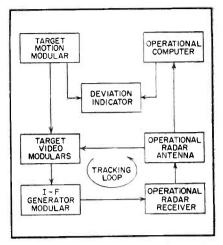
FIG. 1—Typical arrangement for testing radar system
