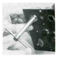
Using ferrule wrench to tighten ferrule of socket
