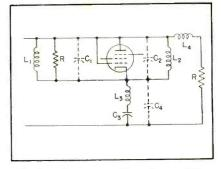
FIG. 3.—All-pass amplifier stage, showing stray capacitance to ground with inductance  $L_k$  inserted in output
