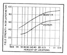
FIG. 3—Percentage of locations that have field strengths greater than ordinate show usefulness of booster
