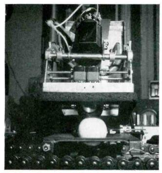
Phototube housing in raised position with cover removed to show placement of components
