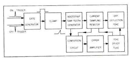
FIG. 1—Commonly used electron-tube system for crt beam deflection
