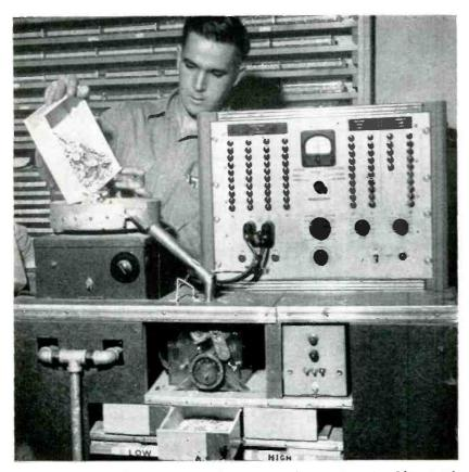
Loading hopper of vibratory work feeder at input of test setup using 1-kc capacitance limit bridge. Disks slide down slanting tube one by one and go through roller-type contacts under table. Four rows of 0-9 buttons at left on panel set capacitance value to four digits. Buttons at right give 0 to 99 percent high limit and 0 to 49 percent low limit for desired tolerance
