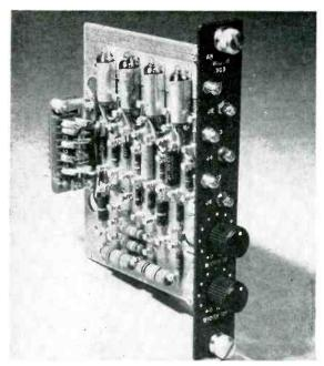
Terminal-board construction is used in modulars, Plug at rear connects unit into system
