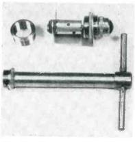
T-handled threaded mandrel used as ferrule wrench, with lamp socket assembly at upper right and the ferrule itself at upper left. Ferrule has flange that bears against front of panel when installed; knurled part of bezel on mandrel tool bears against this flange when tool is installed
