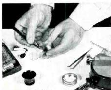
Preparing disc for microscopic examination. On- A microscopic look at disc often provides lead to the-spot examination may reveal acid, alkali, sulfur, soot or other polluting agents peculiar to an area.
