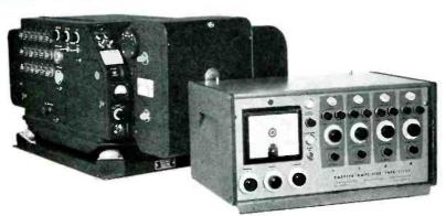
5-114 RECORDING OSCILLOGRAPH... most widely used, most versatile oscillograph in the world today. Either 18 or 26 traces on 7" paper or film. High-speed accessory magazine holds 250 ft. of paper and permits record speeds up to 500"/sec. SEND FOR CEC BULLETIN 1500C-X1.
