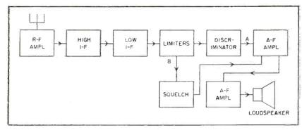
FIG. 1—Conventional squelch operation uses output from limiter circuit to bias off audio in the absence of signal
