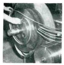
Core plate recoiler being set up for winding twelve %-inch silicon-steel slit strands coming from slitter
