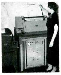
Alden weather map recorder at Logan Airport, East Boston, Mass., produces weather record from continuous roll of paper, making it possible to read copy as it is received.
