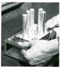
Method of pressing side levers to pry chassis out of jig
