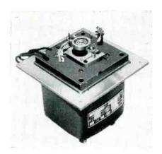
Closeup view of motor-driven switch that switches bridge from high-limit to low-limit standards at rate of 30 times per second to check tolerance
