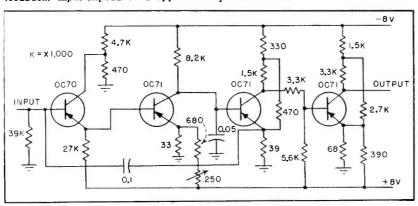
FIG. 3—Direct-coupled amplifier has gain of 25,000 with maximum output voltage of 5 volts into 1,500 ohms
