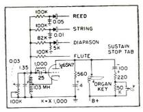
FIG. 2—Sinusoidal output of Hartley oscillator is modified by copper-oxide rectifier circuits to provide four basic tones
