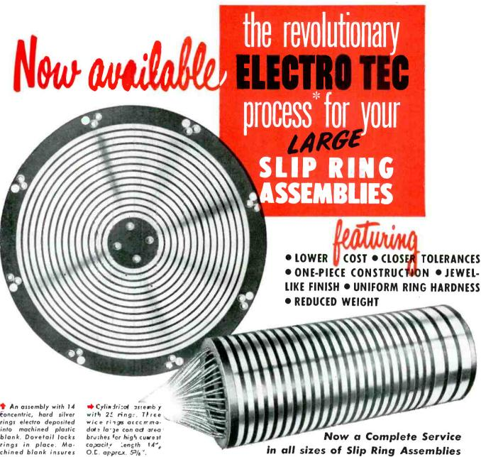
Concentric, hard silver rings electro deposited into machined plastic blank. Dovetail locks rings in place. Machined blank insures accuracy. Diameter approx. 11", thickness approx. 5/16".
