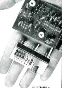
Designs for new Remington Rand ERA computers that are now under development. Upper: general purpose digit register. Lower: packaged transistor logic element.
