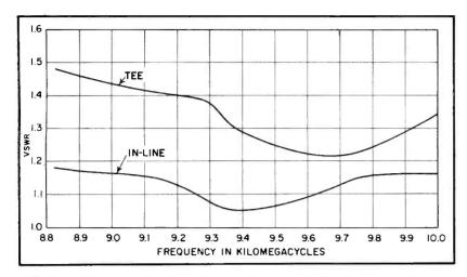
FIG. 5—Frequency versus vswr characteristics of in-line and T junctions
