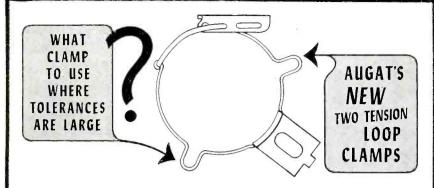
Augat two-tension loop clamps are the long-sought answer for uses where tube base tolerances vary up to .040. The bands of these sturdy clamps are made of Beryllium copper, heat treated to retain original tension and nickel plated to withstand a 96 hour salt spray test with no adverse effect.
