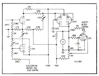
FIG. 4—Direct-coupled amplifier triggers thyratron to reject if ratio of phototube outputs is increased by presence of green rot
