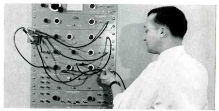
2. 10-minute changeover. Engineer simply connects one new delay unit into the system and sets up controls for new pulse sequence. Units are matched to each other; so no buffers are required. Units connect together through standard cables.
