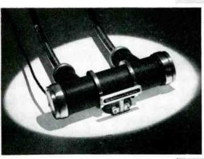
Assembled view of Machlett Dynamax 20-DF rotating anode X-ray tube and mounting.
