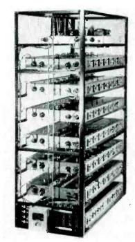
Rack-mounted tone generators can be placed up to 100 ft from console
