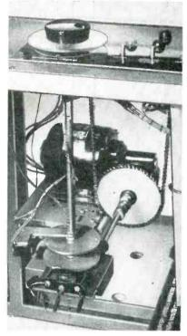
Two cams at bottom control revolutions per cycle. Switch for lower cam is fixed, but switch for upper cam can be rotated around cam by knob on control panel at too
