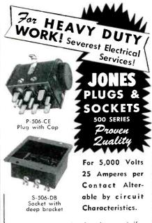
Socket contacts phosphor bronze, knifeswitch type, cadmium plated. Plug contacts hard brass, cadmium plated. 2, 4, 6, 8, 10, and 12 contacts. Plugs and sockets polarized. Long leakage path from terminal, and terminal to ground. Caps and brackets, steel parkerized (rust-proofed). Plug and socket blocks interchangeable in caps and brackets. Terminal connections most accessible. Cap insulated with canvas bakelite.
