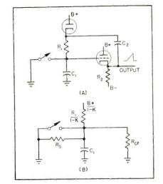
FIG. 2—Bootstrap circuit: schematic (A), equivalent circuit (B)
