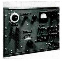
Front panel of 1-mc bridge used for checking low-value disk capacitors. Here only one set of tolerance buttons is used, for 0 to 49 percent
