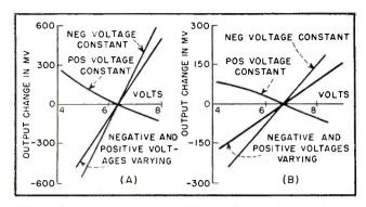
FIG. 4—Change in output of amplifier of Fig. 3 with variation of supply voltages for 68-db (A) and 78-db (B) feedback
