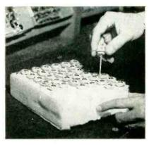
Removing special capacitor from foam plastic shipping block
