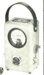
Model 43 with front element in operating position. Dimensions: 7" x 4" x 3" Weight, 4 pounds,
