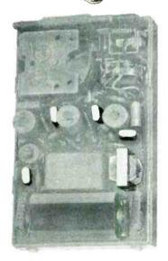
\*With four Texas Instruments grown junction n-p-n germanium low cost, high gain transistors, the Regency radio achieves power gains of 32 decibels in each intermediate-frequency stage and 37 decibels in the audio stage. One transistor is used as a combination mixer-oscillator, two as intermediate-frequency amplifiers, and one as an audio amplifier. Output transformer also TI manufactured.
