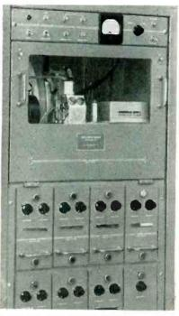
Truck-mounted seismic recorder contains seven dual-channel modulators
