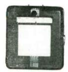
For fast and sensitive recording or controlling one or more points throughout a wide variety of processes. Used originally for temp. ranges of 350-550 Degrees cent. but may be changed for other applications by suitable control units. Control units not incl. with instrument.
