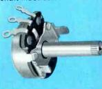
Ear mounted tandem for preset applications. Combines panel space saving features of a concentric tandem with the economy of an ear mounted unit. Available in various combinations of composition or wirewound front and rear sections. CTS type P-C2-45 with composition front and rear sections illustrated.
