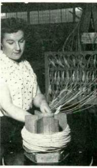
Air motor under bench turns arbor slowly to wind wires for cable as they are pulled off pegs of storage rack in background through holes in vertical plywood board. When winding is completed, operator pulls taped end of cable out from behind paddle board and lifts off the coiled cable
