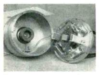
Internal structure of gage. Compensating coil is mounted in cover
