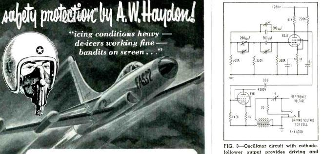
follower output provides driving and reference voltages for pressure gage
