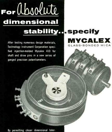
By permitting closer dimensional tolerances, Mycalex glass-bonded mica allows TIC to reduce the size and hold these dimensions constant under toughest environmental conditions. And dimensional stability of the Mycalex coupling arm provides precision transference of rotary shaft motion between adjacent potentiometers without backlash.
