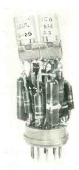
Flip-flop is typical of mountings used in switching-system
