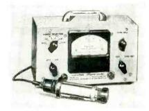
light weight; and a connection for a recorder. It utilizes a sealed radium source that emits alpha particles and produces ionized gas molecules which are collected on a plate to produce a current indidirectly the measured pressure. The gage cannot be damaged by exposure to atmospheric pressure because the ion source operates at room temperature and at zero potential. The Alphatron vacuum gages are less susceptible to contamination than are hot element vacuum gages. The gage is priced at \$425.
