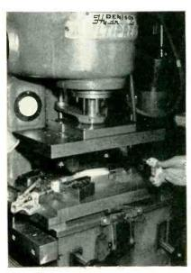
Using light hydraulic press (1 to 6 tons capacity) for punching several holes simultaneously in phonograph pickup
