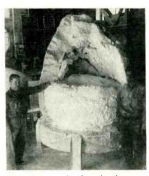
Much larger melts than this four ton pig of crystalline synthetic mica will have to be made before crystals large enough for all uses are produced
