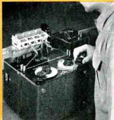
To Check Tracking of Condensers
