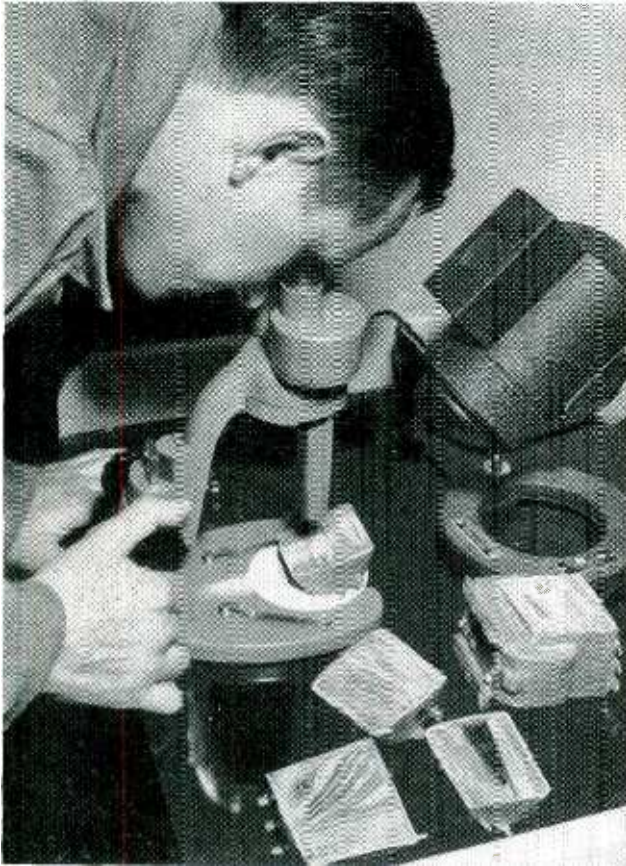
Fig. 3—Section of molded-in-resin transformer is examined under microscope for quality control
