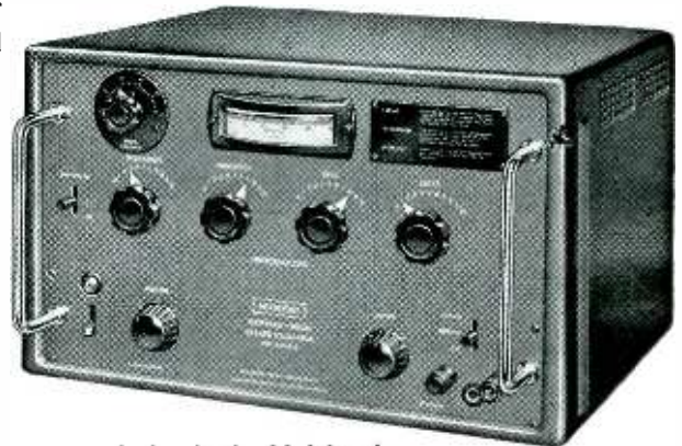
Typical of the best in current design is the Muirhead-Wigan D-650 decade oscillator covering 1c/s to 111,100c/s with a frequency accuracy of \pm 0.2\% or \pm 0.5c/s .
