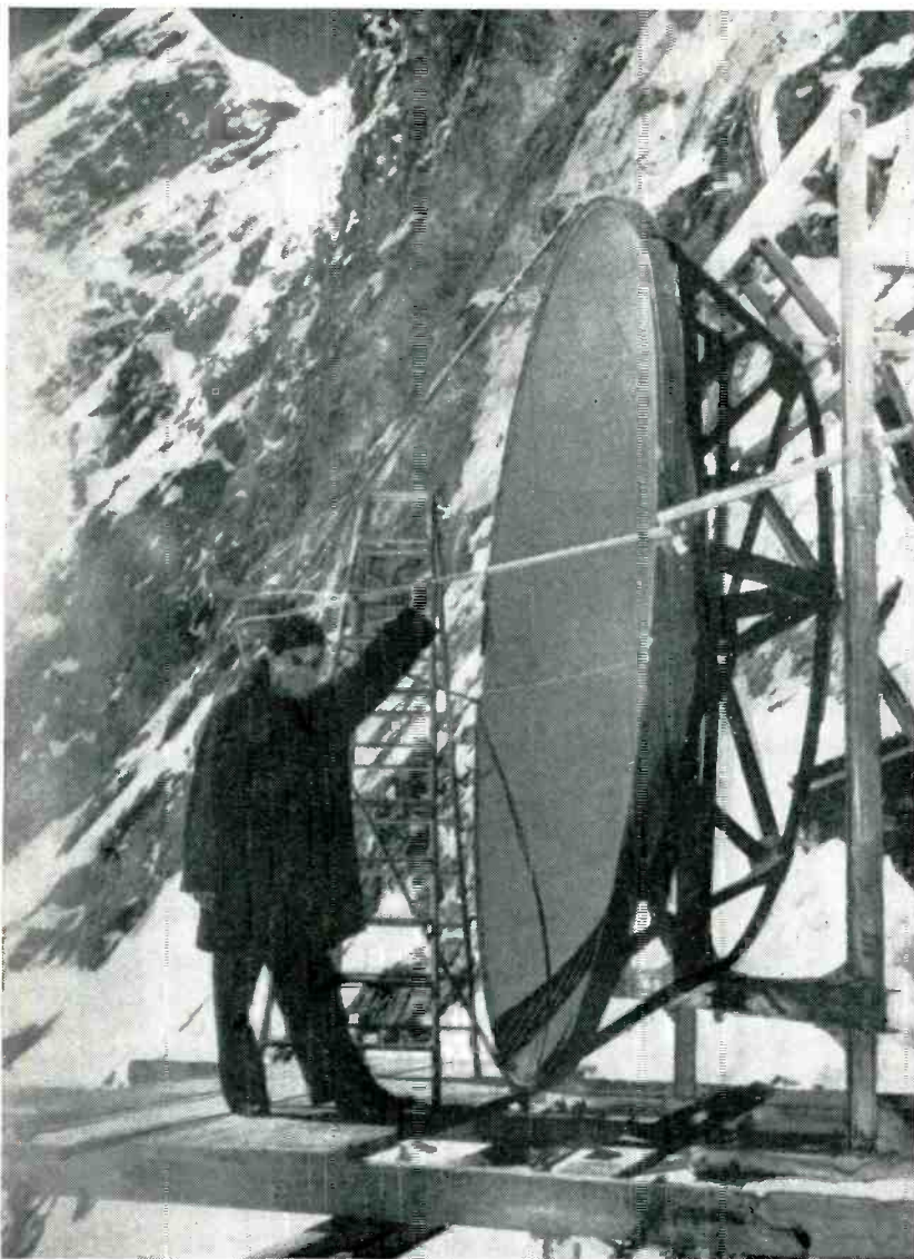
Sole trans-Alpine microwave television link employs antennas like this one, which is mounted on the side of the Jungfrau
