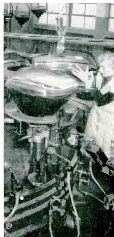
Method of using vacuum lifting aid for loading 27-inch picture tubes into 8-tube automatic sealing machine
