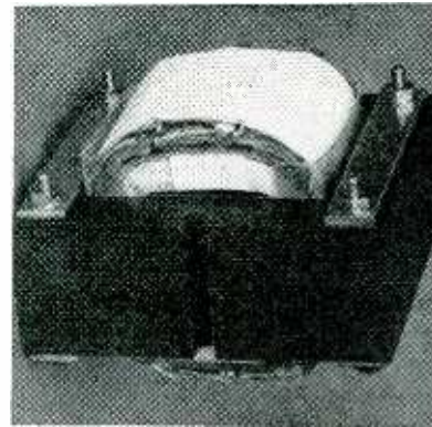
Fig. 9—New materials make small radio and amplifier transformers more compact and improve performance
