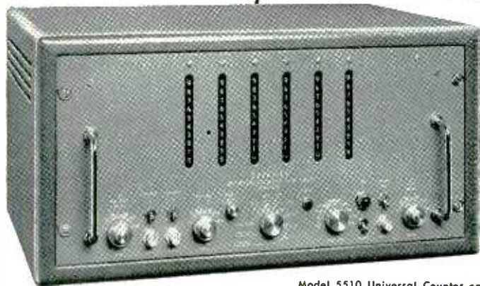
Model 5510 Universal Counter and Timer offers direct-reading digital display of count, frequency or microsecond time interval. Time bases from 1 mc. to 1 cps; gate times from .00001 to 10 sec. Accuracy \pm 1 count, \pm crystal stability (1 part in 10^6 ). Price $1,100.00 f.a.b. factory.
