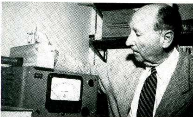
Princeton University research scientist E. N. Harvey uses photoelectric recorder in study of cold light from sea animals at Marine Biological Laboratory at Woods Hole, Mass. Mechanism of light production is being studied in the hope of applying similar principles to artificial synthesis of illumination
