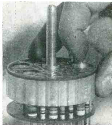
Holding catacomb up against top plate prior to inverting assembly
