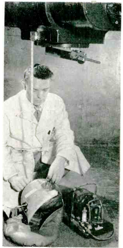
Method of using bag as fixture for supporting x-ray film and tube or other part under industrial x-ray equipment
