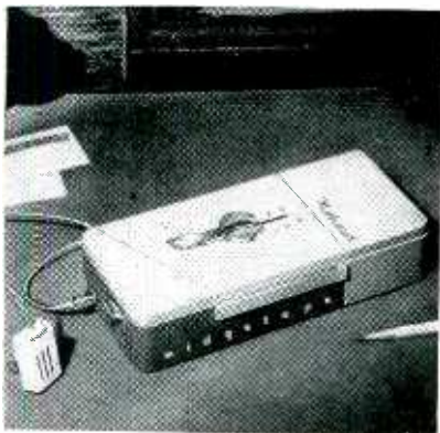
At the New York Audio Fair this Midgetape pocket recorder that utilizes 3 hearing aid tubes and printed circuits was shown
