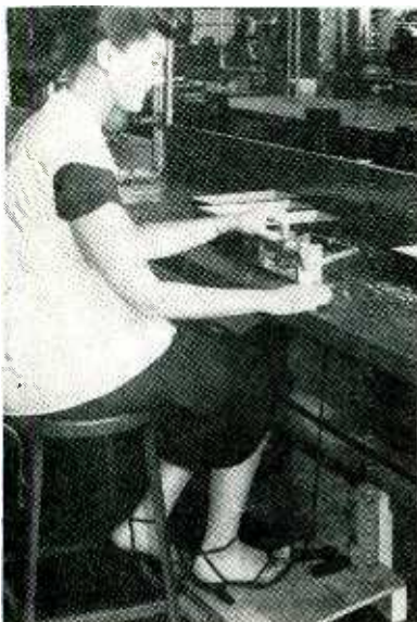
Foot-operated installation of lead-tailoring machine on assembly bench in typical electronic assembly plant
