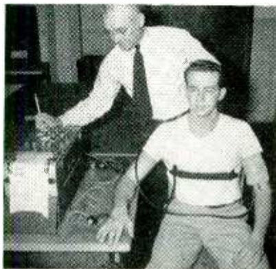
Typical industrial polygraph test setup, using pressure cuff, chest band and wrist electrodes
