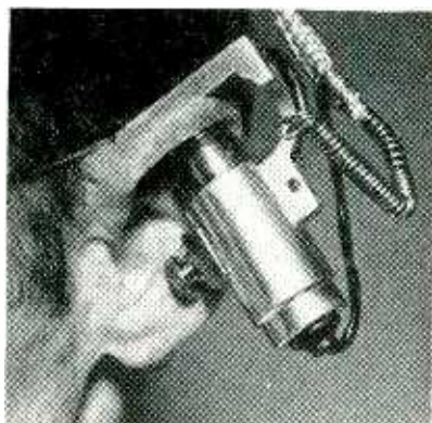
Proposed photoelectric ear clip for monitoring oxygen in blood of suspect to detect lies
