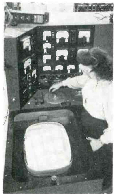
Special test set for picture tubes. Operator swings crank arm on table to 18 different detent positions in turn and observes screen or reads meters
