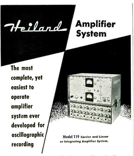
Heiland's model 119 Amplifier System, used in conjunction with Heiland Recording Oscillographs, has received wide acclaim from engineers for its extreme versatility, accuracy and simplicity of operation in the amplification of static and dynamic current phenomena.
