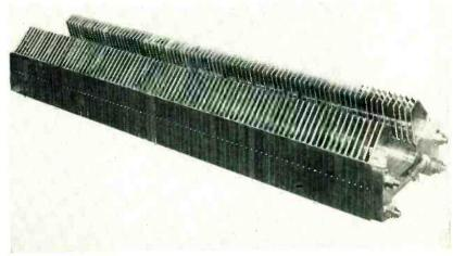
Water-cooled stator of 3,600- $\mu\mu$ f capacitor is mounted in a vacuum with other parts of cyclotron r-f system
