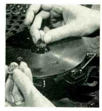
Miniature stem die bends some or all of the nine wires to correct specifications in one operation
