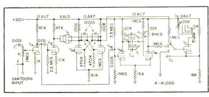
FIG. 3—Swith  $S_2$  provides mode 1 operation in position 1 and mode 2 in position 2. Potentiometer  $R_2$  and  $S_1$  with  $C_2$ ,  $C_3$ ,  $C_4$  (2 0.2, 0.05  $\mu$ F respectively) permit the dwell time of the contacts to be varied from 5 sec to 16 millisec
