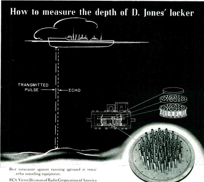
RCA Victor Division of Radio Corporation of America uses the phenomenon of magnetostriction to send and receive supersonic pulses and so determine the distance to a submerged object on the ocean's floor.
