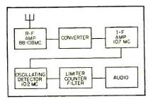
FIG. 5-Block representation of improved receiver using commercial tuner
