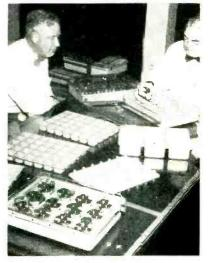
Examples of molded plastic inserts used with containers. Standardized styles were carefully selected to accommodate future components as well as those now in production
