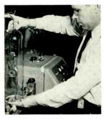
Placing helium-filled bell jar over magnetron sealed into vacuum line of mass spectrometer type of leak detector
