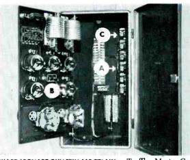
WARD LEONARD BULLETIM 110 EELAYS in Trafflex Master Controller are used for: A. Automatic selection of one of five timing cycles. B. Operation of pilot lights indicating which of three timing dials in Trafflex Secondaries is in use. C. Remote control of off-duty flashing amber and remote control of signal shut-down for entire system.
