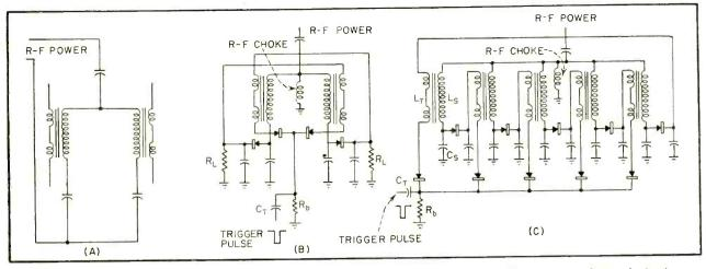
FIG. 1—Basic flip-flop unit (A) can be triggered as shown in (B). Five stage ring counter (C) shows simplicity of circuit
