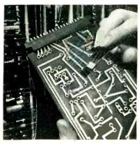
Phenolic plates with circuits etched in advance eliminate elaborate wiring and permit cheaper soldering methods for new rural-line carrier equipment that also includes transistors of the type shown
