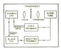
FIG. 1-Image feedback system produces desired type pattern on slave oscilloscope
