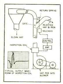
FIG. 1-Iron detector system
