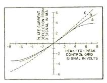
FIG. 6—Demodulator characteristics of 6AS6 (A) and beam-deflection tube with 0-signal cathode current of 10 ma (B) and 16 ma (C)
