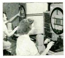
Checking grids with contour projectors. Operator at left is using calibrated enlarged glass scale to measure departure of grid from tolerance on minor diameter. Screen charts for other types of grids are stored in rack between the two projectors
