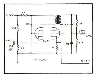
FIG. 3—Alternate plug-in pulse-generator circuit can be used when low power consumption is important
