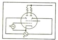
FIG. 1—Schematic representation o beam-deflection tube
