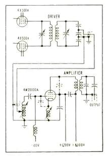
FIG. 1-Circuit of 25-kw amplifier showing coupling methods used
