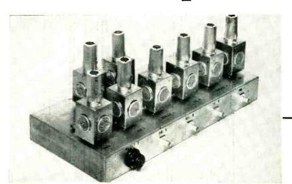
Multipulse generator using eight plug-in units. Controls for all units are brought out to main chassis
