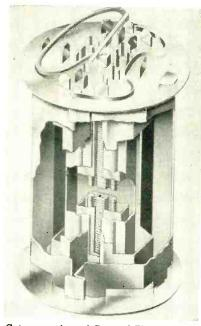
Cut-away view of General Electric 6AR8 beam-deflection tube
