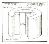
FIG. 3—Coining die used for anode blocks
