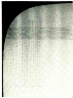
Television raster (left) displays unique appearance of horizontal deflection coil unbalance. Enlarged section of same raster (right) has scan lines emphasized and shows magnetic field lines
