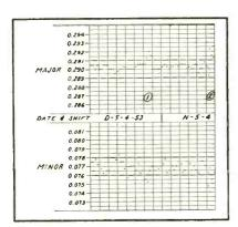
Portion of typical plot of grid-lathe performance when winding 6CB6 control grids. Major diameter was over specifications at 1 and immediately corrected. At 2, major was over specification and minor was under specification
