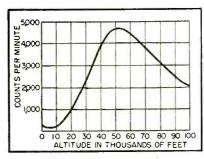
FIG. 4—Representative radiation curve obtained in flights at a latitude of 28-deg north
