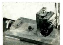
Close-up of tube holder, with pendulum resting at point of impact
