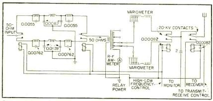
Antenna tuning unit includes low-pass filter, variometer and tap tuning as well as relay controls to change frequency
