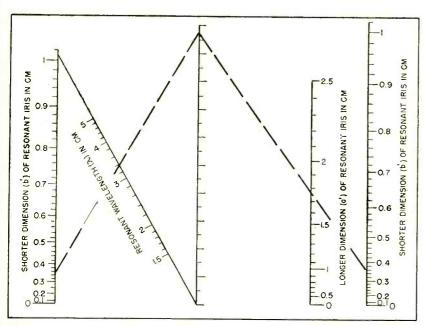
FIG. 4—Nomograph for determining iris dimensions for a waveguide 0.900  $\times$  0.400 inch (2.286  $\times$  1.016 cm)
