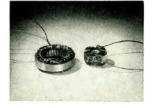
input to the synchro is 26 v, 400 cps. Stator output is 11.8 v. Input power when loaded with one control transformer is 0.973 w and sensitivity at control transformer output is 397 mv per deg. The synchro reflects to its shaft no measurable cogging effects or mechanical loading. Outline drawings, mounting information, complete characteristic basic data and typical error curves will be mailed on request to the company.
