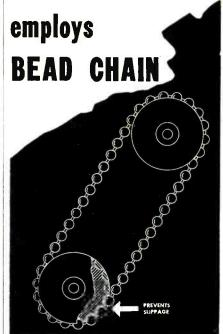
Because of its unique characteristics, Bead Chain is frequently employed by alert designers to make a simple, low-cost and highly efficient sprocket drive. Ideal for many products, it has been proved on business machines, television tuners, venetian blinds, etc. Slippage is absolutely prevented as each bead fits into an individual pocket.
