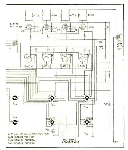
Final stage uses eight type 807 tubes in push-pull parallel
