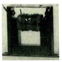
Push-pull output transformer couples type 807 amplifier into unbalanced 50ohm impedance
