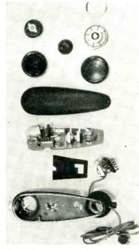
Exploded view of portable transceiver
