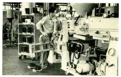
ONE MACHINE produces 200 7-inch or 70 12-inch records per hour when .
