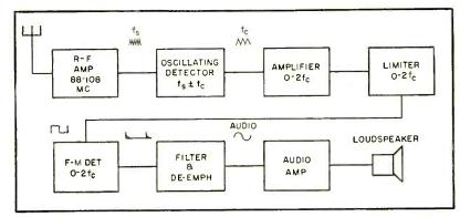
FIG. 2—Block diagram of simple receiver in which  $f_s$  is signal frequency and  $f_c$  the center frequency or half the widened bandwidth
