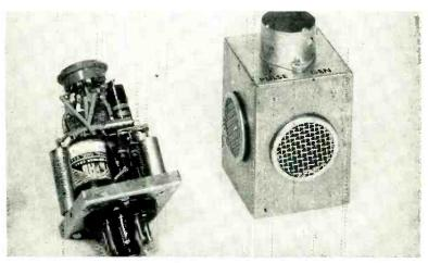
Plug-in unit with case removed. Octal socket makes connections to main chassis and socket at top accepts miniature tube
