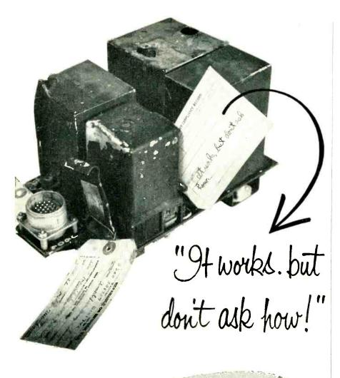
That's what the Tech Sergeant wrote after inspecting this Servomechanisms, Inc. electronic computer that came out of a wrecked fighter in Korea.
