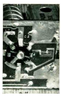
Appearance of panel after dip soldering at 425  $\Gamma$  in 60-40 solder. Gaps up to 0.008 inch can be bridged by the solder
