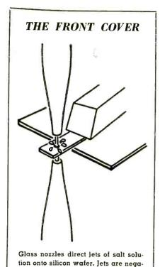
metal salt serve as the cathodes. The silicon atoms under the jets go into solution as atomic sawdust.
