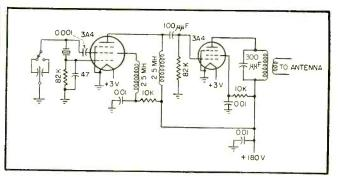
FIG. 2—Schematic and picture of altitude transmitter. Pressure sensitive capacitors at input are alternately switched to created frequency difference indicating altitude
