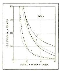
FIG. 2—Path A propagation at 55 mc over sea water. Dashed lines show computed values; free-space (F), horizontal (H) and vertical (V) polarization
