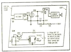
Circuit of gun (below) and relay actuator for gunshot generator in receiver detector output, surrounded by loop
