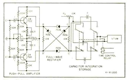
FIG. 1—Bioelectric integrator includes push-pull voltage amplifier using two pnp junction transistors with base input
