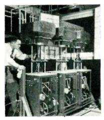
Tipping off picture tubes as they emerge from exhaust oven. Metal clam shells protect tubes from plant drafts that might cause strains in glass walls
