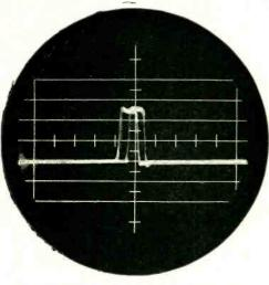
Figure 1. Unique modulating fidelity of -hp-490A is shown in double-exposed oscillogram of 0.1 µsec pulses. First pulse (applied by -hp-212A Pulse Generator) is modulating pulse having rise time of 0.02 µsec; delay through tube approximately 50 millimicroseconds. Second pulse is rfoutput; note absence of deterioration.
