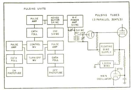
FIG. 2—Pulser circuit turns oscillator on and off to accelerate particles during descending part of the f-m cycle
