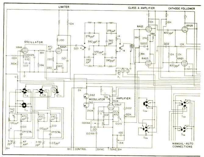
Low-frequency transmitter complete with band-switching and other controls
