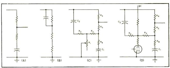
FIG. 1—Low-frequency (A) and high-frequency (B) boost circuits are combined to obtain combination boost circuit (C). Basic tone-compensation control (D) uses triode plate resistance as arm of T-pad
