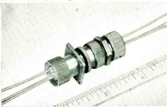
TITEFLEX CONNECTOR—lightweight, corrosion and moisture resistant with temperature ranges of  $-65^{\circ}$ F. to  $+400^{\circ}$ F. This connector's insulation properties will permit 3500 volts at sea level, 1200 volts at 50,000 feet altitude. Connector is available with 2 or 3 pins. 7 amperes. Weight  $\frac{3}{2}$  of ounce. Size  $\frac{2}{1}$  in length.
