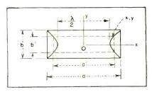
FIG. 3—Sectional view of rectangular waveguide
