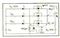
FIG. 3—Equivalent circuit used in calculating power requirements
