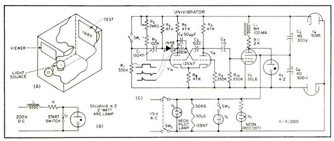
FIG. 1—Example of tachistoscope construction, simplified diagram of arc-lamp control system and complete control circuit
