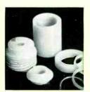
Nylon is drilled satisfactorily with ordinary twist drills. To obtain a smooth hole of uniform diameter, use a slow, uniform feed with the highest speed that will not cause "gumming" or burning. Keep holes chip-free by removing the drill from the hole frequently.
