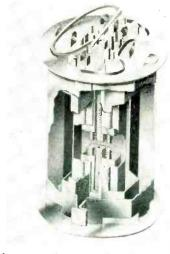
chronous detector circuit include low oscillator injection power requirements freedom from the spacecharge coupled effects which are present in dual-control pentodes and heptodes, linear output voltages, insensitiveness to variations in oscillator amplitude over a wide range, and a high ratio of plate to accelerator current. Complete technical information is given in six catalog pages designated ET-T840.
