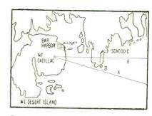
FIG. 1—Unobstructed path A compared with path B over knife-edge used for diffraction observations
