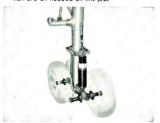
In shock struts The landing gear pistons on some of our largest planes are made of Synthane. Properties of light weight, toughness, durability and shock resistance were needed; Synthane supplied them.
