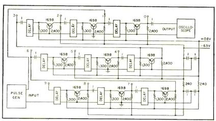
FIG. 4—Nine-section transistorized delay line using cascaded distributed-constant sections of 7.8- $\mu$ sec delay each
