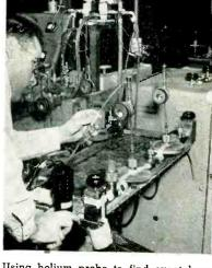
Using helium probe to find exact location of leak in magnetron after bell jar indicated that leak was present
