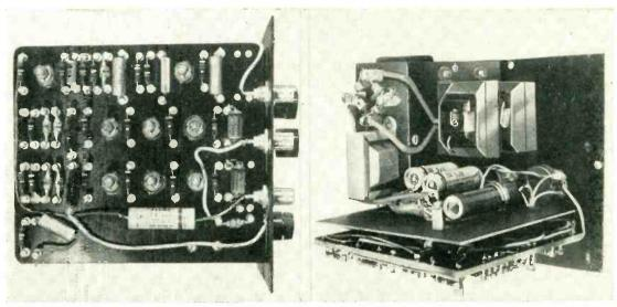
Bottom and rear views of complete pulser. Power supply with diode bridge is mounted on back of panel
