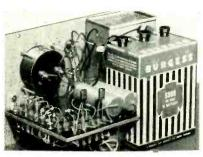
Integrator permits quick change of resistors to match transistor characteristics
