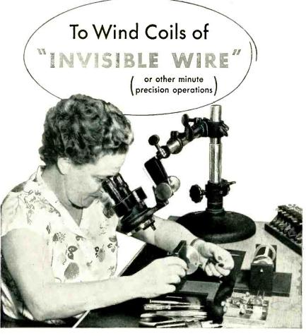
At the Hathaway Instrument Company, tiny galvamometer coils are wound with wire so fine that it is almost invisible to the unaided eye. Ingenious tooling and use of an AO Stereoscopic Microscope assure fast, precise workmanship.
