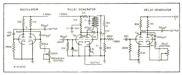
FIG. 1—Oscillator, pulse generator and delay generator circuits have power supply, input and output leads connected to pins of plug-in socket. Frequency and delay-time control potentiometers are mounted on main chassis
