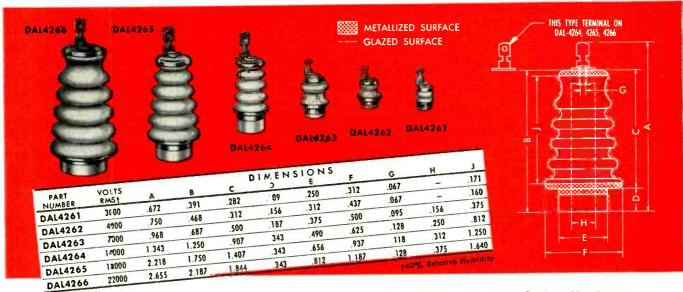
These terminals are made of glazed Alumina Ceramic. Lugs and eyelets are hot tinned brass and metallized areas are silver fired on ceramic, copper electroplated and tin fused for soft soldering. Immersion in 60/40 solder at 450°F for 1½ minutes for dip soldering will not injure the metallic coating. For complete information and quotations call, write or wire today.
