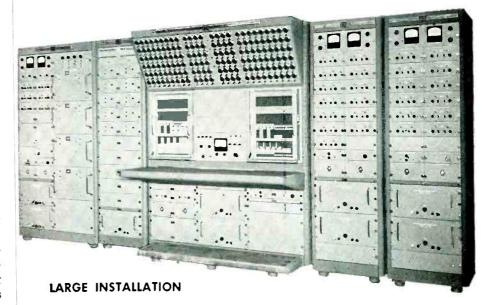
This large computer is used for the rapid solution of aero-dynamic problems. It consists of 50 operational amplifiers, 10 servo multiplying channels, 4 resolving channels, and a control console with two pre-patch bays, 156 attenuators, two
