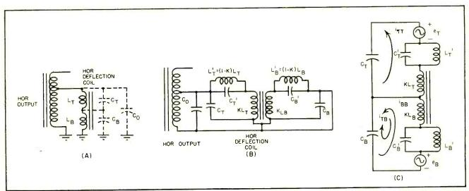
FIG. 1—Simple circuit of horizontal-deflection coil (A) is redrawn (B) to show leakage tuned circuits. Equivalent circuit (C) illustrates how coil balancing cancels ringing currents
