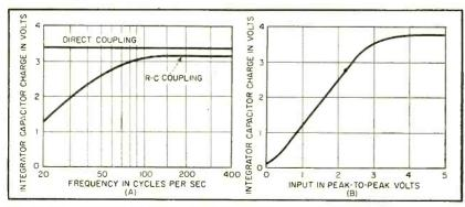
FIG. 2—Characteristics of direct and R-C coupling to transistor amplifier (A) and integrator capacitor charging characteristic (B)
