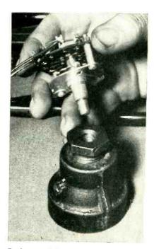
To load switch in pipe-nipple holding jig, operator inserts the assembly and gives it a clockwise spin
