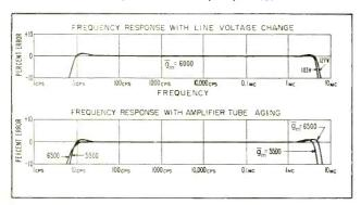
Fig. 1. Typical variation in accuracy with line voltage changes and mutual conductance changes (geometric mean value of the four amplifier tubes).
