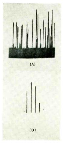
FIG. 1-Scope presentation of 88 pwm channels (A). Commutation system permits viewing selected groups of channels (B)
