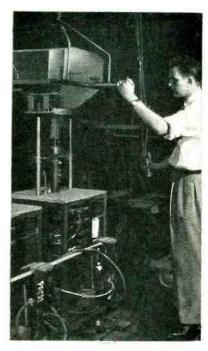
Lowering protected picture tube onto exhaust cart with overhead hoist having a fork-type lift
