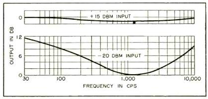
FIG. 3—Response of amplifier to different input signal levels
