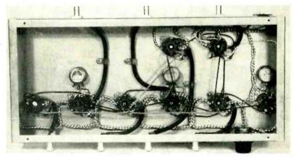
Wiring of main chassis is simplified by plug-in construction. Potentiometers control
