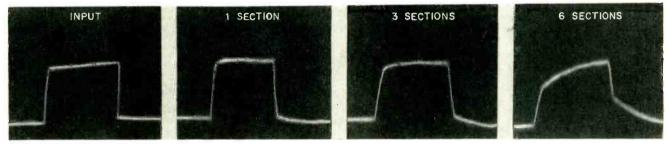
FIG. 2—Pulse distortion is reduced by inserting parallel resistance between delay line sections
