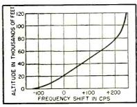
FIG. 3—Altitude-transmitter frequency shift as a function of altitude
