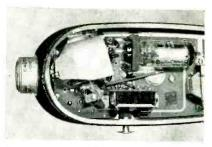
Switching assembly detail, tuning control and tuning loop
