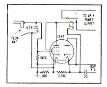
Safety interlock disconnects main power supply when water flow falls below 3 cc per sec
