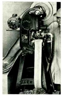
Precision gasket-punching machine in operation. Air blast from vacuum cleaner, acting through pipe at front of press, blows finished washers into hopper at rear of machine
