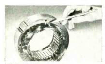
"Mylar" film used to insulate this motor stator is about half as thick as the material it replaces.
