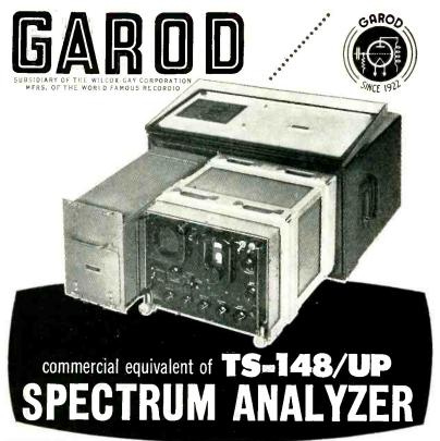
ELECTRICAL DESCRIPTION—The Spectrum Analyzer, a self contained portable unit, is a very sensitive microwave receiver whose output is displayed on a 3 inch cathode-ray The analyzer employs a resonant cavity type frequency-meter calibrated to read directly in megacycles, a frequency-swept (Velocity Modulated) R-F oscillator, a crystal mixer and associated plumbing, narrow band I-F amplifiers, and both regulated and unregulated power supplies.
