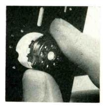
Inserting special snap-in socket into keyed hole in panel
