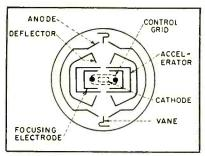
FIG. 2—Cross section showing location of beam-tube elements
