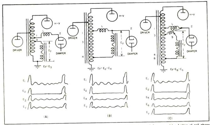
FIG. 4—How deflection coil connections cancel ringing: normal position (A) fails to make use of damper; raising bottom of coil above ground is intermediate step (B); clean waveform results when balance is achieved (C)
