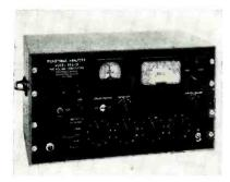
resistor up to a power rating of 1.5 w can be determined down as low as 0.0002 percent per volt. Voltage across the measured resistance is continuously variable in two ranges from 0 to 500 v by a self-contained regulated power supply. Sensitivity of balance is within 0.04 percent on all ranges. It is designed for 115-v, 60-cycle operation.
