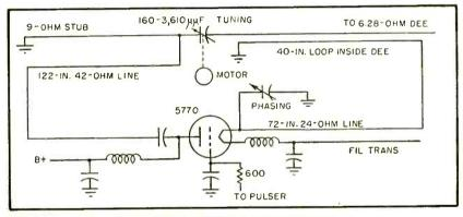
FIG. 1—Sweep-frequency oscillator generates 40-kw r-f signal
