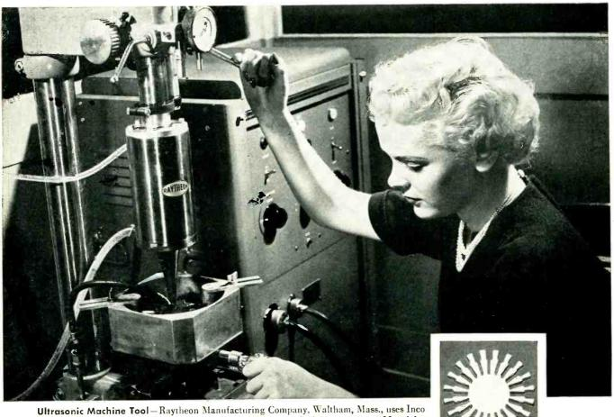
Nickel to keep its magnetostrictive transducer working; tough, fatigue-resisting Monel for the toolholder; chromium-nickel stainless steel for the transducer housing. A pattern Raytheon's UMT can cut in tungsten carbide is shown at right.
