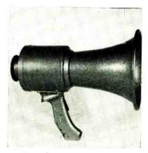
rounding noise conditions. Outstanding feature is the virtual elimination of acoustic feedback. The present unit is completely self-contained with batteries and 3-stage vacuum-tube amplifier in the main housing. It is small and light, only weighing slightly over 5 lb, and being just over a foot long. The form-fitting handle incorporates a press-to-talk trigger switch.
