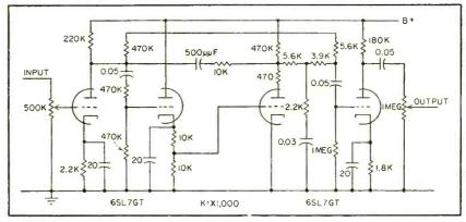
FIG. 2—Audio-frequency voltage amplifier incorporating tone-compensation control
