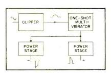
FIG. 1—Positive and negative output stages are separate in pulsing unit
