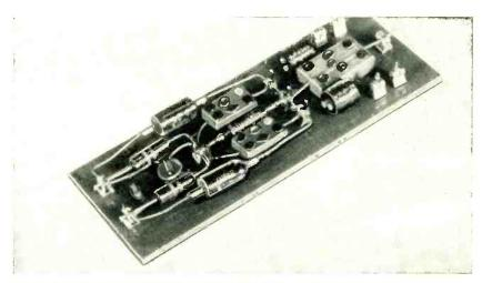
Complete ferroresonant flip-flop unit with coupling capacitor and diodes
