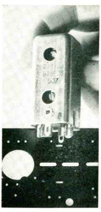
Method of inserting etched i-f transformer in etched video amplifier panel. Wiring is on other side of panel
