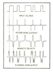
FIG. 2—Waveforms in pwm recorder. Trailing edge of output pulses coincide with leading edge of input pulses
