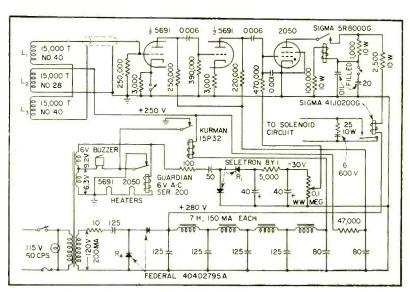
FIG. 2—Circuit of detector, amplifier and control system
