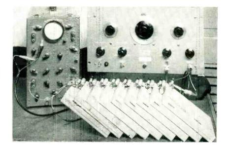
Test setup of  $70 \cdot \mu sec$  delay line with transistors and coupling capacitors mounted on top of delay-line sections
