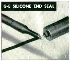
1. Solder right up to the case with new G-E silicone end seal—no need to waste 1/4 inch of valuable space because of danger of cracking glass.
