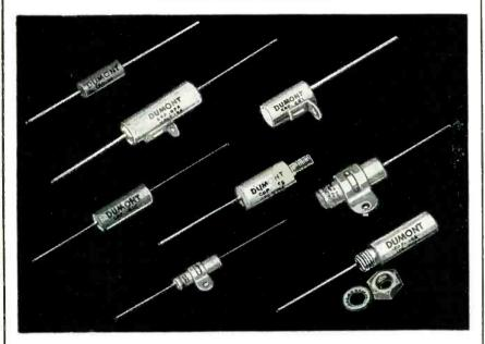
MILCAPS are subminiature paper capacitors hermetically sealed in tinned brass tubular cases. Perfect enclosure of the impregnated paper sections is achieved by the use of glass-to-metal solder seal terminals. MILCAPS are recommended for all applications where size is a primary consideration . . . and are available in any one of the following impregnants: Stabilized Halowax (85° c): Mineral Oil (85°c: or Duroil (125° C).
