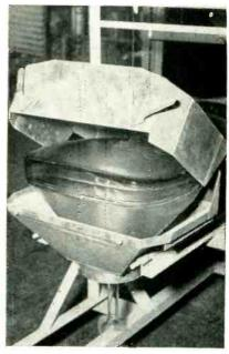
Clam shell metal housing for picture tube. The two latches lock over studs on the lower part when the cover is down
