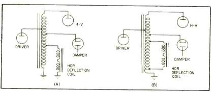
FIG. 3—Cancellation of ringing results when deflection coil is raised electrically from its normal position (A) to new balanced position (B)
