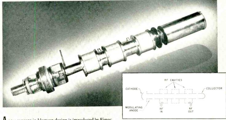
A new concept in klystron design is introduced by Eimac with the X557 modulating anode klystron. An insulated modulating anode placed between the cathode and drift tube section permits:
