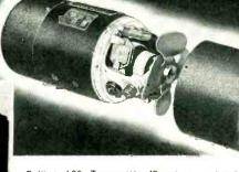
Collins 18S Transmitter/Receiver, extensively used for reliable HF communications in major air-lines and executive aircraft uses a Winco-Engineered Frame 51 Dynamotor.
