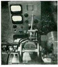
Setup for running in the tuning mechanism of a five-band oscillator by rotating the tuning dial 20 turns in each direction alternately. Clutch-reversing solenoids are at left
