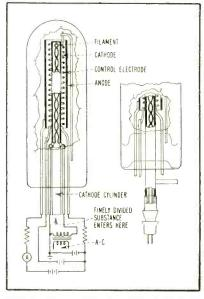
FIG. 1—Vapor detector tube (left) and alternative embodiment (right)
