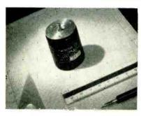
DALMOTOR Co., 1329 Clay St., Santa Clara, Calif. Rated for continuous duty with an output frequency of 20 cps and a maximum of 3-percent harmonic distortion, type 44A generator is recommended for instrument indicating and other similar applications. Voltage is linear with speed, and the unit develops 33 v of 2-phase a-c at 4,500 rpm. Internal
