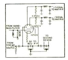
FIG. 5—Demodulator circuit using beamdeflection tube
