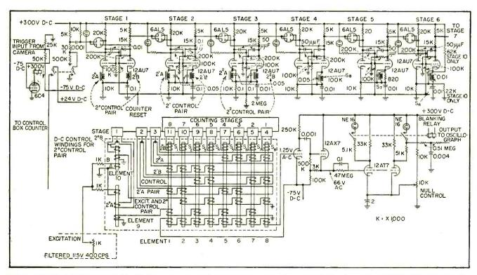
FIG. 3—Schematic diagram of electronic binary counter with magnetic-matrix switch readout. Unit is used in flight-testing airborne fire-control equipment
