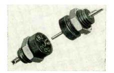
pact strength and arc resistance; and Diallyl Phthalate (blue) with high dimensional stability plus excellent dielectric properties. Precision-machined socket and pin contacts are of spring temper phosphor bronze and brass respectively, gold plate over silver giving low contact resistance and ease of soldering.
