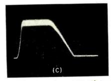
FIG. 2—Step-function response of servo system in mode 1 operation (A). Output of reversible-phase magnetic amplifier with input switched between two different values in mode 2 operation (B). Instantaneous speed of low-inertia servo motor under load with input switched between zero and maximum in mode 2 operation (C)
