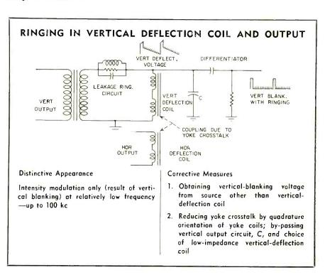
modulation of the electron beam causing successive localized bunches of beam current at the screen. The resulting brightness variation is more discernible than the resulting geometric distortion.
