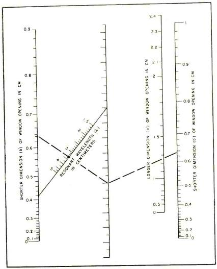
FIG. 6—Nomograph for determining resonant wavelength of sandwich-type ceramic output windows for a waveguide 0.900 imes 0.400 inch with  $\epsilon_r=6$
