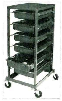
Roller-rack dolly for transporting plastic containers. Runners eliminate dust-catching drawbacks of conventional shelves. Runners can be moved up or down on vertical slides by loosening screws to accommodate different depths of containers used for various sizes of parts
