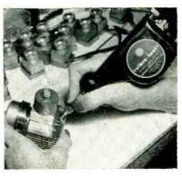
Writing serial numbers on magnetron cavity assembly with vibrating tool
