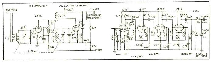
FIG. 3—Simple receiver using single r-f amplifier, oscillating detector, triple limiter and counter detector
