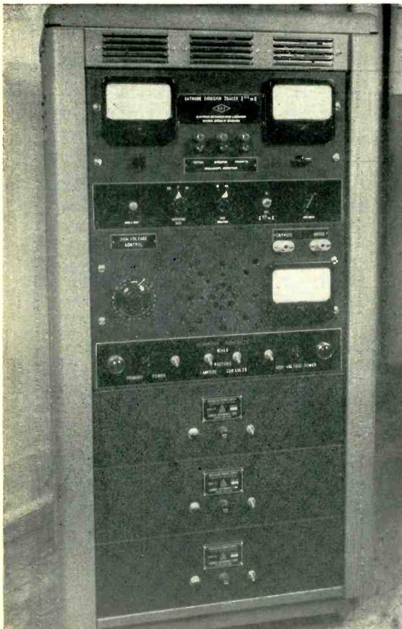
Complete emission plotter as used in NBS vacuum-tube laboratory
