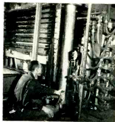
Regulating pressure and heat input to laminating press used for curing
