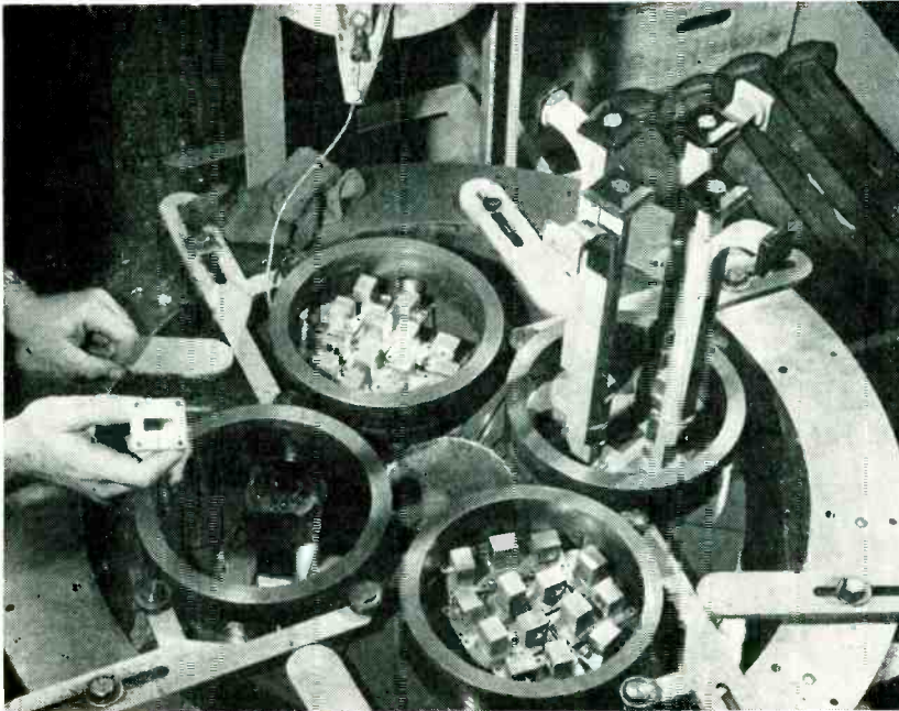
Surfaces of directional couplers and various sizes of waveguides are finished on revolving lapping table. At left a 5-lb lead weight speeds lapping; smaller lead weights are banded onto the couplers (right rear) as counterbalances. A cut-out jig holds the couplers in position
