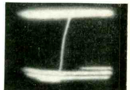
FIG. 3—Coil-discharging circuit. Current-discharge waveform, above, becomes steep, right, when discharge tube is employed
