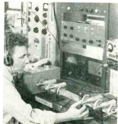
Operator is here adjusting micrometer of one of the five frequency meters being calibrated simultaneously
