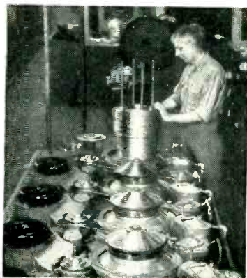
Wire is drawn on this Sylvania machine from .100 to .040 inch diameter.
