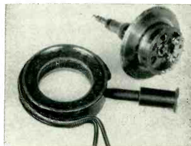
Internal structure of carcinotron. Periodic anode structure can be seen in circular housing
