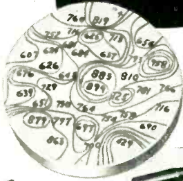
These rough contours of equal attenuation through the sample indicate lack of uniformity in the sample.
