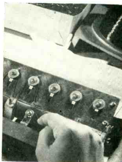
Method of loading five-at-a-time jig for winding single-turn vhf coils that will later be bent around coil form to serve as a bifilar inductance. Operator pulls wire off spool on bench
