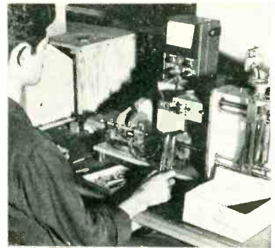
Automatically-controlled spiralling machine for deposited carbon resistors. Pitch of spiralling is changed by turning hand wheel at top of pitch change box at right
