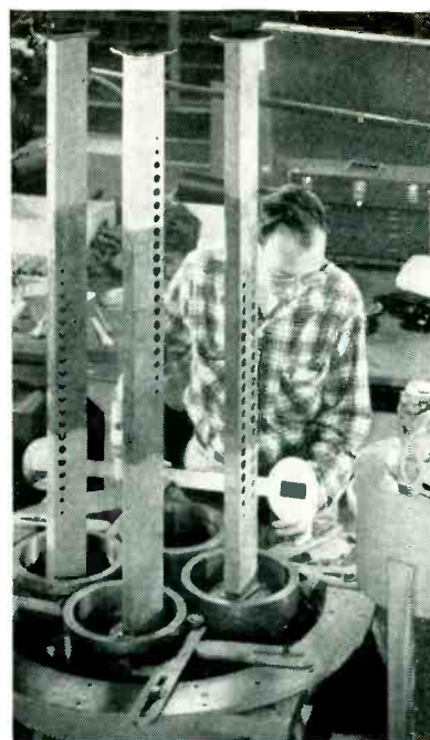
Revolving lapping table gives slightly convex surface to waveguide flanges. Workman makes visual check on progress of finishing operation. Abrasive is suspended in oil in tank at right, and is fed to the table surface via a wire by surface tension
