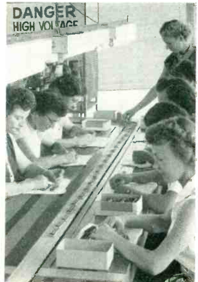
Operators fill Transite trays with terminal assemblies and place the trays on the conveyor belt for automatic transport through the induction furnace
