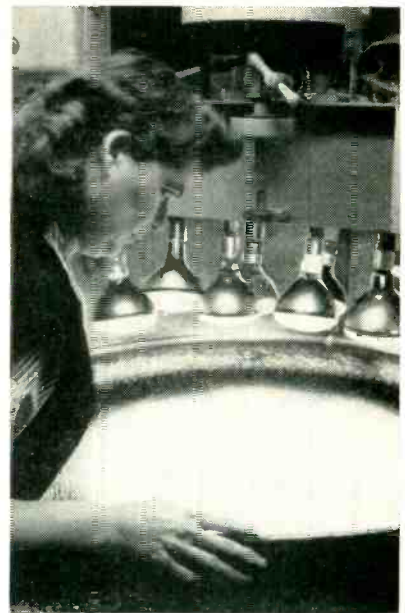
Drying machine in action, with whirling plastic sheet visible only as white blur in tank
