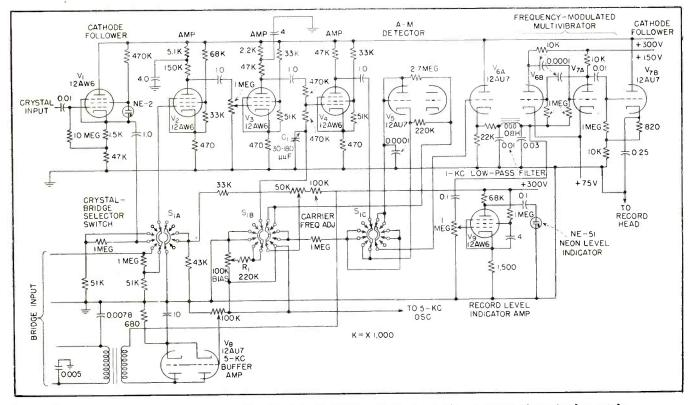
FIG. 4—Circuit used in each of the six f-m recording channels of vehicular research recording equipment shown in photographs
