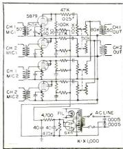
FIG. 2-Preamplifier-mixer unit
