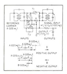
FIG. 3—Basic circuit of phase sensitive detector and output signal vectors
