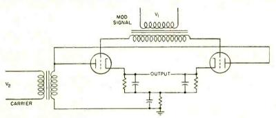
BALANCED-TRIODE DEMODULATOR<sup>15</sup>— Push-pull modulated signal is applied to grids. Unmodulated carrier is used as reference and to supply plate voltage. Output is push-pull error signal
