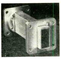
Method of placing flat brazing material in joints of aluminum waveguide in preparation for preheating
