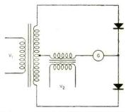
VHF RADIO-RANGE COMPARA-TOR<sup>3</sup>— Meter indicates zero when  $V_1$ and  $V_2$  are 90 degrees out of phase or when either or both voltages are zero. Used to demodulate 10-kc f-m subcarrier
