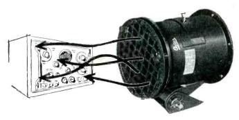
Type AXB-2107—100 CFM output with input of 27V DC, 115V AC, 60 or 400 cycle.
