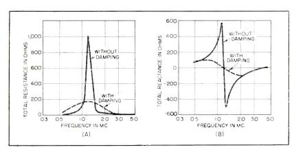
FIG. 9—Impedance of ferrite core with and without series resonant damping
