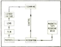
FIG. 1—Flying spot scanner and computer-input tape recorder
