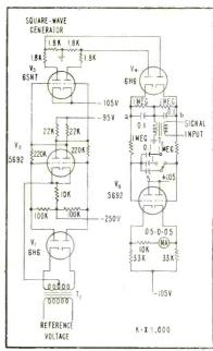
FIG. 1—Synchronous amplifier combines reference square wave with signal to obtain error voltage across filter circuit
