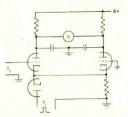
GATED-CATHODE DETECTORs—Similar in operation to gated-grid circuit except that pulses are applied to cathodes. Common cathode resistor for all tubes provides nearly push-pull grid-cathode voltages
