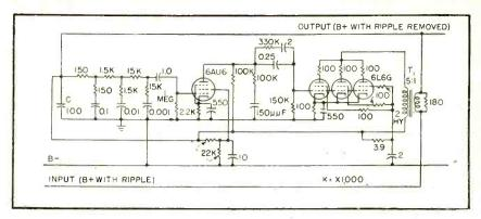
FIG. 3—Complete circuit diagram of electronic filter for 300-volt 18-ampere power supply. Equivalent L-C filter would require 50 cubic-foot capacitor
