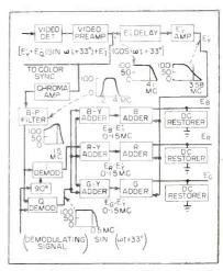
FIG. 3—Video system for ceiling-performance receiver
