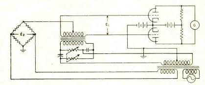
BRIDGE-BALANCE DETECTOR<sup>10</sup>— Current in meter is proportional to  $E_1E_2\cos\theta$ . By adjusting phase of  $E_1$ , output current can be made dependent on only the reactive or resistive component of either voltage. Phase is adjusted by dual potentiometer in phase shifting circuit
