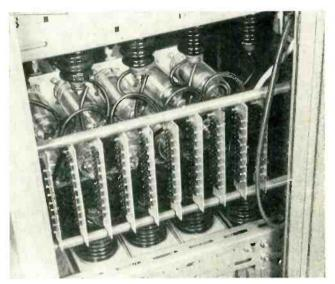
Thyratrons of pulser unit connect energy storage capacitors at bottom if picture across light source when triggered by counter circuit
