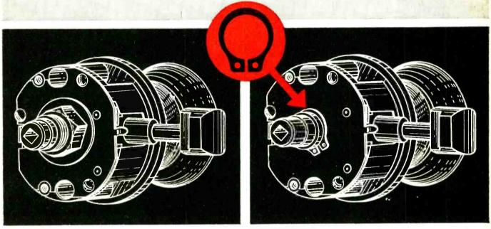
**OLD WAY.** Main shaft required costly threading. Assembly was slowed by the double application of washer and nut and time-consuming tightening operation.
