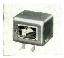
Boonton Radio Corp., Boonton, N. J. Type 590-A line of inductors is designed for use in the Q circuit of the company's Q meters types 170-A and 190-A. The new inductors, available in 6 types, are useful for measuring the r-f characteristics of capacitors, resistors and insulating materials over a frequency range of 20 to 230 mc. Each inductor consists of a high-Q coil mounted in a shield and is provided
