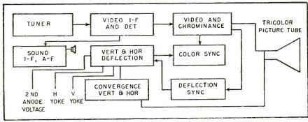
FIG. 1—Stages of basic receiver, emphasizing sections handling color signals
