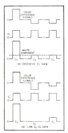
FIG. 7—Excessive  $E'_F$  gain (A) results in desaturated red vertical bar. Low  $E'_G \cdot E'_F$  gain (B) adds green component
