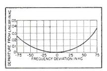
FIG. 7—Departure of frequency deviation from linear with alpha-cutoff
