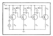
FIG. 4—Four-stage transistor amplifier using emitter degeneration to stabilize gain and raise input impedances. Values for  $R_c$  and  $R_e$  are given in text
