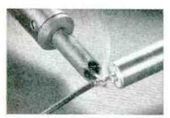
Solder right up to the bushing with G-E Silicone end seal-no danger of
