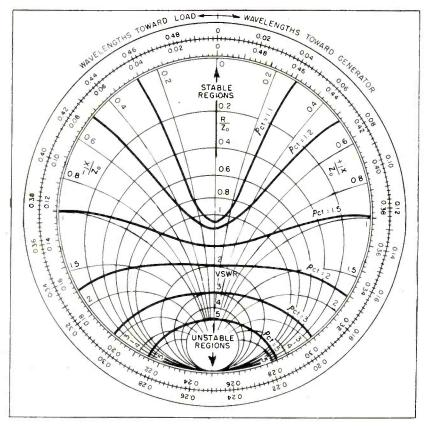
FIG. 5—Rieke diagram showing frequency-jumping contours for c-w tube
