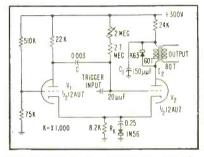
FIG. 2-Circuit of multivibrator cathodeshunt diode and plate-shunt capacitor to extend delay time
