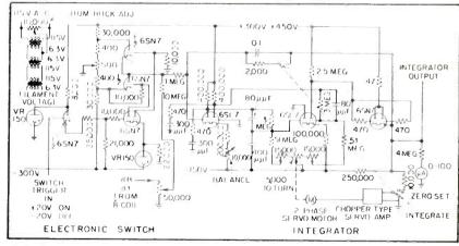
FIG. 3—Integrator and electronic switch provide voltage analog of magnetic field strength variation. Integrator uses Miller feedback circuit with d-c amplifier
