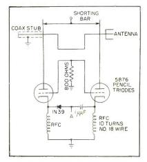
FIG. 2—Crystal in cathode circuit of f-m transmitter applies modulation
