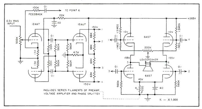
FIG. 5—Complete transformerless amplifier capable of outputs of 8 watts. Bridge-type ouptut circuit matches voice-coil impedance
