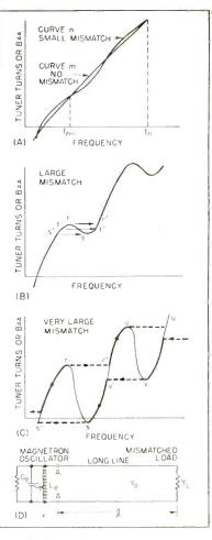
FIG. 1.—Tuning curves of radar magnetron oscillator connected to long mismatched transmission line, and equivalent circuit for load mismatch
