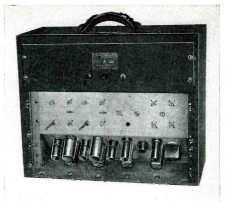
View of instantaneous multiplier with cover removed. Top section is power supply
