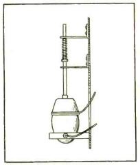
FIG. 2—Arrangement of electrodes in electronic egg grader
