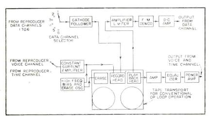
FIG. 3-Two-channel analyzer employed for detailed analysis of recording
