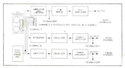
FIG. 2—Arrangement of reproducing equipment used at laboratory
