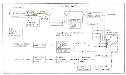
FIG. 1-Block diagram of eight-channel magnetic tape recorder
