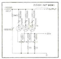
FIG. 4—Diode network converts voltage wave'orm from integrator to corresponding oscillator control signal
