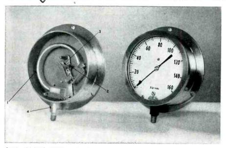
Interior of Ashcroft Duragauge at left shows where copper-base alloys are widely used because of their dependability and corrosion resistance. Brass and Bronze are especially important at the following key points: (1) Bourdon Tube, (2) Gear Segment, (3) Rotary Geared Movement, (4) Socket, Courtesy of Manning, Maxwell & Moore, Inc., Stratford, Conn.
