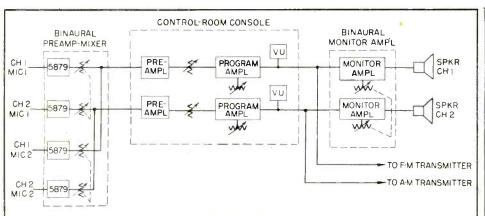
FIG. 1—Typical binaural broadcasting setup showing use of preamplifier mixer and monitor
