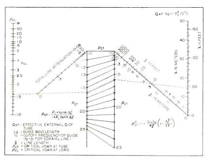
FIG. 7—Nomograph for calculation of the critical voltage standing-wave ratio at which frequency-jumping begins in the oscillator tube
