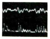
Lower waveform is square of complex waveform shown above
