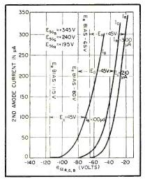
FIG. 10—Equal signal drive for color balance in one type of operation
