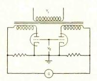
COSENS PHASE-SELECTIVE BRIDGE<sup>7</sup>— Triode amplification provides high sensitivity. Output proportional to phase angle divided by V<sub>1</sub> V<sub>2</sub>
