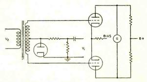
GATED-GRID DETECTOR<sup>8</sup>— Rectangular reference waveform produced from sinewave  $V_1$  by diode and R-C circuit (continued on p. 190)
