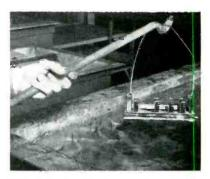
Lowering dip-brazed part into cold water quench, for heat-treatment
