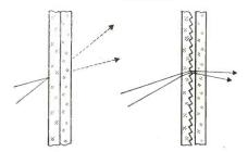
Fig. 2. Diffusing properties of ground-glass screen scatter oblique light away from viewer's eye.
