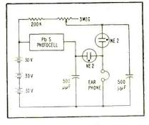
FIG. 1—Two neon-tube relaxation oscillators are initially tuned to same frequency so that discontinuity in reflected light shows up as beat frequency. Effect is caused when light variations produce small variations in cell resistance
