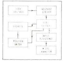
FIG. 1—A node current checker for phototubes used in Navy equipment
