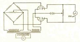
MACNAMARA PHASE BRIDGE<sup>11</sup>—Has accuracy of 0.1 percent with an input of 20 volts at frequencies up to 50 kc
