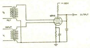
GATED-BEAM PHASE DETECTOR<sup>14</sup>—Plate current is at maximum for in-phase operation, and at a minimum for 180-degree phase difference
