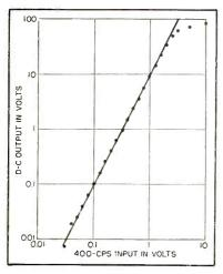
Amplitude range of input functions over which true product is obtained
