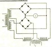
PHASE-SELECTIVE DETECTOR FOR BRIDGES<sup>17</sup>— Double-bridge system for use at high frequencies
