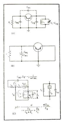
FIG. 2—High-frequency equivalent circuits of transistor oscillator
