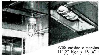
With outside dimensions of 13' 2" wide x 11' 2" high x 16' 6" long, this standard model chamber has an interior working area of 10' x 10' x 8' high. Door is 5' wide x 8' high, its window 30" x 30", and wall window 36" x 36".
