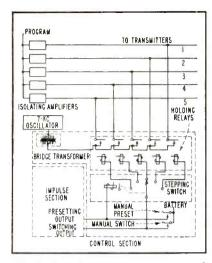
FIG. 1—Switching tone is superimposed upon one of five transmitter lines
