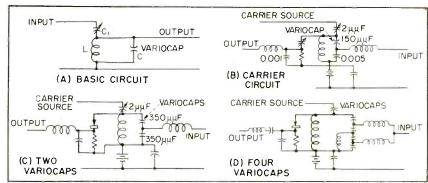
FIG. 2—Single-stage dielectric amplifier circuits using nonlinear variocaps in four ways
