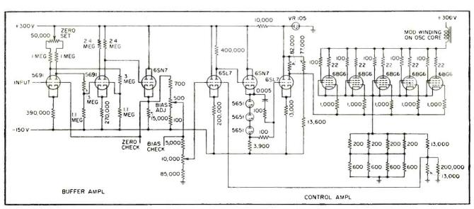
FIG. 5—Control amplifier delivers desired current waveform to control winding on oscillator tuning coil
