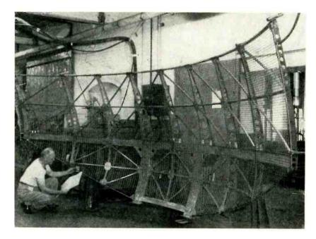
screens must be accurately shaped and must retain this shape to preserve the operating characteristics of the radar.
