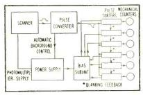
FIG. 1—Block diagram of the stain counter uses spiral scanner
