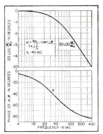
FIG. 3—Magnitude and phase of current amplification factor
