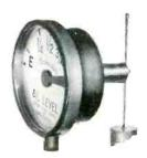
Rochester Liquid Level Gauge utilizes synchronous magnetic torque drive principle to operate pointer, keep gauge head pressuretight. Magnets eliminate stuffing box and shaft—permit mounting gauge in any position without danger of leakage.
