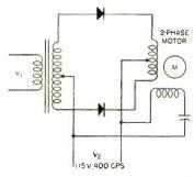
VARIATION OF WALTER CIR-CUIT - Suitable for output stage of amplifier in self-balancing bridge. Germanium power rectifiers or diffusedjunction diodes can be used
