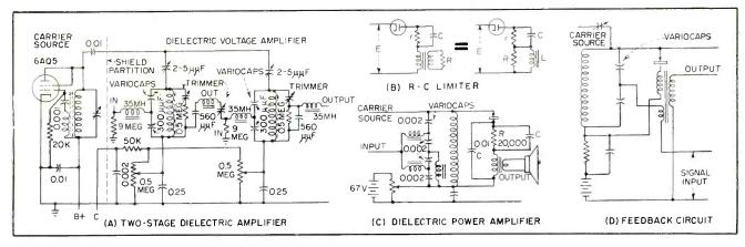
FIG. 3—Examples of dielectric voltage and power amplifier circuits using carrier sources. These circuit techniques are also adaptable to the small capacitance value used in vhf f·m oscillators. Mathematical derivations and further details are given in the original NBS reports by the author, 13.4-74R and 13.4-102R, available from the NBS Technical Reports Section
