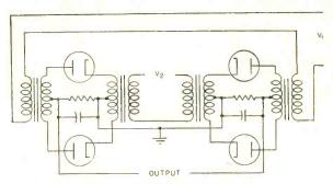
WARD-LEONARD SYSTEM DETECTOR<sup>18</sup>— Commercial variation of full-wave demodulator system. Output is used to control d-c motor through d-c amplifier
