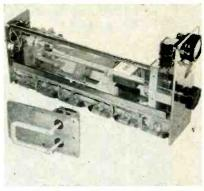
UHF frequency-modulated transmitter uses two pencil triodes in output
