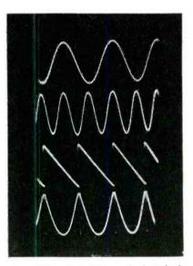
Sine wave (first line) applied to both inputs gives squared waveform (second line). Fourth line is squared version of sawtooth shown in third line
