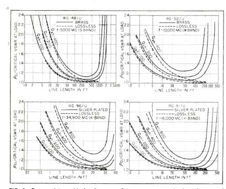
FIG. 8-Curves giving critical voltage standing-wave ratios at load as function of system constants. Curves shift as tube is tuned through the operating range
