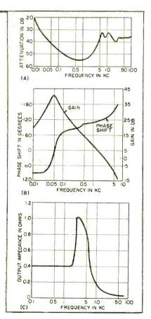
FIG. 4—Curves showing filter attenuation and amplifier gain and output impedance vs frequency
