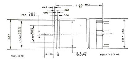
Rugged, environmental-resistant unitized construction with guaranteed maximum error 7 minutes of arc from electrical zero. Average error spreads within 5 minutes. The accuracy of this series eliminates the need for complicated 2-speed Synchro systems in many applications. Advanced manufacturing techniques now make these performance advantages available at minimized cost.
