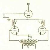
CATHODE-GATED DETECTOR WITH CURRENT OUTPUT<sup>8</sup>— Used with d-c servo motor. Coils  $L_1$  and  $L_2$  are split field of servo motor or differential relay. Provides differential current with low output impedance
