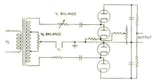
R. L. FRANK PHASE COMPARATOR<sup>20</sup>—Insensitive to the third and all even harmonics of both input voltages. Combines two 120-degree-conduction cascade doubler circuits
