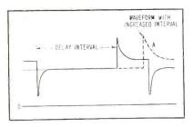
FIG. 1—Voltage between cathode and ground in monostable multivibrator showing effect of increasing delay time
