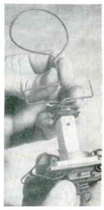
Waveguide flange assembly fixture consisting chiefly of wire springs and stainless steel spring clamps. Wire loop at top serves for placing assembly in preheating furnace and later suspending it in dip pot
