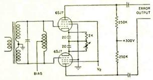
PENTODE PHASE DETECTOR<sup>12</sup>—Used in radar units. Has a gain of 70 using 6SJ7 tubes; with 6AS6 tubes gain is 120 with 40-volt, 2,000-cps reference voltage on  $V_2$
