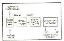
FIG. 14—Basic elements of crystal filter color sync circuit
