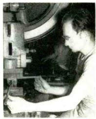
After the tubing has been shaped to the right curvature, a hydraulic press flattens it for easy joining to radar-screen rib ends. Rapid and uniform pressure of the press insures a perfectly flat joining surface without affecting the tube's parabolic shape, without distorting the sections along spans where rigidity is specified and without unduly stressing the metal at flattened areas
