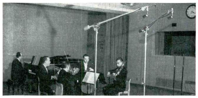
Microphone arrangement for a binaural broadcast. Announcer's microphones are at right near control-room window
