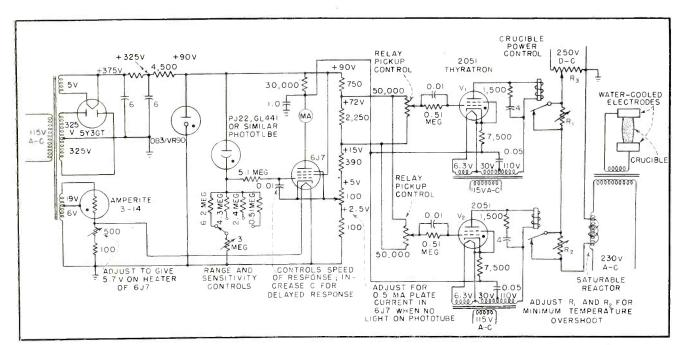
FIG. 1—Complete circuit of stabilized photoelectric amplifier as used for two-point control of temperature in graphite crucible
