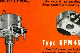
For TV preset control applications. Recessed screw-driver slotted shaft remains solder-free during panel dipping. Control may be held rigidly to panel before soldering by twisting 2 ears. If ears are left straight, the solder will permanently anchor control to circuit panel. Terminals extend per-pendicularly 7/32" from control's mounting surface.
