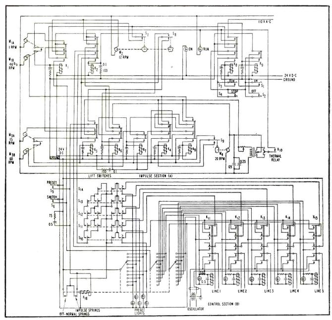
FIG. 2—Complete circuit of the impulse and control sections of the keyer. Synchronous motors provide pulses that are random because of thermal-delay relay. Relays are preset by stepping switch
