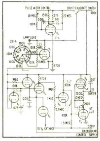
FIG. 2—Phototube, amplifier and pulse converter circuits used in counter
