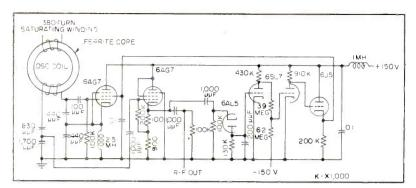
FIG. 6—Permeability-tuned master oscillator sweeps in frequency from 370 kc to  $4.2~{\rm mc}$  during the one-second cosmotron magnet pulse
