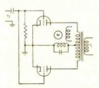
BROWN DISCRIMINATOR 9— Basic circuit for electronic potentiometer. Modification of Cosens circuit for use with two-phase a-c servo motor
