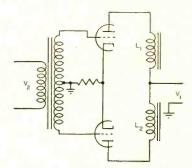
MODIFIED COSENS BRIDGE DETECTORs—Applicable to servo control. Coils  $L_1$  and  $L_2$  are differential relay coils or fields of d-c servo motor
