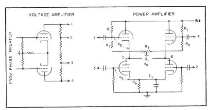
FIG. 2—Basic circuit diagram of transformerless amplifier
