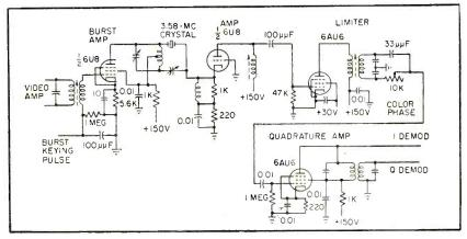
FIG. 15—Crystal filler and associated circuits for color sync
