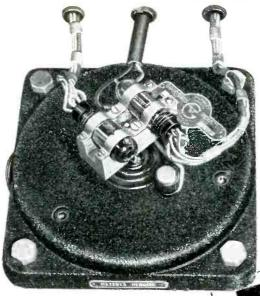
Illustrations by courtesy of Standard Telephones and Cables Limited. England, who say that these Goodmans Permanent Magnet Shakers "have been chosen as they give a faithful reproduction of the input wave form and enable high accelerations at any frequency to be obtained".
