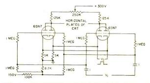
SCR-615 PHASE-SENSITIVE AMPLIFIER<sup>16</sup>—Radar application with cathode-ray tube display. Cathodes are gated by sine-wave generator. Reference voltage comes from two-phase generator synchrononized with antenna
