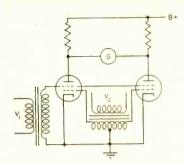
MORTON SCREEN-GRID PHASE DETECTOR<sup>13</sup>—Reference voltage  $V_2$  is applied to control grids and variable voltage  $V_1$  is applied to screens. System puts light load on power supply of variable phase
