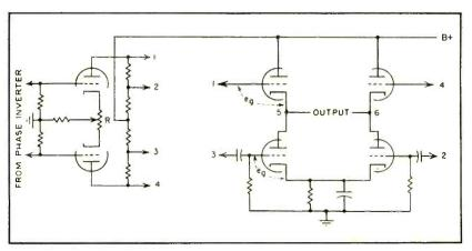
FIG. 4—Basic circuit of transformerless amplifier using direct coupling
