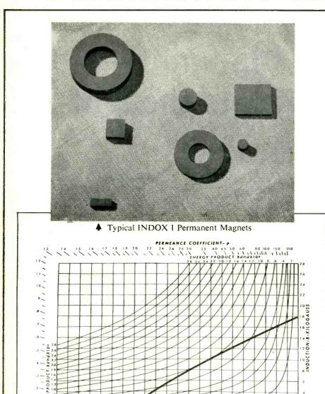
▲ Demagnetization and Energy Product Curve for INDOX I
