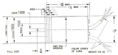
series R200 Control Transformers, Transmitters and Resolvers-maximum error spread 20 minutes of arc. Repeaters and Differentials—maximum error spread 30 minutes of arc. For 26 volt operation. Certain models for 115 volt and with variations in shaft dimensions also available.
