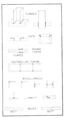
Typical joint designs used with dip brazing of microwave plumbing
