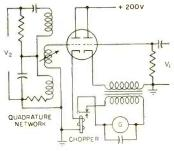
WALD REBALANCING PHASE INDICATOR<sup>22</sup>—Similar to Wald indicator, but higher precision. Resolver is rotated so meter indicates zero. Phase shift is indicated on resolver dial
