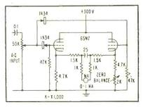
FIG. 1—Electronic voltmeter uses cathode followers to obtain push-pull output, high input impedance and good linearity at low cost in parts
