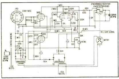
FIG. 1—Circuit diagram of the electronic colorimeter used in gas detector
