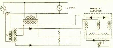
MAMON PHASE DISCRIMINATOR<sup>5</sup>— Uses balanced, polarized magnetic amplifier to boost output of phase-selective detector. Application shown is used to operate relay to disconnect alternator in case of field-excitation failure, loss of synchronization or drive failure
