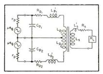
FIG. 1—Equivalent circuit of a typical output transformer illustrates its frequency dependence
