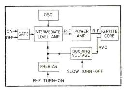
FIG. 7—Intermediate and high-level power amplifiers deliver 2,000-volt f-m signal
