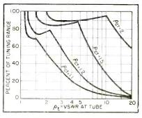
FIG. 6—Percent of tuning range accessible to continuous-wave oscillators when tube is tuned be a ways
