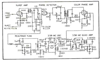
FIG. 17—The automatic phase control color sync circuit
