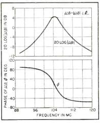
FIG. 4—Magnitude and phase of  $\mu\beta$  in oscillating frequency region
