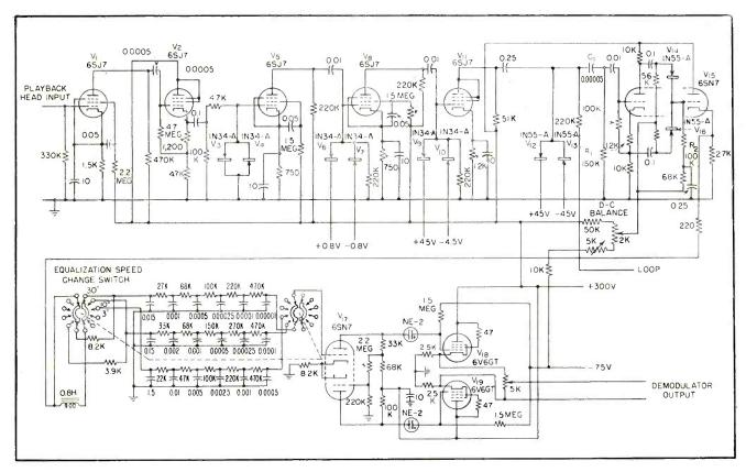
FIG. 6—Playback amplifier and demodulator for f-m channels. A separate channel amplifies voice and timing signals
