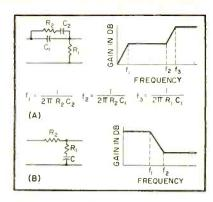
FIG. 2—Low-frequency (A) and high-frequency (B) networks and responses
