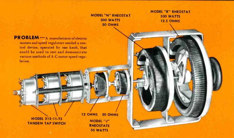
**SOLUTION**—Ohmite produced a special combination of four rheostats and three 11-position switches, all coupled together in tandem, and operated by one knob. The tap switches are loosely coupled to the rheostats so when the quick-make taps close, the rheostat settings are not changed. All units are electrically independent. Any unit or all units can be connected in the circuit to be tested, and can be wired
