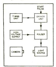
FIG. 1—Block diagram of flash system. Pulser connects series of charged capacitors across flashlamp
