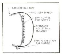
Technique used for cementing fine mesh screen to face of cathode-ray tube
