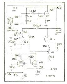
FIG. 1—Low-frequency closed-loop telemetering control uses inductor
