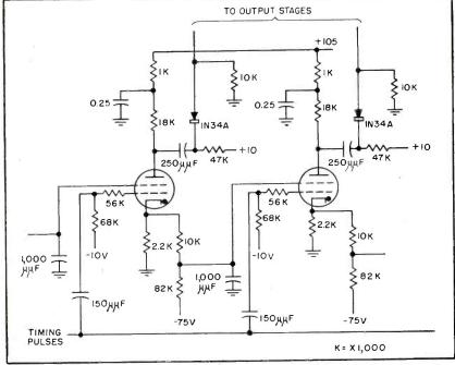
FIG. 3—Two of ten ring-counter stages. Circuit constants give a maximum count of 10,000 per second using component values indicated
