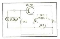
FIG. 2—Amplifier circuit used to obtain data given in Table I
