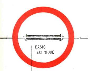
A thin coating of pre-cured and stabilized resistance material is bonded to special glass or an inorganic core to form IRC's exclusive filament type element. This is in contrast to the carbon pill or slug principle of construction. Its uniformity and stability have proved superior since the earliest days of radio.
