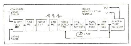
FIG. 16—Block diagram of automatic phase control circuit for color sync
