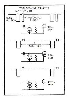
FIG. 12—Setting up of 'blue' d-c restorer on recovered burst
