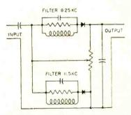
VHF OMNIRANGE DEMODULA-TOR — Recovers 60-cps modulating signal from 10-kc f-m subcarrier
