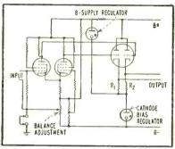
FIG. 5—Regulator tube is used in cathode-follower for bridge amplifier
