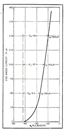
FIG. 11—Unequal signad drive takes advantage of tube curve
