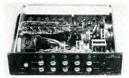
Equipment in use at New York makes provision for control of five broadcast stations, but circuits can be modified for additional transmitters
