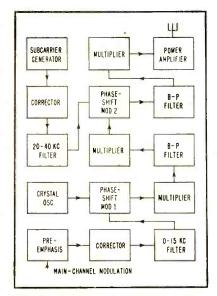
FIG. 1—Method of introducing subcarrier in multiplex f-m system
