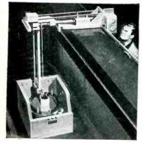
Containers made of Carboloy Hevimet are making the job of handling and transporting radioactive materials easier and safer.
