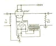
WALD PHASE INDICATOR<sup>22</sup>— Has high input impedance. Accuracy is  $\pm$  1 percent. Average output current  $I_{\rm max}$  cos  $\theta/\pi$ . Upper frequency limit is determined by chopper used
