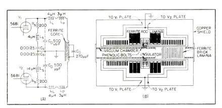
FIG. 8-Power-output system of r-f generator; push-pull 5681 triodes operating in class  $A_2$  deliver 100 kilowatts to ferrite-loaded output loop
