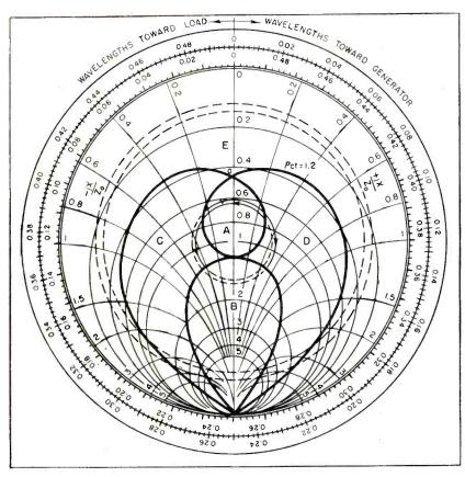
FIG. 4—Example of frequency-jumping behavior of a continuous-wave tube
