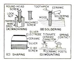
FIG. 1—Construction of variocap components
