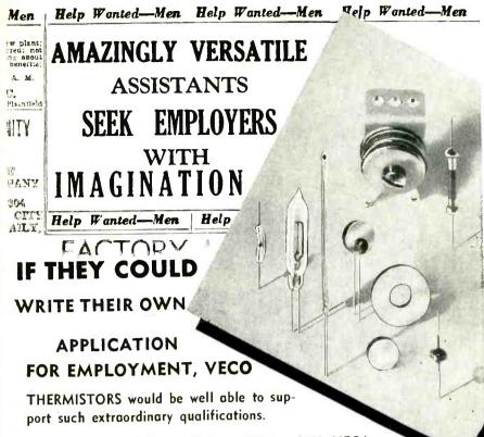
VECO THERMISTORS HAVE A VERY HIGH NEGA-TIVE TEMPERATURE COEFFICIENT OF ELECTRICAL RE-SISTANCE. Their SMALL SIZE and EXTREME SENSITIVITY TO THERMAL CHANGES offer engineers a circuit element which can be utilized in new designs, and in improving old equipment.
