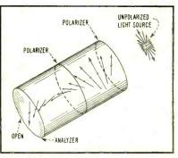
FIG. 1—Rotational effect of two polarizers and an analyzer
