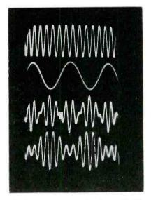
Third line is product of first two. Fourth is product obtained by adding d-c to low-frequency input and multiplying this sum by higher frequency input
