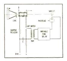
FIG. 2—Basis of a single-element magneto-optical shutter
