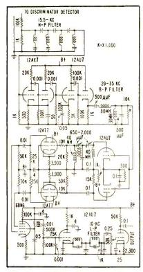
FIG. 2—Auxiliary channel section of multiplex broadcast receiver
