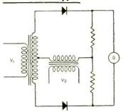
WALTER PHASE - SELECTIVE RECTIFIER1. 2— Gives square-law response, with sensitivity decreasing near balance point. Meter reads zero if  $V_1$  and  $V_2$  are 90 deg out of phase
