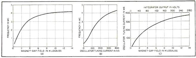
FIG. 1—How r-f generator frequency tracks cosmotron's magnetic field. Desired frequency vs field strength characteristic (A) is achieved by using voltage analog of magnetic field-strength variation to control oscillator tuning current
