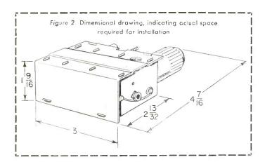
The circuit will tune continuously from 460 to 910 megacycles (channels 14 to 83) in 180° rotation of the single tuning shaft. It works into any IF amplifier that operates over the 41.25 to 45.75 band. The assembly consists of a double-tuned RF preselector, oscillator, crystal mixer and tuned IF coil.
