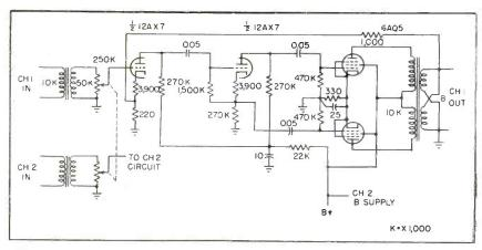
FIG. 3—Monitar amplifier furnishes 10 watts to each of two wall-mounted speakers
