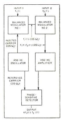
FIG. 1-Block diagram of multiplier
