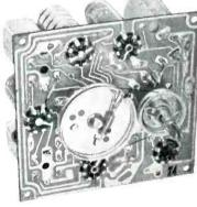
A five tube superheterodyne in volume production utilizing multiple soldering and semi-automatic assembly techniques . . . an excellent application of printed wiring methods by Raytheon Manufacturing Company.
