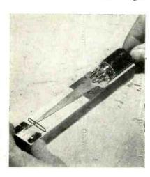
A V-BLOCK and a small pivoted indicator constitute a simple and efficient means of measuring the amount in degrees by which the bottom of a subminiature tube is off square from the plane of the tube. The tube is placed in the machined V of the metal block and
