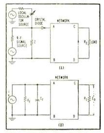
FIG. 2—Hetroydne mixer circuit (A) and its equivalent (B) at intermediate frequencies
