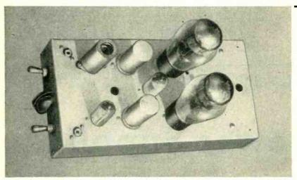
View of transformerless amplifier including preamplifier
