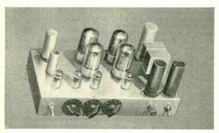
Chassis of 18-watt amplifier includes preamplifier and power supply
