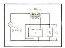
FIG. 1—Basic a.c equivalent circuit of electronic power supply filter
