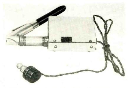
Equipment for blind has battery drain of 30  $\mu$ amp resulting in 700-hour life
