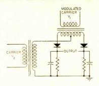
PHASE-SENSITIVE DEMODULA-TOR4— Has push-pull output. Input may be from balanced or single-ended carrier. Carrier signal is reference
