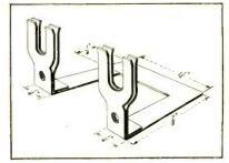
FIG. 1—Mounting bracket for two pencil triodes is grid-feed back loop
