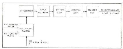
FIG. 2—Block diagram of frequency-control system illustrates how feedback from cosmotron magnet controls r-f generator frequency
