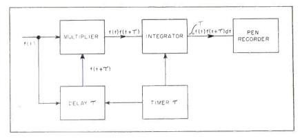
FIG. 4—Block diagram of circuit for obtaining autocorrelation of a function
