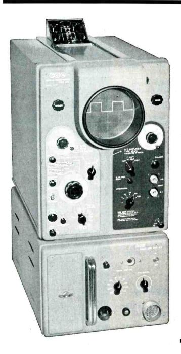
By using interchangeable D.C. Amplifier and Time Base Units, one CAE Oscilloscope performs the operations of several different types of oscilloscopes resulting in a considerable saving in capital expenditure.
