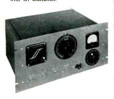
Inductance range is from one to 200 henries. Direct current through the reactor under test is accurately controllable from one to 500 milliamperes, limited only by the resistance of the coil windings. The effect of a change of dc on the inductance value is immediately measurable, by simple rebalancing. The inductance is measured at a constant frequency of 120 cps.
