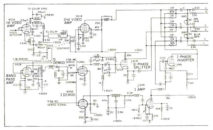
FIG. 6—The I-Q video system for a ceilingperformance receiver contains several new types of tubes
