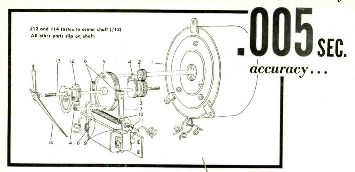
Formula S-1: Expensive high torque, ball bearing motor, low inertia of moving parts, high proportion of precision and ground parts, no thrust bearings as found in ordinary clutches.
