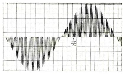
Autocorrelation of sine wave. Stability of equipment is indicated by absence of discontinuity at point where machine was turned off for sixteen hours
