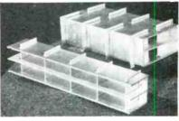
Complicated microwave component produced with high accuracy by dip brazing of stainless steel pieces
