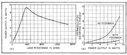
FIG. 6—Curves show output versus load (A) and distortion (B)
