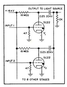
FIG. 4—Series of 5C22 thyratrons sequentially switches ten 0.25- $\mu$ f energy-storage capacitors across flashlamp
