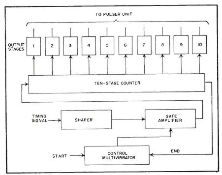
FIG. 2—Driver unit, shown in block form, supplies ten pulses to the pulser unit when triggered by signal from marker generator or magnetic pickup
