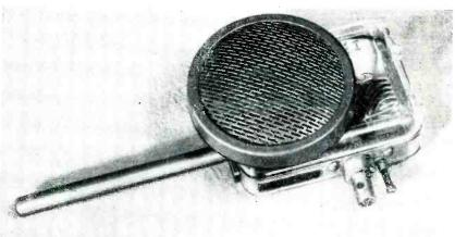
Transmitter containing extra transister audio stage for use with crystal microphone. At left is lapel microphone model, and at right is hand microphone design in which microphone is mounted directly on transmitter housing
