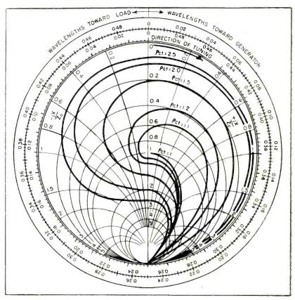
FIG. 2—Rieke diagram showing frequency-jumping contours for pulsed tube
