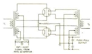
AMPLIDYNE SYSTEM PHASE DETECTOR<sup>18</sup> — Has provision for antihunt signal injection from rate generator. Circuit gives high power amplification
