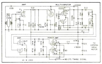
FIG. 5—Method of using tuning fork to generate precise 60-cps power for capstan drive motor and for timing purposes during analysis of the tape recordings
