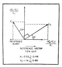
FIG. 13—Relationship between  $E'_I$ ,  $E'_Q$  and color difference signals
