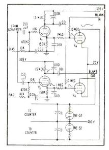
FIG. 3—Pulse sorter and counter outputs are handled in this stage by the thyratron circuits shown
