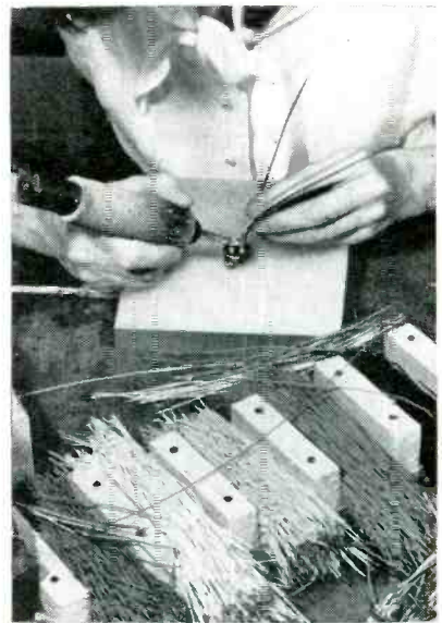
Simple wood block arrangement for holding different colors of wires used in cable plug. Cork sleeve covers almost entire length of pencil-type soldering iron, to give improved grip and minimize accidental burning of hands or fingers
