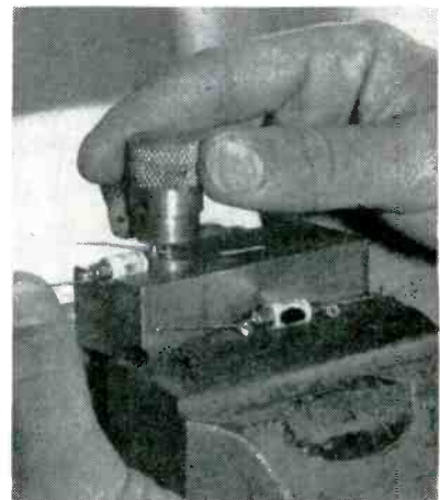
Using tool for placing heat-blocking coils in leads of a crystal diode
