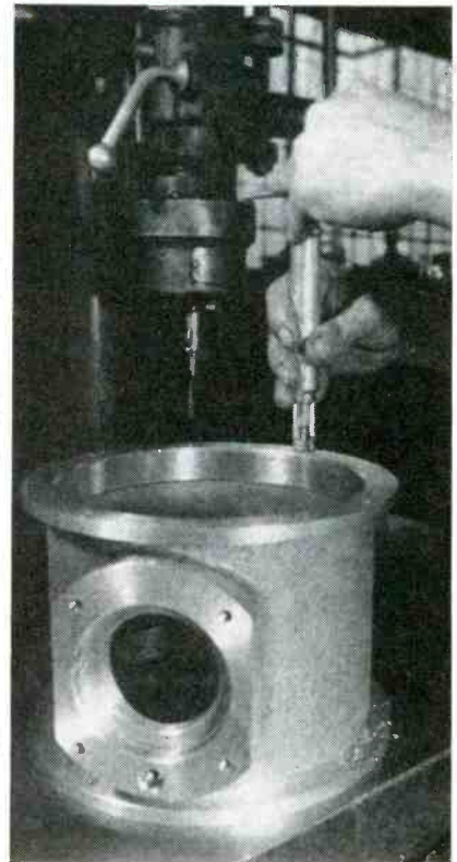
Use of Heli-Coil inserting tool for quick seating of wire thread insert in a tapped hole in x-ray tube housing. Cap screws can then be installed conventionally during assembly of the housing, as shown in first photo
