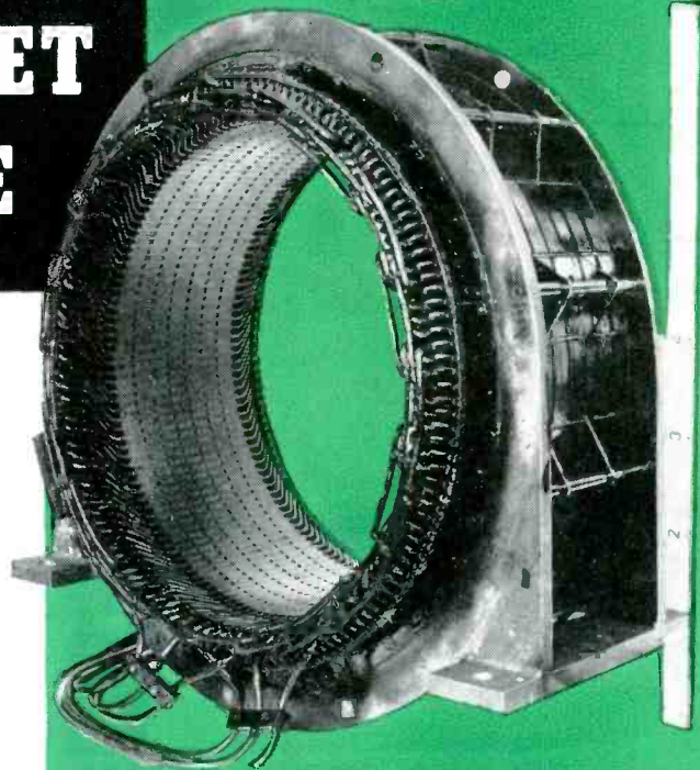
Stator showing open slot construction of the Fairbanks-Morse Type TGZO Alternator, 1405 kva — 300 r.p.m. — 3 phase — 60 cycle — 2400/4160 volts — 80% p.f. — for direct connection to a diesel or dual-fuel engine, for utility, municipal and industrial power generation. Since they are frequently subjected to prolonged overloads in this type of service, they are designed for 50°C temperature rise above 40°C ambient. Coils, insulated and protected with "Natvar 400" extruded tape are tested at 9320 volts for one minute.
