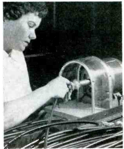
Motor-driven flaring tool for pushing back braided metal shield on cable
