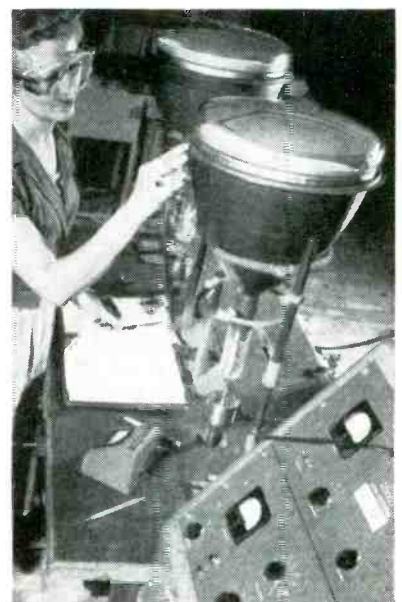
Use of Veeco mass-spectrometer leak detector (made by Vacuum-Electronic Engineering Co., New Hyde Park, N. Y.) to make certain that weld which joins cone to faceplate of RCA color picture tube is vacuum-tight at all points
