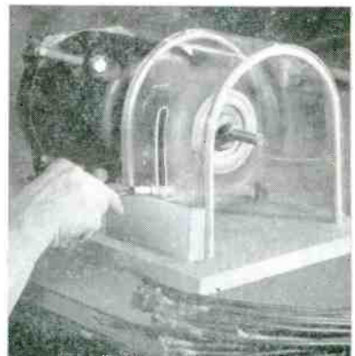
Motor-driven wire-brush setup for combing braided shield on cable
