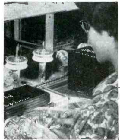
Loading uncoated cathode sleeves in rotary holder preparatory to spraying. Roller chain conveyor brings holders back to operator for unloading after spraying and baking. Finished cathodes are placed in the self-stacking molded plastic trays at rear on bench
