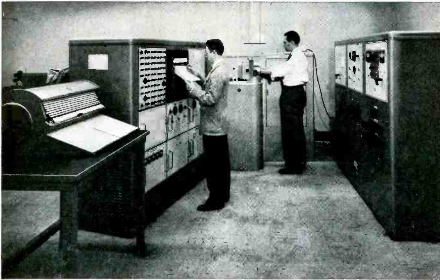
The Production Control Quantometer can make a complete analysis of copper-base alloys in approximately four minutes as compared to several hours by the chemical method.
