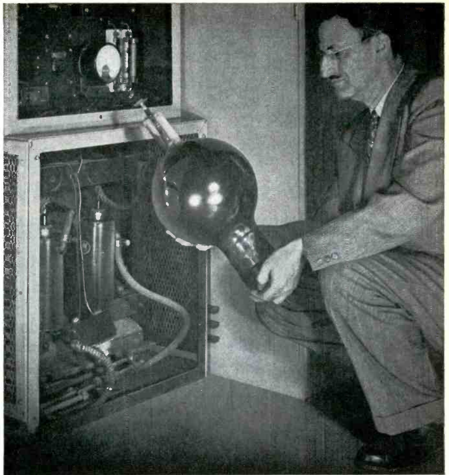
In the Westinghouse plant in Elmira, N. Y., Donald E. Marshall, Section Manager of Gas and Industrial Tube Development, holds a KU-671 Ignitron retired after more than 32,000 hours service.
