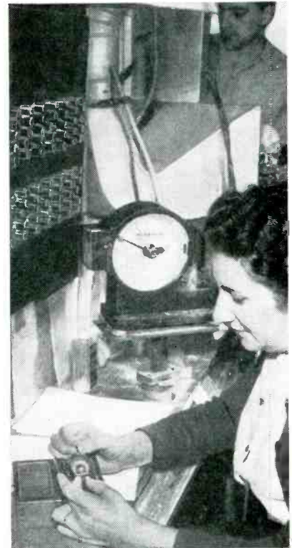
Measuring cathode diameter with micrometer. Weight of coating is measured with precision balance in background. Pushbutton switches above bench control lamps in front of spray operator in background, to give him a continuous visual indication of product quality
