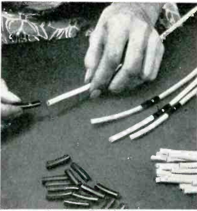
Use of hot-stamped black vinyl sleeving for identifying correcting wires
