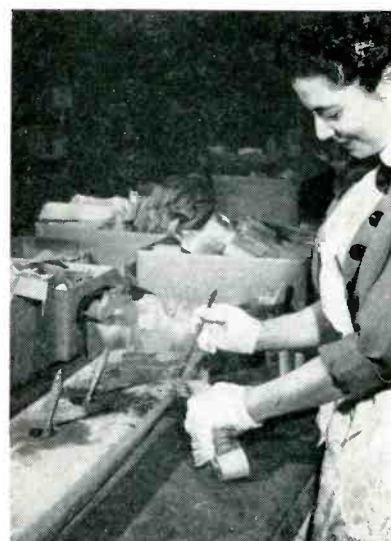
Painting leads of electrolytic capacitor plates at Pyramid Electric Co. The etched foil must be handled with gloves to prevent contamination
