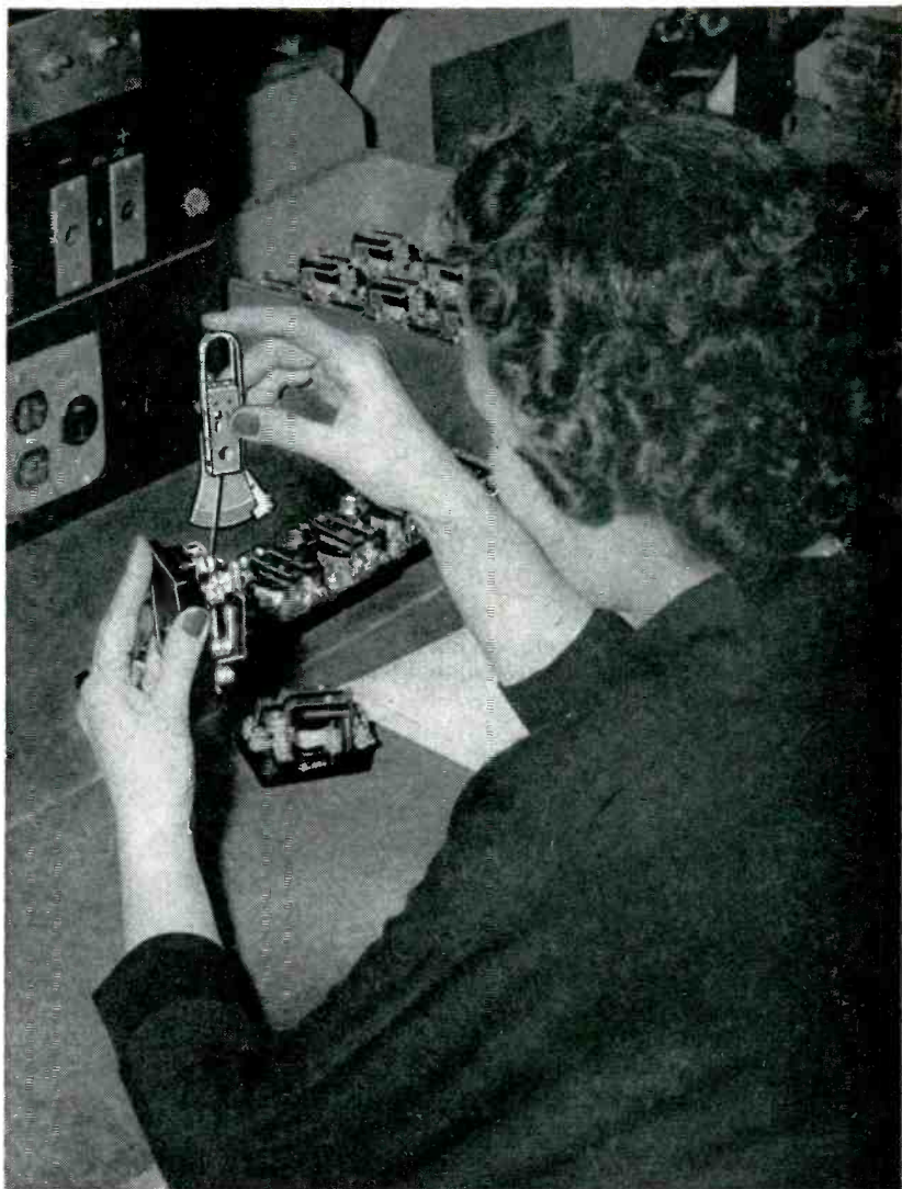
CONTACT PRESSURE OF EVERY RELAY is measured on a gram gauge in Ward Leonard's Mount Vernon plant.
