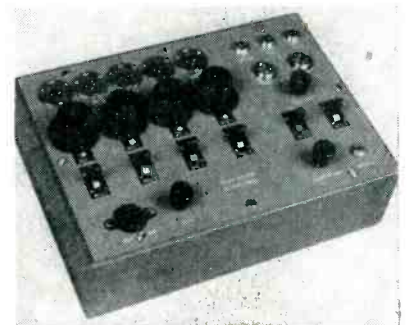
Control box switches floor microphones
