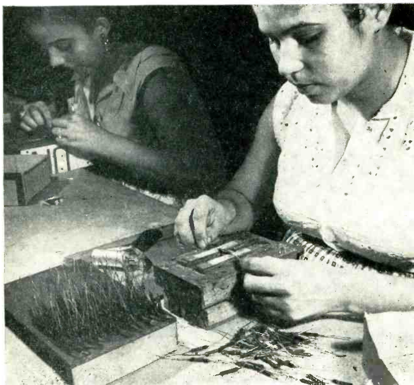
All-manual setup for applying silver lettering to deposited carbon resistors. Drying board holds exactly 300 resistors
