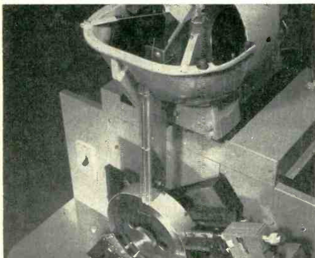
FIG. 9—Rapidly rotating wheel carries needle bearing past measuring head at rate of 400 per minute
