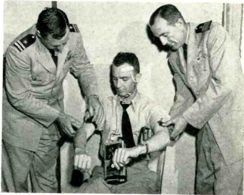
PILOT being wired up will have his emotions and reactions recorded on the ground by way of uhf-radio telemetering system when . . .
