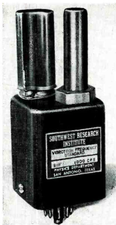
Plug-in unit contains amplifier and 1,000-cps frequency standard shown in other photograph
