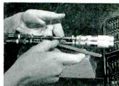
Four-micrometer setup used by Tung-Sol for dimensional checking of tweezer-held cathodes during sampling inspection for quality control
