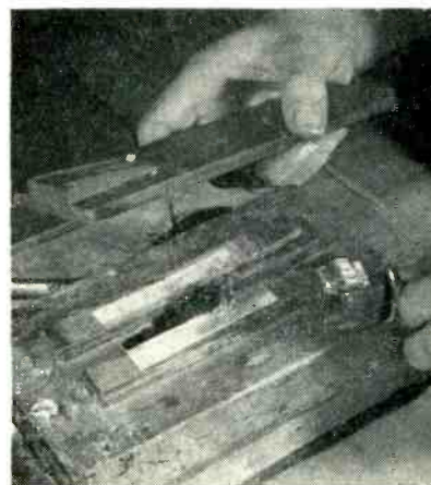
Construction details of fixture holding rubber type for lettering resistors. Type holder is in operator's left hand. Sliding strip with wedge, in right hand, is placed under type holder for adjusting type to correct height
