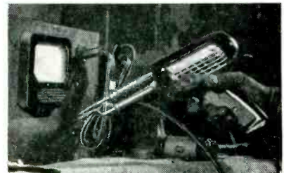
Making 1,700-volt leakage test on finished soldering gun by checking between gun and one side of line cord. Operator wears rubber glove as safety precaution
