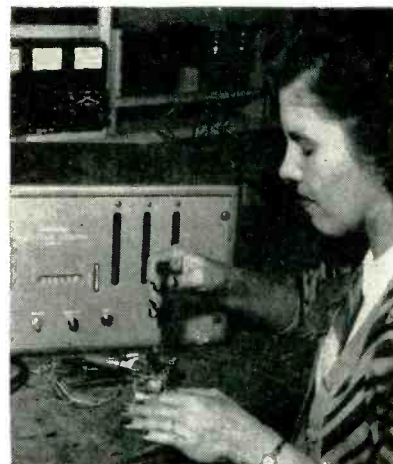
Method of adjusting relay after measuring release time with electronic counter and signal generator
