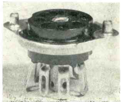
Closeup of integral-eyelet socket that eliminates need for separate mounting rivets
