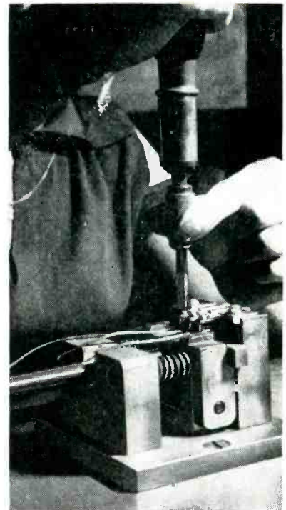
Method of using Yankee screwdriver to tighten contact screws while armature bracket is held rigidly in jig screwed to bench
