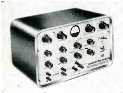
Simplified transistor tester traces characteristics on screen of cathode-ray tube
