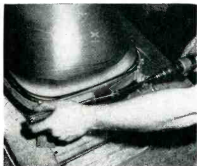
Tightening clamping band of 21-inch picture tube while face of tube is centered on special pallet
