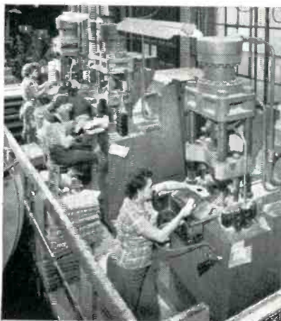
Production operations—including mixing, molding, drilling, tapping and stamping are mechanized. This assures uniform quality, fast operation, low costs.
