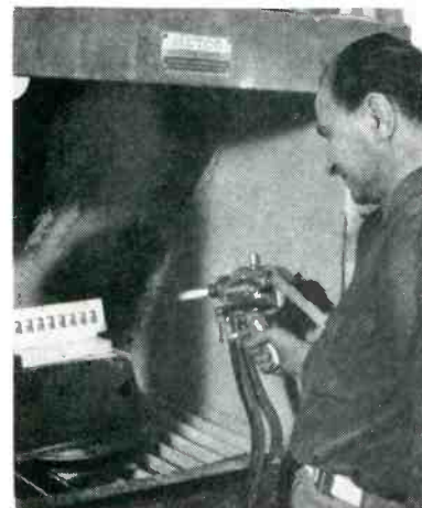
Spraying group of 10 Bakelite pivot blocks for electronic dictating machines with molten metal for shielding
