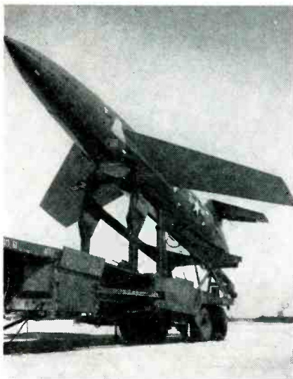
MATADOR —Designated B-61, this Martin-built Air Force tubojet aircraft is designed for long-range bombardment
