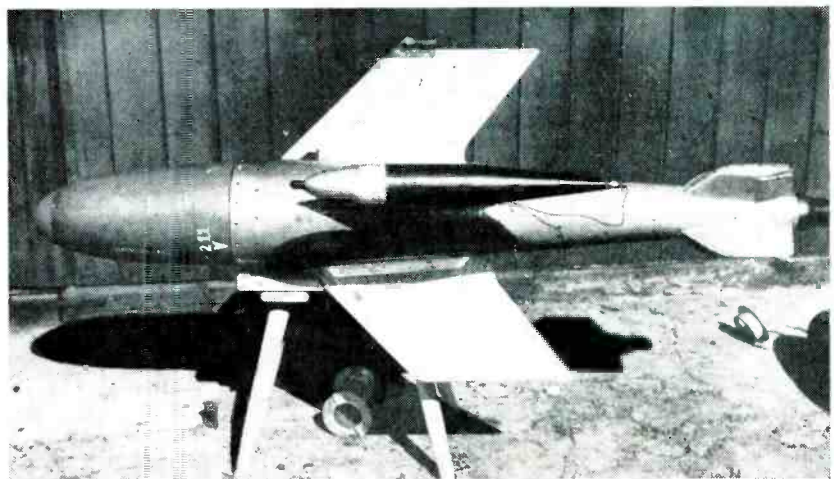
SPIELER —Developed by German Luftwaffe, this air-to-air missile received control signals over wire, making it immune to electronic countermeasures. Proximity fuze increased missile's deadliness
