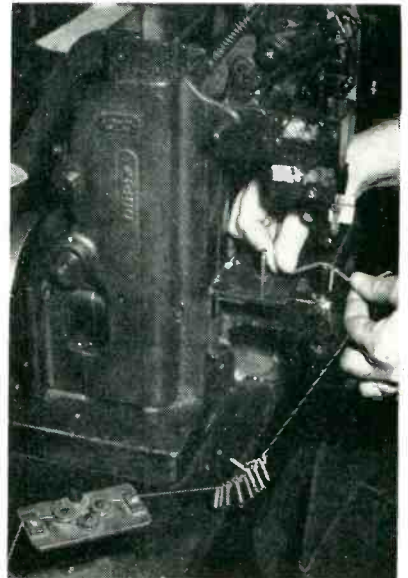
Setup for producing dial cords, each with an attached spring. Tension-controlling jig is in foreground
