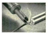
Solder right up to the bushing with G-E Silicone end seal-no danger of cracking glass.
