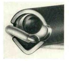
End of wrapping tool, with wire in position ready for wrapping. Wire is inserted in outer slot of spindle as shown, and terminal goes in round hole of spindle
