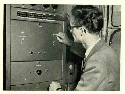
Shawinigan Falls, P. Q. radio station CKSM is remotely controlled by this CGE equipment. Dial is located at studio. Transmitter engineer tests selector with pushbutton
