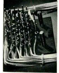
Closeup view of relay base, showing appearance of solderless wrapped connections. The wrapping tool starts its winding at the bottom of the terminal and works outward until it runs out of wire
