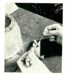
Method of pressing capacitor against pigtail held in jig
