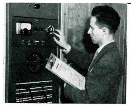
Studio engineer dials control impulses in sequence then selects desired monitor function to check remote transmitter
