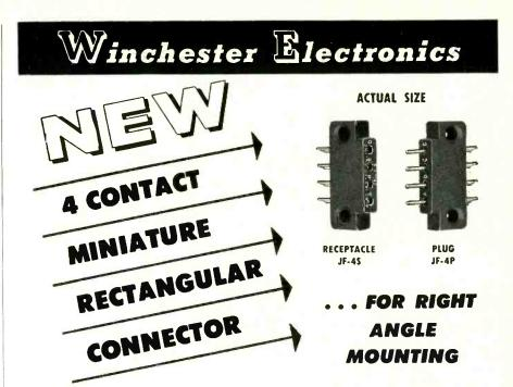
Another special design added to our extensive line of miniature connectors. The JF-4 has four miniature contacts in a mineral filled phenolic insert body and provides, on both the plug and receptacle, two transverse mounting holes for right angle panel or chassis mounting. It is ideal for limited space and weight requirements in portable or airborne equipment.
