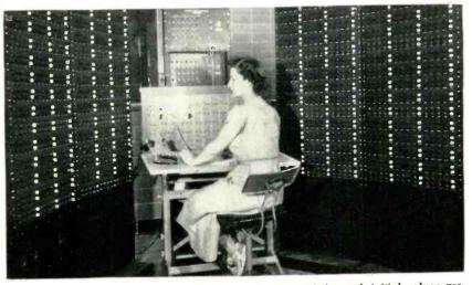
Computer operator reads answers on counter-chronograph (center), initial values are set up on data boards, left and right
