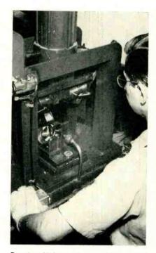
Pressing 90-degree yoke coils to shape
