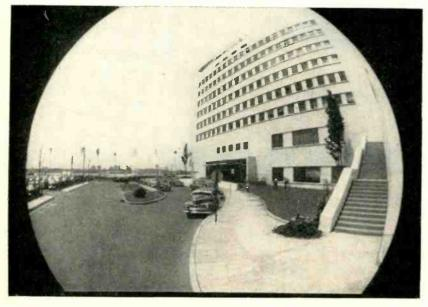
Wide-angle lens giving 142-degree field of view, as used  $\boldsymbol{\omega}$ t the Navy's Special Devices Center, Sands Point, N. Y. in a gunnery trainer. A television system using this wide-angle lens and a spherical-screen projection receiver to provide three-dimensional television is presently under development at RCA
