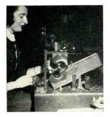
Placing yoke coil assembly in insulation-wrapping fixture, after placing tape on slide, adhesive side up, and placing end of varnished cambric strip on tape
