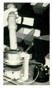
Wood rod used to keep dirt out of completed yoke assembly during testing of individual coils
