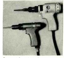
Commercial versions of wrapping tool, with air-operated model below. Both have trigger-type control for starting and stopping the rotation of the inner spindle
