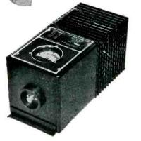
This series of instruments was designed to measure RF power up to 400 watts, and serve as an excellent dummy antenna load over the frequency range 50 to more than 1000 MCS in 52 ohm coaxial line circuits.
