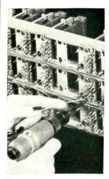
Using air-operated commercial version of wrapping tool for making solderless connections to plain rectangular terminals on a relay rack
