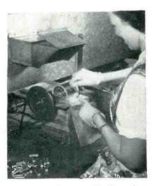
A quick brush across the face of a drum rotating in molten aluminum-alloy solder is sufficient to compress and tin the exposed foil ends of a rolled aluminum-foil capacitor unit
