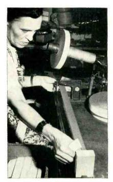
Setup for cutting picture-tube cushioning bands
