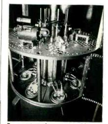
Power output of any current 5-kw whf transmitter can be stepped up to either 25 or 20 kw, depending on the channel, with this RCA vhf conversion amplifier. The equipment consists of aural and visual power amplifier and blower units, aural and visual power supply and filter units, aural and visual control units, vestigial side-band filter and other accessories
