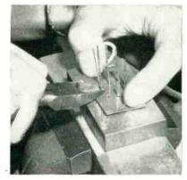
Use of spacer sheet as guide for cutting leads at other end of group to final length. Heat-absorbing brass block is divided into two parts so it can be removed after soldering is completed. Finished end plate rests in hole in wood iig clamped in vise
