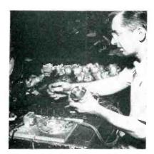
Rotating yoke by hand to wrap insulation around it under pressure. Tape sticks to Saran and pulls the cambric around as the yoke is turned
