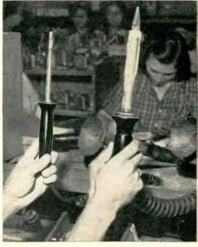
You can often replace heavy irons with this 120-volt, 60-watt lightweight iron for communications soldering.
