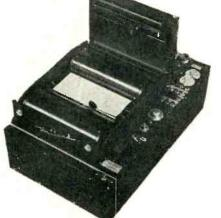
OPEN VIEW OF 708-8 (8") recorder showing supply and take-up drums, operating controls.
