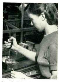
Assembly of RCA Victor single-channel uhf selector. Operator is inserting resistor lead in tiny punched slot for grounding to chassis. Simple wood jig supports chassis during assembly work
