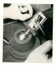
Combination slide and peg fixture for terminal board subassembly work in connection with subminiature equipment. Terminal board slides in grooves. going down between metal spacing rods inserted in bottom of fixture. Rods on one side serve to space silver-button mica capacitors off the chassis, and rods on the other side space four paralleled ceramic capacitors off the chassis
