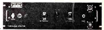
THRESHOLD MONITOR provides means for the control of voltage levels or rate of change.
