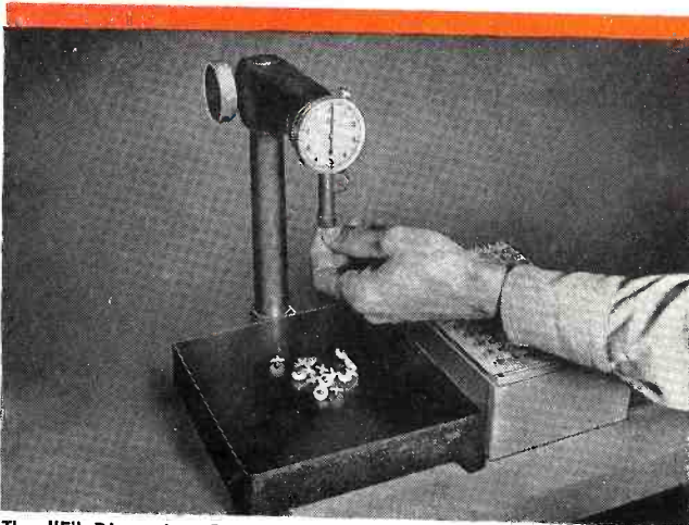
The "E" Dimension Gauge measures the critical spacing between the ceramic surface and the surface of the emitting cap in Disc Cathodes. Tolerance limits must be accurate to \pm 0.0005'' since the dimension controls cut-off voltage and adds uniformity to the characteristics of cathode-ray tubes.
