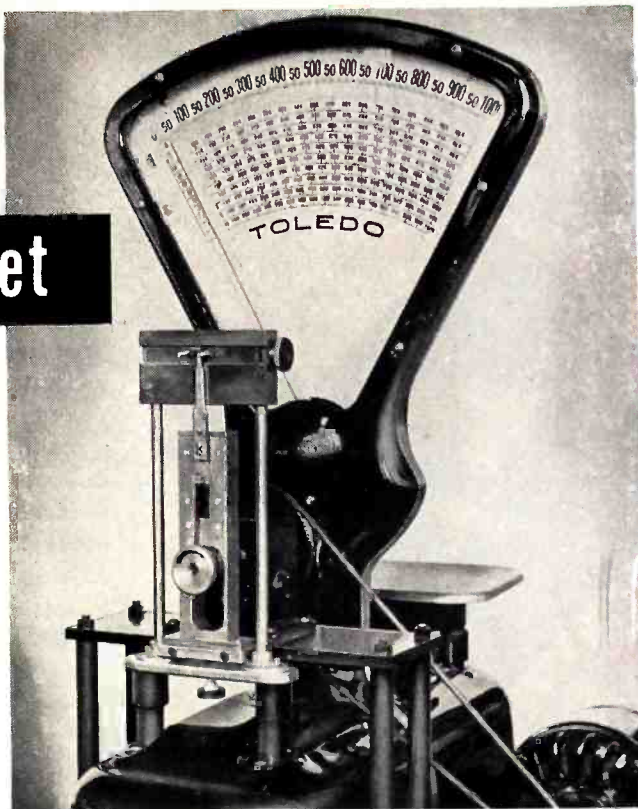
Developed in Superior Laboratories, this Collapse Tester is now accepted by A.S.T.M. The instrument is used to determine the degree of resistance to bending in finished cathodes.
