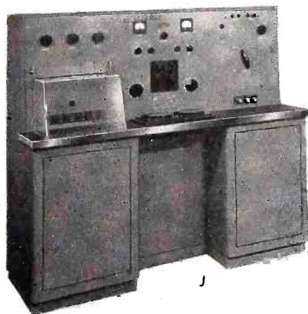
Fig J Model 261B Standards calibrates AC meters to 0.5% thru ranges of 10 millivolts to 1500 volts and 1 microampere to 200 amperes. Uses Weston Mod. 341 and 370. Electronic generator provides 50/1600 cycles test voltage, controlled sine wave. Operates on 105/125 volts, 50/1600 cycles, w/internal voltage regulator. Price $9250.
