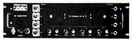
DC CONVERTER —for low level DC recording such as thermocouple output.
