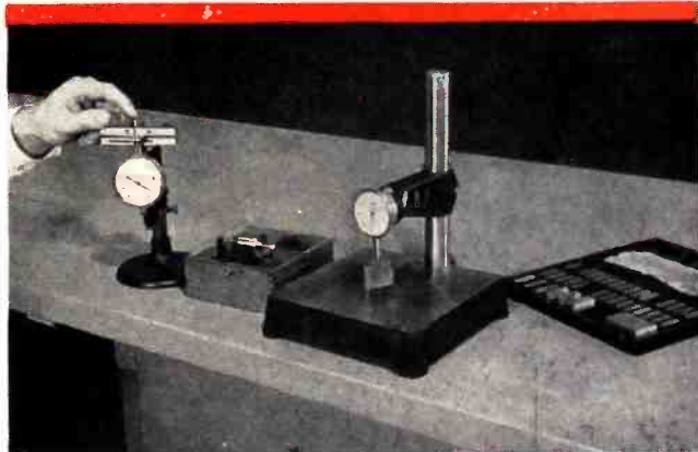
The Flat-Faced Hand Micrometer checks cathode length and is accurate to .001". Conical Faced Barrel Micrometer checks wall thickness to tolerances of .0001". The Flat Faced Barrel Micrometer checks O.D. and bead dimensions, can be read to .0001". The Ultra Precision Barrel Micrometer measures shaped cathodes (O.D.) and beads and is readable to .00004". The "Go" and "No Go" pin gauges measure the inside diameter of round cathodes.
