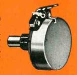
TYPE 252, (JAN-R-19, Type RA20) 2 watt, 1 17/64" diameter variable wirewound resistor. Also available with other special military features not covered by JAN-R-19 including concentric shaft tandem construction. Affached switch can be supplied.
