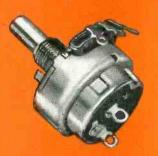
TYPE GC-35, 1 1/8" diameter variable composition resistor. Wattage rating: 3/4 watt for resistances through 10,000 ohms, 2/3 watt for resistances over 10,000 ohms through 25,000 ohms, 1/2 watt with 500 volts maximum across end terminols for resistances over 25,000 ohms. Available with or without illustrated attached switch and in concentric shaft tandem construction C2-35 as shown above.
