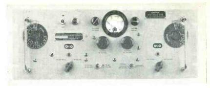
Front panel of newest addition to crystal-testing series, the TS-683/TSM. This is intended for the range of 10 mc to 75 mc, but has actually been calibrated up to
