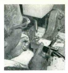
Press setup for producing strips to be used in insulating a toroid board assembly for military electronic equipment
