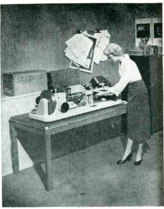
Tabletop model of photoelectric engraver, known as Fairchild Scan-a-graver Cadet, produces 85-screen four-column halftone in 24 minutes after photo is loaded as shown. Amplifiers and tonecorrecting circuits are in separate housing on shelf at rear
