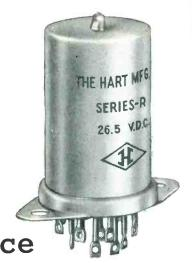
Rating for rating, "Diamond H" Series R hermetically sealed, miniature aircraft type 4PDT relays are smallest (1.6 cubic inches), lightest (3.76 ounces), have widest temperature range ( $-65^{\circ}$  to  $+200^{\circ}$ C.), greatest operating shock resistance (to 50 "G" and higher) and excel all others in their field in ability to break high currents and high voltages.
