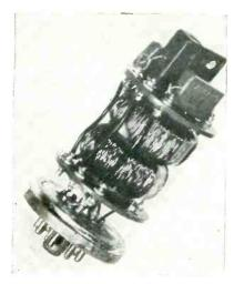
Complete oscillator assembly showing placement of toroids under investigation
