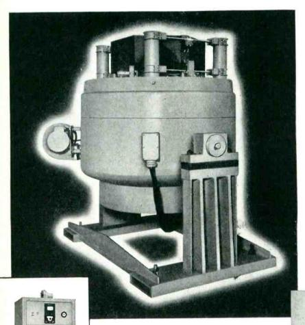
H est - vibration exciter ever built for shake testing. Developed by MB vibration specialists, this unit incorporates all the advances made in the last seven years for assuring dependable operation, pure table motion, and absence of resonances. These include specially designed table flexures, forced air cooling, built in protection against overtravel of the table and against misoperation of the equipment.
