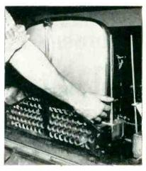
Adjusting position of picture tube with respect to fixture locked in position over front of television receiver chassis. Drilled holes lighten weight of fixture without impairing the rigidity
