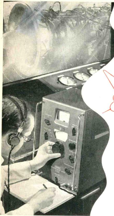
Vibration Analysis with the MUIRHEAD-PAMETRADA WAVE ANALYSER at Armstrong Siddeley works, Coventry
