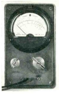
Meter dial and controls of multimeter.
