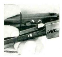
Method of using wire-stripping section of new tool
