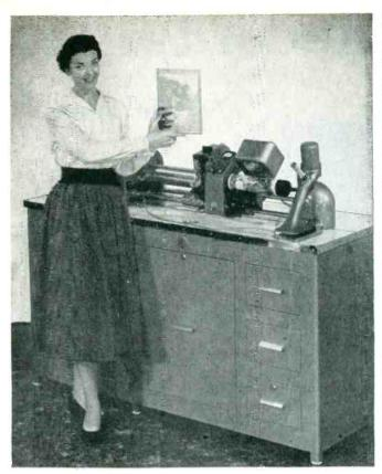
Console model of engraves, with operator holding finished plate. Flashing-lamp microscope is provided for examining dot-burning operation while machine is in operation. All amplifiers are underneath, along with a fireproof compartment for plates
