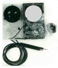
Internal \*parts of multimeter showing printed circuit and switch, at right, that mounts on it
