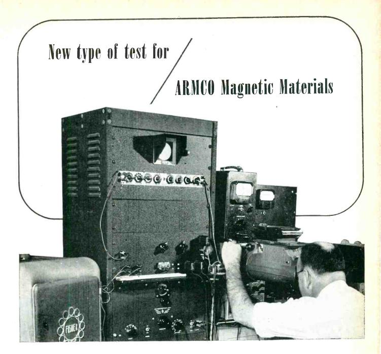
This Armco laboratory technician is measuring the performance of 4-mil thick Armco Electrical Steel under a new test condition. To find out what this steel will do in actual service, the test sample used is a typical magnetic amplifier core. Moreover this core is heated to 105 degrees C and held at this temperature to approximate one of the extremes of working conditions.
