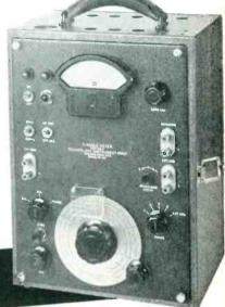
Impedance Range: .5 to 100,000 ohms, covered by a single dial and a four position range switch.
