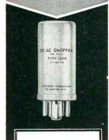
These Choppers convert low level DC into pulsating DC or AC so that serva-mechanism error voltages and the output of thermocouples and strain gauges, may be amplified by means of an AC rather than a DC amplifier.
