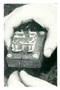
Method of using piano-wire C clamp to hold down ends of outer laminations
