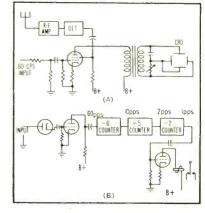
FIG. 1—Circuit for oscilloscope repeater clock (A) and circuit for synchronizing clock to line current (B)
