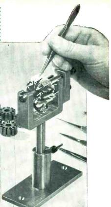
MIGHTY MITES! In spite of their size, Autosyn Synchros must operate with extreme reliability over a wide temperature range. Stators are being assembled in approximately 150 varieties at Eclipse-Pioneer, and strict adherence to engineering specifications is a must. They are insulated with strips of Natvar bias cut varnished cambric because of its uniformly high dielectric strength and flexibility.
