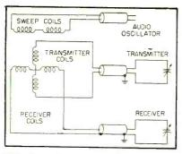
FIG. 2—Probe contains three sets of coils
