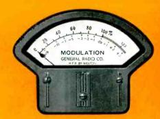
Modulation in both percentage and db is indicated continuously on this meter. Panel switch selects either peak, or indicates both peaks simultaneously. Meter ballistics meet FCC requirements.
