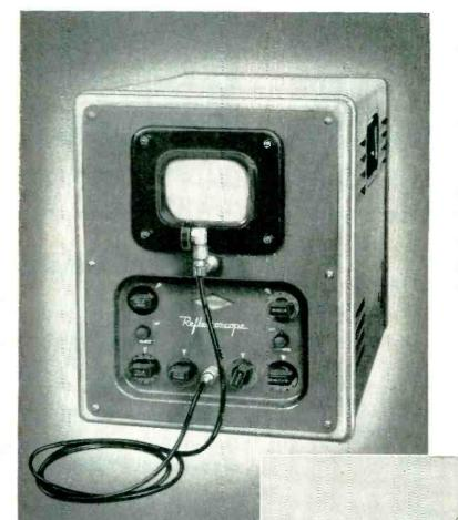
The Sperry ultrasonic Reflectoscope, a compact, portable unit designed for onthe-job inspection, "listens" for defects through as much as thirty solid feet of aluminum and even greater thicknesses in steel and other materials.
