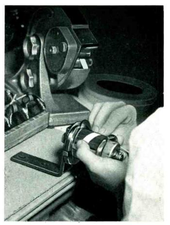
TOUGHNESS AND CONFORMABILITY of "Scotch" Yellow Crepe Paper Tape No. 38 with Thermosetting Adhesive means dependable, compact TV deflection coils.
