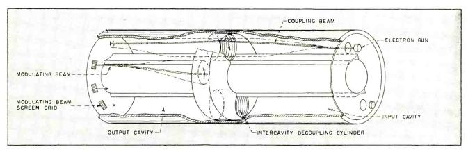
Electron coupler is 18 in. long by  $5\frac{1}{2}$  in. in diameter. Details shown in cutaway include the two coupling-beam electron guns and three of the five modulating beams. Coupling loops are not shown
