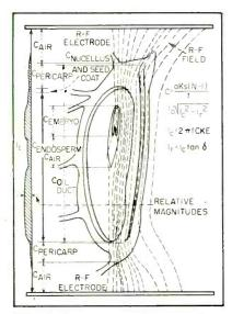
FIG. 1—Course of r-f lines of force longitudinally through a carrot seed
