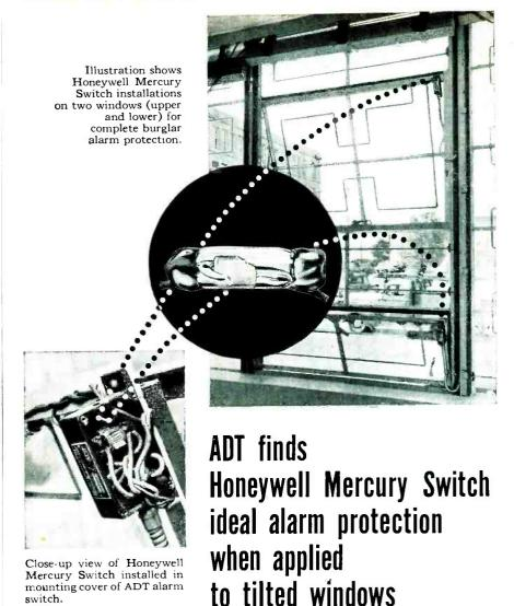
• Electric protection services of the American District Telegraph Company include the use of a Honeywell Mercury Switch as part of the burglar alarm protection applied to horizontally pivoted windows of the fenestra or projected type.
