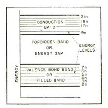
FIG. 2—Energy of a quantized particle, such as an electron. Only the ordinate is to scale. Figure shows how energy, according to quantum mechanics, can change in discrete amounts only, and often in large jumps
