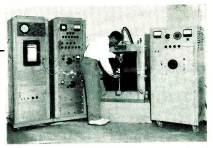
Sample of material being tested (usually liquid) is placed in test tube and inserted between jaws of large magnet where analysis process is accomplished
