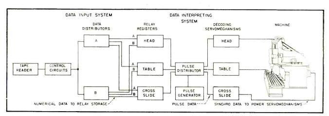
FIG. 1—Tape reader and digital-to-analog converter supply synchro data to power servomechanisms. Orthogonal motions of table, head and cross slide can produce any desired cut
