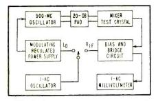
FIG. 6-Production test equipment arrangement
