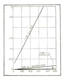
FIG. 2—Gas ratio for any given tube is a constant regardless of emission when gas current in  $\mu \alpha$  is plotted vertically against cathode current in  $\mu \alpha$
