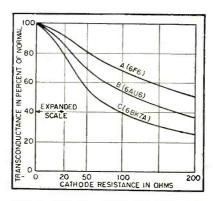
FIG. 2—Loss of transconductance with increasing cathode resistance illustrates effect of cathode interface. Curve A shows low-\(\mu\), low g<sub>m</sub> 6F6, triode connected; B shows medium-\(\mu\) medium g<sub>m</sub> 6AU6, triode connected; and C, high-\(\mu\), high-g<sub>m</sub> 6BK7A
