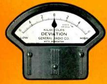
Large-scale illuminated meter continuously indicates frequency deviation of aural transmitter in terms of highly stable crystal oscillator. Zero correction for crystal oscillator easily accessible from panel, to compensate for long-time drift.
