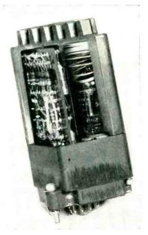
FIG. 1—Navy Electronics Laboratory packaged replacement unit with section cut away to show placement of components
