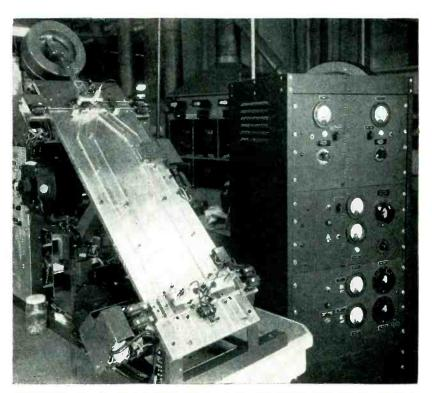
Automatic tester for tiny rectifier plates. Parts are loaded into circular rotating hopper at upper left, sorted according to polarity at V junction in chute, and tested for reverse leakage at bottom. Test rack is at right
