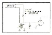
FIG. 7—Simple system claimed to eliminate static and interference
