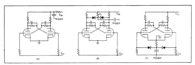
FIG. 6—Flip-flop with triggering network designed for large-amplitude negative pulses or steps (A); for smaller negative pulses (B); and for still smaller negative pulses of short duration (C)
