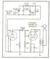
FIG. 1—Diagram of ultrasonic oscillator used in tire inspection unit
