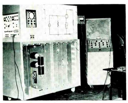
FIG. 1—Classroom demonstration board allows nine different circuits to be demonstrated to a large group. Projection oscilloscope at right makes it possible to show what is happening at various points in the circuit
