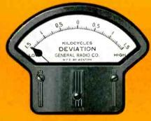
Visual transmitter frequency deviation is continuously indicated by this large scale meter, in terms of the same master crystal
