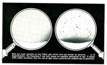
Non-porous FLUOROFLEX®-T rod, tube, sheet assure optimum electrical stability in parts
