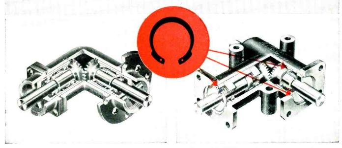
**OLD WAY** 2 Threaded nuts locked bearings in place. 8 screws and washers positioned bearing and shaft assemblies. This fastening method required expensive tapping and threading. Assembly was slow and costly.
