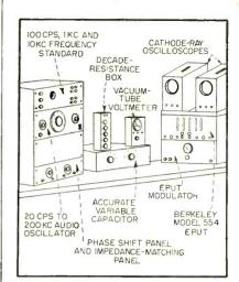
FIG. 2—Filter test station using new method
