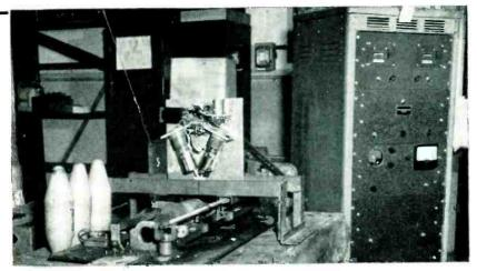
Artillery projectiles are tested by x-ray gauge to detect filler irregularities and voids inside shell
