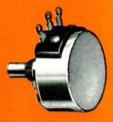
TYPE 25, JAN-R-19, Type RA30) (May also be used as Type RA25) 4 watt, 1 17/32" diameter variable wirewound resister. Also available with other special military features not covered by JAN-R-19 including concentric shaft tandem construction. Attached switch can be supplied.
