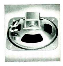
RADIO, TV SPEAKERS—In these speakers, current passes through the voice coil which is the magnetic field set up by the Carboloy permanent magnets. The uniformity and strength of the magnets help produce truer tone.
