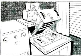
Grant Industrial Slides were used. With them, units may be withdrawn and locked in a fully extended position in a matter of seconds, with no more effort than opening a filing cabinet.
