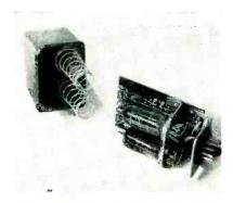
FIG. 3-Mounting board and tube chassis. Terminals are placed on board depending on type of circuit being wired
