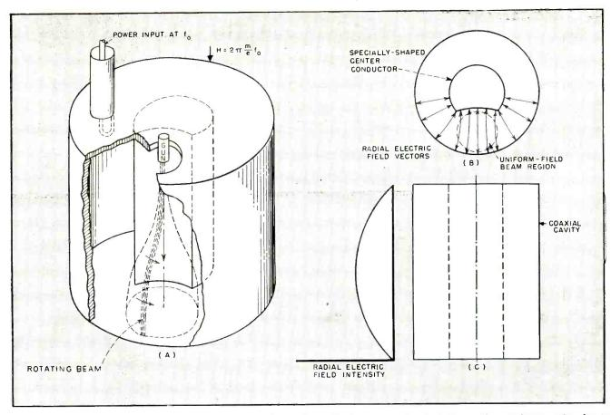
FIG. 1—Rotating coupling beam in coaxial cavity has milk-bottle shape (A). Transverse electric field is uniform in beam region due to specially-shaped center conductor (B) and varies sinusoidally along axis of cavity
