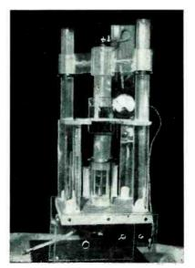
Preliminary experiments were carried on with oscillator using two 5-250A tetrodes
