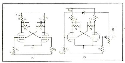
FIG. 1—Basic bistable multivibrator circuit (A) is modified for switching (B) by adding triggering network
