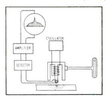
FIG. 10—Alternative technique using electronic sweep for flaw detection
