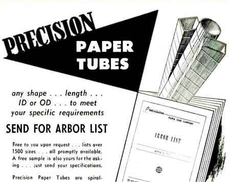
Precision Paper Tubes are spiralwound of finest dielectric kraft, fish paper, cellulose acetate, or combinations.
