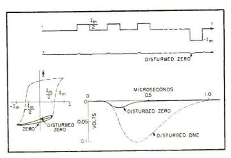
FIG. 5—Results of pulse test used to determine largest possible voltage from a toroid holding a zero
