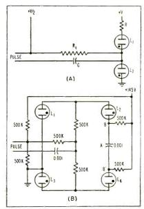
FIG. 1—Basic circuit (A) used in flipflop and binary counter. Flip-flop (B) uses NE-2 neon lamps
