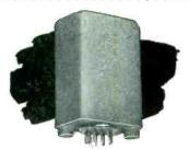
R 94 SERIES—Hermetically sealed small telephone type relay with pin hinge construction for long life. Available in D.C. only with contact springs up to 4 pole doublethrow. In 1 amp., 3 amp., or 5 amp. capacity. Plug-in or solder terminals. Overall size 1-5/8 x 1-1/32 x 2-1/4 D.
