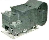
The Century Model 409 Oscillograph has been designed for recording data where space and weight requirements are limited. The Oscillograph has been tested to record faithfully while subjected to accelerations up to 20 G's.
