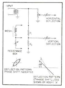
FIG. 4—Method of using resistance decade box to determine effective a.c resistance of a mesh
