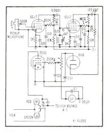
FIG. 2—Receiver circuit for ultrasonic tire inspector
