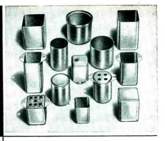
hot tin dipped . . . fabricated terminal and vent holes . . . smooth, one-piece construction using cold rolled steel . . . draw depths up to  $2\frac{1}{2}$ " . . . inside fit covers for easy hermetic sealing in all sizes . . . available as stock sizes and as special fabrications.
