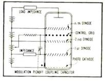
FIG. 11—Electron multiplying device applicable to television
