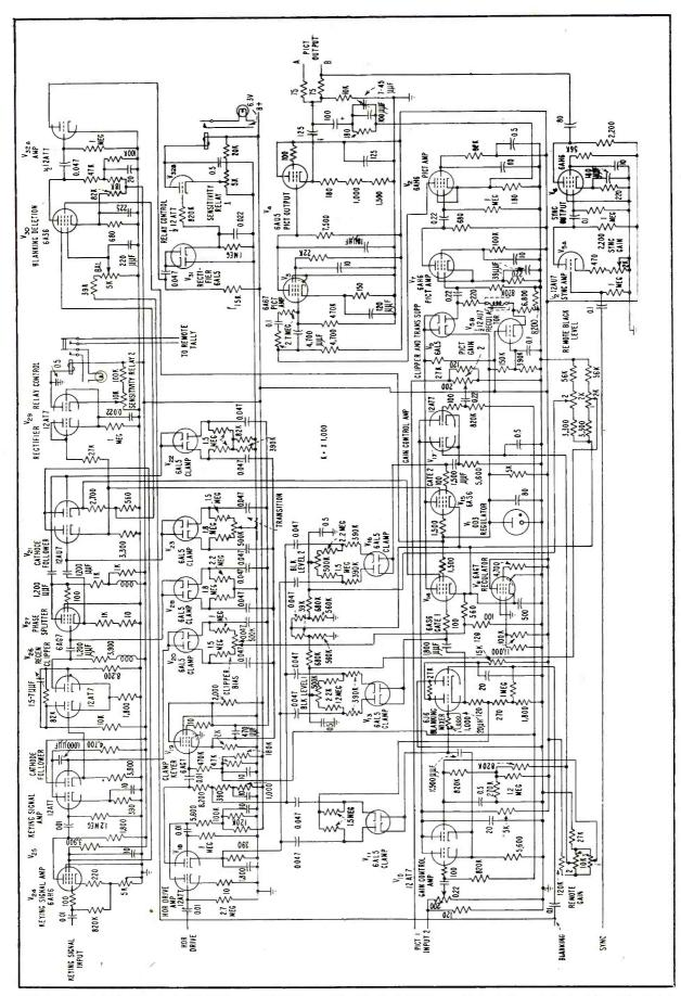
FIG. 5—Schematic diagram of the RCA type TA-15A special effects amplifier used as an integral part of the video inset system
