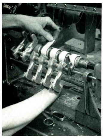
**STRONG THERMOSETTING ADHESIVE**, tough backing and thin caliper make "Scotch" Yellow Flat-back Paper Tape No. 39 ideal for outside wraps on primary windings.
