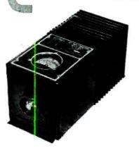
This series of instruments was designed to measure RF power up to 400 watts, and serve as an excellent dummy antenna load over the frequency range 50 to more than 1000 MCS in 52 ohm coaxial line circuits.
