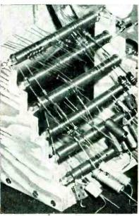
Stand made from springs, metal strips and plywood here holds parts needed for three terminal board subassemblies. Operator keeps original sample in front of her to serve as guide, supplementing prints mounted above sample
