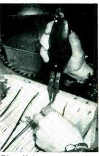
Using soldering tweezers to get heat exactly where it is needed on a joint
