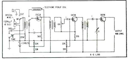
FIG. 2—Circuit diagram of Zenith hearing aid using transistors exclusively. Battery cost is 1/25 that of comparable all-tube instrument
