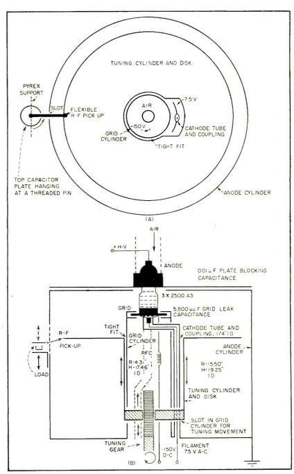
FIG. 2—Cross section of cavity oscillator (A) tuning cylinder at level of upper loading plate and (B) vertical section details
