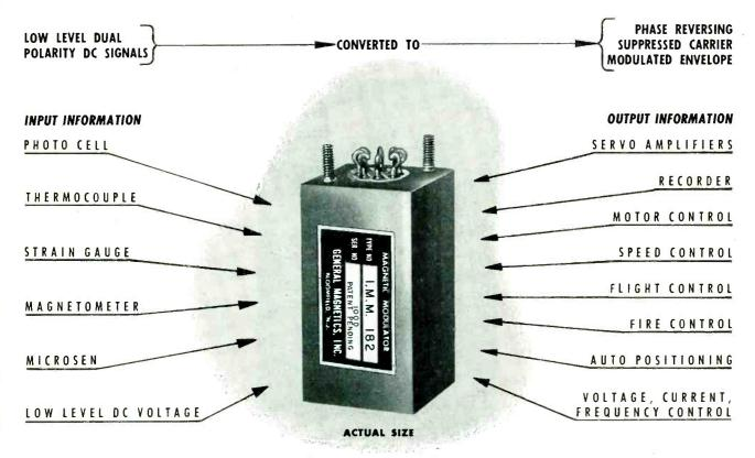
he IMM 182 Magnetic Modulator is designed to convert low level dual polarity DC signals into 400 cycle signals of corresponding amplitude and phase sense.
