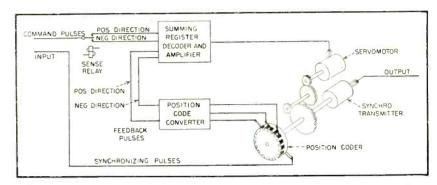
FIG. 3—Digital-to-analog converter changes input pulse data to equivalent shaft rotation. Commutator-type coder wheel generates feedback pulses for checking
