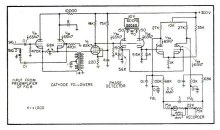
FIG. 9-Differential amplifier and phase sensitive detector circuits. Signals from preamplifiers feed differential transformer with toroidal core
