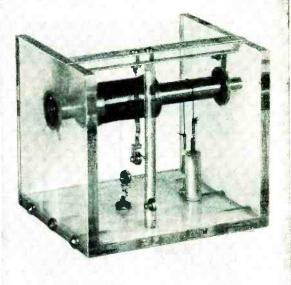
Slotting device for preparing delay line cores. Indexing head is shown in foreground
