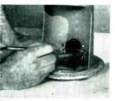
Cutting a piece of hard, brittle metal manually by means of the "Airbrasive"
