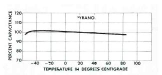
Capacitance vs. Temperature is shown by this typical curve. G-E Pyranol subminiature metal-clad capacitars have only a small capacitance change through the entire range from -55 C to +85 C.
