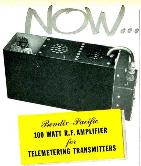
This new Bendix-Pacific TAV-2 Amplifier will extend the range of low power transmitters, such as the Bendix-Pacific TXV-13, by increasing the output power. It nominally provides 100 watts of RF output power to a 50 ohm load through a type N coaxial fitting. The unit requires two watts drive at 50 ohms. The power connection is a multicontact, quick disconnect plug.
