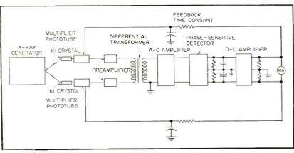
FIG. 1—Block diagram shows self-balancing bridge arrangement of differential x-ray gauge whose output is independent of line voltage variations
