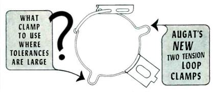
Augat two-tension loop clamps are the long-sought answer for uses where socket tolerances vary up to .040. The bands of these sturdy clamps are made of Beryllium copper, heat treated to retain original tension and nickel plated to withstand a 96 hour salt spray test with no adverse effect.
