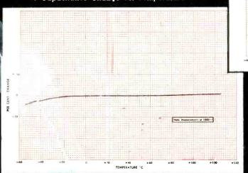
These graphs show typical performance characteristics of the Pyramid "Glasseal X" type, which is designed for 125°C. operation. Full information on all "Glasseal" capacitors is provided in new catalog PG-3.
