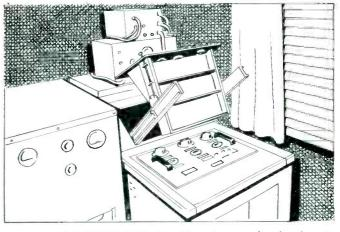
A full 90° tilt brings the wiring under the chassis into full view for repair. Unit locks at this and other angles, and may continue to operate in any of these positions.
