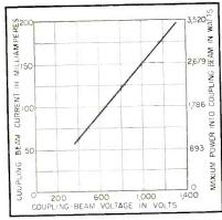
FIG. 3—Input cavity presents match to 50-ohm line over wide range of coupling-beam current and voltage
