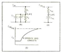
FIG. 4—Effect of coupling capacitor on switch-over
