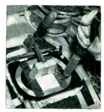
Flattening plastic peg by applying heat and pressure with electric soldering iron, while clamping jig holds antenna flat against inside of cover for threeway radio
