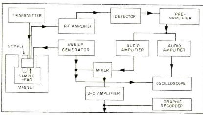
FIG. 1—Block diagram shows use of r-f transmitter, receiver and associated equipment
