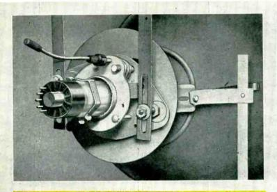
The external ion-trap magnet on this standard tube, is an extra cost item for the TV manufacturer and requires special adjustment. The focus coil and complicated mounting also mean extra cost. They take up space, add weight, consume assembly and adjustment time. Get rid of all three parts with G. E.'s new i-m-f tube!
