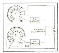
FIG. 2—Dynode feedback reduces unbalance between the two phototubes by varying their dynode potentials
