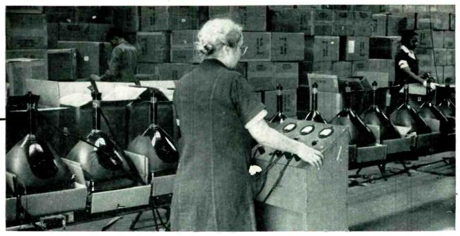
Gas-buggy test unit used at Electronics Park plant to check for gas in tube and leakage between elements, at rate of one tube per minute. Four tubes are connected at a time so that three are being preheated while the fourth is checked. Tubes are aged for several days in storage before this final checkup
