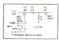
FIG. 1—Effective lens capping for a camera in the TK-10A chain is accomplished by insertion of a toggle switch as shown
