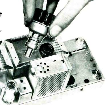
Motorola's 18-20 watt RF power transmitter uses two Eimac 2C39A's
