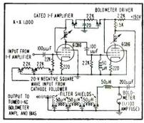
FIG. 5—Measurement of relative output noise power is obtained with this circuit
