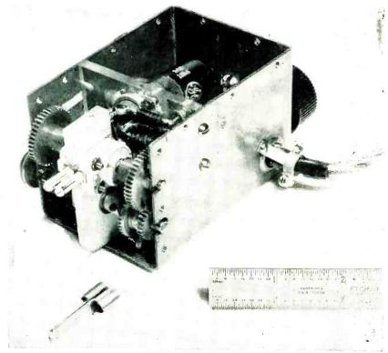
Experimental model using ceramic capacitors covers the frequency range from 430 to 975 mc continuously
