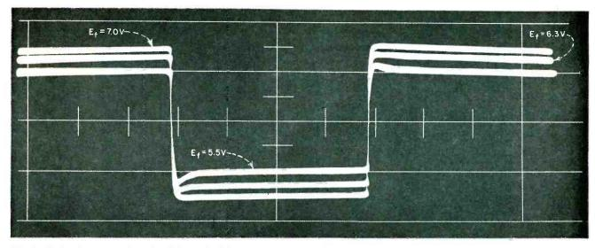
FIG. 3—Plate-voltage waveform for 6AH6 with 50-kc square-wave excitation. Overshoots due to cathode interface resistance are noted as heater voltage is reduced
