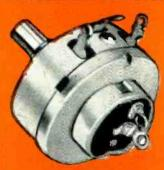
TYPE GC-25, 4 wett, 1 17/32" diameter variable wirewound resister. Available with or without illustrated attached switch and in concentric shaft tandem construction C2-25 as shown above.
