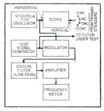
FIG. 1—Block diagram illustrating method formerly used for measuring frequency during testing of filters for carrier telephone and telegraph equipment
