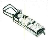
This 25-milliwatt f-m transmitter was designed by Motorola engineers to extend the range of the microphone used with a loudspeaker system in railroad yards. It operates in the 152-to-174 mc band, produces a 15-kc deviation and measures approximately 2  $\times$  3  $\times$  7 inches
