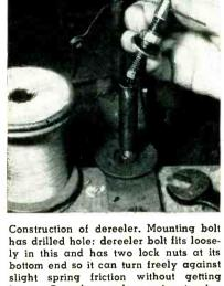
loose. Dereelers reduce wire tension and make it more constant, since heavy spool does not turn
