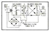
FIG. 12—Analyzer for combustible gases
