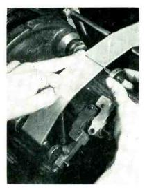
Inserting arbor pin to lock start of next winding after indexing head to bring newly-finished capacitor forward
