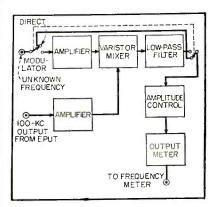
FIG. 5—Block diagram of Eput modulator
