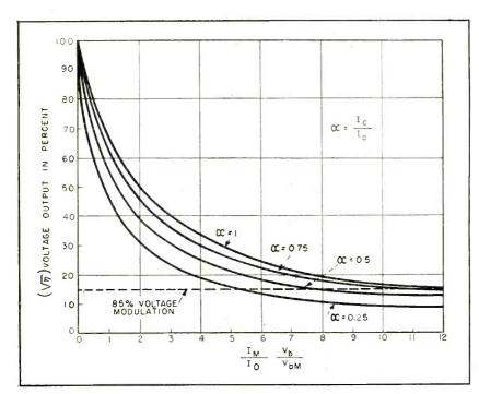
FIG. 2—Voltage output is function of optimum coupling-beam current, modulating beam current and operating parameters of tube
