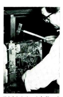
Method of using improvised rubber mallet to check for intermittents
