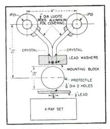
FIG. 4—Details of balanced x-ray detector system with two scintillation crystals fixed a small distance apart to allow scanning complete volume
