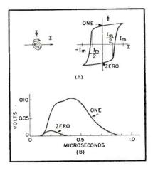
FIG. 1—Characteristic curve (A) of ferrite toroid. Voltages produced (B) by α one or zero stored in α toroid
