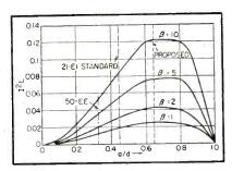
FIG. 2—Curves for silicon steel, showing that optimum core shape is obtained at a dimension ratio a/d of about 0.65
