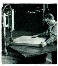
Trimming excess metal from edge of formed shell for electronic equipment housing. Rollers on bottom of pressure arm permit sidewise movement while maintaining downward pressure
