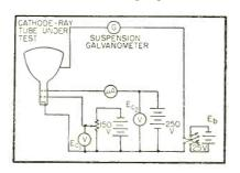
FIG. 1—Circuit used for laboratory version of gas ratio test unit
