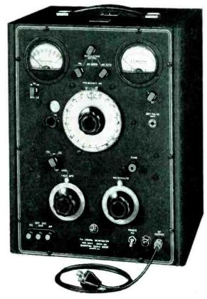
modulation is less than 3% and for 50% AM less than 6.5. At 100% the distortion is 12% to 15% depending upon the modulating frequency.
