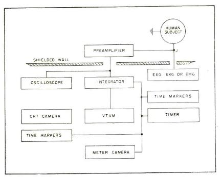
FIG. 1—Arrangement of instruments used to study human strain and effort by measuring bioelectric potentials
