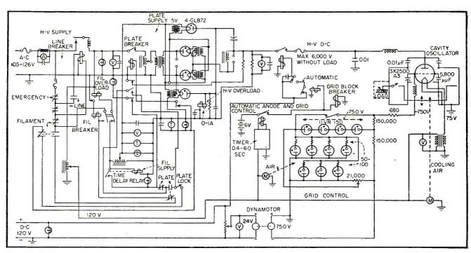
Circuit diagram of the radiation equipment includes timer for accurate dosage and safety controls for nontechnical personnel
