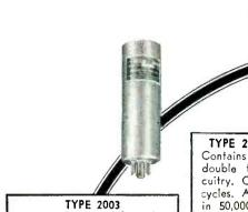
TYPE 2003 Same as Type 2007 (at right) except Tube 12AT7 and 5 pigtail components are external. TYPE 2007, BASIC UNIT Contains shock-mounted fork, double triode and all circuitry. Output, 400 or 500 cycles. Accuracy ± 1 part in 50,000. Octal base container, 1½" x 4½". Weight, 10 oz. Power required, 75 to 200 V-D.C. at 1 to 5 m.a. and 6.3 V. at 300 m.a. De-
