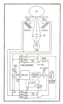
FIG. 1—Shell-color determinator utilizes light reflected from egg shell through red and blue filters to photocells
