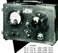
The input circuit is a type N connector (UG-58/U) . . . The output is monitored by a 1N21B crystal and microammeter circuit with adjustable sensitivity control for varying input power levels. The output of the crystal may be obtained from pin jacks provided on the panel of the instrument. A switch is provided to change the output from the microammeter to the pin jacks.
