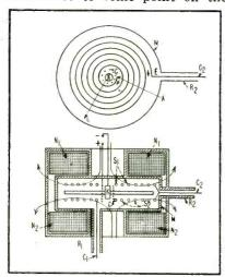
FIG. 4—Spiral traveling-wave tube ele-
