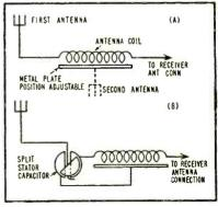
FIG. 2—Two methods of coupling opposing interference signals
