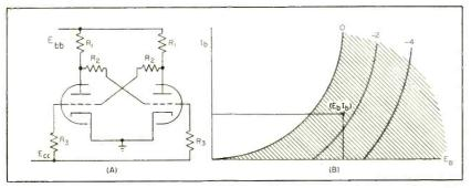
FIG. 2—Rudimentary circuit for steady-state design (A) and tube characteristic (B) showing operating point
