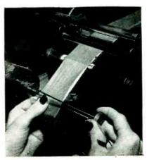
Inserting arbor pin to lock start of winding on single-capacitor machine
