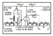
FIG. 4—Contents of Y-factor box used in noise temperature test
