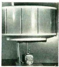
Carousel contains basic colors that are mixed according to the setting of controls. Using this electronic device, the merchant can avoid large inventories of seldom-used colors
