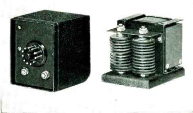
400-CYCLE PLUG-IN AMPLISTAT is a push-pull output DC linear amplifier with three separate input windings. Tube-type base simplifies mounting.
