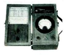
Compact test meter for audio signal level and recorder bias. A 100  $\mu \alpha$  movement is used
