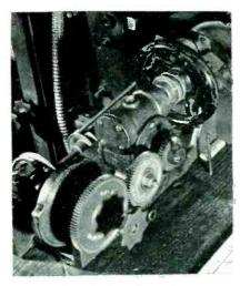
Headstock end of dual semi-automatic machine with protective housing removed to show cam and quick-change gears that shut off machine when correct number of turns is wound. Push rod under cam goes down through table to actuate motor clutch
