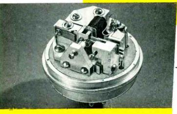
View of Clare Type T High Frequency Impulse Relay with dust cover removed
