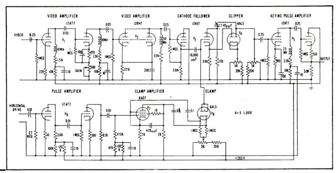
FIG. 3—Circuit diagram of the NBC keying separator amplifier
