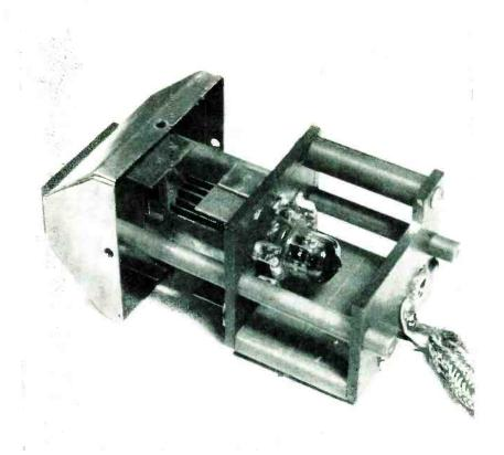
Final version uses 6F4. Tube and circuits are mounted on movable carriage
