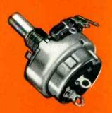
TYPE GC-35, 1 1/8" diameter variable composition resister. Wattage rating: 3/4 watt for resistances through 10,000 ohms, 2/3 watt for resistances over 10,000 ohms through 25,000 ohms, 1/2 watt with 500 volts maximum across end terminals for resistances aver 25,000 ohms. Available with or without illustrated attached switch and in concentric shaft tandem construction C2-35 as shown above.
