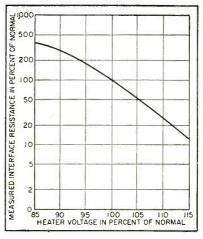
FIG. 1—Measured values of cathode interface resistance plotted as a function of heater voltage
