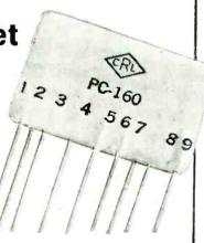
Talk about compactness—this new Pendet has it! You get 4 resistors and 5 capacitors screened and fired to a single Ceramic-X plate. It replaces 9 conventional components. Only 9 connections are required instead of the usual 18.
