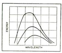
FIG. 1—Black-body radiation curves, showing variation of energy with wavelength. Energy increases with absolute temperature, and the peaks shift toward the shorter wavelengths
