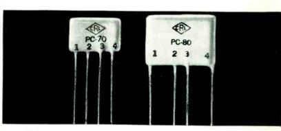
**CENTRALAB TRIODE COUPLATES** replace 5 components normally used in audio circuits. Triode Couplates are complete assemblies of 3 capacitors and 2 resistors bonded to a dielectric ceramic plate. Available in a variety of resistor and capacitor values. Technical Bulletin 42-127.
