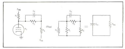
FIG. 5—Equivalent circuit showing the effect that the coupling capacitor has **on** the triggering rate
