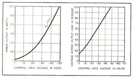
FIG. 4—Power and voltage outputs versus control-grid voltage for peak power output of 300 watts, corresponding to 750 volts beam voltage
