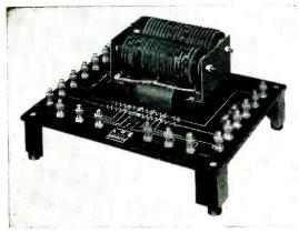
**EDUCATIONAL-LABORATORY AMPLISTAT (10**volt-amperes) has multiple input for flexibility. Diagram molded into panel allows easy demonstration.
