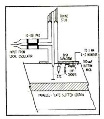
FIG. 3—Local oscillator injection and monitor probes
