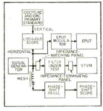
FIG. 3—Block diagram illustrating new method employing an Eput (events-perunit-time) meter to indicate frequency
