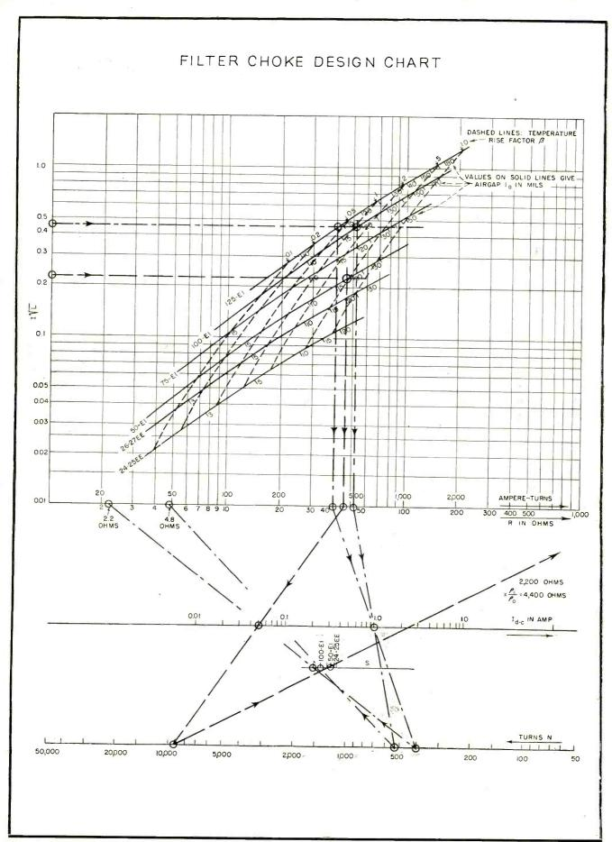
FIG. 3—Calculation chart for chokes using 7-mil laminations of 4-percent silicon steel with square stack. Dash-dotted lines show solution worked out for Example 1, and long dashed lines apply to Example 2
