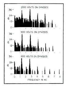
FIG. 10-Output spectra of 1P21 tube at various accelerating voltages indicate better signal-to-noise ratio at lower dynode voltages
