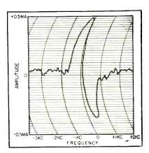
FIG. 4—Record of blip showing abundance of oxygen 17 in water. Nuclear resonance is at point where curve crosses centerline
