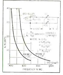
FIG. 3—Variation of  $k_1$  with frequency for grid-dip meter using series tuning
