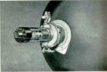
Now, no hard-to-adjust external ion-trap magnet! No focus coil, or external focus magnet, with cumbersome bracket! Instead, an *i-m-f* tube calls for just two parts when installed, both of them compact: (1) a close-fitting steel shunt band that is easily slipped on and (2) a small centering device to position the picture.
