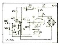
FIG. 9-One kilocycle millivoltmeter for production testing
