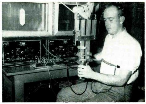
Electrodes take bioelectric potentials from arm muscle and frontal lobe of brain to measure strain and effort of subject exercising on isometric dynamometer
