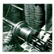
Left hand of operator is holding forked tool used to push out first half of split arbor preparatory to releasing finished units. Winding is already under way here on the next two units
