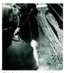
Method of using air gun to twist filament leads together after they have been cut and stripped on an Artos machine
