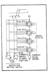
FIG. 3—A four-position magnetic matrix switch using ferrite toroids
