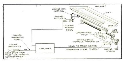
FIG. 2—Power servomechanism controlling table motion consists of synchrocontrolled hydraulic rotary transmission driving lead screw. Identical units control head and cross slide
