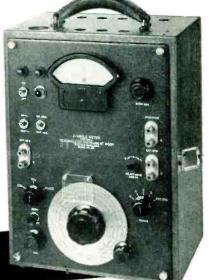
The type 310A Z-Angle Meter measures impedance directly in polar coordinates as an impedance magnitude in ohms and phase angle in degrees: Z 🖰
