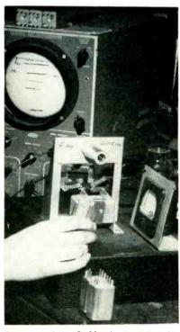
Setup used in DuMont's incoming inspection department to check i-f transformers. Jig gives free access to adjusting screws at both ends of the transformer
