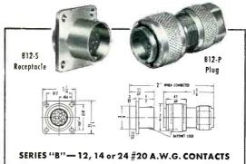
The cadmium plated aluminum die cast shells are available in % and 1-7/32" dia. with bayonet locking for quick engage and disengage. Shells have synthetic rubber gaskets. Flanges permit mounting of receptacle in panel or housing and special gland construction provides cable entry in plug,
