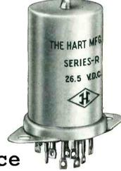
Rating for rating, "Diamond H" Series R hermetically sealed, miniature aircraft type 4PDT relays are smallest (1.6 cubic inches), lightest (3.76 ounces), have widest temperature range (-65° to +200°C.), greatest operating shock resistance (to 50 "G" and higher) and excel all others in their field in ability to break high currents and high voltages.
