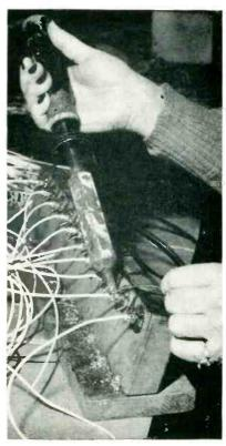
Jig for holding phono-type plugs while soldering leads to outer skirts of plugs for use as speaker cables. Plugs were previously soldered to the center conductor at a dip soldering operation
