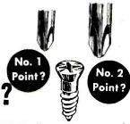
The Phillips screw and the two XCELITE Phillips points are shown actual size. You <u>can</u> use the #1 point—but it will fit somewhat loosely, and damage results to both screw and point. The #2 point does fit snugly, even though it <u>appears</u> too large. So, to make your points last longer, always try a size larger screwdriver than you think would fit.
