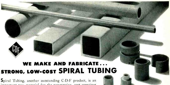
important new material for the progressive, cost conscious design engineer (and purchasing agent). It is a high strength plastic made from paper or fibre that is spirally wound, then impregnated with phenolic resin or insulating varnishes and carefully cured at high temperatures. The resulting tubes (round, square, rectangular or formed to special shapes) are stiff, sturdy, resistant to crush, with good tensile strength.
