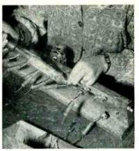
Jig for holding and rotating nine subminiature sockets simultaneously
