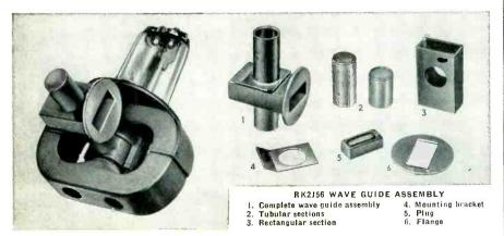
RK2J56 Magnetron and Wave Guide Assembly. Courtesy Raytheon Manufacturing Co., Waltham, Mass.
