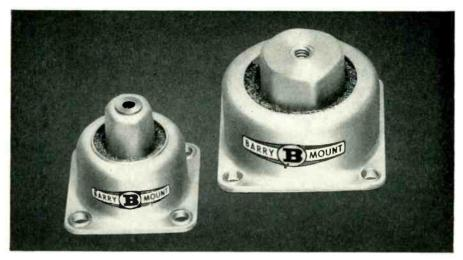
The new Type 7630 and Type 7640 ALL-METL Barrymounts have been specifically designed to eliminate loss of efficiency due to damper packing. Previous wire-mesh unit vibration isolators exhibited a definite loss of damping efficiency after a period in actual service, because the wire-mesh damper tended to pack. These new unit Barrymounts have eliminated this difficulty, because the load-bearing spring returns the damper to its normal position on every cycle.
