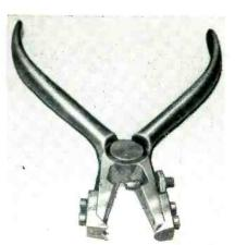
Long-nose pliers as modified for wire stripping
