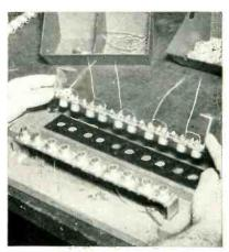
Two-position jig for assembling jack strip of distribution amplifier for field television camera
