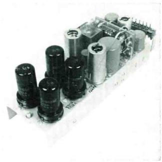
Control weighs  $2\frac{1}{4}$  lbs, compared to 6 lbs or more for previous model. Built on plug-in chassis, unit reduces servicing problems
