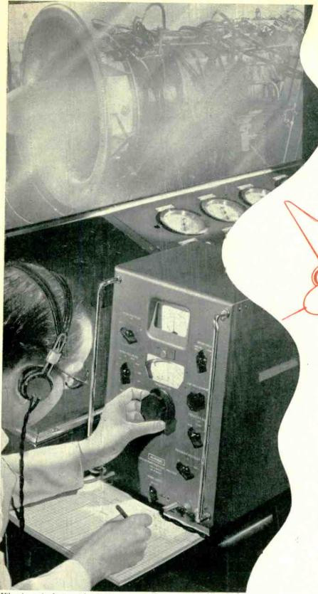
Vibration Analysis with the MUIRHEAD-PAMETRADA WAVE ANALYSER at Armstrong Siddeley works, Coventry
