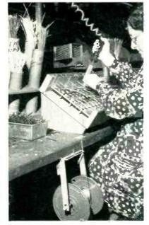
Fixture for holding three-potentiometer strips. Soldering iron is plugged into overhead outlet, and rests in horizontal holder at back of bench when not in use. Solder reel holder is screwed to bottom of bench
