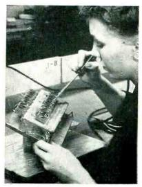
This chassis support jig rotates on an angle-cut pedestal. Spinning the jig changes the angle as required for optimum work with the pencil-type solder-ing iron
