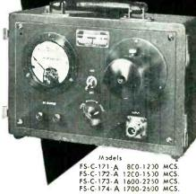
The input circuit is a type N connector (UG-58/U) . . . The output is manitored by a 1N21B crystal and microammeter circuit with adjustable sensitivity control for varying input power levels. The output of the crystal may be obtained from pin jacks provided on the panel of the instrument.
