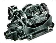
Erection motors: 5 watts (each), Caging operation: 12 watts (operating); 6 watts (standby).
