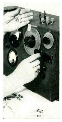
Testing small choke coils by using calibrated terminals on top of Q meter
