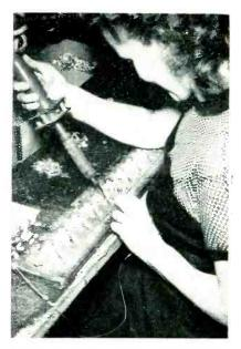
Recessed jig for trimmer subassembly work
