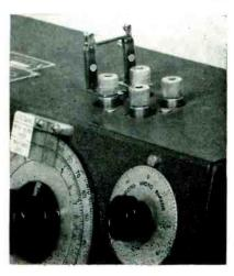
Calibrating bar in place on Q meter
