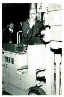
Two-way radio on lift truck
