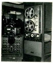
Test setup for evaluating short sample method of measuring flutter introduced by magnetic tape recorders used in guided missile instrumentation. Discriminator is on panel below tape recorder. Dual-beam oscilloscope and recording camera are at left
