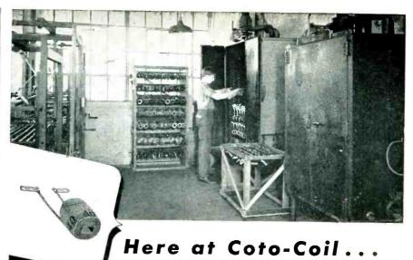
Finished coil impregnated with varnish coating ... the Impregnating Department applies the final protective coating to precision-made Coto Coils. Each coil is pre-heated, immersed in varnish and drained . . . sometimes 3 or 4 times. The varnish finish, baked in these modern ovens, not
