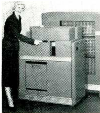
Electronic calculator made by IBM has 1,400 tubes. Over 1,000 of the machines are now used in business offices in the U. S.
