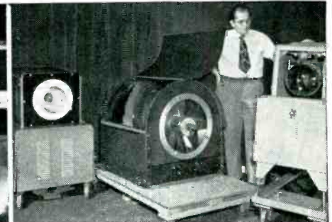
Rauland large-screen projectors using three different optical systems, all of which give theater-size pictures.
