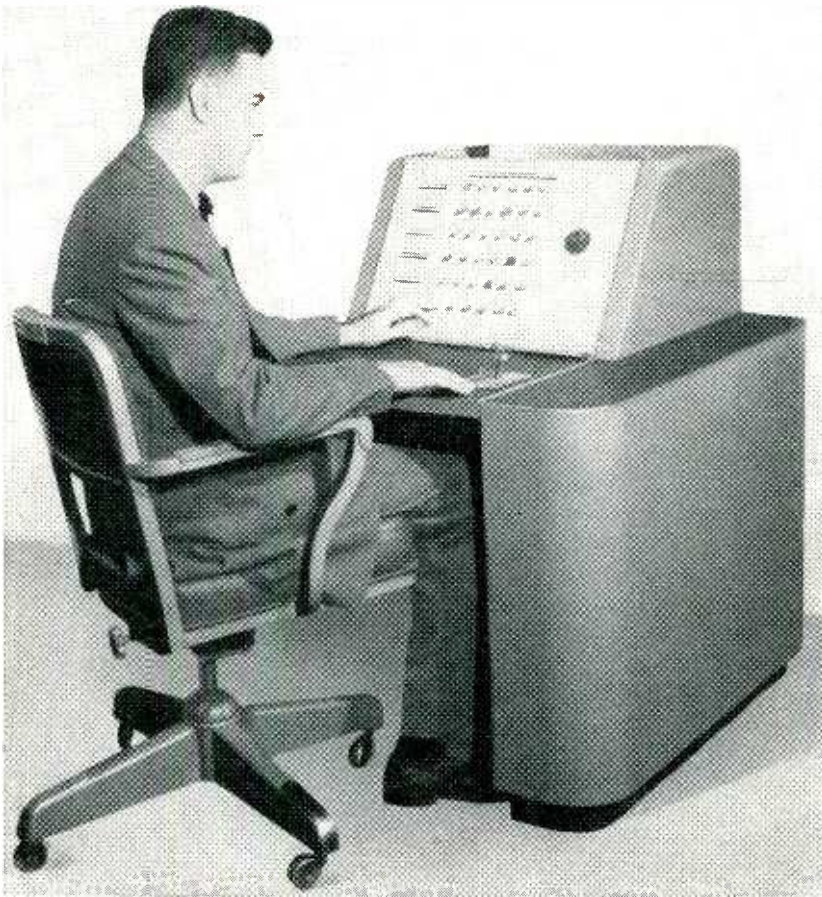
Control console with six inputs and six outputs can be expanded with growth in studio operations. Relays normally furnished in console can be remotely operated if it is desired to shorten video lines
