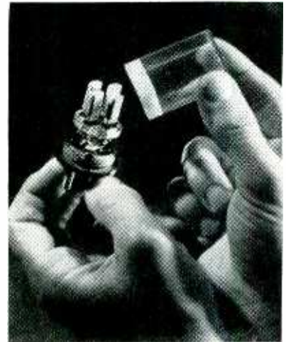
In this four-transistor audio amplifier pnp and npn types are combined to provide transformerless class-B amplification with direct coupling to loud-speaker voice coil
