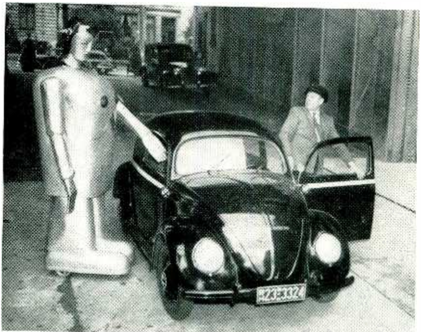
Mr. "Sabor IV" the 500-pound robot shown in the photograph, has its movements directed by a built-in short-wave radio receiver. Cost of the metal giant was $7,140
