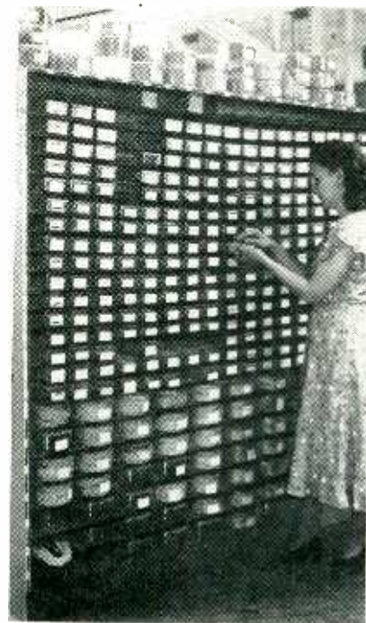
Rack for plastic boxes containing pre-cut wires
