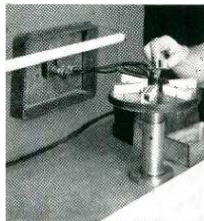
Six-position pedal-operated work table brings tin-plated steel housings under work coil for soldering of seams. Strips of precut solder are in wood box, and unsoldered housings are stacked neatly on table. Finished housings go into bin on floor at right of operator
