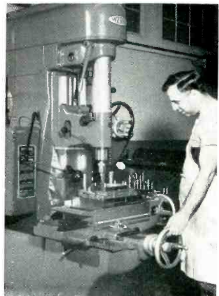
Use of new jig borer in Sylvania's Buffalo plant for drilling required holes in punching die for auto-radio switch contact
