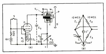
FIG. 1—Simple circuit diagram for thyratron-controlled electromagnetic system (A) and grid control via hand-capacitance bridge (B)
