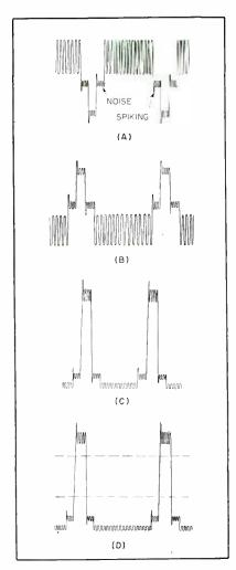
FIG. 4—Operation of sync-channel cleanup of spiking
