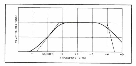
FIG. 4—Average system amplitude characteristics showing relative frequencies in megacycles
