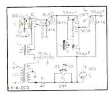
FIG. 1—Schematic diagram of the linearity test generator for tv adjustment
