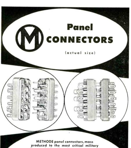
produced to the most critical military quality standards, offer substantial current carrying capacity for a multiplicity of conductors in compact polarized arrangements of 11, 15 and 20 terminals. Insulator blocks are type MFE low loss mica filled phenolic, per MIL-P-14A. Silver plated plug pins of micro-machined brass alloy and socket contacts of precision fabricated beryllium copper feature easily wired solder dipped terminals. Small pins are .040" diameter and large pins .093" diameter.
