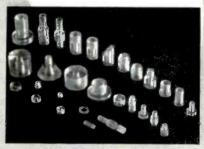
Rexolite 1422 has been specifically designed and developed to meet the growing need for a lightweight - low cost U. H. F. insulating material.
