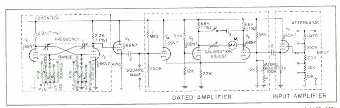
FIG 3—Complete circuit, less power supply. The multivibrator range switch provides frequency-multiplying factors of 2, 10, 100, 1,000 and 10,000. Auxiliary terminals are provided for using the square wave output of the multivibrator separately
