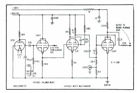
FIG. 3—Record modulator-amplifier converts a-m signal from electronic accelerometer to pulse-width modulated wave train for recording on magnetic tape
