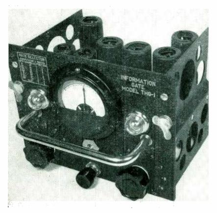
Information gate is basic building block of electronic decommutator
