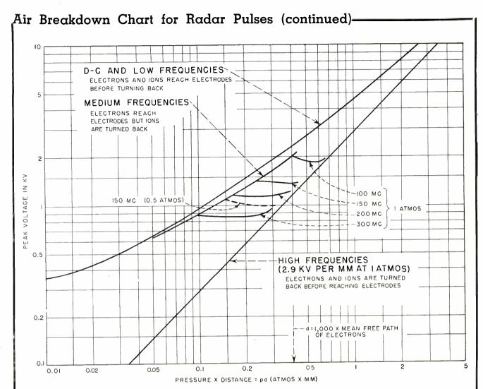
Chart giving breakdown voltage in air between parallel planes. For atmospheric pressure, horizontal scale represents distance in millimeters between the plane electrodes
