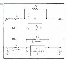
FIG. 1—Basic analog computer element consists of an input impedance, a d-c amplifier and some form of feedback loop
