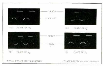
FIG. 4—Oscillograms show waveforms on plates of meter tubes
