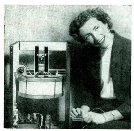
Operator playing the electronic drum. The electromagnetic system is mounted above the drum diaphragm
