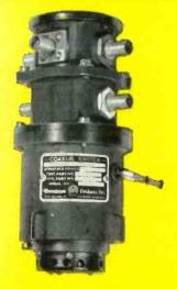
Model CA-31, 2P2T Sensing or Lobing Switch, 115 volt, 380-1000 cycle AC motor actuator. Switching speed, 15-35 Rev/sec. For use with RG-58/U cable.
