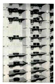
Rack used for storing socket panels. Some have a special top-cap connecting lead or a shield-connecting spring
