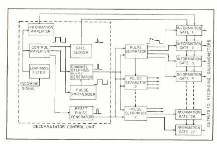
FIG. 3—Block diagram of electronic decommutator for 27 channels. Counter circuits supply sequencing trigger pulses to information gates
