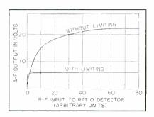
FIG. 4—Action of dry-battery limiter stage of receiver
