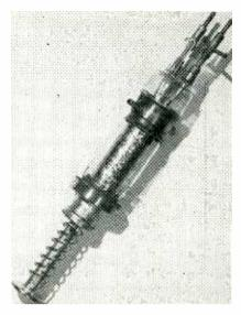
Pure-tungsten hot cathode with maximum heating power of 5 kw
