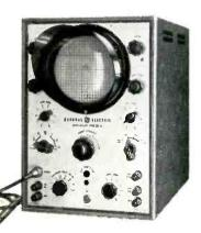
TypeST-2A-For general purpose use in laboratories. Excellent wide frequency response for TV receiver circuit work and industrial testing. Special features include a DC vertical amplifier to adapt the equipment to a wide range of applications. Deflection pattern can be expanded to several times the diameter of 5-inch tube.
