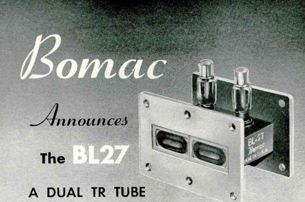
Each section of the BL27 is electrically similar to Type 1863A. The two sections have a common wave guide wall and a common gas fill. Used with short-slot hybrids.\* the BL27 provides a highly compact duplexer of utmost simplicity, with excellent performance over the band of 8500-9600 mc. with respect to both transmission and reception characteristics.
