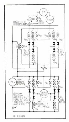
FIG. 2—Complete circuit showing parts values for 60-cps and 400-cps (in parenjheses) two-stage magnetic servo amplifiers
