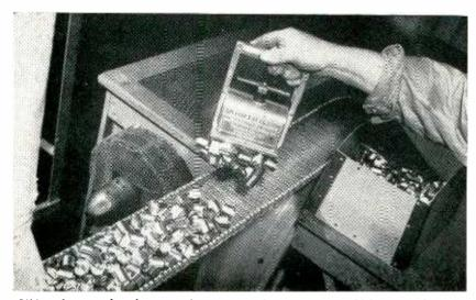
Lifting hot anodes from moving woven-wire conveyor which runs through baking oven
