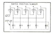
FIG. 5—Portion of special instruction section of switch matrix
