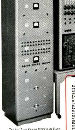
Typical Low Priced BECKMAN EASE COMPUTER Installation showing 20-channel operational amplifier and power supply, 2-channel function generator, 3-channel function multiplier, typical variable component and over-voltage panel, 30-channel
