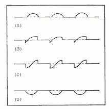
FIG. 1—Curves show output of gated amplifier for sinewave input at various phase angles
