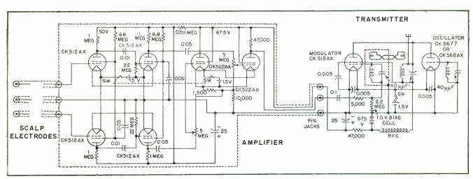
FIG. 1—Portable voltage amplifier and transmitter of radioelectroencephalograph, in two housings having total weight of only 2.6 lb
