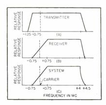
FIG. 2—Standard tv broadcast system transmission-amplitude characteristics
