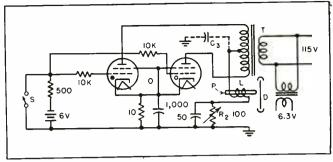
FIG. 2—Practical direct a-c type thyratron circuit free from mechanical contacts. Thyratrons are connected in push-pull arrangement
