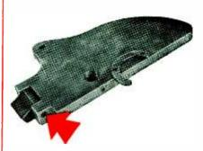
AS A CLEVIS PIN... here Rollpin holds firmly in clevis, permits free action of moving member. Rollpin application above is with the plate of a home workshop tool.
