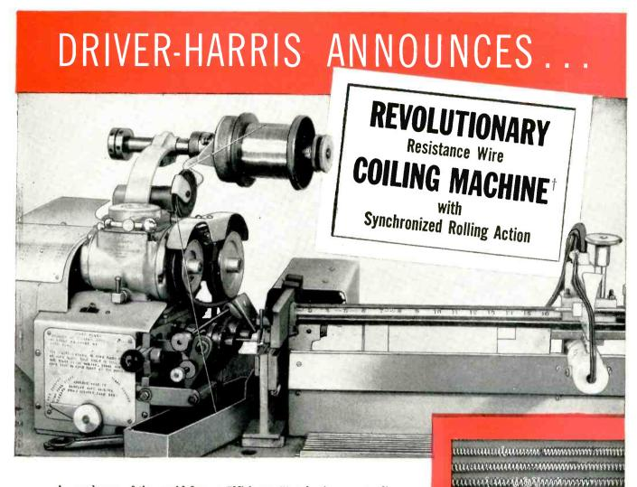
As producers of the world famous "Nichrome"\* and other outstanding electric heating and resistance alloys, Driver-Harris engineers are interested in obtaining application results commensurate with the exceptional advantages their alloys afford. Therefore they have developed a new coiling machine which eliminates wire coiling faults—especially coil irregularity due to work-hardened areas produced during coil formation.
