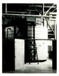
White-cedar sonar test tank at NADC is used in calibration of barium-titanate transducers
