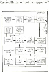
FIG. 1-Block diagram of the polyneumograph
