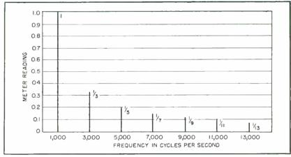
FIG. 7—Chart shows analyzer readings for 1,000-cps square-wave input
