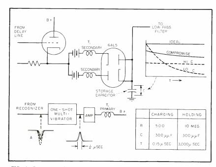
FIG. 9—Recognizer drives receiver gate through multivibrator and balanced transformer
