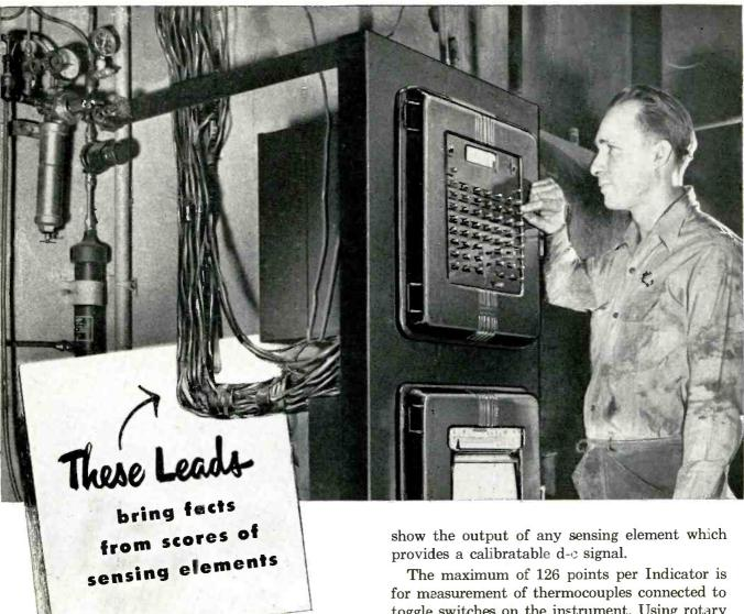
The scientist or test engineer who has a Speedomax Model G Electronic Indicator at his disposal is ready to save himself a lot of time and energy in running tests at as many as 126 different locations.
