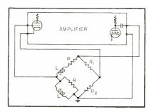
FIG. 1-Basic schematic of oscillator
