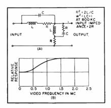
FIG. 7—Amplitude-correcting network for use at video-frequency level
