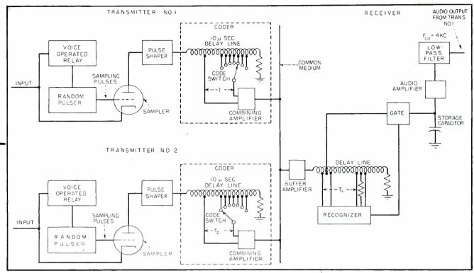
FIG. 2—System block diagram shows how receiver recognizer distinguishes between transmitter outputs by code delay introduced between pulse pairs
