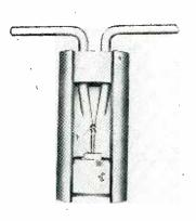
FIG. 1—Type-A cartridge structure used in earliest transistors
