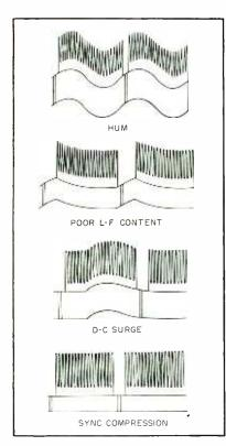
FIG. 3—Some common types of incoming video distortion
