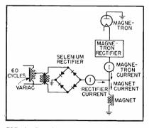
FIG. 8—Rectifier circuit supplying starting field for electromagnet
