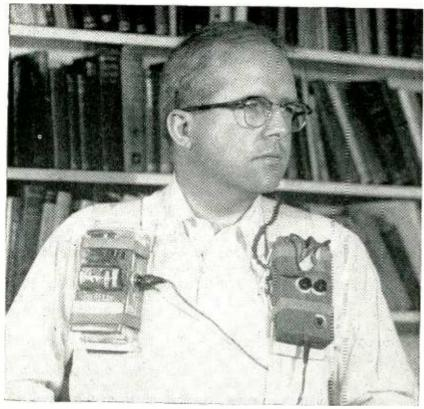
Subject wearing complete two-unit radioelectroencephalograph (REEG), with voltage amplifier on left shoulder and transparent plastic-encased transmitter on right shoulder. The three leads coming from top of amplifier go to electrodes on scalp
