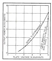
FIG. 6—Effect of plate voltage on output power
