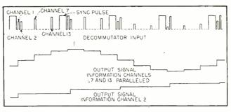
FIG. 2—Typical decommutator waveforms illustrate action of storage circuit. Output signal from information channel 2 shows original intelligence-carrying waveform reconstructed from sample pulses
