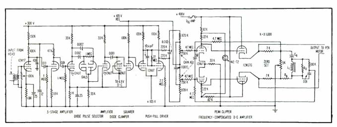
FIG. 4—Playback demodulator-amplifier restores accelerometer waveform for recording on strip chart. Tape recorder is slowed down to 1/10 record speed for playback
