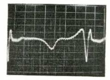
Example of heart-potential pattern obtained with equipment connected as radioelectrocardiograph (RECG), with center electrode at sterno-xiphoid junction on chest and other electrodes two inches to right and left. This location gives minimum interference from signals generated by working muscles. Timing voltage and plastic grid overlay are superimposed on pattern
