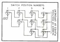
FIG. 3—Switching arrangements for the counter circuit
