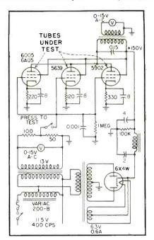
FIG. 2—Test circuit for measuring output of tube for given grid voltage
