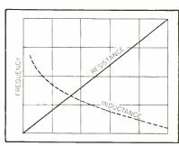
FIG. 3—Tuning characteristic of the oscillator
