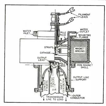
FIG. 3—Mountings and connections for the magnetron of Fig. 2
