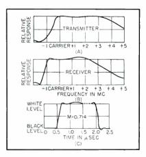
FIG. 8—Transmitter (A), receiver (B) and square-wave (C) characteristics of proposed system standards
