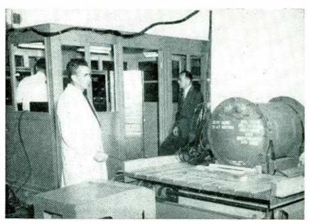
Instrument container with accelerometers attached mounted for acceleration-table test. Table connects to vibration recorder housed in shelter, left
