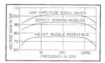
FIG. 2—Overall frequency response curves for three different gain settings of the REEG
