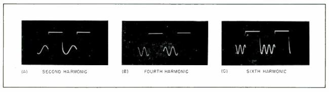
FIG. 6—Oscillograms of meter tube plate waveforms for even harmonics
