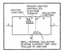
FIG. 4—Schematic diagram of a junction transistor
