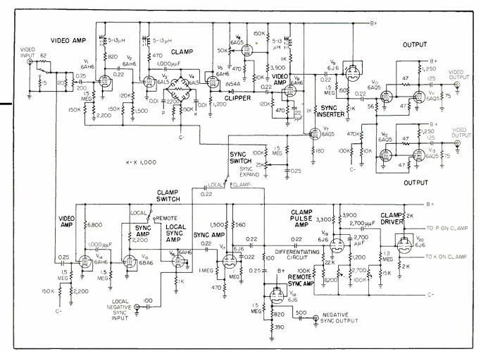
FIG. 1—Simplified schematic diagram of television video stabilizing amplifier
