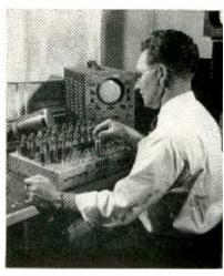
Tube under test with electronic circuits designed for use in a high-speed printer
