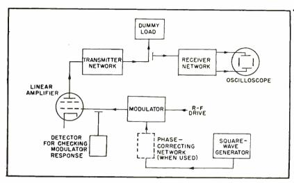
FIG. 1-Experimental system used to determine tv system characteristics
