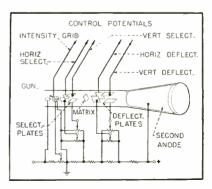
FIG. 1—Schematic-mechanical drawing of the special cathode ray tube
