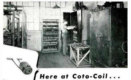
Finished coil impregnated with varnish coating the Impregnating Department applies the final protective coating to precision-made Coto Coils. Each coil is pre-heated, immersed in varnish and drained . . . sometimes 3 or 4 times. The varnish finish, baked in these modern ovens, not
