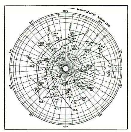
FIG. 5—Rieke diagram for a plate current of 1.0 amp and magnetic field of 1.200 gauss. Radial coordinate is the voltage reflection coefficient (scale marked in swr in db) and azimuthal coordinate is phase angle of reflection coefficient (scale marked in wavelengths displacement of standing wave minimum). Upper numbers are wavelength (add 29,000 cm), dotted lines are constant-wavelength contours, lower numbers are percent efficiency and solid lines are constant-efficiency contours
