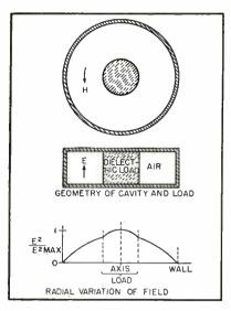
FIG. 1—Distribution of heating in a cylindrical resonant cavity
