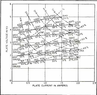
FIG. 4—Performance curves taken with transmission line matched to load
