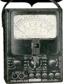
Compact, laboratory style, high sensitivity test set. "Application Engineered" for production, test, laboratory, school and service-maintenance phases of modern radio-electronics-communications.
