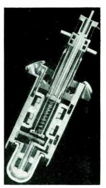
FIG. 12—Cut-away view of a 14-kv magnetron with magnetic field of 1,500 gauss
