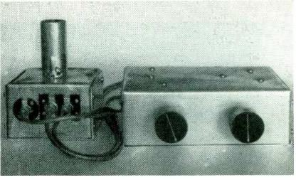
Typical oscillator construction. Tuning unit and amplifier have separate chassis
