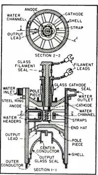
FIG. 2—Cross-sectional view of a 5-kw water-cooled magnetron
