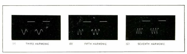
FIG. 5—Oscillograms of meter tube plate waveforms for odd harmonics
