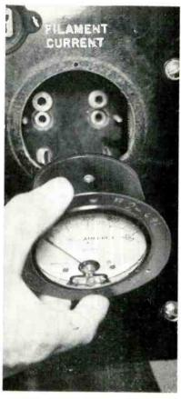
Plugging meter into test set
