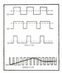
FIG. 2—Typical waveforms illustrate pulse-width modulation technique
