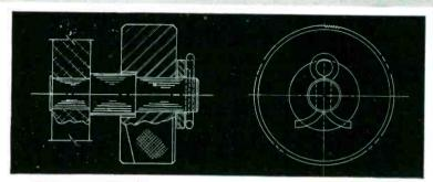
COTTER PIN WAY: Flint wheel shaft in lighter assembly requires cotter pin, washer. Difficulty in drilling perfect hole causes rejects. Assembly is slow, costly.
