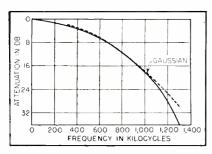
FIG. 7—Attenuation characteristics of pulse shaper
