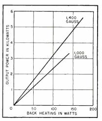
FIG. 9—Back heating of the cathode in a 5-kw magnetron with matched load
