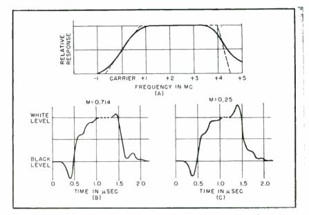
FIG. 3—Standard system ampliture characteristics (A) and output envelope waveforms for varying degrees of modulation (B) and (C)
