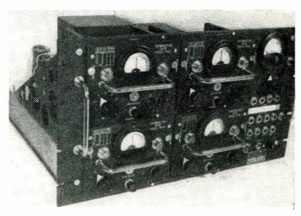
Four-channel separator incorporates four basic information gates and common power supply
