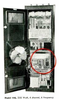
transmitter (A1, A3), manufactured by Aerocom. Frequency range from 2.5 to 24 Mcs. Stability .003% using CR-18/U crystals. Operates on any stable voltage from 200 to 250 volts, 50/60 cycles, single phase. This transmitter uses three ADLAKE Relays.
