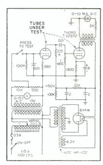
FIG. 1—Circuit arrangement for incoming-inspection test of voltage amplifier tubes for airborne electronic equipment
