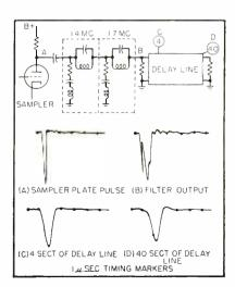
FIG. 6—Pulse shaper smooths pulses to forestall pulse interference
