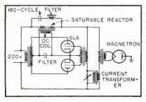
FIG. 10—Constant-temperature filament regulator circuit
