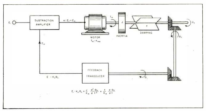
FIG. 3—Closed-loop servo system and its differential equation
