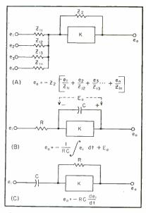
FIG. 2—Fundamental processes in analog computing are (A) summation, (B) integration and (C) differentiation
