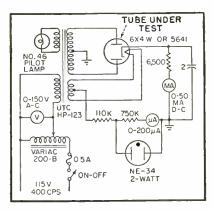
FIG. 3—Simple test circuit for checking 6X4W ruggedized and 5641 Arinc rectifier tubes
