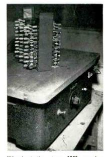
Vibration-testing type 5900 premium subminiature tubes a hundred at a time in fixture resting on table of paper jogger. Amplitude-measuring coil is at right rear corner of table
