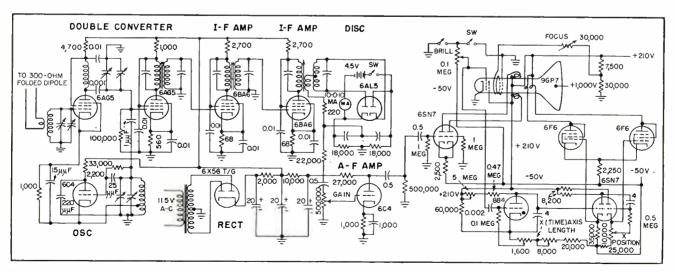
FIG. 3—Receiving and observing system of the REEG. The a-f amplifier delivers a signal output of several volts to the viewing section at the right, using a special long-persistence cathode-ray oscilloscope with a plate camera
