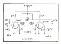
FIG. 2—Test circuit for obtaining the square-law characteristic
