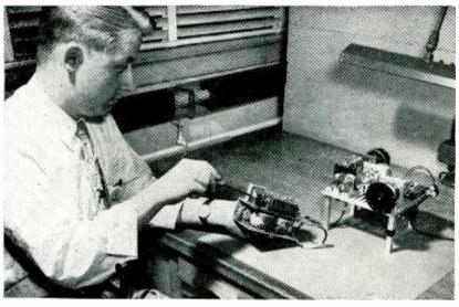
Compact size of amplifier is evidence of half-wave circuit economy. Amplifier shown drives 5-watt servo motor
