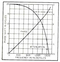
FIG. 4—Attenuation and phase characteristics of 10-microsecond delay line
