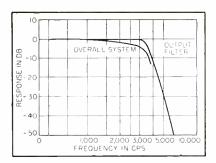
FIG. 10—Frequency response of output filter and overall system characteristic
