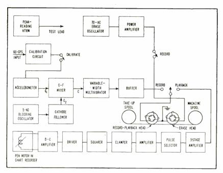
FIG. l—Block diagram shows how system frequency response is extended using tape recorder to play back data at reduced speed
