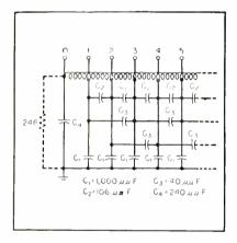
FIG. 5—Compensating capacitors help achieve phase-linearity in delay line
