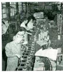
COMPONENTS OF A-C SOLENOID STARTERS are being assembled in Ward Leonard's plant in Mount Vernon, New York.
