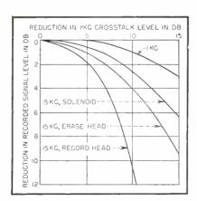
FIG. 1-Effect of selective erasure fields produced in three ways, when using 15-kc recorded signal. With 1-kc signals, all three erasing devices give the same results, represented by uppermost curve
