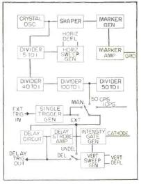
FIG. 2—Simplified block diagram of the sweep oscillograph
