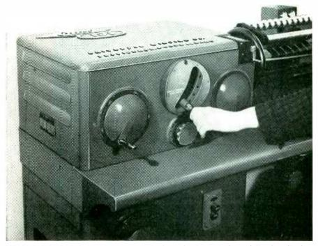
LEESONA NO. 108 COIL WINDER, award winner in the 11th Annual Product Design Competition sponsored by "Electrical Manufacturing," meets the demand for a modern manual paper feed machine for winding paper insulated coils in multiple or "stick" form. It winds coils from #20 to #44 (A.W.G.) in coil lengths from 1/4 in. to 35/8 in., in diameters, up to 5 in. round or square.
