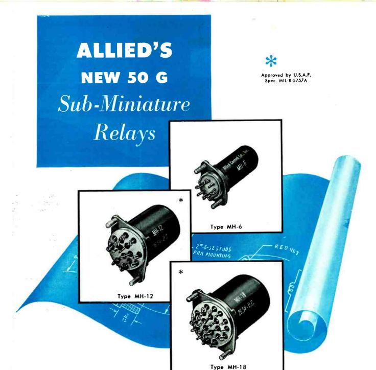
Developed specifically to meet the rigid requirements of U.S.A.F. Spec. MIL-R-5757A, the new Allied line of subminiature double throw relays includes the MH-18 (6-Pole). the MH-12 (4-pole), and MH-6 (2-pole). • Contacts are rated at 2 amps resistive or 1 amp inductive at 28 volts D.C. • The high performance of these relays has been achieved in an extremely compact, unitized construction and parallels the most recent advances in airborne equipment design.
