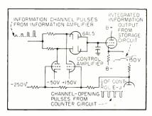
FIG. 4—Information gate is opened by sequencing pulse. Storage circuit holds information during off time
