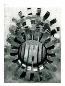
Water-cooled magnetron anode rated at 80 kw
