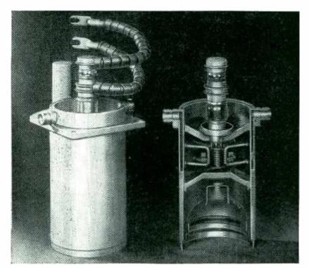
Complete and cut-away views of a water-cooled 915-mc magnetron with plate dissipation rating of 3,000 watts
