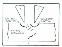
FIG. 2—Schematic diagram of a pointcontact transistor
