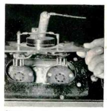
Plug-in socket panel for tube under test. Coil spring stretched between posts back of socket makes connection to shell of 6SQ7 for checking continuity to No. 1 pin
