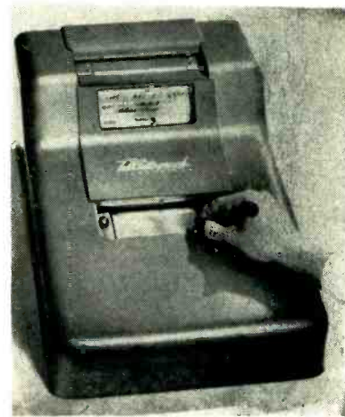
FIG. 1—Transceiver unit containing both a transmitter and receiver
