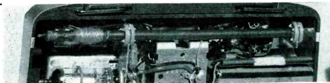
An RCA personal portable receiver showing relative size and location of antenna near top
