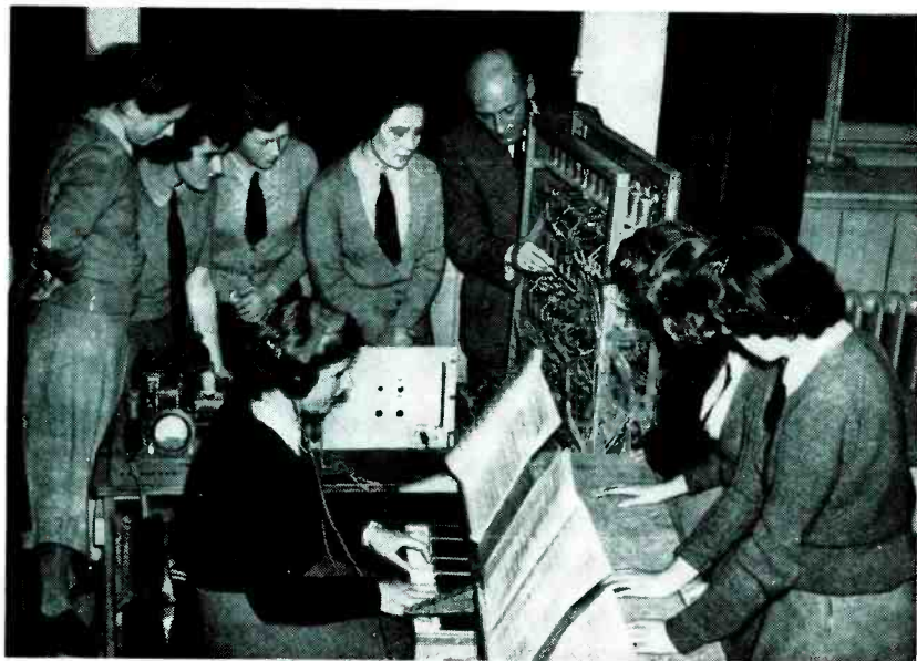
Inventor of the first silent electronic organ, N. D. N. Belham, science master at the Mid-Essex Technical School, Chelmsford, England, makes adjustments at the electric unit which operates the instrument. Up to 24 keyboards can be used, supplied from one tone unit in the console. Pupils can all play different pieces and listen to themselves on the earphones, while no sound is heard elsewhere. The teacher can listen in to any of the players, speak to them, correct their mistakes and play the correct version back to them
