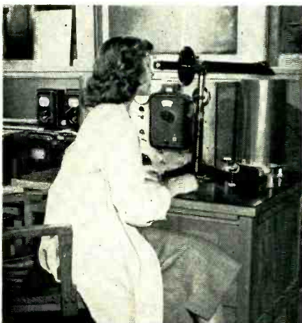
VITROHM vitreous enamel is measured by interferometer for coefficient of thermal expansion, melting and annealing points.
