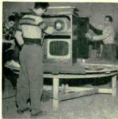
Cabinet merry-go-round used in place of conveyor line at CBS-Columbia when only a few cabinet operations are needed
