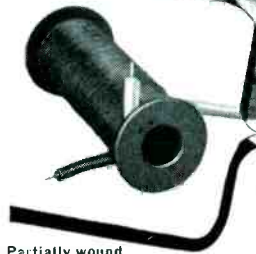
Partially wound bobbin-type coil
