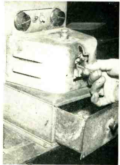
Using heat to strip rubber-covered insulation from wire. Stripped insulation drops into drawer below. Rheostats permit independent control of current through each heating jaw
