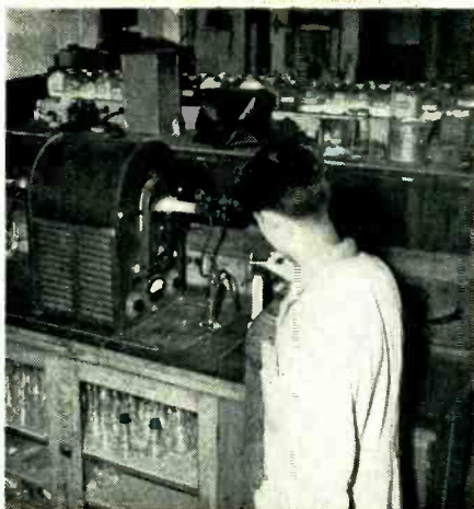
RESISTANCE WIRE sample is being processed in the combustion furnace to insure accuracy of alloy formula.
