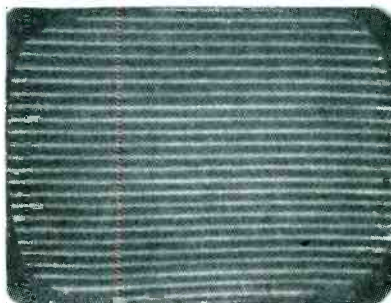
Test pattern illustrates degree of vertical linearity obtainable
