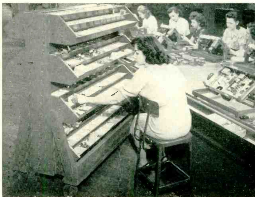
Self-service parts supply cart used in conjunction with Crosley merry-go-round production line. Cart is loaded in stockroom with quantities to match single day's production, giving close control of material. Each operator takes from the cart the individual filled trays she will need, and places them in the raingutter-type holder that runs the full length of the work table. Ball-caster chassis jacks are used on this particular line
