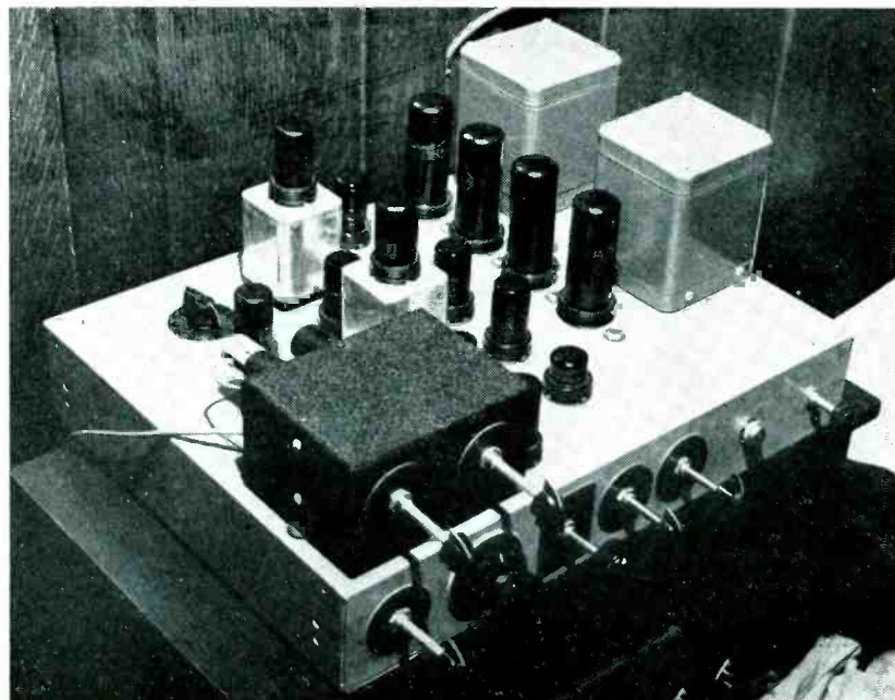
Top view of home-built Drisko power amplifier. A phonograph preamplifier and a dynamic-noise-suppressor circuit are included on the same chassis in this photograph
