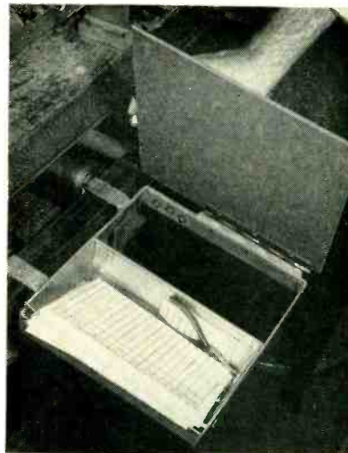
Method of supporting writing board on conveyor line and storing spare sheets
