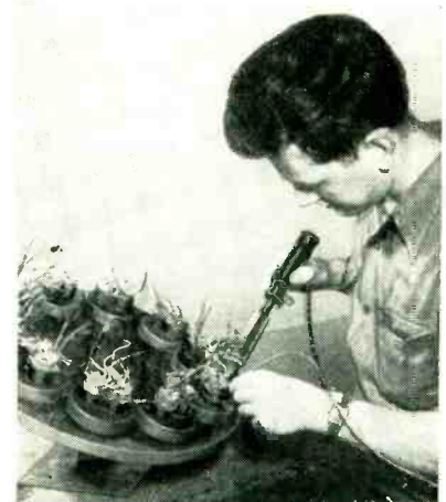
Subassembly merry-go-round at North American Philips Co. holds ten pairs of sockets. Each pair is on a pivoted wood disc that can also be turned
