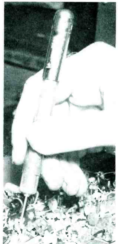
Oiler filled with red lacquer is used in place of brush to mark soldered joints that pass inspection
