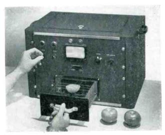
The Agtron, photoelectric bridge spectrophotometer designed for grading tomatoes by color
