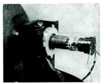
FIG. 5—Offset open ring magnet centering device
