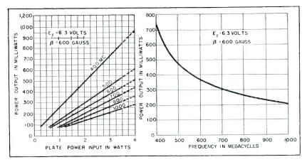
FIG. 9—Curves show power output as function of input (left) and frequency (right)
