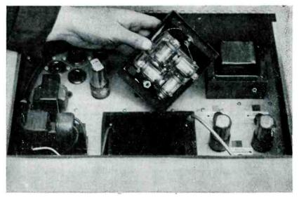
Plug-in phototube enclosure projects downward through the chassis above the grading compartment. The inner surfaces of the compartment are finished in black to prevent unwanted spurious reflections. Reference control and band-selection control are on front panel
