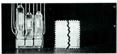
Here's the latest outgrowth of Centralab's constant research in Printed Electronic Circuit development. The remarkably small dimensions of this new amplifier unit are approximately  $1\frac{1}{2}$ " x  $1\frac{1}{6}$ " x  $1\frac{1}{3}$ ". Check coupon for Technical Bulletin 42-130.
