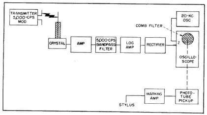
FIG. 5—Block diagram of automatic amplitude-contour-plotter system
