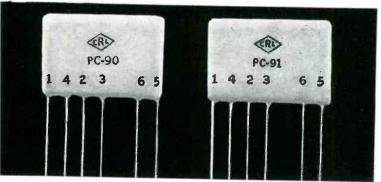
Pentode couplates are complete interstage coupling circuits consisting of 3 capacitors and 3 resistors on a small 6 lead ceramic plate. Compared with old-style audio circuits, they actually reduce soldered connections 50%—wiring errors accordingly. Technical Bulletin 42-128.
