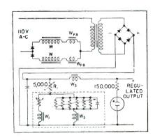
FIG. 3—Circuit diagram of magnetic amplifier voltage regulator
