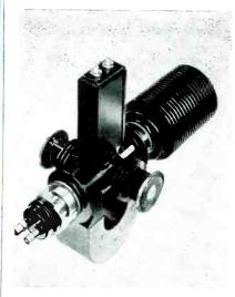
FIG. 1—SAX-22 pulse-amplifier klystron for 9,300 mc. A permanent magnet is used to focus the beam
