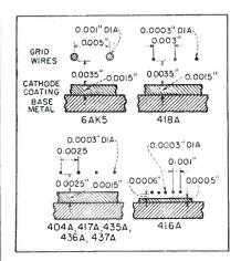
FIG. 1—Close spacing and small grid wire size provide improved transconductance to capacitance ratio
