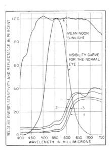
FIG. 2—Spectral reflectance curves for four grades of tomatoes. Normal visibility curve and spectral energy distribution of sunlight have been superimposed
