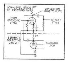
FIG. 1-Method of connecting the selective circuit to the amplifier
