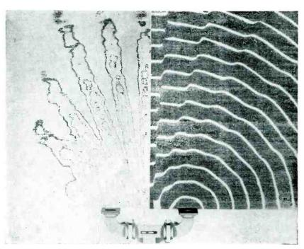
FIG. 6—Amplitude and phase plot of two point sources
