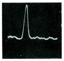
Proton resonance line using a water sample adjusted with ferric nitrate
