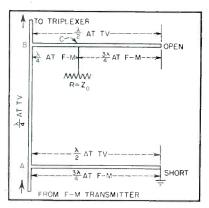
FIG. 2—First approximation of a filter interposed between the WNBC-FM transmitter and common-antenna triplexer
