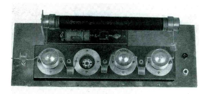
Four-tube bank with one tube removed to show pin connections. Three banks stacked vertically constitute complete amplifier
