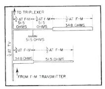
FIG. 6-Completely developed filter differs from that of Fig. 2 by its effectiveness at television frequencies
