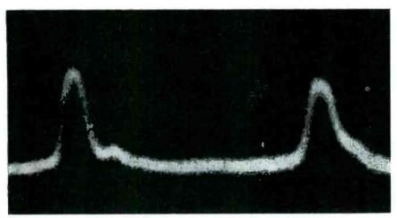
Comparison between 0.015-microsecond pulse directly viewed (left) and delayed and amplified (right), showing how little it is distorted in the amplifier
