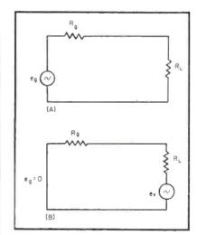
FIG. 1—Equivalent circuits showing audio amplifier damping
