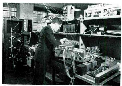
SYSTEMS CHECK Rare today is the single-chassis airborne electronic unit. Many units must be hooked together each time an advanced development is checked, as is being done in this electronics lab at The Glenn L. Martin Company's plant in Baltimore. Interconnection of systems, layout and shielding of wiring, layout of equipment so units cannot bump each other and provision for clearance needed to remove units are just a few new duties of the electronic engineer
