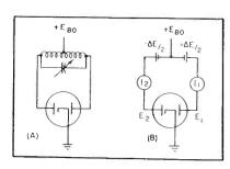
FIG. 3—Circuits for low-frequency oscillator and for measuring negative conductance of miniature magnetron
