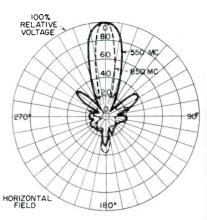
RHOMBICS more than several wavelengths on a leg proved highly successful in uhf field tests when adjusted and terminated for unidirectional operation. Gain is adequately high for fringe areas. Major forward lobe is quite narrow and decreases with frequency as shown. Major vertical lobe, not shown, is about three times as broad as corresponding hori-
