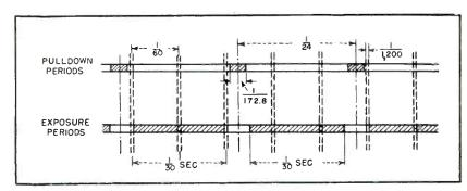
FIG. 1—Time division for recording 60-field-per-second transmissions on film
