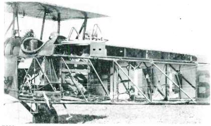
EARLY BLACK BOXES Experimental installation of Radio Set SCR-134 in De Haviland two-seater fighter about 1926, using coil springs instead of shock cord to support the two boxes in fuselage space behind machine-gunner. Vibration was so great that they went back to shock cord. Weighted trailing-wire antenna was lowered through slanting pipe under gunner's feet—Air Force Photo
