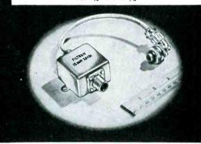
15 amp. -28 VDC filter, size  $2'' \times 2'' \times 11/4''$ , with pressurized AN connectors - high attenuation from 150 KC to 400 MC.
