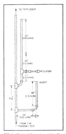
FIG. 7-Physical dimensions of the filter show how it can be constructed from standard fittings
