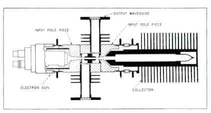
Cross-sectional view of 9,300-mc klystron
