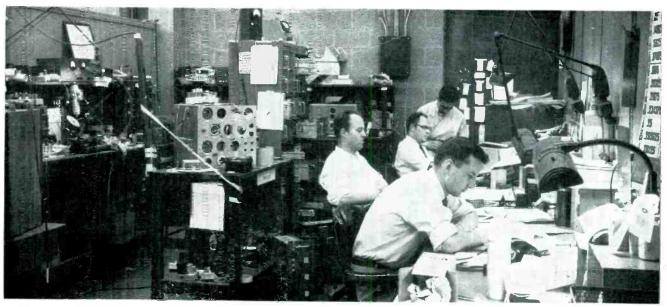
COMPUTER TEAM Electronic engineers make extensive use of analog computers to replace try-and-see or crystal-ball techniques for finding out whether a proposed new idea will work. Here evaluation group for experimental analog computer at Cornell Aeronautical Laboratory converts computer readings into yes-or-no decisions for new airborne electronic control designs
