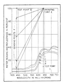
FIG. 5—Graphical representation of tomate grading procedure. Curves 1 to 4 have the same identification as in Fig. 2 and are described in text
