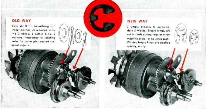
Using 2 Waldes Truarc "E" Retaining Rings in their Automatic Cabinet Ironer, saved The Horton Manufacturing Co., Fort Wayne, Ind., \$.0219 per unit. Truarc Rings saved 50% in assembly time ... cut down on rejects ... increased efficiency of the unit...eliminated risk of damage to hands and clothing of workers in assembly.
