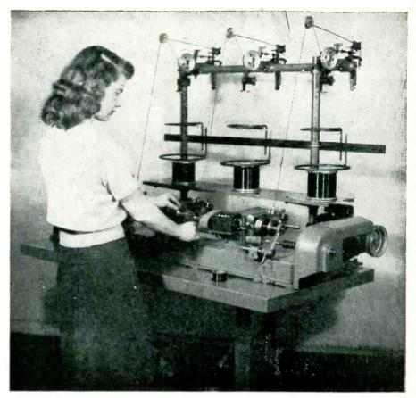
WHEN OPERATOR FINISHES manual procedure on one head, another coil will have just been completed. By synchronizing winding and handling time on the No. 102 Universal Hi-Speed Coil Winder, you get maximum production per operator. Coils up to 15,000 turns can as a rule be handled efficiently on a 3-head machine at a maximum of 5000 rpm.
