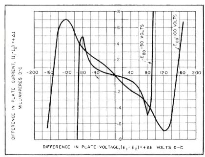
FIG. 5-Negative-conductance characteristic for 600-gauss field
