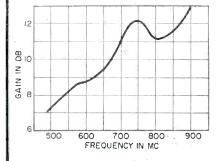
CORNER REFLECTOR having 90-degree included angle, using fan-dipole element also folded at 90 degrees, gives ultimate in gain for its compact size. It should be one of best fringe-area uhf antennas, being truly unidirectional in both horizontal and vertical planes. Negligibly small unwanted lobes minimize reflection and multipath troubles. On all gain curves here, 0 db reference is gain of thin half-wave dipole adjusted to resonance at each frequency and matched into 300 ohms
