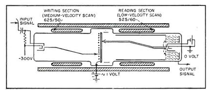
FIG. 5-Standards converter with image-orthicon-type reading section
