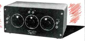
This equipment is particularly applicable to extremely accurate measurements from D.C. to 200 kc. and can be used up to the lower radio frequencies. The Decade type switches make the box convenient to use. In addition, there are switch stops which prevent return from full to zero attenuation when making adjustments. A total of 110 Db. is available in 1.0 Db. steps, or 111 Db. is available in 0.1 Db. steps. Both of these types may be obtained in either a balanced H or an unbalanced T network.
