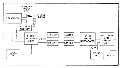
FIG. 3-Block diagram of the plotter system
