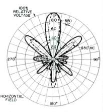
STACKED V antenna uses same rods as standard dipole cut for channe; 2 and thus contains about same amount of metal as simple whi dipole and reflector. Efficiency is good considering simplicity of construction and ease of mounting on existing masts. Gain is high enough for medium and weak signal areas and increases desirably with frequency to overcome propaga-
