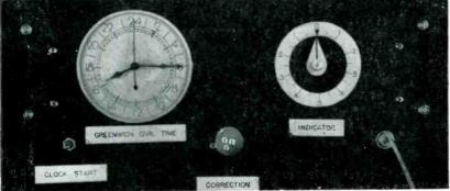
Top chassis shows commercial frequency standard built in. Portion of front panel indicates master clock and stroboscopic monitor also shown at top
