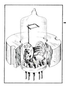
FIG. 1—Cut-away drawing of miniature magnetron shows interdigital construction. A permanent magnet furnishes the required field of 500 to 600 gauss
