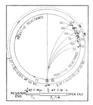
FIG. 5-Open-circuited stub can be formed from two different diameters of inner conductor to represent infinite impedance
