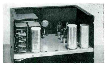
Rear view of the complete oscillator with back and top removed. Resistor R in center.
