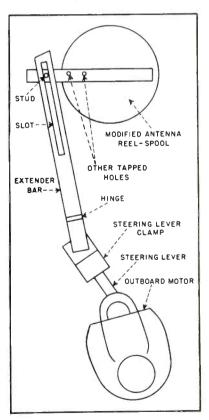
FIG. 4—Mechanical connection to outboard motor as used in first model
