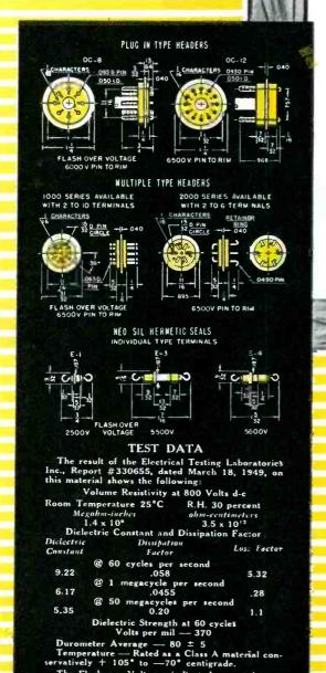
The Flashover Voltages indicated were tak temperature of 68° Fahrenheit, and 47% e Humidity.
