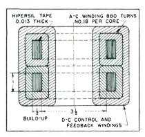
FIG. 1—Construction of magnetic amplifier used in voltage regulator
