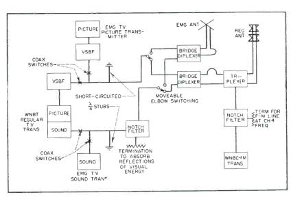
Complete transmitter and antenna system used at WNBT and WNBC-FM
