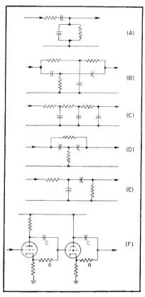
FIG. 1—Frequency-selective networks employed in resistance-capacitance oscillators
