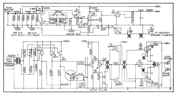
FIG. 2—Features of the timing system include clipping and filtering circuits (upper part of drawing) so that discrete time ticks from WWV allow resetting with great accuracy; and phase splitter for selsyn reset
