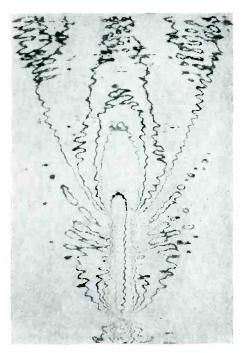
Amplitude plot of a polyrod antenna
