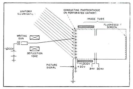
FIG. 11—Principle of storage kinescope (Schroter)
