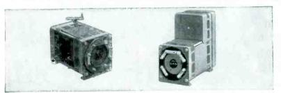
For precise and dependable stepless voltage regulation or variation it's G-E inductrols. These singlephase units are available in ratings from 3 to 240 kva for circuits 600 volts and below. Motor-operated units, used with automatic control, maintain voltage within narrow limits regardless of line-voltage variation. Hand-operated models provide smooth and precise voltage adjustment for instrument calibration, rectifier control, and similar uses. Check Bulletin GEC-795.
