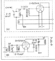
FIG. 1-Circuit of f-m oscillator and amplifier for telemetering respiratory information
