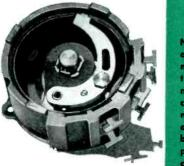
New Clarostat Series 42 potentiometer. Available in single and multiple assembles up to 20 sections. Precision windings to plus/minus 0.5% and better. Positive contact rotor, smooth rotation, minimum wear. Perfect tracking of all units in assembly. No backlash or play. Rotor of each potentiometer maynted an centerless-ground shaft passing through all sections.
