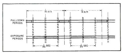
FIG. 2—Time division for recording 50-field-per-second transmissions on film
