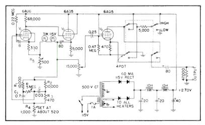
FIG. 3—Complete circuit of the single-resistor (R) oscillator. In low position, maximum output is 5 v at 250 ohms; in high position, 30 v is obtained at an impedance of 5,000 ohms
