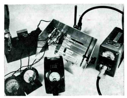
Turret tuner uses six tuner strips of the type shown in Fig. 6 and can be adjusted for any six frequencies between 400 and 1,000 mc
