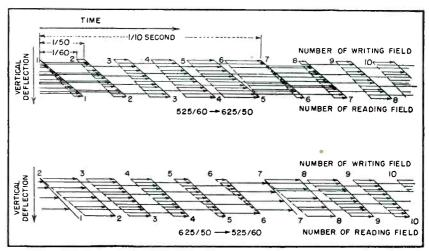
FIG. 7—Relationship between writing and reading process when single-line-width reading spot is employed
