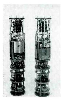
Two views of the repeater switch. The switch is sealed in a steel cylinder
