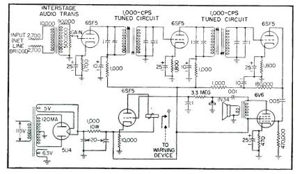
FIG. 1—Schematic of the 1,000-cycle warning device for bridging network program lines
