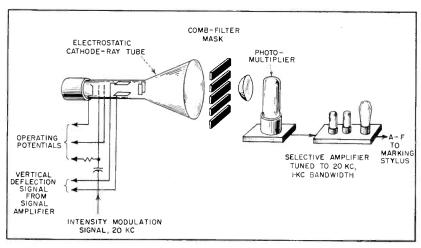
FIG. 4—Operation of comb-type amplitude filter
