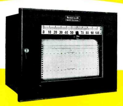
Self-contained Electronik narrow span potentiometer, incorporating new (40X) amplifier, is ideal for measuring low level potentials.
