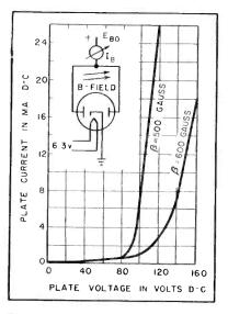
FIG. 2—Typical static plate characteristics of miniature magnetron
