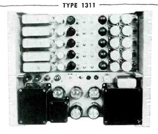
TYPE 1311 Video Distribution Amplifier is specifically designed to distribute video or synchronizing signals to several outlets. Thus, five separate equipments can be fed from a single synchronizing signal generator and monoscope combination.
