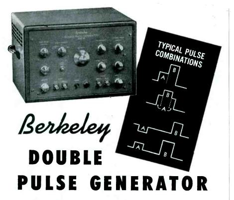
**DESCRIPTION:** The Berkeley Model 903 Double Pulse Generator is a general-purpose laboratory instrument that produces either single or paired pulses. Pulses are individually variable in width, amplitude, and spacing. Pulse polarity is individually selectable. Separate connectors provide impedance levels of 50 or 1,000 ohms for each pulse output.
