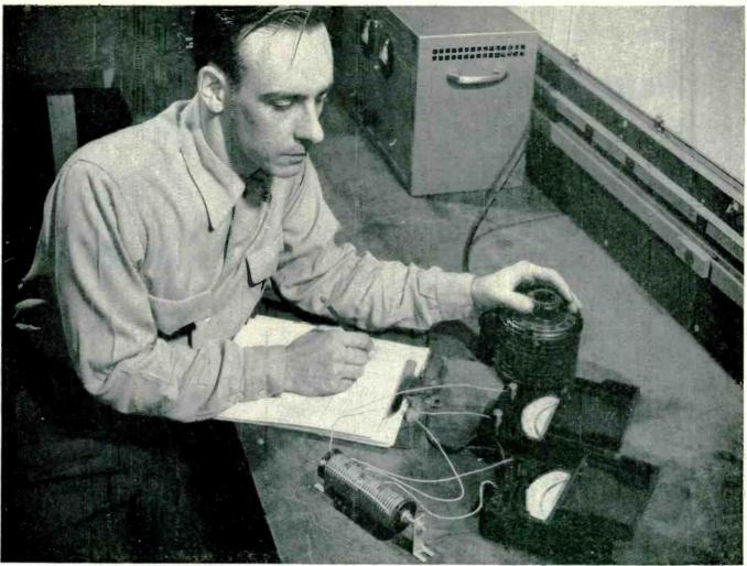
TEST FOR FORWARD VOLTAGE DROP (ABOVE) REQUIRES ONLY VARIABLE A-C SUPPLY, A-C VOLTMETER AND D-C AMMETER
