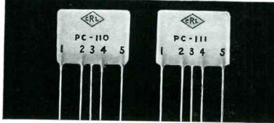
FILPLATES (2 resistors and 2 capacitors) for bypass and filter ap plication in TV, FM and AM, where filter networks of comparable component values and layout are needed. Smaller than special delivery stamp. Save vital low wattage resistor stocks. Technical Bulletin 42-131.
