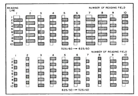
FIG. 8—Picture signal (shaded area) and charge left after reading (clear area) for flat object field when double-width writing beam and single-line width reading beam is employed
