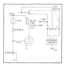
FIG. 3—Simplified diagram of experimental model
