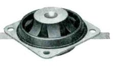
4. MIL-I-5432 (AN-I-16a) can be met with the Type 17 ISO-MODE Mount. This unit available for loads from 0.5 to 100 pounds, and controls all modes of vibration with equal efficiency because of equal spring rate in all directions.
