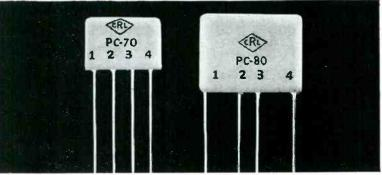
Centralab Triode Couplates replace 5 components normally used in audio circuits. Triode Couplates are complete assemblies of 3 capacitors and 2 resistors bonded to a dielectric ceramic plate. Available in a variety of resistor and capacitor values. Technical Bulletin 42-127.
