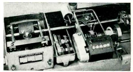
READILY-ADJUSTABLE TRAVERSE MECHANISM permits winding any length of coil from 1/16 in. to 2 13/16 in. without changing cams. A single setting applies to all the winding heads.
