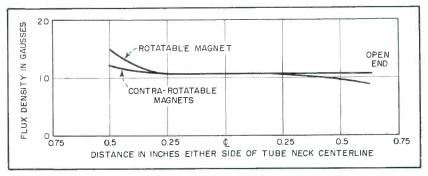
FIG. 1—Curves show linearity of flux distribution across neck of tube
