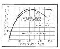
FIG. 2—Output power as a function of r-f drive power
