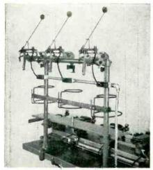
WIRE BREAKAGE DETECTOR is optional equipment for stopping arbor promptly when wire breaks or runs out. This relieves operator of having to watch wire spool continually and prevents counting of turns when wire is not being wound.
