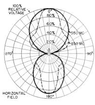
FAN DIPOLE, simplest of all uhf receiving antennas, requires only two triangles of metal supported by an insulating bar. Dipoles are set in metal frame for stacking, which with proper phasing gives greatly increased gain. Bandwidth is excellent. Stacking narrows vertical directivity but does not affect horizontal directivity. Fourstack unit uses two two-stack units connected by twin-lead
