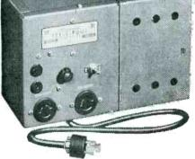
Illustrated above is the "Tel-E-Foul" control box. When the bowler oversteps the foul line the electronic brain conveys an impulse causing a light to flash above the alley. A 75 MA SELETRON miniature is built into the control box on each bowling lane.
