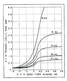
FIG. 2—Transfer characteristic of magnetic amplifier
