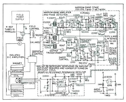
FIG. 4—Circuit of the magnetic regulator applied to control of 35-ton magnet
