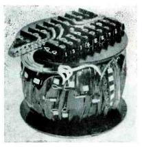
Magnetic amplifier used in voltage reg-
