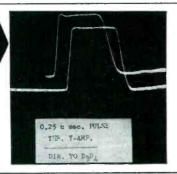
The pulses in the oscillogram at left are identical pulses of 0.25 microsecond width. The first pulse was applied through the Y-axis amplifier of the Type 294-A, and the second, directly to the vertical deflection plates. A comparison of their waveforms illustrates the excellent transient response of the Y-axis of the Type 294-A.
