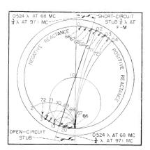
FIG. 3—General method of plotting values of ¾ wavelength f-m lines to find characteristic at television frequencies
