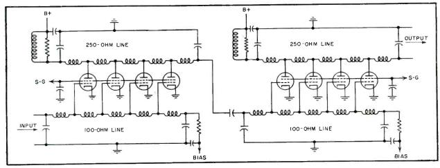
FIG. 1—Circuit diagram showing interconnection of two banks of the distributed-line amplifier. The tubes are all type 4X150A, matched by groups for high and low emission
