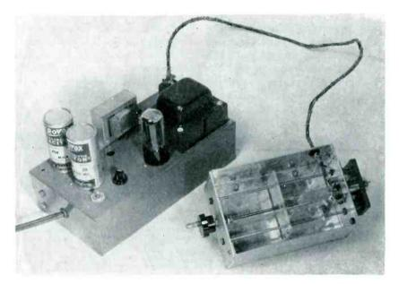
Magnetron tuner and power supply for continuous tuning from 515 to 930  $\,\mathrm{mc}$
