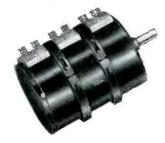
Type RV1%\* and RV2\* High Precision . semi-standardized types Potentiometers . of precision machined aluminum base potentiometers with exceptionally high electrical accuracy and mechanical precision. For both linear and non-linear functions. Designed for precision instrument, computer and military applications. Accurate phasing of individual units possible with clamp-ring method of ganging.
