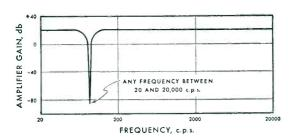
Figure 1. Rejection Characteristics, -hp- 330 series
