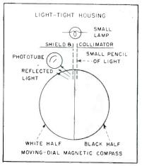
FIG. 2—More versatile direction-sensing device
