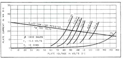
FIG. 4—Stable dynamic plate characteristics for 400 to 900-mc turret tuner
