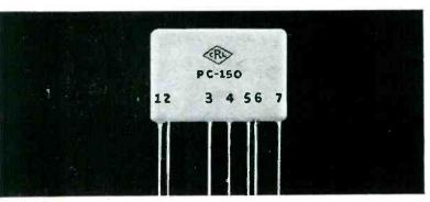
Audet Printed Electronic Circuits furnish all values of all components generally found in the output stage of AC-DC radio receivers. They provide 4 capacitors and 3 resistors on a small plate with only 7 leads. Technical Bulletin 42-129.
