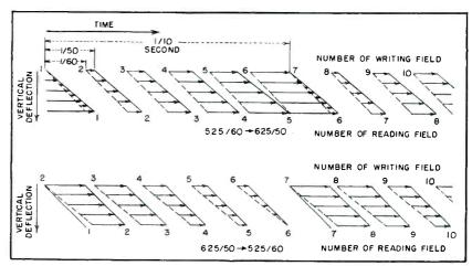
FIG. 6—Relationship between writing and reading process when double-width reading spot is employed
