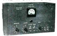
LETTINE MODEL 240 TRANSMITTER WITH MOBILE CONNECTIONS AND A.C. POWER SUPPLY
