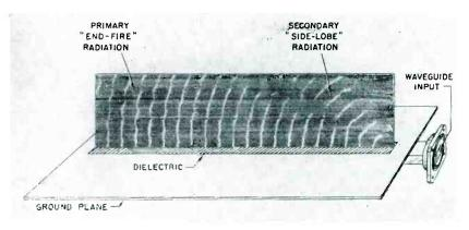
FIG. 7-Phase-front contours of a metal-clad dielectric antenna
