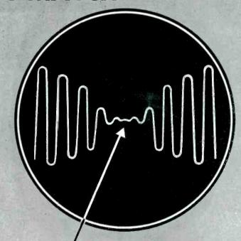
Envelope is the curve of reflection coefficient vs. frequency over 30 mc. band
