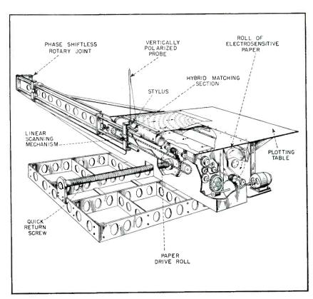
FIG. 2-Cutaway illustration of automatic phase-front plotter
