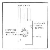
FIG. 1—Direction-sensing mechanism of experimental model
