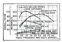
FIG. 3—Signal and noise characteristics of amplitude bridge
