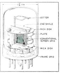
FIG. 3—Structure is rigidly supported from stem which eliminates distortion when bulb is placed over the mount
