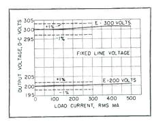
FIG. 4—Constant-line-voltage curves show regulation of output for varying output current values
