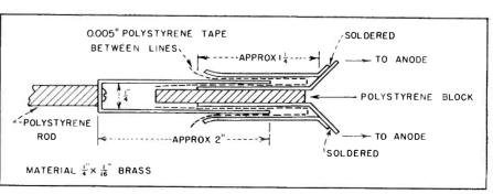
FIG. 8—Tuning element for continuous coverage of frequency range from 515 to 930 mc
