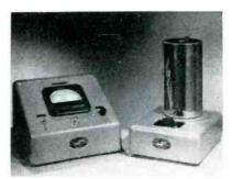
Commercial gammometer that operates on atomic battery principle
