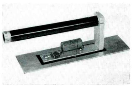
Reverse-termination resistor assembly uses capacitor mounting as one plate of bypass capacitor to chassis
