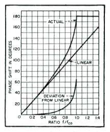
FIG. 2—Phase shift per section of the constant-k filter
