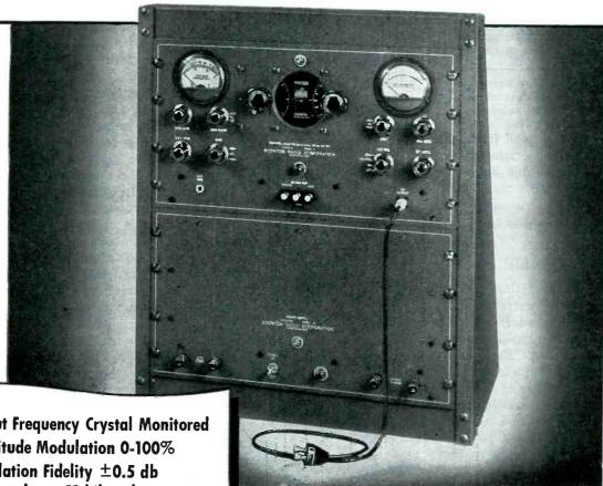
**Output Frequency Crystal Monitored Amplitude Modulation 0-100%** Modulation Fidelity ±0.5 db 30 cycles to 11 kilocycles **Negligible Spurious FM**
