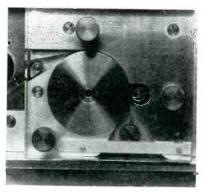
One of two continuously running rollers against which tape is pressed when movement in that direction is desired. This technique provides very fast acceleration
