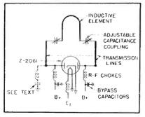
FIG. 7—Equivalent electrical circuit
