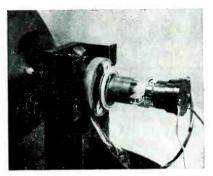
FIG. 4—Contrarotatable unit consists of two open ring magnets
