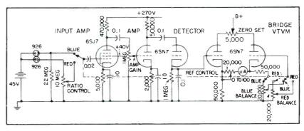
FIG. 4—Circuit of the bridge spectrophotometer includes two stages of amplification and a detector ahead of the measuring bridge
