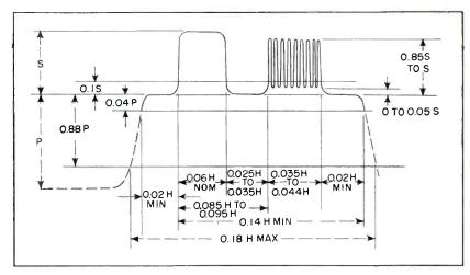
FIG. 2—Color synchronizing signal. This waveform is that which exists at the studio before transmission over limited bandwidth circuits. The burst follows each horizontal pulse. It is omitted following the equalizing pulse and during the broad vertical pulse. Vertical blanking is 0.07 to 0.08 of the vertical scanning period
