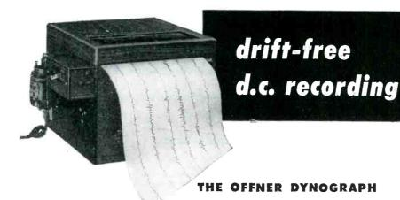
Here's a direct writing, high speed oscillograph with microvolt d-c sensitivity—made completely drift-free through an exclusive chopper type amplifier. Now you can obtain a precise record of transient variables—some formerly recorded only by photographic means—at about 100 times the speed of other recorders with comparable sensitivity.
