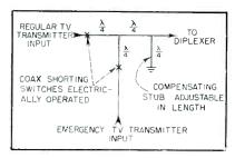
FIG. 1—Elementary arrangement of coaxial shorting switches and compensating stub for emergency transmitter changeover
