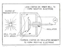
FIG. 1—Drawing shows components of battery with radioactive energy source
