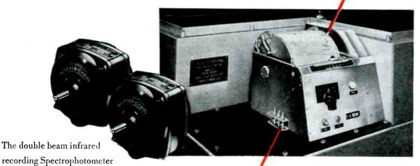
developed and manufactured by Baird Associates of Cambridge, Mass., is an ingenious instrument which has proven itself invaluable in quickly and surely identifying and defining complex chemical compositions.
