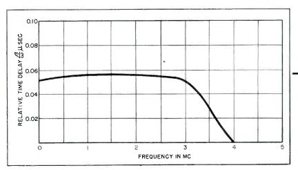
FIG. 1—Delay characteristic of network for compensation of phase distortion associated with cut-off in receiver. Relative time delay versus frequency characteristic of radiated envelope is to be held within + 30 percent and - 0 percent. Ordinate scale may be multiplied by a factor of 1.0 to 1.5
