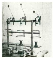
WINDING STARTS INSTANTLY WITHOUT DANGER OF WIRE BREAKAGE with the overend tension. The first turn can be started tightly against the spool or bobbin head, improving "lay".
