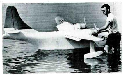
RADIO-CONTROLLED MODEL Free-flight radio-controlled models such as this are used extensively at Consolidated Vultee Aircraft Corporation's San Diego labs to facilitate solution of many Convair hydrodynamic design problems. For many electronic engineers, assignment to the radio control group is play combined with work
