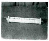
FIG. 2—Laboratory mockup shows enlarged model of grid-cathode structure proposed for use in transmission-line tubes. Grid will be wound helically around ceramic form shown
