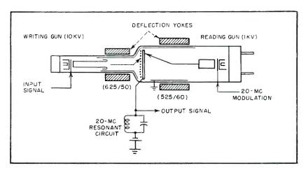
FIG. 4—The Graphechon as standards converter. The writing beam produces bombardment conductivity in the screen-supported insulating target
