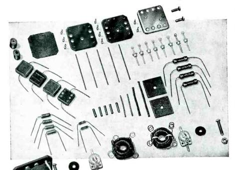
All of these 66 parts are from a single B&W Toroidal-coil type discriminator only 13/4" square by 31/2" long exclusive of terminals!
