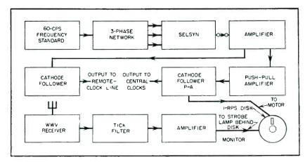
FIG. 1—Elements of the standard time-clock system show dual outputs for local clocks and remote line, stroboscopic monitor to check with WWV and selsyn reset control
