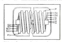
FIG. 1—Drawing showing configuration of five-element transmission line tube for broad-band amplifier applications
