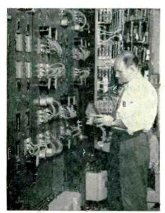
TESTS FOR LIFE of high-voltage, G-E selenium rectifiers made on convection-cooled and forced ventilation racks (above) indicate that forward resistance increases less than 6% after 10,000 hours operation.
