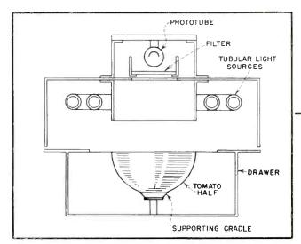
FIG. 1—Cross-section of the light source and phototube assembly for the instrument
