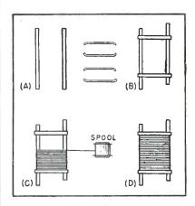
FIG. 2—We'ded grid frame structure permits use of finer wire with closer spacing
