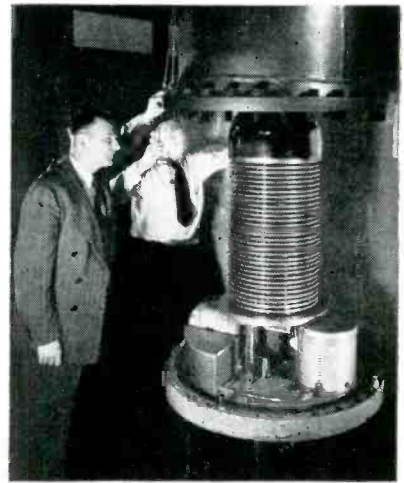
Lowering hood over 3,000,000-volt electrostatic generator used with MIT sterilizing equipment
