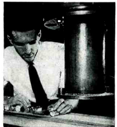
Packages to be sterilized pass beneath high-energy x-ray source
