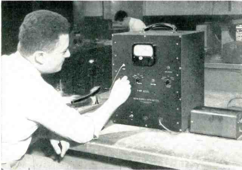
Equipment being used to test a standard production turntable
