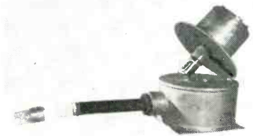
Light-piping device for remote detection of radioactivity using an anthracene crystal coupled to a 1P21 multiplier phototube by a lucite rod
