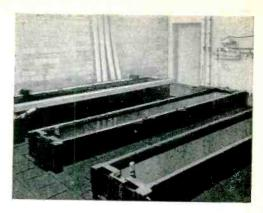
Acid House Equipment where material is eleaned and rinsed before bright annealing.
