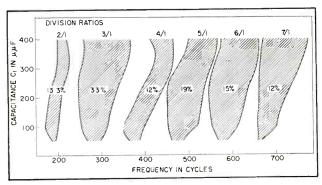
FIG. 2—Shaded areas indicate the locking range as a function of input coupling and frequency. Supply voltage is 300 v, frequency 100 cycles and resistance R is 200.000 ohms
