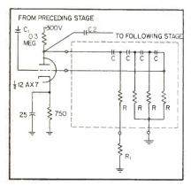
FIG. 1—Basic divider circuit illustrates importance of couplings
