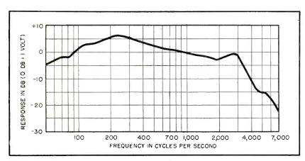
FIG. 8—Response-frequency characteristic of Shure P81 pickup cartridge terminated with 1 megohm, with all-purpose 2-mil radius needle on Auditone record. High-frequency response is attenuated by means of an internal mechanical filter
