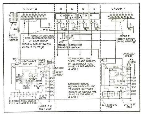
FIG. I—Test set for making life test runs of up to six groups of electrolytic capacitors, each at different values of a-c ripple current and d-c polarizing voltage that are set up on a jack panel. Temperature oven is used for electrolytic capacitors under test. Paper capacitor banks at top provide various ripple currents needed
