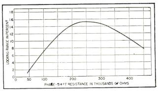
FIG. 3—Locking range in percent as a function of phase-shift resistance in thousands of ohms. The oscillator frequency used is 100 cycles and division ratio is six-to-one
