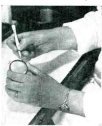
FIG. 9—Complete mesh-target system ready for insertion in the tube structure
