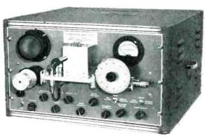
X BAND SPECTRUM ANALYZER 8500-9600 Mc. calibrated linear below cut-off attenuator, calibrated frequency meter, tuned mixer, 4 i.f. stages, 3 video stages overall gain 125 db., regulated power supply.
