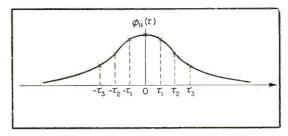
FIG. 2—Autocorrelation function of random time function that can represent a voltage or current
