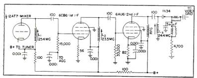
FIG. 3—Circuit of conventional single-tuned staggered stages
