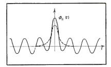
FIG. 13—Autocorrelation function of additive mixture of random noise and sine wave
