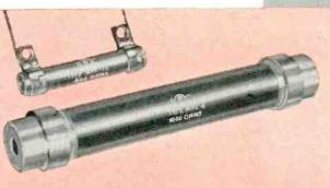
IN CRITICAL HIGH-FREQUENCY CIRCUITS, Type MP High Frequency Resistors offer dependable performance and unusual stability. Special resistance film on a steatite ceramic form provides a stable resistor with low inherent inductance and capacity—entirely suitable for broad band RF amplifiers, RF probes, dummy loads for transmitters, television sideband filters, radar pulse equipment, and other circuits involving steep wave fronts. Send coupon for Bulletin F-1.
