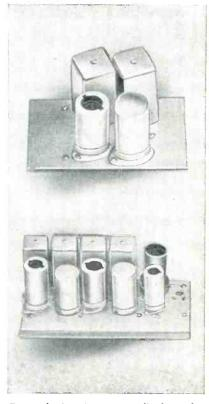
Two of the frequency dividers described. The upper one is based on 1.800 cycles and the the lower upon 90.72 kc
