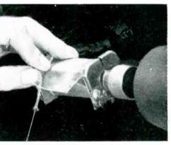
Inserting a sample preparatory to a voltage breakdown test on Kodapak Sheet.
