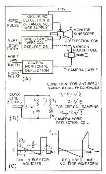
FIG. 8—Block diagram of scanning circuits. (B) and (C) explain operation
