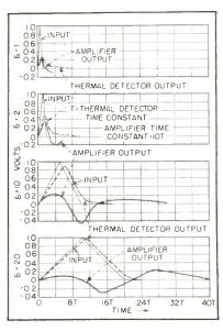
FIG. 3—Curves of pulses in relative time domain for detector and amplifier
