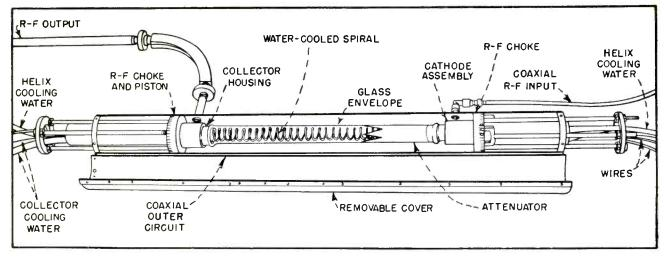
In the 1.000-wait tube, both the spiral and collector are cooled by a continuous flow of water
