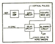
FIG. 4—Stages of the decoder unit at the receiver
