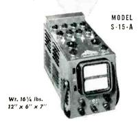
A new concept in multiple trace oscilloscopy made possible by Waterman developed RAYONIC rectangular cathode ray tube, providing for the first time, optional screen characteristics in each channel. S-15-A is a portable twin tube, high sensitivity oscilloscope, with two independent vertical as well as horizontal channels. A "must" for investigation of electronic circuits in industry, school, or laboratory.
