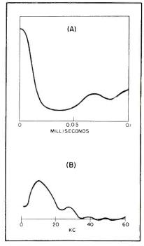
FIG. 12—Correlation function (A) for noise from a type 884 gas tube, as obtained with electronic correlator, and corresponding power spectrum obtained by making cosine transformation of function with an electronic differential analyzer
