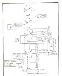
FIG. 1—Functional diagram of the automatic ionization gage circuit
