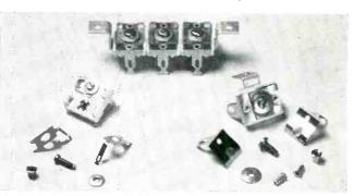
Padder condenser is shown on left and trimmer condenser and parts on right. Ganging, as shown at top right, may include any number of individual condensers. Courtesy Electro Motive Manufacturing Co., Willimantic, Conn.
