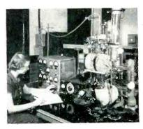
The three-stage nonmagnetic mass spectrometer in experimental operation at the National Bureau of Standards
