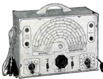
$\bigstar$  TUBES USED: 12AU7—One section is used as oscillator and the second is modulated cathode follower. T-2 is used as modulator. 6C4 is used as rectifier.
