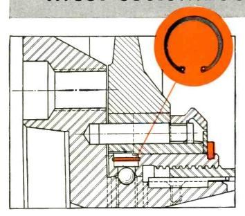
INTERNAL RING: Used instead of a shoulder screw, Truarc internal ring #5000-37 locks disc over ball loading hole. Saves 1/8 inch in overall diameter. Eliminates tapping. Withstands machine vibration and vibration from impact device within chuck. Used with Truarc pliers, it facilitates assembly and disassembly.
