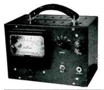
THIS instrument is designed to replace high-sensitivity galvanometers in many applications. Due to its ruggedness, freedom from burnout, and relative insensitivity to shock, it is an ideal instrument for use in balancing resistance bridges, measuring crystal rectifier output, photo-cell, strain-gage, thermocouple, and leadsulphide cell currents, etc. The instrument may also be used as a DC pre-amplifier for recorders. When used in this manner, current amplification of 1,000 is available.
