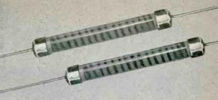
IN RIGH VOLTAGE APPLICATIONS where high resistance and power are required, Type MVX high chaic, high voltage resistors afford exceptional stability. Construction is similar to that of Type MV, but distinctive terminal permits mounting through a hole in mounting block of insulating material without terminal interference.
