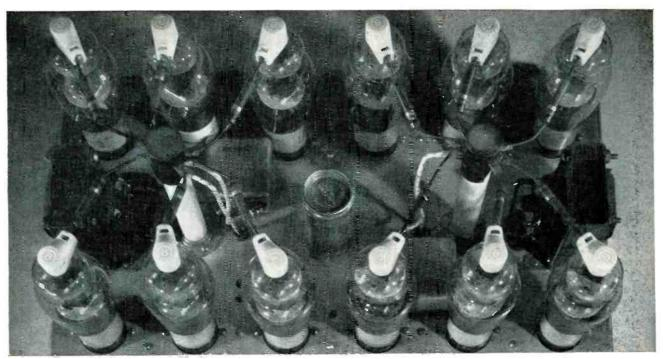
Amplifier used to provide controlled field current for dynamometer, employing twelve 807's in parallel
