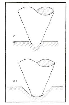
FIG. 9—(A) Profile of Unipoint needle in α fine groove. (B) Profile of needle in α 78-rpm groove
