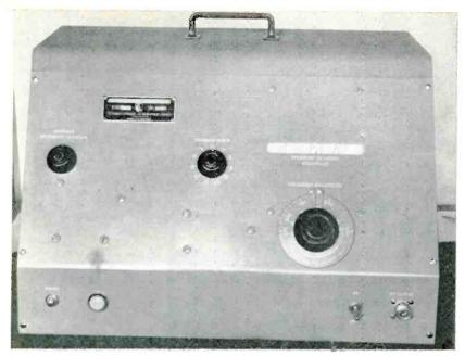
Magnitude of the frequency sweep is shown automatically through a panel slot as the oscillator frequency is varied
