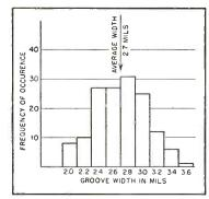
FIG. 3 — Distribution of groove widths of 147 fine-groove records
