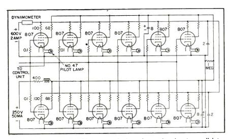
FIG. 4—Dynamometer amplifier, using 12 identical pentode tubes in parallel to provide an output current that follows the control signal despite high inductance of dynamometer field coils
