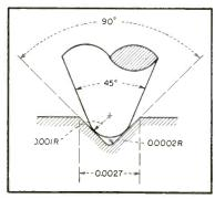
FIG. 2—Profile of typical fine-groove and standard 1-mil radius needle
