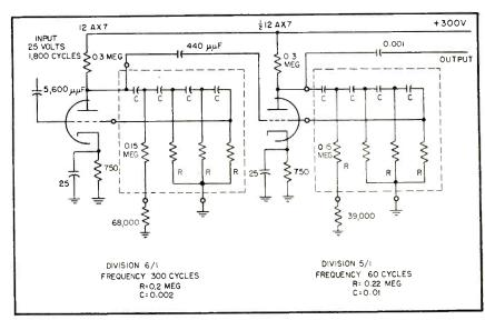
FIG. 4—Synchronous motor-control giving frequency division of 30
