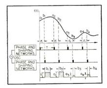
FIG. 9—Method of sampling a random function at regular intervals with an electronic correlator
