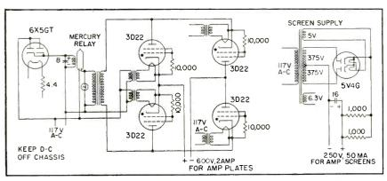
FIG. 5—Power supply circuits for amplifier and control unit. Filament heating time of 6X5GT rectifier provides time delay for application of plate voltage to gas rectifier tubes in full-wave bridge arrangement
