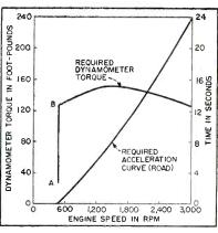
FIG. 1—Acceleration curve of 1941 Chevrolet going from 10 mph to 70 mph in high gear at full throttle on a level highway, and torque curve that electronic control system must produce to simulate this acceleration in laboratory
