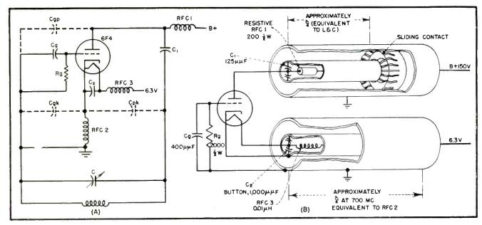
FIG. 1—Basic oscillator circuit and coaxial-line equivalent
