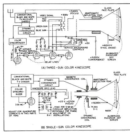
Circuit arrangements for the two types of RCA color picture tubes
