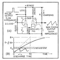
FIG. 5—Basic oscillator-counter operates at twice horizonal scanning frequency
