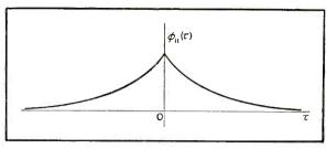
FIG. 4—Autocorrelation graph for random-width pulses of Fig. 3
