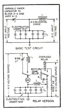
FIG. 2—Basic circuit used for life-testing electrolytics
