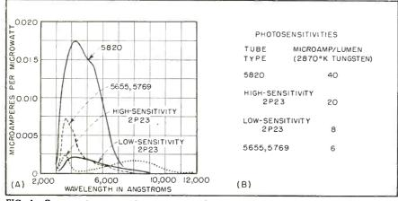
FIG. 1—Comparative spectral responses and overall sensitivities of the four types of image orthicons
