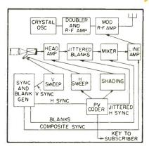
FIG. 1—Block diagram of typical Phonevision transmitter
