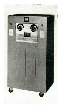
The No. 2500 has a power supply of 220 volts, 60 cycles, single phase, output of 3 kw, output frequency of 27.12 megacycles and power consumption of 5.5 kw. Size of the compact unit is 50" x 26" x 18". Weighs approximately 400 lbs. Sealing cycle is automatically controlled.
