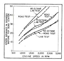
6-Correlation of knock-rating curves obtained on road and with electronic control system in laboratory
