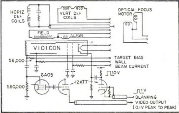
FIG. 1—Vidicon camera unit contains two miniature tubes FIG. 2—A standard 24-conductor cable connects the camera and control and the picture tube
