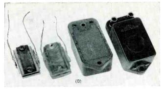
FIG. 4—Precision capacitor made by two methods, the case filled with silica gel, ground cork, paper and wax at (A), and dipped in wax and embedded in plastic within the case at (B)
