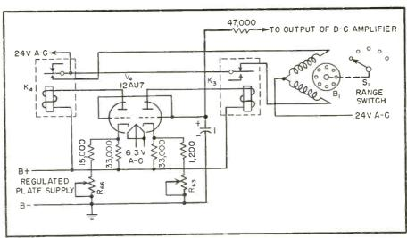
FIG. 2—Automatic scale-changer circuit prevents off-scale operation of the indicating meter without attention from operator
