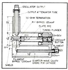
Fig. 2—Physical construction of coaxialline oscillator
