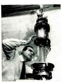
Individual filament and grid elements of the unit triodes in the array are tungsten rods 8 inches long, supported at both ends by means of knife-edge V-notch arrangements. A pantagraphic mounting device has flexible spring-loaded fingers to which the filament rods are hooked. This makes each filament strand and grid rod mechanically independent, and allows vertical movement without disturbing the precise alignments and spacings essential to effective electron optics.
