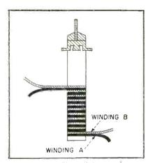
FIG. 1-Construction of bifilar coil
