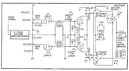
FIG. 5—Differential signal receiver circuit used to control reversible motor over radio link between airport station and remote station
