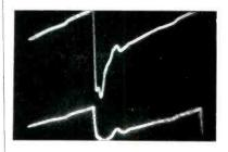
TV horizontal output tube waveform upper trace—grid volts lower trace—cathode current
