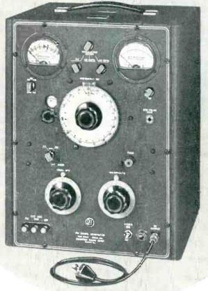
It may also be switched off. Eight fixed frequencies between 50 cycles and 15 kilocycles are available, any one of which may be selected by a rotary type switch.
