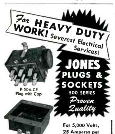
Socket contacts phosphor bronze, knife-switch type, cadmium plated. Plug contacts hard brass, cadmium plated. 2, 4, 6, 8, 10, and 12 contacts. Plugs and sockets polarized. Long leakage path from terminal, and terminal to ground. Caps and brackets, steel parkerized (rust-proofed). Plug and socket blocks interchangeable in caps and brackets. Terminal connections most accessible. Cap insulated with canvas bakelite.
