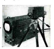
Complete industrial television system draws a total of 350 watts
