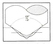
12-Wide-angle needle with the outlines of a 78-rpm groove and a fine groove
