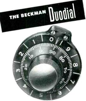
The inner, or Primary dial of the DUODIAL shows exact angular position of shaft during each revolution. The outer, or Secondary dial shows number of complete revolutions made by the Primary dial.
