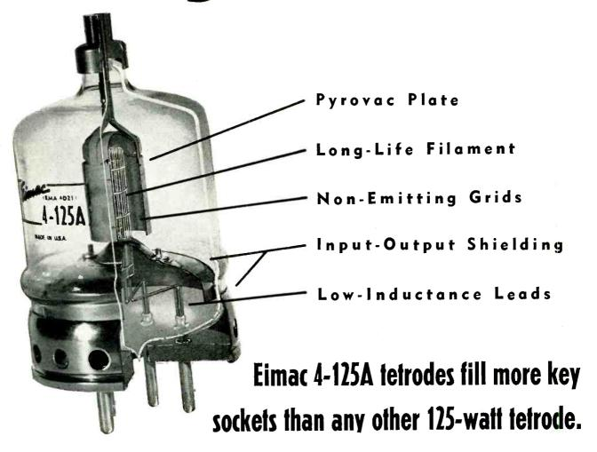
The Eimac 4-125A is the heart of modern radio communication systems. Its dependability-of-performance has been proved over years of service in many thousand transmitters. It will be to your advantage to consider carefully the economy and circuit simplification the Eimac 4-125A offers.
