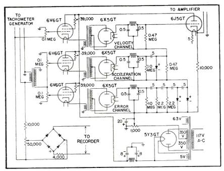
FIG. 3—Three-channel control unit. Input voltage is obtained from tachometer generator on engine, and output drives power amplifier that furnishes dynamometer field current
