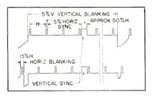
FIG. 7—Composite waveform for the industrial television system
