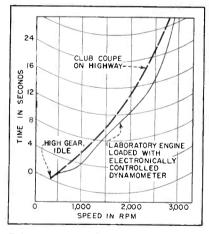
FIG. 7—Correlation of acceleration curves obtained for 1941 Chevrolet club coupe on road and with engine alone in laboratory
