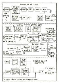
FIG. 2—Setup of stages in the four main sections of the coder unit for the
