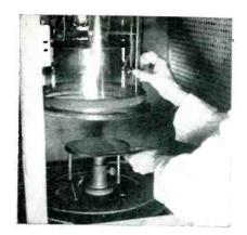
FIG 6-Glass master is placed in sputtering system to form 500-mesh screen
