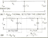
FIG. 1—Equivalent circuits for thermal detector A and for detector with low-pass filter B
