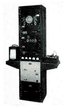
FIG. 10—Electronic correlator built at MIT for obtaining complete autocorrelation curve of a random function automatically on recorder at left
