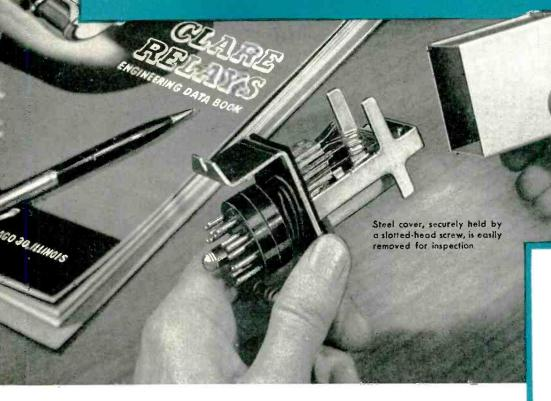
This new CLARE dust-tight plug-in enclosure for the small Type "J" Relay offers designers a number of unusual features for installation on industrial equipment.
