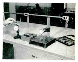
**Inspection and Gaging** ... equipment for checking dimensions of Seamless and Lockseam Cathodes.
