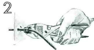
Snap HEYCO into chassis hole. (The Heyco imparts a positive non-slip grip; does not injure wire.)
