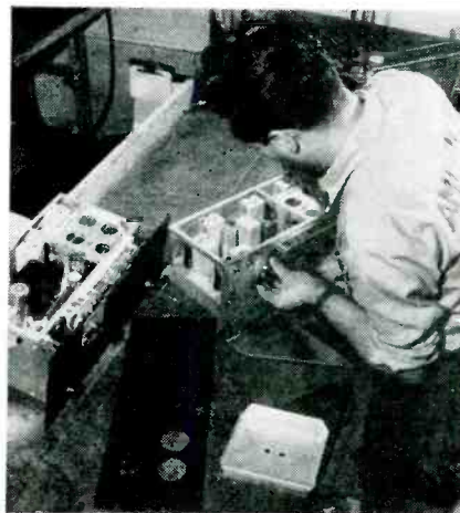
FIG. 2—Popular on the two-meter amateur band, the SCR 522 has been adapted by American Airlines as a ground station receiver
