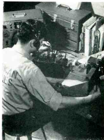
FIG. 3—The AVR 7A beacon receiver is fitted to a standard rack panel and chassis which also contains the accessory units to make it a complete receiver
