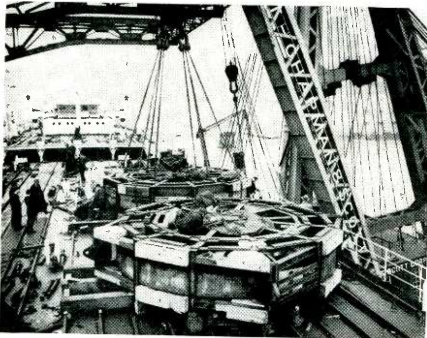
Two giant coils, one weighing 92 and the other 97 tons, are made secure aboard the Seatrain New Jersey for shipment to New Orleans, La. Built at the Brooklyn (N. Y.) Navy Yard for the cyclotron at the Carnegie Institute of Technology, Saxonburg, Pa. (about 375 mi. from N.Y.C.), the coils were too large to go by rail or highway and had to be shipped coastwise to New Orleans, and thence by river to Pittsburgh, Pa., a short highway haul to Saxonburg. The coastal route is about 3,000 miles
