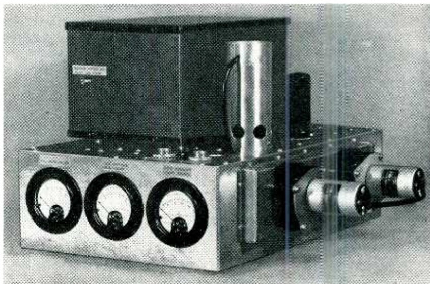
Sweep generator includes electron-coupled oscillator in box on top and sweep circuit in chassis below; blowers are for resistors in sweep circuit
