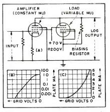
FIG. 1—Balancing voltage developed by variable-mu tube acting as load gives amplifier a logarithmic amplitude response
