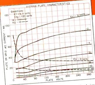
Note the low voltage "knee" on the chart. The design factors of low triode mu and optimum beam plate shapes combined with high mutual conductance make this a *high efficiency* video output tube. It produces ample video out-
