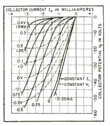
FIG. 1—Typical operating point on the static transfer characteristics of a transistor is at a few milliamperes reverse current in the collector and about one milliampere forward current in the emitter
