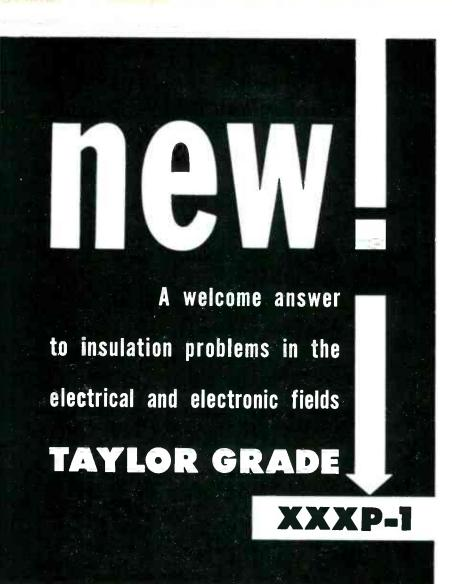
For switch stators and rotors, socket bases, condenser stators, insulating washers, and similar applications . . . Taylor Grade XXXP-1 brings a new combination of insulation resistance plus low power factor and low dielectric constant, *regardless* of humidity.
