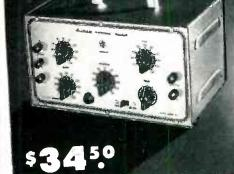
Gives two separately controllable traces with individual inputs on any scope. See both the input and output traces, locate distortion, phase shift, etc., immediately.
