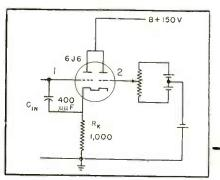
FIG. 1—Functional diagram of yariable reactance
