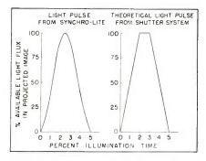
FIG. 6—Comparison of light pulse from Synchro-Lite with theoretical light pulse from shutter system having 2-percent opening and closing times
