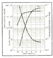
FIG. 4—Characteristics of a single section of a 6J6 tube vary considerably with change in grid voltage
