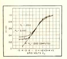
FIG. 6—Values of (1—A) for dual triode
