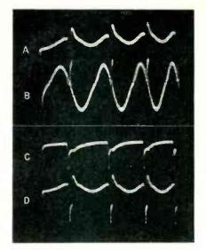
FIG. 5—Pulse transmission through the locked oscillator. Waveform A is the pulse input and oscillator voltage drop across the input resistor, showing  $i_{osc}$  in phase with the pulses. Waveform B is grid voltage lagging 90 degrees behind the pulse fundamental. Waveform C is the output from the discharge tube and Dthe signal input, showing that the discharge is ahead of the sync pulse thereby saving time for retrace
