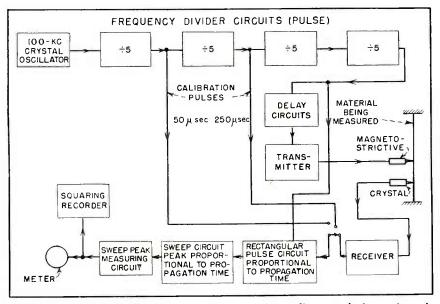
FIG. 1—Block diagram of pulse propagation meter for quality control of a variety of materials ranging from textiles to metals, plastics, concrete and even soap
