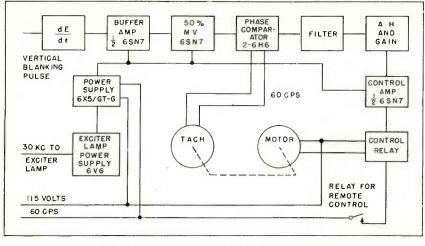
FIG. 3-Speed control amplifier for the projector
