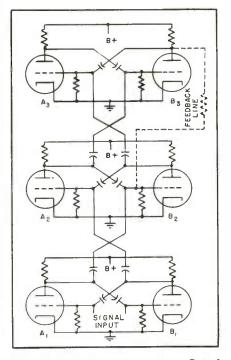
FIG. 2—Multivibrators in series. Dotted portion shows feedback network for nonintegral frequency division
