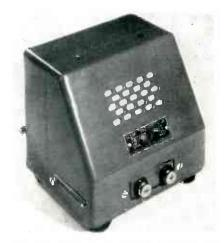
can be used as a sound source, as an annunciator, code practice oscillator, or similar device. Frequency can be adjusted over about 10-percent range.
