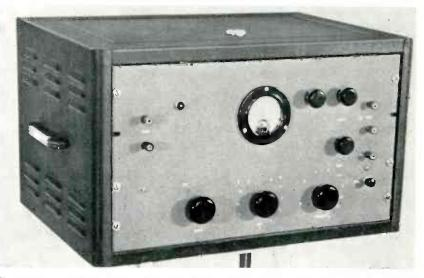
Test equipment, housed in cabinet, could equally well be mounted in rack. Upper lefthand terminals are for connecting oscilloscope; righthand terminals are for input. Three lower controls are, left to right, power switch, attenuator and frequency switch. Upper pair of controls are for bridge resistance, middle one is level control
