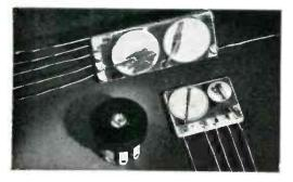
**Two-Piece P.E.C. "Ampec" and Model 1 "Radiohm" Switch** are the Centralab units Paravox uses in its 4½-ounce hearing aid. See below for schematic diagram of this custom "Ampec".
