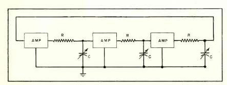
FIG. 13-Block diagram of f-m audio oscillator
