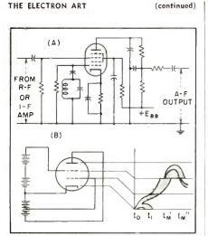
FIG. 1—(A) Phasitron circuit is a multigrid demodulator for fm having the characteristic shown here. (B) Action of demodulator depends on the space charge coupling between two control grids
