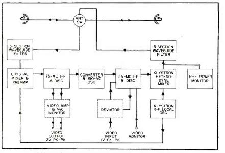
FIG. 3—Block diagram of 6,000-mc television relay repeater
