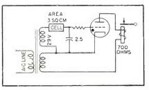
FIG. 1—Typical circuit for photocell and thyratron that supplies 88 milliwatts to operate the relay
