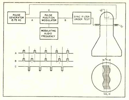
FIG. 9—Test equipment for sync filters using pulse position modulation
