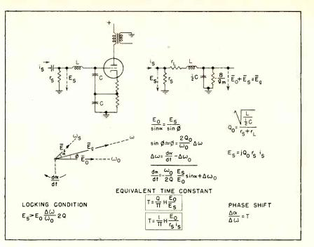
FIG. 8-Derivation of transient response of locked oscillator
