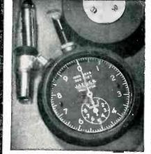
PORTABLE (CHRONOMETRIC) TACHOMETER
