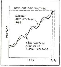
FIG. 1—Signal voltage superimposed on regular discharge curve causes grid voltage to reach cut-off at  $T_1$ , whereas without signal, tube would have triggered at  $T_0$
