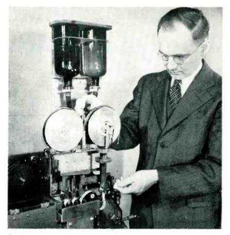
Charles Kunz of Kodak feeds a leader strip through the experimental high-speed hot developing machine used at the receiver
