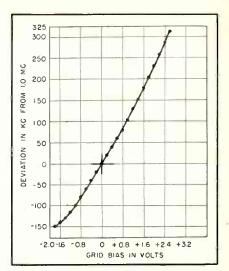
FIG. 11—Frequency deviation of the onemegacycle oscillator
