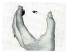
replace such elements as 6H6 and 6AL5 tubes, copper oxide, selenium, and silicon rectifiers. Safe forward current is 0.05 amp and safe back voltage, 60 volts. Shunt capacitance is 0.8 gaf maximum.
