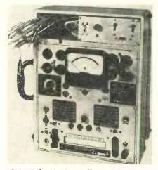
plete tube tester. The instrument represents a combination of the model 805B tube and set tester with the model 730 signal generator.
