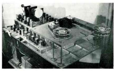
The experimental transmitter employs 35-mm film as data source. Flying-spot scanner at left. Phototube in box at center
