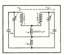
FIG. 8-Circuit to indicate capacitor-shaft coupling
