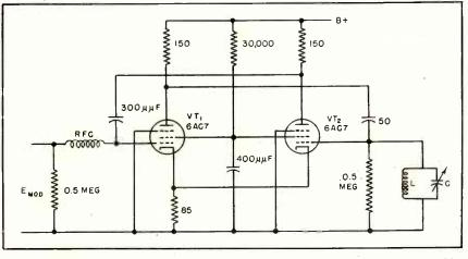
FIG. 10—One-megacycle f-m oscillator using a two-stage amplifie: as a variable reactance
