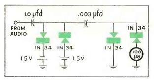
IN THIS PORTION OF THE CIRCUIT, the two 1N34's at the left are used as limiters. They are connected across the audio bus, but are biased so as to pass  $\pm$  1.5 volts of audio. Voltages above this level are clipped off by the action of the diodes. The two 1N34's at the right are used in a full wave counter circuit, and provide a d-c output proportional to the frequency input.
