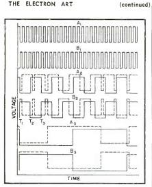
FIG. 3—Plate voltage waveforms for a three-stage multivibrator with and without feedback
