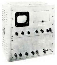
and input impedance is 250,000 ohms. The instrument is useful for determining the characteristics of p-a systems, hearing aids and a wide variety of audio devices.
