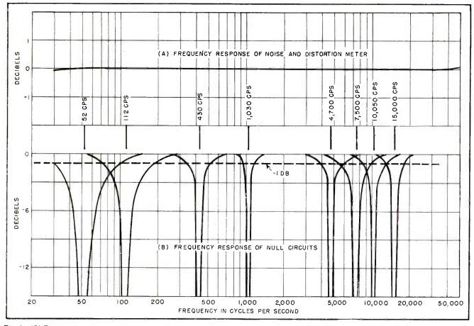
Fig. 3—(A) Frequency response of the meter, with the null bridge bypassed, is flat over the full audio spectrum. (B) The rejection of the null bridge is sufficiently sharp so that second harmonics are attenuated less than a decibel. Problem is to find large inductance with low loss for use at low frequencies
