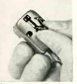
3 Insert new stylus into cartridge with fingers.
