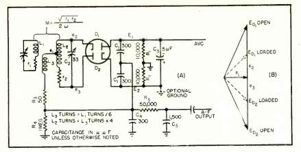
FIG. 2—Ratio detector for f-m. Transformer turns ratios are given and the vector diagram indicates optimum transformer performance
