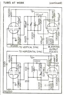
FIG. 1—Circuit diagram of crosshatch generator. Type 12AU7 tubes are used throughout
