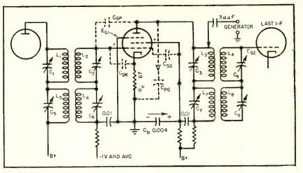
FIG. 5—Representative a.m and f-m intermediate-frequency stage with notations for discussion of regenerative effects
