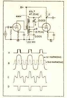
FIG. 1—Test pattern obtained for triggered synchronization with weak noisy signal
