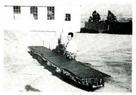
An 18-foot scale model Essex-type aircraft carrier is used to test equipment at the Navy's Electronics Laboratory, San Diego, Calif. While revolving on a turntable in the center of a wire-covered "ocean", the performances of the model's scaled-down radio and radar aniennus are traced on plotting machines in the office at the rear
