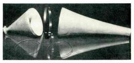
Parts for f-m dummy-antenna assembly. Silver-plated copper spinnings are simultaneously brazed to the brass support ring by induction heating
