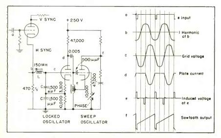
FIG. 4-Circuit and waveforms of locked oscillator
