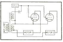
FIG. 3—Suggested circuit for operating a series of motors from different light levels
