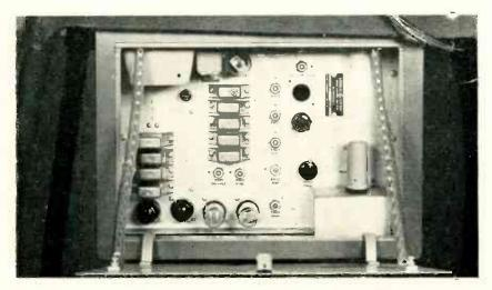
Tube and adjustment side of the speed-control amplifier
