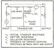
FIG. 2—The transistor can be represented by an equivalent resistance network at low frequencies. A typical load would be 10,000 ohms, a typical input resistance is 500 ohms
