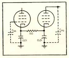
FIG. 6-B-minus decoupling circuit
