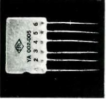
Like all CRL *Couplates*, pentode (above) consists of plate lead and grid resistors, plate by-pass and coupling capacitors. See Bulletins 999, 42-6.
