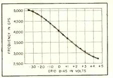
FIG. 14—Frequency deviation of the audio oscillator is linear for about 10 percent each side of the center frequency
