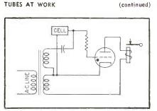
FIG. 2—The relay releases when illumination is removed from the photocell
