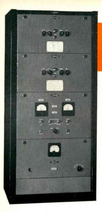
Top to bottom: two Collins 51N-4 communication receivers, Collins 706A-1 radiofeletype converter, and Collins 707A-1 power supply.
