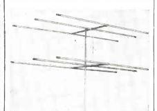
ception in areas remote from transmitters, is constructed of one-inch aluminum tubing stock.
