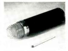
FIG. 2—Small capacitor microphone modulates high-frequency oscillator in highfidelity sound recording system that uses new demodulator circuit
