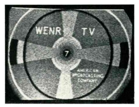
FIG. 6—Test pattern obtained for locked oscillator with weak noisy signal
