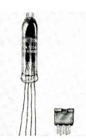
miniature diode with characteristics similar to those of one-half of a 6AL5. Resonant frequency is over 1,200 mc. The tube has a 6.3-volt 150-ma heater and is intended for applications up to a few hundred megacycles where very small size is important.
