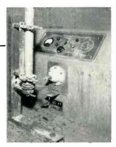
This simple jig positions and aligns stainless-steel parts for brazing. Heating time required with the 4-turn coil is about onehalf minute
