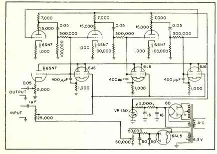
FIG. 12-Circuit of frequency-modulated audio oscillator
