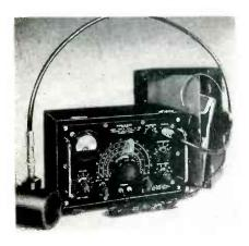
tector contains new features such as instrument indication (for use in noisy locations) adjustable frequency-modulation (facilitating measurement of seriously corroded parts), permeability tuning unit, and increased frequency range for measurement of steel down to  $\frac{1}{16}$ inch. Normally battery powered, the unit can be furnished for a-c power if desired.
