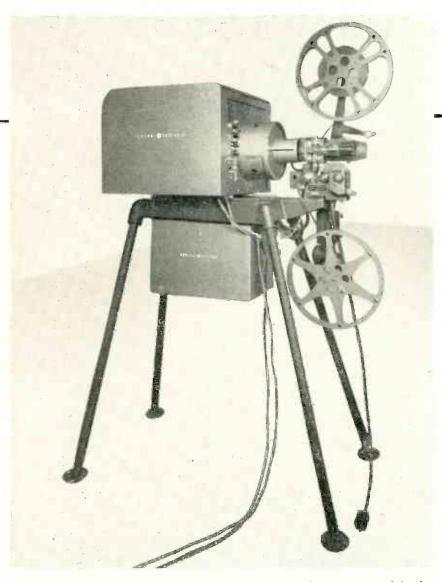
Complete television film projector. The speed-control amplifier is mounted in the suspended cabinet
