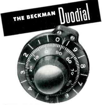
The inner. or Primary dial of the DUODIAL shows exact angular position of shaft during each resolution. The outer, or Secondary dial shows number of complete revolutions made by the Primary dial.
