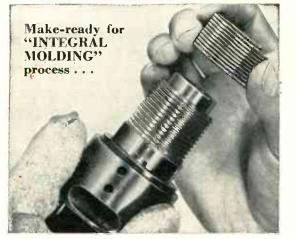
The coiled resistance element is threaded on the molded core
