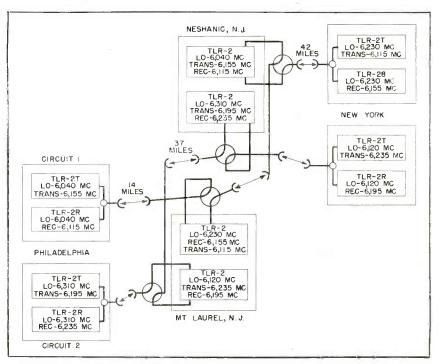
FIG. 1—The 6.000-mc two-channel television relay system, reversible, linking New York and Philadelphia
