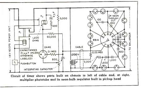
tube breaks down, and relay  $R_2$  is energized, thus releasing  $R_1$ . In dropping back,  $R_1$  turns off the enlarger and the power to the phototube and also connects a 50,000-ohm resistor across the integrating capacitor, thus discharging it in preparation for another cycle. Between timing cycles the equipment draws no power and thus can be left permanently connected. It has no warmup delay, so to operate it for the next cycle all that is necessary is to push the button again.
