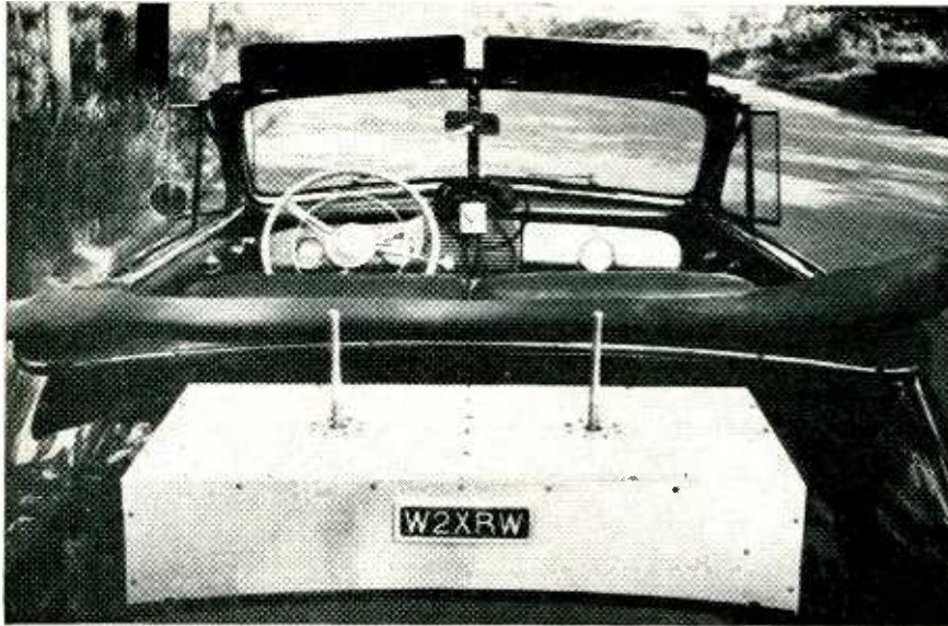
Transmitting and receiving ground-plane antennas and of Mobile 2 unit. Dashboard mounting of handset and send-receive switch provides convenience
