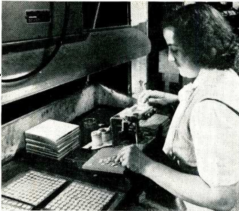
Manufacturing disc-type capacitors using ceramic dielectrics
