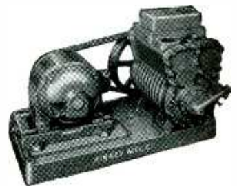
Kinney Compound Pumps are available in 2 sizes with displacements of 15 and 46 cu. ft. per min. They regularly maintain low absolute pressures to 0.5 micron or better.
