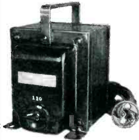
PORTABLE AUTO TRANSFORMER Pri.: 220V-110V— One KVA, 50 60 cycles, single phase Sec.: One KVA
