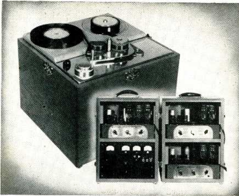
The experimental three-channel stereophonic drive unit and (inset) the amplifiers and mixer. Three microphones and three loudspeakers complete the system
