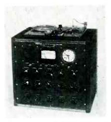
bias and erase oscillator, playback amplifier, monitor amplifier and speaker. Bias frequency range is adjustable from 30 to 80 kc with a total recording and playback distortion under 3 percent at 400 cycles.
