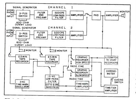
FIG. 3—Simplied block diagram of more important elements making up a complete monitoring station
