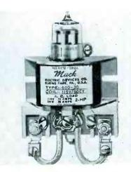
relays with 3-coil terminals and featuring a replaceable tube which is hermetically sealed with the contacts, having mercury-to-mercury make and break in inert gas. Contact ratings and coil data may be found in bulletin 410.
