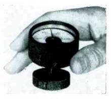
of 0.052 inch, permits measurement of flux in small-gap magnets of standard or irregular shape. Also available is a triple kit combining three meters of different ratings in a single carrying case. Ask for bulletin GEC-238.
