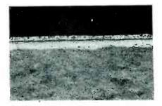
FIG. 3 --- Photomicrograph showing (bottom) alloy, aluminum cladding, and (top) solder
