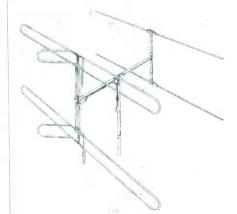
conversion kits has been assembled. In all there are 22 different types ranging from the single straight dipole to the double-stacked folded dipole with high-frequency lobes, as illustrated. The line covers the 44 to 216-mc range, channels 1 to 13 and f-m bands.
