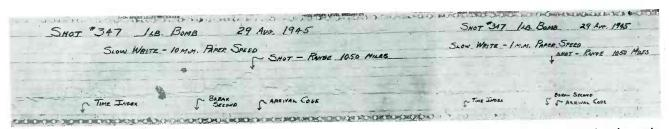
FIG. 6—Slow and fast graphic recordings of bomb signals from 1,050 miles. This record has been made from a replaying of the magnetic tape record. Point of maximum energy is timed to an accuracy of 0.1 second. The arrival code mark is made by the observing operator when he hears the maximum signal arrive and is chiefly useful in identifying the peak
