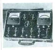
sion investigations and cathodic protection testing both in field and laboratory. It provides all of the instrumentation required to cover the wide range of d-c current and potential measurements necessary in this field. The unit weighs about 23 pounds.
