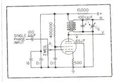
FIG. 3-Circuit of circular sweep generator
