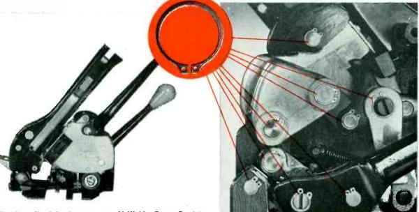
The Acme No. 3 Steelstrapper uses 23 Waldes Truarc Retaining Rings to position and hold shafts against frequent heavy pressure.
