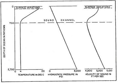
FIG. 1—Graphic explanation of the sound channel effect upon which the solar system depends
