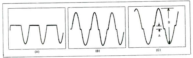
FIG. 1—Clipped sine wave (A); double clipped sine wave (B); double clipped sine wave showing phase shift (C)
