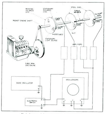
Block diagram of the rocket-engine pump-seal tester
