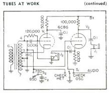
FIG. 2—Audio oscillator and mixer circuit. The center position of switch  $S_1$  is the normal position
