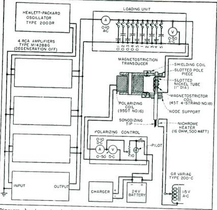
Diagram showing setup for tinning aluminum alloys. A switch (not shown) permits paralleling of 4, 7.5 or 15-ohm amplifier taps
