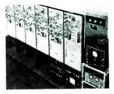
High speed computer developed at the Servomechanisms Laboratory of M.I.T. uses germanium diodes, performs arithmetical operations using five-place binary numbers, and indicates solution by neon lamps
