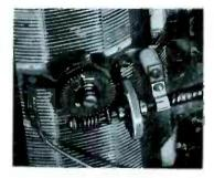
Close-up of flexible shaft connection to a variable resistor through simple worm gearing. With arrangements like this you can get smooth, accurate fingertip control.
