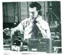
and is completely housed in one cabinet with handset attached. The receiver delivers 2.5 watts of power to the speaker, operation being from a 6-volt battery with a current consumption of 7.5 amperes. Power output of the transmitter is 5 watts of r-f carrier.
