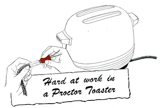
In the streamlined Proctor Toaster it takes a 1-inch length of BH Fiberglas Sleeving to provide supplementary insulation over the asbestos-covered leads on the built-in heater cord. With BH Fiberglas Sleeving there is no possibility of a partly uncovered braid . . . no threads to break or unravel. This extra margin of safety means trouble-free service.
