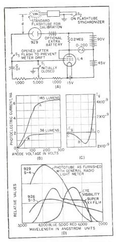
FIG. 1—Circuit and characteristic curves of photoelectric light-integrating meter for capacitor-discharge electric flash lamps
