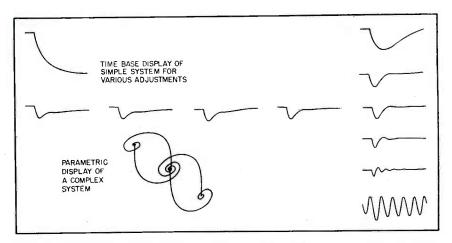
FIG. 4—Reproduction from oscilloscope tracings show how optimum response of plant can be determined by systematic adjustment of various controller adjustments
