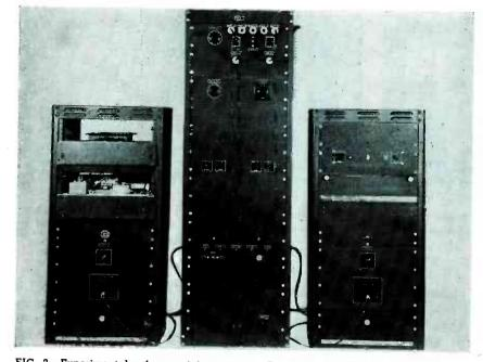
FIG. 2—Experimental sofar receiving station. Recorders and timing equipments are in smaller racks. Center cabinet comtains controls, amplifiers and power
