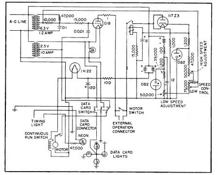
FIG. 1-Circuit of electronic variable-speed-control for the camera motor
