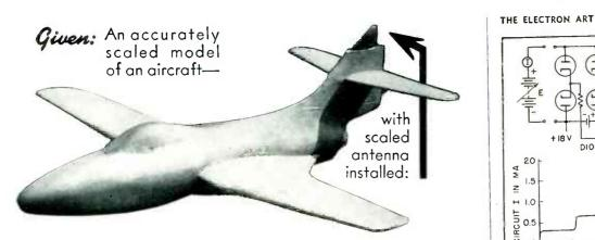
**Find:** The radiation pattern of that antenna on that aircraft in any plane and for either vertical or horizontal polarization.
