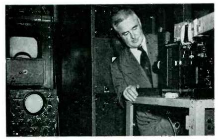
Television picture is recorded on 35 mm film, which is then completely processed in 66 seconds, by the equipment that Paramount's vice-president Pcul Raiborn is inspecting
