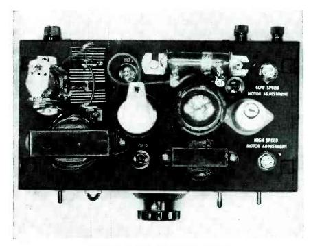
Top view of motor speed-control chassis
