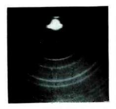
Aluminum mounted on a Formvar film to give a total thickness less than 500 Angstrom units produced this transmission electron diffraction pattern
