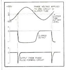
FIG. 5—Phase relations in pulse-forming circuit
