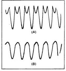
FIG. 6—Clipped sine wave with fundamental partially suppressed (A); and with fundamental partially accentuated (B)
