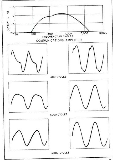
FIG. 5—Response of a communications amplifier. Oscillograms at left show effect on clipped sine waves and, at right, on double clipped waves
