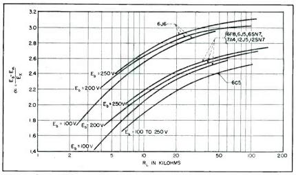
FIG. 4—Curves giving value of  $\alpha$  in terms of load resistance and plate voltage for several types of tubes
