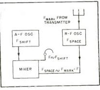
FIG. 1—Essential stages of a system for checking carrier shift
