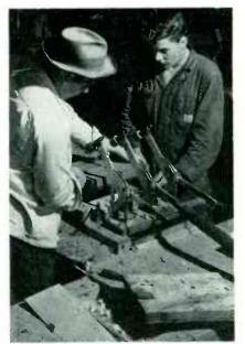
A loudspeaker mount board and several small blocks are glued simultaneously in about 30 seconds with this jig
