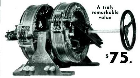
11.5 KVA; Fixed Winding; 115 Volts; Commutator Range 0-115 Volts, Maximum Amperage 100. Can be reconnected for 230 volts with maximum amperage of 50. Blueprint of connections supplied.
