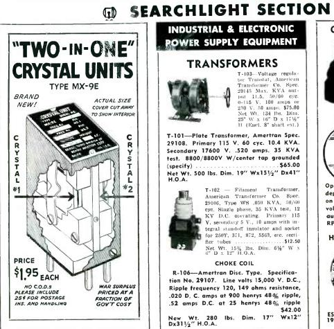
Each unit contains two 3/4" sq. crystals differing in frequency by 455 k.c. The following combinations are available:
