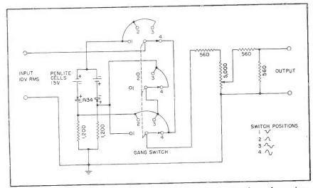
FIG. 2—Circuit diagram of a sine wave clipper with output waveforms for various switch positions indicated
