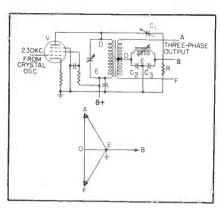
FIG. 2—Single-phase to three-phase transformation circuit and phase diagram
