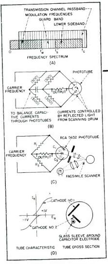
FIG. 1—Basic considerations in design of bridge modulator for fascimile
