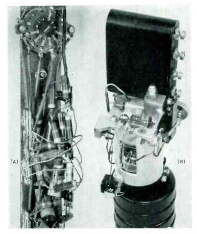
FIG. 1-Electrical analog (A) simplifies design of pneumatic controller (B)
