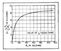
FIG. 7-Effect of load resistance
