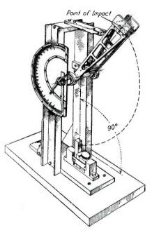
Figure 1—Cantilever Beam (Izod Type) Impact Machine used in testing impact resistance of electrical insulating materials,
