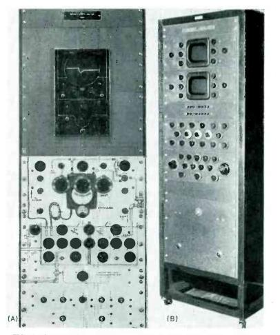
FIG. 2-Circuits of analog computer simulate plant and controller
