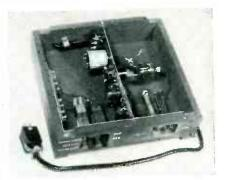
Constructed in this fashion, the carrier shift check meter fits under a BC-221 frequency meter
