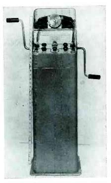
A balloon-supported antenna is used on this lifeboat equipment. When cranked it automatically sends out SOS
