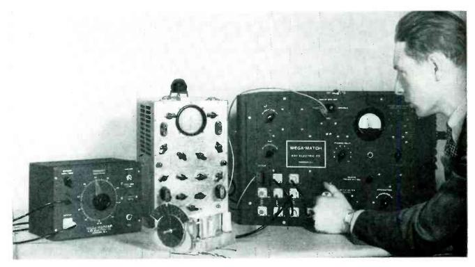
FIG. 1—Frequency-scanning vhf impedance meter in use, with conventional oscilloscope used as indicator
