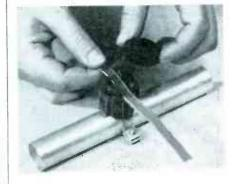
arrester designed to fit into television and f-m receiver installations. The device features a new method of attaching the transmission line which avoids cutting and splicing.
