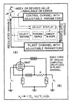
FIG. 3—(A) Block diagram of automatic control computer, and (B) basic circuit of used in the analog computer elements
