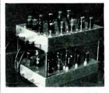
Ten delay circuits with their input bridges and the pulse mixer are on the upper chassis. Coaxial cables connect to the lower chassis containing the rest of the experimental system for reducing bandwidth
