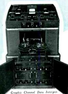
tation Equipment-Type D1-2: showing front compartment doors open for tape loading and ad-justment. Unit provides 1 time base and 2 information channels.
