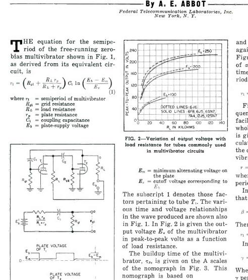
$\tau_B = 4 \left( R_L + r_p \right) C$ The value of  $\tau_B$  obtained here covers the period required for the voltage wave to reach 98 percent of its peak value. FIG. 1-Basic zero-bias free-running mul-
