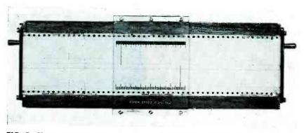
FIG. 7—Shot arrival time evaluator for two different recorder speeds. The long vertical line is placed over the maximum signal and tenths of seconds read off to the nearest chronometer time mark
