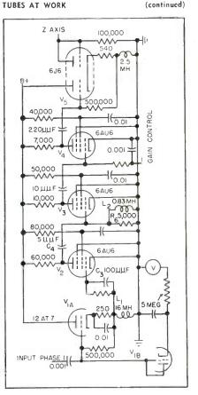
FIG. 4-Pulse generator for one phase
