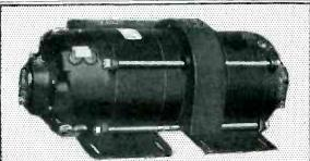
MODEL 5AM49AB3 INPUT: 440 volts, 3  $\phi$ , 60 cycles, 1 ampere OUTPUT: 250 volts, 1.5 amps. 375 watts, cont. operation, 40 c.—Temp. Rise. 3450 RPM.
