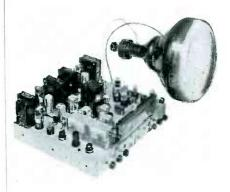
wired and tested unit, less cabinet. The receiver tunes continuously from 44 to 216 mc and a switch is provided to turn off sweep and high-voltage circuits when f-m reception alone is desired.
