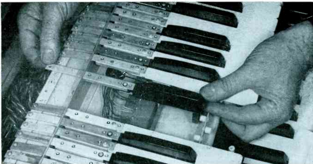
New organ-type electronic instrument uses conventional keyboard; and pipe organ playing and control techniques are directly applicable. Contacts located under the keys control individual vacuum-tube oscillators. To avoid humidity problems in hot and humid areas, windings have been potted where convenient, and coils have been wax impregnated
