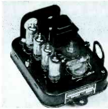
Top view of control amplifier with sprayed wiring
