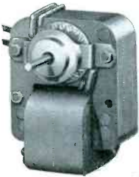
MODEL K —Used in all 25 cycle and some 50 and 60 cycle Alliance Phonomotors. This basic 2-pole induction type motor will adapt to any standard AC voltage or frequency. Develops up to 1/100 h.p. Drives the heavier type record changers, radio-phonograph turntables, tuning devices and operates many other controls and automatic devices.
