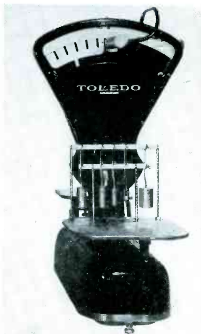
FIG. 2—Scale modified to check fuel consumption of automobile engines. Weights are automatically added as tank empties, to spread out readings
