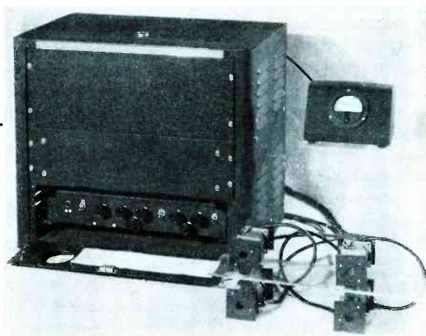
Electronic thickness gage. The indicating meter may be seen at the upper right. Standard and measuring heads, shown without their mounting fixtures and roller wheels, are at the lower right
