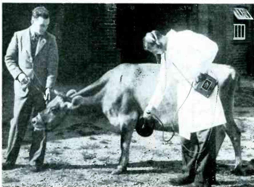
Metal detectors offer a means of diagnosis for sick cows who swallow stray bits of metal with deleterious effects
