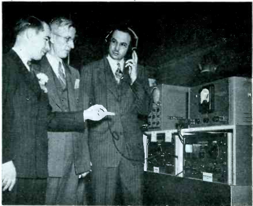
Broadcast engineers Glenn Koehler and Harold Engel of WHA, Madison, Wisconsin, measure distortion and noise in an audio signal while Bill Broughton of GE (at left) explains the operation of the equipment
