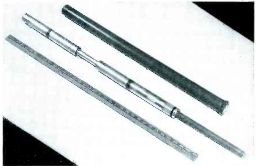
Internal view of two-section colinear array for broadcast service. A cover of fiberglass tubing protects the array from the weather
