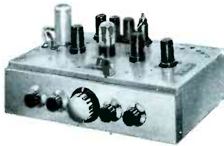
PRE-AMPLIFIER CHASSIS — 15¼" x 7¼" x 2½" — aluminum, finished in an aluminite finish.
