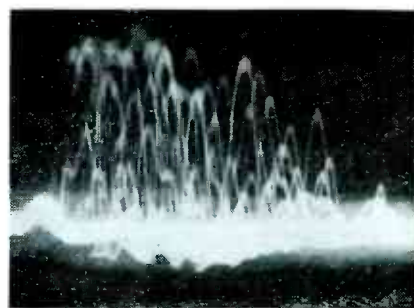
FIG. 3—Oscillogram showing echo fluctuations as a person approaches
