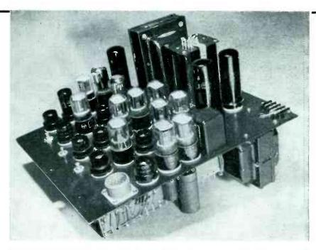
Each 24-tube control amplifier that feeds a Diehl motor contains eight 6H6 tubes used to sharpen and clean the pulse caused by a registration mark to a width of less than 20 microseconds. This is necessary to distinguish the pulse caused by a registration mark from that caused by irregular reflections from the web of metal foil
