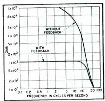
FIG. 5—Frequency characteristics of the electromechanical system with and with out feedback
