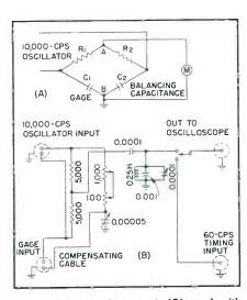
FIG. 2—Basic bridge circuit (A) used with gage, and final version (B) using tuned filter and compensating cable for limiting response to narrow band of frequencies around 10.000 cps
