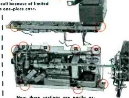
Now three sections are easily assembled separately, and quickly fastened together with SPEED NUTS into completed unit.
