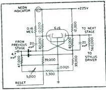
FIG. 2—Binary counter stages use this typical flip-flop circuit
