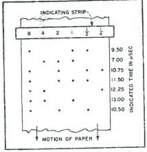
FIG. 3—Interval measurements are shown as rows of dots. Sum of dot values in each row equals interval duration
