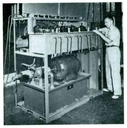
Complete setup of electronic and hydraulic units that connect to the printing press.
