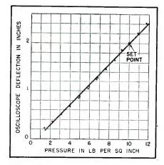
FIG. 4—Static calibration curve of pickup when using 0.02-inch thick steel diaphragm
