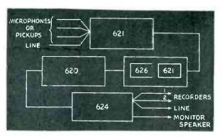
Single Chamnel Systems: for recording from a microphone or record or playing back from a pickup.
