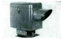
distances up to 1,000 ft. Its applications include traffic control, counting and limiting, and the like. The light source contains a lamp, transformer, and motor-driven slotted disk which modulates the light beam at about 900 cps. The relay, because of its tuned circuit, is responsive only at this frequency.
