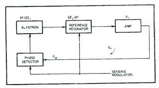
FIG. 4—A basic electronic automatic frequency control
