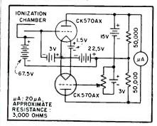
FIG. 4—Radioactivity meter uses nonmicrophonic subminiature electrometer tube
