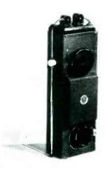
complete with batteries. It operates in the 144 to 148-mc band up to three miles or farther. Featured in the design is adjustable tuning on both transmitter and receiver.
