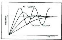
FIG. 5—Motor tuning time plotted against corrective feedback
