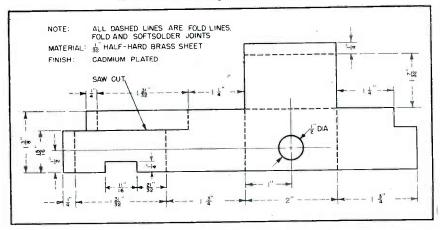
FIG. 6—Shield can for 465-mc resonator. If dimensions are followed accurately, both resonators may be tuned over band without mechanical adjustment, by adjusting loading capacitors
