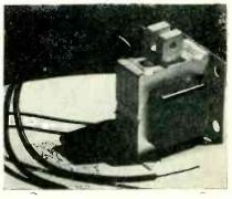
Frame and bracket as well as frame laminations are all welded together. Eddy current losses are thus reduced.
