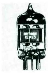
a discriminator, ratio or diode detector, avc. diode, clipper, or lowpower rectifier. Each set of elements can be used independently of the other and each has a resonant frequency of about 700 megacycles.
