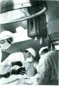
The three-lens television camera, requiring no special lighting, is installed on a track above the operating table. The microphone mounted just behind the camera picks up the running commentary of the operating surgeon. RCA equipment was used
