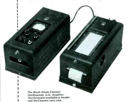
Instantaneous, permanent, ink-on-paper recordings by Brush Oscillographs make their use almost unlimited. Accurate recordings of strains, pressures and countless electrical phenomena can be made over a frequency range of D.C. to 100 c.p.s. Either A.C. or D.C. signals can be measured. Whenever desired, recordings may be stopped for notations on chart-paper.
