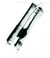
FIG. 1-Variable-inductance myograph has supporting columns made of 5-cm lengths of soda straw. Points are usually so spaced on specimens that coils are 2 to 3 mm apart
