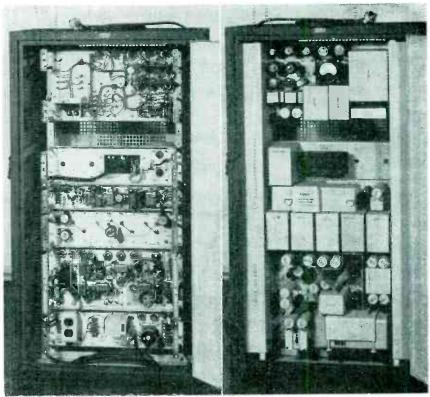
FIG. 2—Front and rear views of video amplifiers used in short haul circuits
