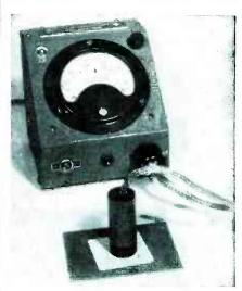
FIG. I—Electronic micrometer measures change in coupling between probe coils caused by displacement of probe from metallic reference surface
