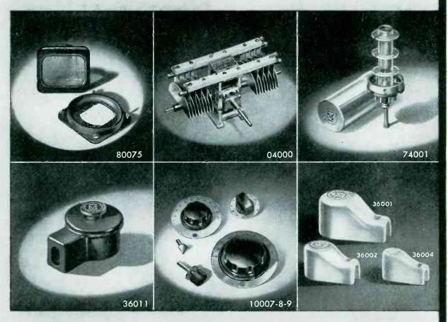
Illustrated above, left to right; Top row: The No. 80075 cathode roy tube Bezel, the No. 04000 series of adjustmble shaft angle, center drive variable transmitting condensers and the No. 74001 permeability tuned shielded plug-in coil form. Bottom row: The No. 36011 snap tock multiple finger contact plate caps, the small panel dials and finally the Ceramic insulated plate caps.
