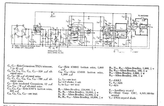
FIG. 2—Complete schematic of transmitter. Socket orientation and feed-through numbers correspond to mechanical layout of chassis, shown in the drawing at the right
