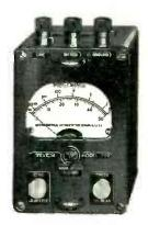
Direct Reading Insulation Tester — Model 799. Compact, one-hand-operated insulation tester with .1 to 10,000 megohm range, using a test potential less than 50 volts d-c. Indicates: 1. Insulation properties. 2. Leakage resistance. 3. Conductivity of insulating materials. 4. Leakage due to moisture absorption.
