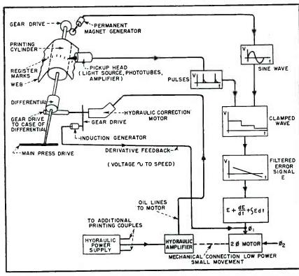
FIG. 2.—Schematic of the register control system. Functions of the electronic stages are illustrated in blocks at right
