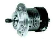
Fixed phase voltage 26 volts, variable phase voltage 49 volts max. 1.05 in/oz stall torque. Rotor moment of inertia 7 gm/ cm<sup>2</sup>. (Stock #S-97)
