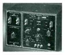
mitter carrier frequencies and other h-f signals against WWV. Model 90515 combines the functions of the secondary frequency standard model 90505 and the h-f multiple and mixer unit, model 90511. Model 90511 is also available separately.
