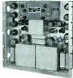
Unit has its own power switch, fuses, pilot light, and voltage control.
