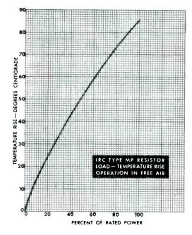
DERATING. Type MP Resistor power ratings are based on an ambient temperature of 20°C. When operated at any higher ambient, it is recommended that they be derated according to the following curve. For example, suppose an MPO Resistor is to be operated in an ambient temperature of 40°C. From the curve it is seen that the permissible load is 74% of the rated load. Since the MPO is normally rated at 30 watts, then at 40°C., it should not be loaded to more than 74% of 30 watts, or 22.2 watts.
