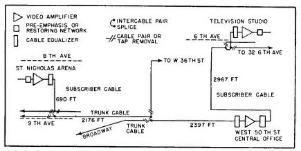
FIG. 4—A typical short haul circuit connects studio, telephone central office, and remote pick-up points
