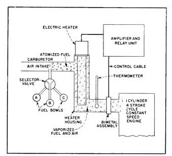
FIG. 1—Block diagram of knock-testing engine used for determination of octane ratings of various gasolines in refineries and petroleum-testing laboratories, showing location of bimetal assembly used with vacuum tube for temperature control
