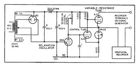
FIG. 2—Cycler circuit for sweeping pen of recorder periodically back to zero, to black in entire area between signal strength curve and zero. Rate of sweep may be varied from once per second to once every 5 seconds by adjusting 30-megohm resistor
