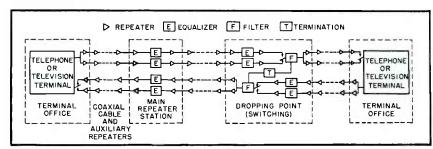
FIG. 6—An auxiliary parallel circuit in each direction is provided for emergency use in this layout of a typical coaxial system
