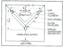
Convectron vertical position sensing tube made by Eclipse-Pioneer Div. of Bendix changes resistance of its two arms when displaced in the plane through its legs
