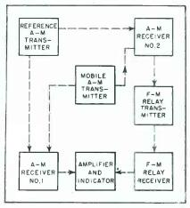
FIG. 1—Airline distance is measured with this setup
