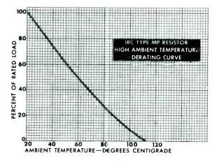
TEMPERATURE COEFFICIENT. -.005% °C. for low resistance to -.07% °C. for high resistance value.
