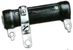
The IRC Adjustable Power Wire Wound Resistor consists of a standard tubular resistor with a track of exposed wire. Contact is kept with the wire by means of a metal band which, when power is turned off, can be adjusted to any position along the resistor.
