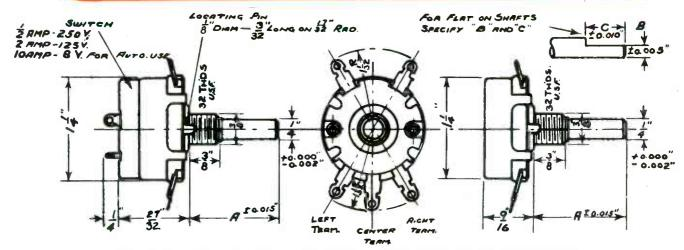
Depth from Mounting Face. Dual  $1\frac{1}{4}$  Triple  $1\frac{29}{32}$  For Switch Add  $\frac{9}{32}$
