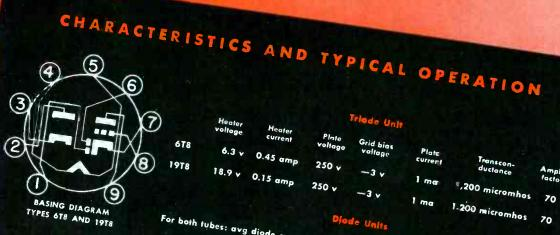
For both tubes: avg diode current, per unit, with 5 v d-c applied..................................20 ma
