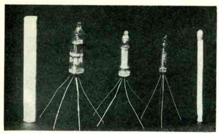
FIG. 1-Triode in T-3 bulb compares in size to cigarette; diode in T-1 bulb is approximately the same diameter as a wooden match; triode at center in T-2 bulb
