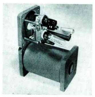
The pickup head and explosion-proof housing are mounted on the press. It contains two phototubes and two amplifier tubes so that if one set fails, the other set is switched into the circuit
