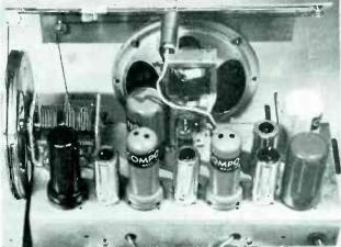
Photographs here show how Cosmo Electronic Corp., New York City, achieves complete plugin construction (except for the gang tuning capacitor) in their five-tube universal a-c/d-c superheterodyne radio receiver. Promotion will feature ease of servicing; any plug-in unit, including loudspeaker unit which screws to chassis but has plug-in connections, is to be available from dealers at price of \$1.85.
