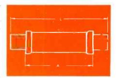
WINDING FORMS. Highest grade, non-hygroscopic ceramic winding form, chosen for mechanical strength, resistance to thermal shock and freedom from moisture absorption.
