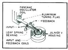
FIG. 3—Construction details of the galvanometer-type movement. The input and feedback coils are wound one above the other
