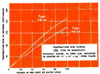
RESISTANCE VALUES. 1 ohm to 5,000 ohms for the PR 25 Rheostat, and 0.5 ohm to 10,000 ohms for the PR 50 Rheostat are standard.
