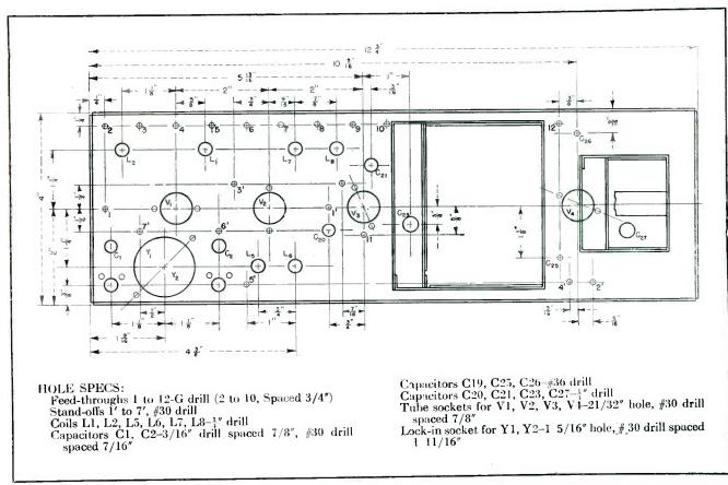
FIG. 3—Mechanical layout of chassis. Slight differences from layout shown in photos have been introduced to simplify construction.
