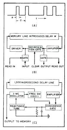
FIG. 1—For use with delay lines, information is in the form of pulse chains (A). These chains can be recirculated (B) through gates and the line so as to be stored as long as necessary. To compensate for temperature effects on the mercury lines, a timing oscillator (C) can be frequency controlled by an auxiliary line, the output being used to time pulses to the bank of mercury memories
