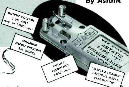
Where high sensitivity, excellent reproduction, low needle noise or needle talk, and low needle pressure are required . . . and cost economy is an important factor . . . Astatic earnestly recommends this new Model "LT" Crystal Cartridge.
