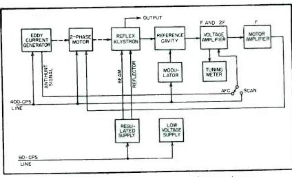
FIG. 9—Block diagram of an afc system with automatic scan
