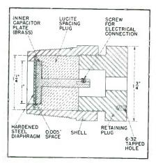
FIG. 1—Cross-section of capacitance-type pressure pickup. Sound waves act on steel diaphragm at left, causing capacitance between grounded diaphragm and insulated brass plate behind it to vary. Shell and retaining plug are turned from 1%-inch hexagonal steel stock
