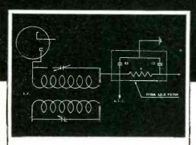
"Filpec" gives you flexibility! Schematic diagram above shows typical Filpec application as a balanced diode load filter. Filpec can be designed for you to meet a wide range of filter applications.
