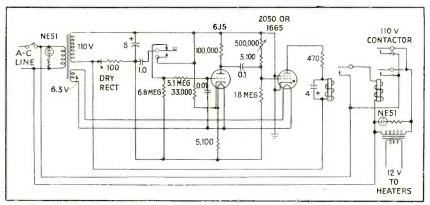
Timer circuit for automatic control of heat from the permanent wave machine
