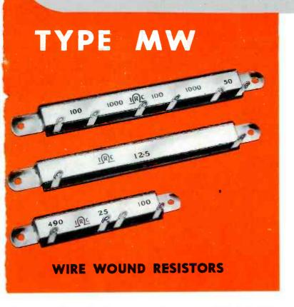
Because of its radical departure from conventional design, the type MW Insulated Wire Wound Resistor is unsurpassed for adaptability to an extremely wide variety of design requirements. Completely insulated and protected, these flat type resistors are encased in durable molded phenolic compound and mounted with a metal bracket of unique design. The mounting bracket actually transfers heat from inside the chassis to the outside, thus providing unusually rapid heat dissipation.
