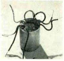
connected to give primary impedances of 500, 150, or 50 ohms. The coils can also be used in a pushpull circuit. The unit is flat within plus or minus 1 db up to 25,000 cycles. Further characteristics can be obtained from the manufacturer.
