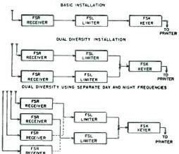
The FSR Receiver, the FSL Limiter and the FSK Keyer are the three units comprising this equipment and the use of multiple FSR's and FSL's makes passible space or frequency diversity or both.
