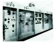
transmitter illustrated features front-panel continuous tuning over its entire frequency range from 2.85 to 22.5 mc.
