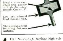
age and small size for television applications. For use as filter and bypass capacitors in video amplifiers.
