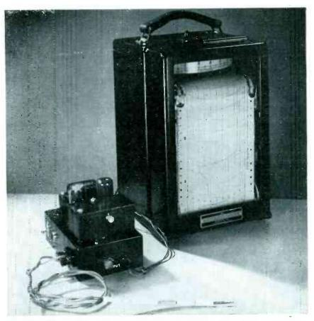
Small chassis at left contains the d-c amplifier and power supply used with the recorder and thermocouple (bottom) to measure transients in a thermal process
