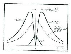
FIG. 2—Resonator-detector output
