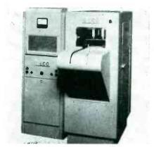
single-phase power. It can operate in either the 13- or 27-mc range, and at full load, power consumption is 3.6 kva. Total weight is 350 pounds.
