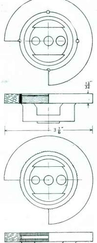
SOLUTION: RICHARDSON PLASTICIANS RECOMMENDED ADOPTION OF MOLDED PROCEDURE, INSTEAD OF THREADING THE SPIDER, THIS SECTION WAS DEEPLY KNURLED & A CENTRAL GROOVED RECESS WAS CUT AFTER KNURLING. THE SPIDER WAS MOUNTED IN A SUITABLE MOLO & DISKS OF SATURATED MATERIALS WERE MOLDED INTO PLACE. MATERIAL FILLED RECESS & KNURLED PORTIONS TO GIVE PERFECT BONDING.
