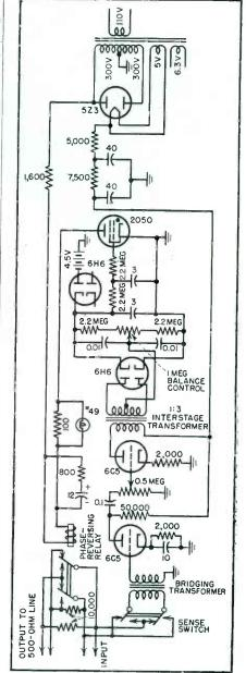
Automatic phase reversal of an audio signal is done by this circuit
