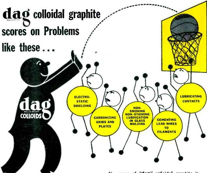
These are but a few of many problems for which "dag" colloidal graphite is often the only practical answer. Any problem requiring a slippery dry solid lubricant which conducts heat and electricity and resists extremes of temperature; which is truly colloidal in size and therefore capable of capillary penetration; which is chemically inert and anticorrosive, opaque and gas-absorbent, is a problem for the "dag" team of properties to challenge.
