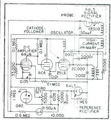
FIG. 3—Changes in probe coil coupling produce variations in rectified output of secondary winding. These are measured by microammeter to give readings of thickness. Reference rectifier, d-c amplifier, and cathode follower form feedback network controlling oscillator screen voltage to give practically constant output
