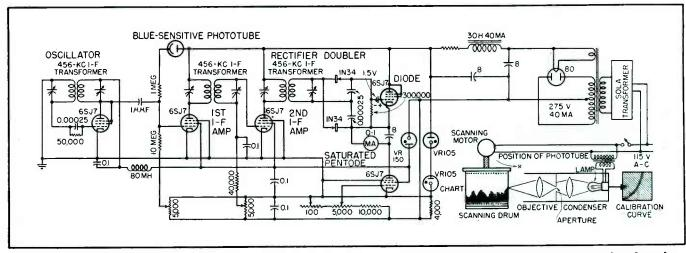
FIG. 3—Circuit of electronic scanner used for analysis of charts. Arrangement of optical system is shown at lower right; phototube is mounted on carriage along with lenses and lamp, and picks up light reflected from spot on chart
