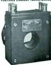
Wesfon Model 481 Type 4 (see illustration). This unit can be used with any precision 5 Amperes A.C. Meter to extend the ranges of the meter to 50. 100, 200. 250, 500 or 1000 Amperes A.C. Accuracy within % of 1%; Normal Secondary Capacity = 15 Va; Binding Posts for 50 Ampere tap; Inserted primary for 100, 200, 250, 500 and 1000 Amperes; Insulated for use up to 2500 volts, List Price \$98.00......NET fob. NY \$35.00
