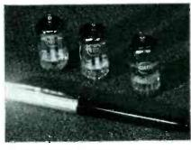
Both the triple-diode triodes contain three high-perveance diodes and a high-mu triode in the same envelope. They are designed as combined a-m and f-m detectors and audio-frequency amplifiers.
