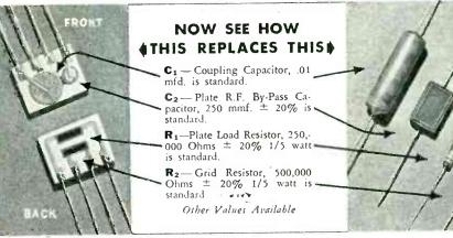
First commercial application of the "printed circuit", CRL's new Couplate offers a complete interstage coupling circuit consisting of an integral assembly of *Hi-Kap* capacitors and resistors closely bonded to a steatite ceramic plate and mutually connected by metallic silver paths "printed" on the base plate.
