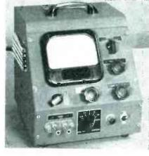
electronic microammeter has five sensitivity ranges from 0.01 microamperes full scale to 100 microamperes full scale with 40 millivolts full-scale input on all ranges. The instrument can also be used as a null-detecting galvanometer with a sensitivity of about 10 millivolts full scale. Write for descriptive literature.
