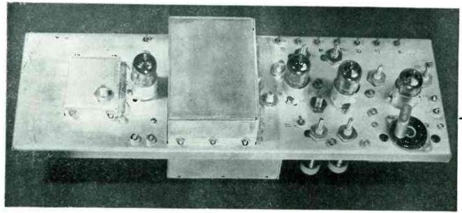
Top view of transmitter. Output of 4.3-mc crystal (lower right) is multiplied 108 times in three tubes to 465 mc. Final stage, a 674 triode (left), produces one-quarter watt output
