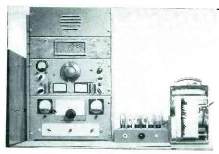
Receiving rack, cycler chassis, and graphical recorder used at Ottawa frequency monitoring station for recording sky-wave signals from broadcast stations
