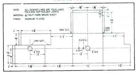
FIG. 5—Shield can for 232.5-mc resonator. Made from brass sheet, this structure can be bent into shape without machining
