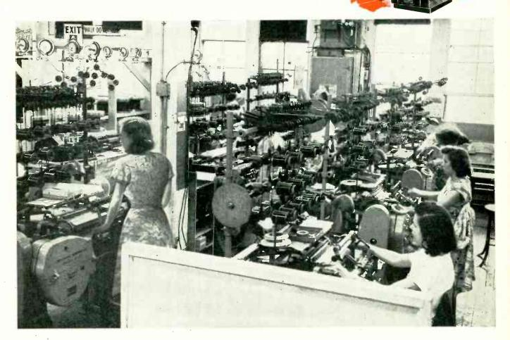
Transformer coils are wound, 14 at once on the same machine, at speeds up to 2500 rpm... on the No. 104 Universal Coil Winding Machines used by a company famous in the field of electronics.
