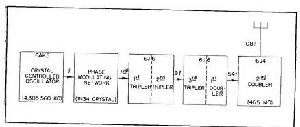
FIG. 1—Block diagram of transmitter. Tubes are conserved by operating three 636 triode sections as triplers. Phase modulation network produces 25-kc deviation
