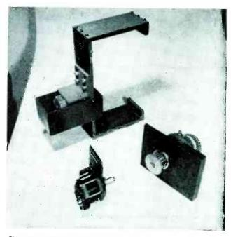
Sinewave p.m generator at lower left, ten-horsepower hydraulic motor at right, and induction generator for tackometer feedback at top
