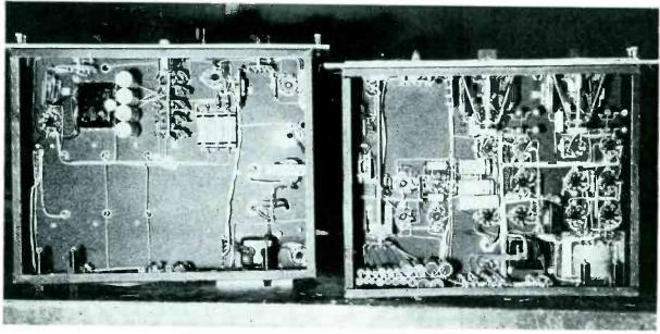
Wiring is kept close to chassis to minimize stray fields
