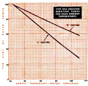
**DERATING.** If necessary to operate Type FRW Resistors in an ambient higher than  $25^{\circ}$  C., it is recommended that they be derated according to the Derating Curve for High Ambient Temperatures. For example, if the resistor is normally a 50-watt type and is to operate at  $60^{\circ}$  C. ambient, it should not be loaded to more than 82% of 50 watts, or 41 watts.
