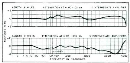
FIG. 5—Frequency characteristics for two video circuits of the type shown in Fig. 3
