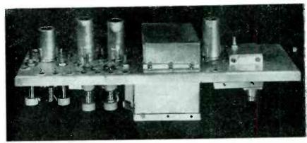
Side view, showing enclosed quarter-wave-line resonators at input and output of final stage
