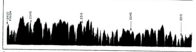
Example of strip chart obtained with sky-wave signal recording equipment at Strathburn, Ontario. Curve shows variation in input signal strength to receiver over period of several hours at night for signals of station WGY. Schenectady, N. Y.
