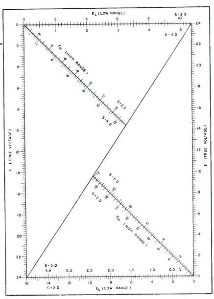
FIG. 2—Voltmeter loading nomograph. Take voltage readings on two ranges, divide higher range scale by lower to get S (either 2, 2.5, 4, or 5 on standard volt-ohm-milliammeters), then place straightedge on measured values ( $E_L$  and  $E_H$ ) for S scale in question and read true voltage on adjoining E scale. If range of any scale is inadequate, multiply all scale values by 10, 100, or any other convenient factor
