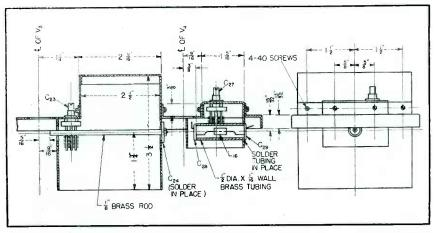
FIG. 4—Side view of chassis, showing constructional details of resonators operating at 232.5 and 465 mc
