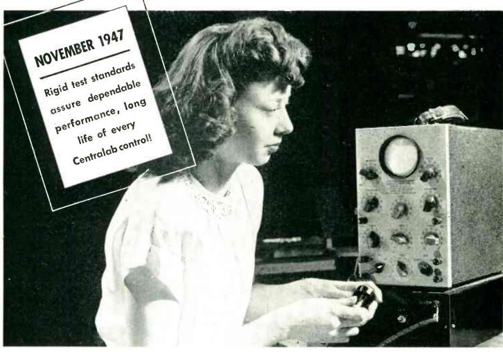
100% electrical test for continuity and "shorts" completes Centralab's program of tests for each control before it is shipped. This includes testing for resistance at various degrees of rotation, taper, noise, mechanical dimensions, etc. It's the
