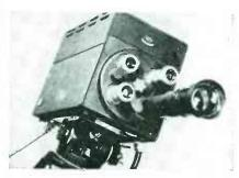
camera features a lens turret that takes up to four lenses of various focal lengths. Turret, diaphragm setting, and focusing are controlled from the rear of the camera. Hinged and removable panels make components and circuits immediately accessible. The electronic viewfinder avoids parallax difficulties.
