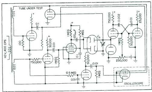
Circuit shows principal components of each stage
