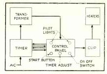
Block diagram of the electronically controlled permanent wave machine
