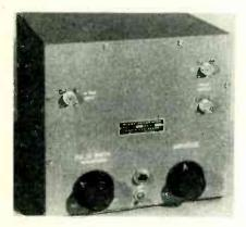
trigger of from 10 to 20 volts is required for each output pulse, the latter being variable in amplitude from minus 20 to plus 20 volts. The unit consumes 40 watts at 115 volts, 60 cycles.
