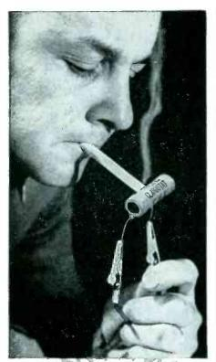
★ Here's a GREENOHM on 500% overload. It's hot enough to light a cigarette. Yet its special cold-setting inorganic cement coating doesn't soften, bubble or change. When cooled, it doesn't crack, peel, flake. Yes, GREENOHMS can take it. They're tough.
