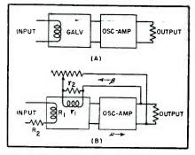
FIG 1—Basic principle of the electromechanical system is illustrated at (A). The method of adding feedback is shown at (B)
