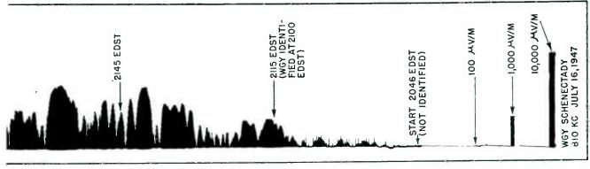
Analysis of above chart with photoelectric scanner showed that signal exceeded 6.100  $\mu$ v 5% of the time, 5.300  $\mu$ v 10%, 3.000  $\mu$ v 30%, 1.700  $\mu$ v 50%, 1.400  $\mu$ v 60%, 820  $\mu$ v 90%, and exceeded 700  $\mu$ v 95% of the time
