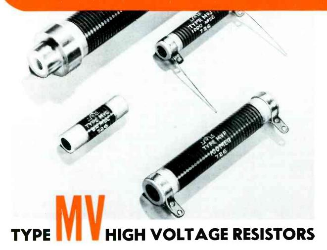
IRC Type MV Resistors are designed for high voltage applications where high resistance and power are required. Unique application of IRC's famous filament resistance coating in helical turns on a ceramic tube provides a conducting path of long effective length.
