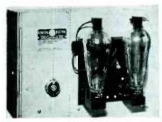
for use with ignitron contactors or nonsynchronous control combinations not having the heat control feature, when the power supply is 230 or 460 volts.
