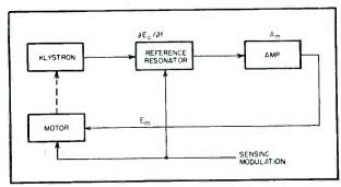
FIG. 3—A basic motor-operated automatic frequency control
