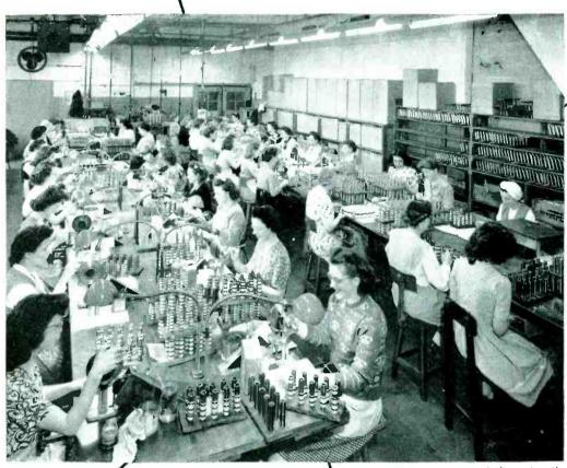
Skilled Operators winding voice coils, the heart of Magnavox dynamic speakers
