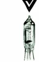
The VX series of subminiature vacuum tubes are especially adaptable to electrometer applications in fine instrumentation and for circuits used in radiation measurement. Feature 10 ma. filament current, grid resistance of 10<sup>15</sup> ohms. Unusually stable.
