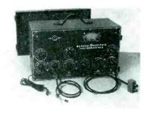
and a variable-frequency audio oscillator. Fundamental range of the r-f oscillator is 100 kc to 150 mc
