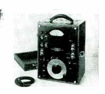
electrical and electroacoustic instrumentation is possible with the type 310-A Z-Angle Meter. Balance is accomplished by means of a single dial that reads directly in impedance and the phase angle is indicated on a direct-reading meter.
