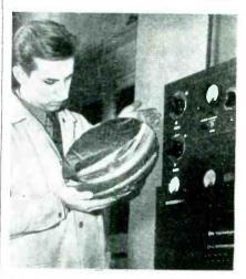
Spherical mirrors for projection television receivers are aluminized by evaproration in vacuum chambers
