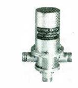
ing and remote control instrumentation. It has a minimum reflection loss up to 5,000 megacycles. The voltage standing wave ratio curve is almost flat from 500 to 4,000 megacycles. At 3,000 megacycles it is less than 1.2. Its characteristic impedance is 50 ohms, insertion
