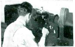
The mic-3-strue ure of nickel base material is checked constantly to insure selection of only the highest quality stock.
