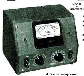
An extremely sensitive amplifier type instrument that serves simultaneously as a voltmeter and high gain amplifier.
