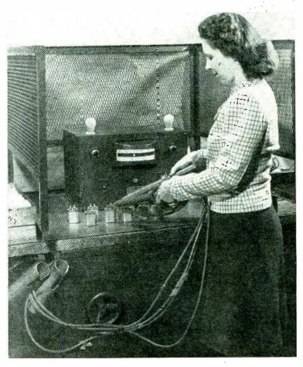
For voltage tests up to 5,000 volts, test prods handled by an operator can be safely used. Buttons on the handles of the prods control application and removal of test
