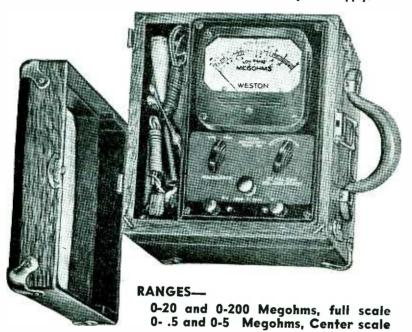
This unit was designed for the Navy to operate off eight  $67\frac{1}{2}$ volt batteries which provided a test potential of 350 to 500 Volts.
