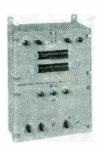
radio operator in maintaining a watch on the 500 kc calling frequency while he is busy or off duty. An ingenious relay system that can be set up to respond to assigned call letters or any other number or letter code is common to all equipments and can be reset to another combination in a few moments. Audible and visual alarms indicate the reception of a call.
