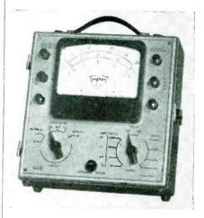
2,000, 4,000 at either 130 or 260 volts; four a-c current scales, 0 to 0.26 ampere at approximately 8 volts; 0 to 6.5 amperes at approximately 0.4 volts; 0 to 13 amperes at approximately 0.3 volt; 0 to 26 amperes at approximately 0.2 volt; two a-c/d-c volt scales, 0-130-260.
