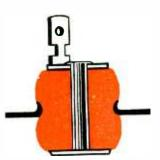
This bushing represents one of the newest uses for the recently developed G-E family of chemicals called silicones. Permanently elastic, formed to close tolerances, it seals itself by compression to the capacitor casing.
