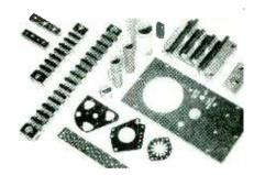
LAMICOID, a thermosetting laminated plastic insulation, made of paper or cloth fillers bonded with quality resins, has good dielectric strength. It is recommended for use as terminal blocks, switch and instrument panels, coil ends, tube socket bases, armature slot wedges and many other uses where a combination of dielectric strength and mechanical strength is needed.
