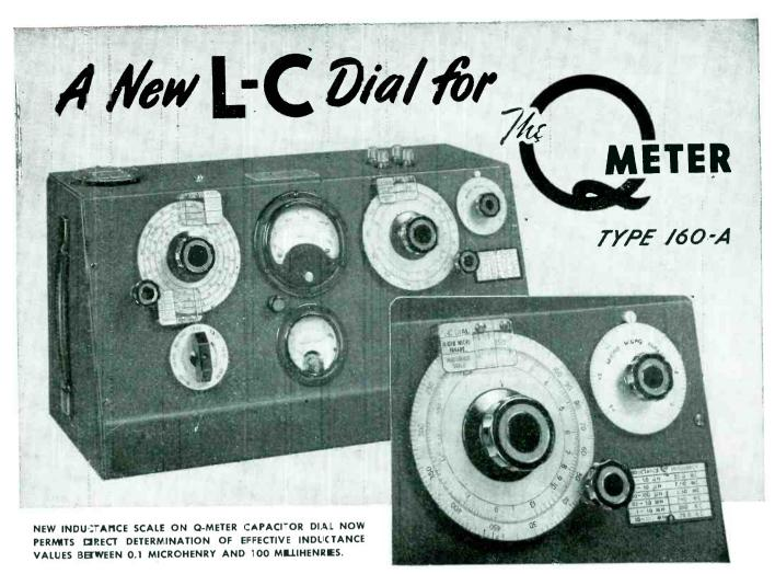
The 160-A Q-Meter is universally recognized as a rapid and simple means for measuring effective inductance. The customary method of measurement employed by engineers is to resonate the coil under test at a known frequency using a known capacitance, and thus obtain the effective inductance value of the coil by calculation. The use of the new L-C dial, as explained below, further increases the speed and versatility of the 160-A Q-Meter by eliminating the necessity for inductance calculations.
