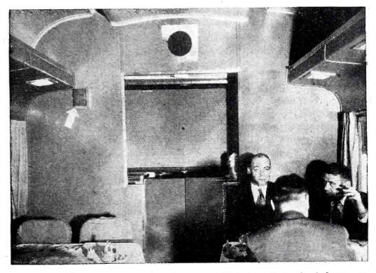
Remote control (arrow) and loudspeaker near ceiling in a Rock Island dining car
