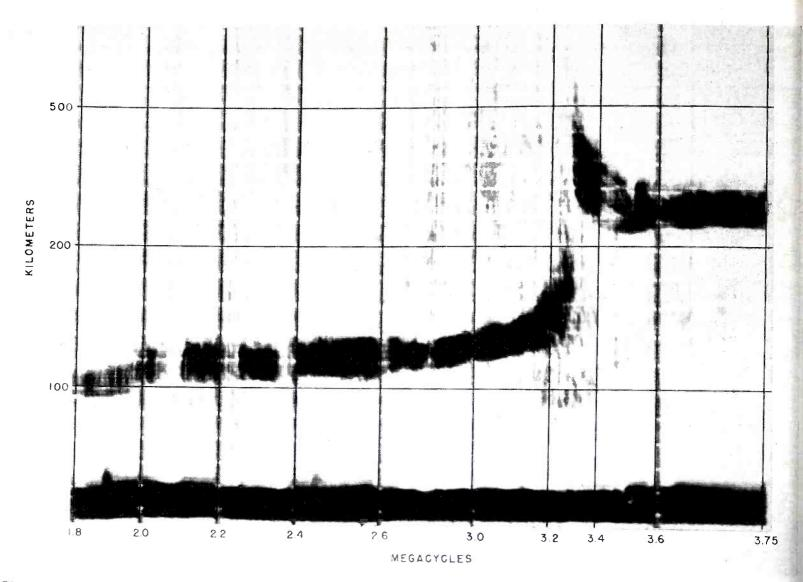
FIG. 7—Sweep-frequency record of November 24, 1946, at 1222 local mean time, showing the E-layer critical frequency at 3.3 megacycles (vertical incidence). This control data was taken the day after the eclipse
