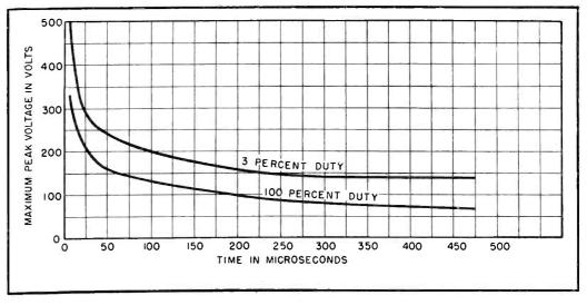
FIG. 10—Ignitor firing voltage as a function of linear buildup of voltage on ignitor of welding type ignitrons shows higher firing voltages at fast buildup
