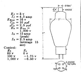
onds; deionization time 1 millisecond; mercury temperature 40 to 80 C.
