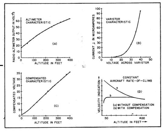
FIG. 2—(A) Nonlinear voltage output of radio altimeter. (B) Varistor characteristic. (C) Varistor-compensated altimeter characteristic. (D) Comparison of rate-of-climb indications of uncompensated and compensated altimeter
