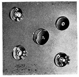
Integral Ceramic Construction: Each Couplate is an integral assembly of "HI-KAP" capacitors and resistors closely bonded to a steatite ceramic plate and mutually connected by means of metallic silver paths "printed" on the base plate. Think of what that means in terms of time and labor savings! Send for bulletin 943.
