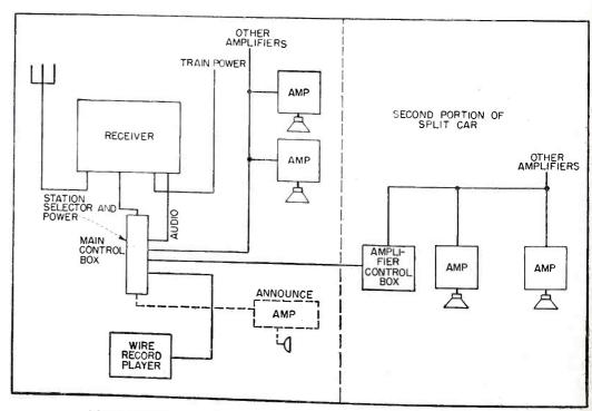
Block diagram of the equipment installed in one railroad car
