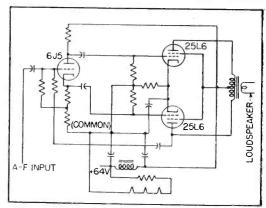
Circuit of a loudspeaker amplifier
