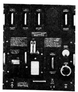
meter has been designed for use in the region between that served by the conventional 1,000-cycle bridge and the array of equipment usually employed at radio frequencies. In five decades it covers continuously the ranges of 1 microhenry to 100 millihenrys. The instrument can also be used for direct measurement of small capacitance up to 1,000 micromicrofarads, or for indirect measurement of larger capacitance. The equipment is rack mounted.
