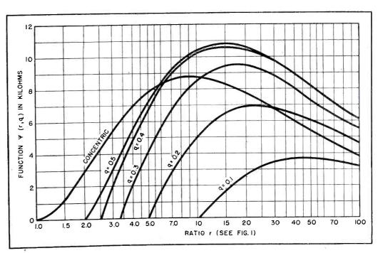
FIG. 5-Unloaded tank impedance cross-section parameter (see Eq. 7) is given as a function of the dimensionless ratios of line size
