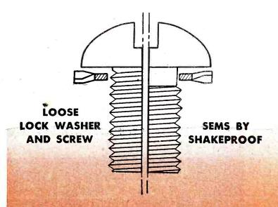
This combination cross section drawing illustrates the greater tooth engagement of sems by Shakeproof as compared with the tooth engagement of the washer which has been placed on a separate screw.
