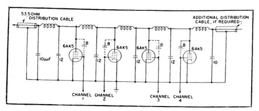
FIG. 7—Low-pass filter (cutoff 300 mc) used as a common load impedance for the final stages of channel amplifiers (four shown)
