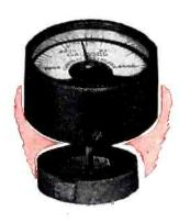
A tiny SILMANAL cylinder magnetized along a diameter is the heart of the G-E gauss meter. When the probe is placed in the field of a permanent magnet or a d-c electromagnet, the SILMANAL magnet on the shaft tends to line up with the flux. Flux density is measured by rotating the instrument until the pointer reaches its highest reading. This occurs when the probe-magnet flux is at right angles to the flux being investigated. The pointer when at zero scale position indicates flux direction.
