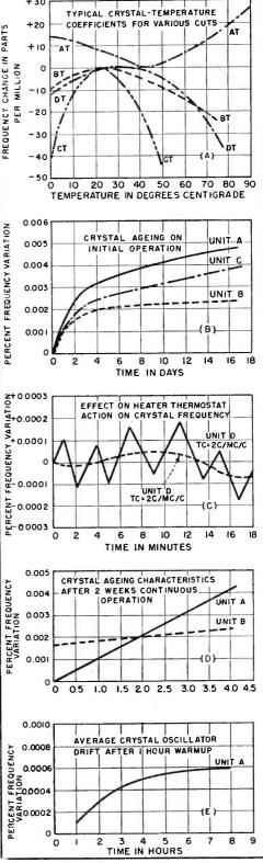
FIG. 1-Typical instabilities of crystals
