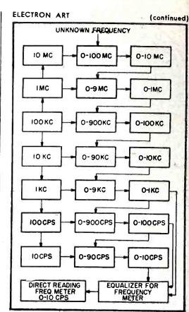
To the left is a chain of decade standard frequency generators. In the center are harmonic generators, each driven from its decade frequency. These generators feed mixer circuits that are simultaneously fed by the unknown frequency. To the right are low-pass filters passing only components of the unknown frequency lower than the decade being measured. In this manner each digit of the frequency can be determined
