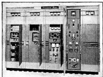
Grandard Radio Type D.S.10 5kW Transmitter—first of its kind to use air-blast cooling of valves. It has a frequency range of 2.5 to 25 Mc/s and operates on up to three C.W. channels with independent keying; or on two C.W. channels with common keying or one C.W. and one PHONE channel with simultaneous transmission on two different frequencies. The equipment is remarkably compact and is designed for tropical conditions.
