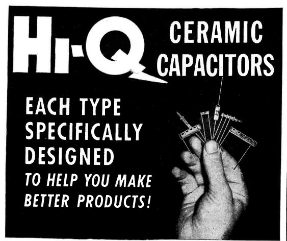
Hi-Q Ceramic Capacitors are manufactured of titanium dioxide (for temperature compensating types). Electrodes are of pure silver, precision coated. They are individually tested for accuracy of physical dimension, temperature coefficient, power factor and dielectric strength. Available in C. I. type (axial leads) and C. N. type (parallel leads) also S. I. type Durez coated for fullest protection against extremes of fungus and climatic conditions.
