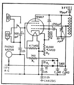
FIG. 1—Circuit of versatile phonograph oscillator using a selenium rectifier
