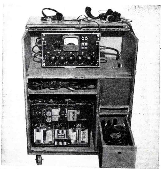
FIG. 1—Remote pickup equipment for scheduled broadcasts includes mixer-amplifier, telephone equipment, a-c and battery power supplies mounted in cabinet with spares
