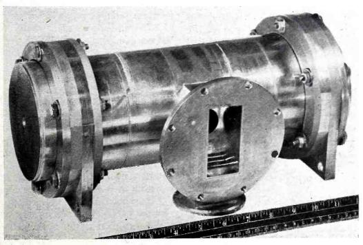
Six-section cavity, used for the linear acceleration of electrons at microwave frequencies in studies of nuclear physics (MIT)
