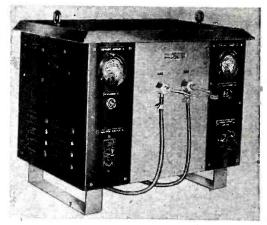
and one work coil which can be from ½ to 2½ inches in diameter; the unit will operate with a coil of one turn to a maximum of 20 turns. The price is \$650.
