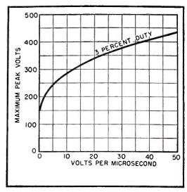
FIG. 12—Ignitor firing voltage versus rate of rise of applied voltage
