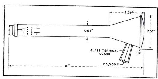
Extremely compact cathode-ray tube designed for projection television receivers. Maximum diameter of the tube is just a little over  $2\frac{1}{2}$  inches, but it is capable of projecting a 12 by 16-inch picture (Philips)
