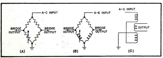
FIG. 1—Typical input circuits used with carrier-type amplifier
