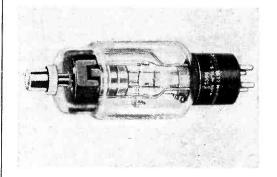
ambient temperature range of from -50 to +90 C. Maximum ratings: peak forward anode voltage, 2,500 v; peak inverse anode voltage, 5,000 v; average anode current, 0.5 amp; peak anode current, 2.0 amp; filament voltage, 2.5 v; filament current, 5.0 amp.
