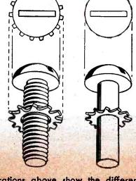
The illustrations above show the difference between hand assembly of separate washers and screws and the mechanical pre-assembly of sems by Shakeproof. Note the smaller internal diameter with the teeth pulled in beneath the screw head when the lock washer is placed on the screw blank before the thread is rolled. Also, note how the teeth of the hand-assembled combination protrude out from under the screw head.
