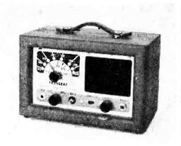
the receiver is operating from a-c or d-c. A built-in loop gives bearings within two degrees. The complete equipment weighs  $7\frac{1}{2}$  pounds.
