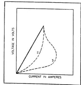
FIG. 2—Oscilloscopic traces of arc transfer show high currents for slow transfers
