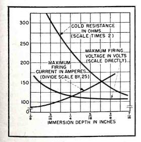
FIG. 9—Typical variation of ignitor characteristics with immersion of ignitor
