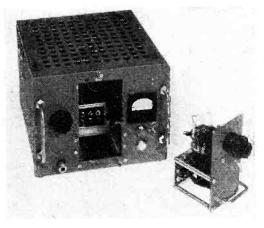
Oscillator with plug-in klystron unit
