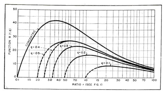
FIG. 6—Selectivity function (see Eq. 8) indicates optimum relative line dimensions for any application. If design is begun with this graph, optimum tank efficiency can be obtained
