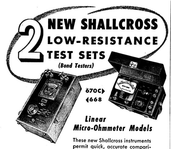
son tests of extremely low resistances between 2 and 800,000 micro-ohms. They are ideally suited for testing electrical bonds, heavy current switch and relay contacts, resistivity of heavy conductors or for making low resistance measurements. Both instruments utilize the 4-terminal method of measurement, thereby minimizing lead and contact resistance.
