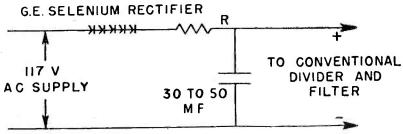
Typical diagram for radio receivers using the new G-E selenium rectifier. A ballast resistor "R" is usually provided to limit the output voltage of the rectifier to that required by the particular circuit. The value of "R" is usually between 25 and 50 ohms, but may be modified to meet any particular circuit requirements.
