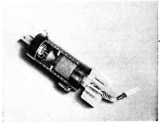
Cutaway of rectifier type ignitron
