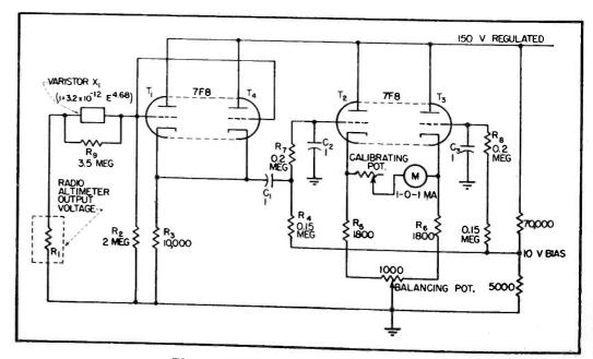
FIG. 1—Vertical velocity meter circuit
