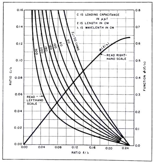
FIG. 3—Left hand scale gives ratio of loading capacitance to wavelength as a function for line length (see Fig. 2) for various characteristic impedances (see Fig. 4).
