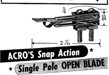
Here is the **Snap-Action** Open Blade switch that is in a class by itself. Its patented **Rolling Spring** construction is the basis of almost unlimited variations as to length and shape of actuators, movement and pressure. Terminals may be at side or rear.
