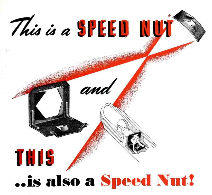
Take a look at this one SPEED NUT that does three jobs. Conceived by our development engineers to simplify automotive parking lamp assembly, it retains light socket, spaces wires and fastens entire assembly to the base. (See sketch). It replaced four separate parts and eliminated three machining and welding operations.
