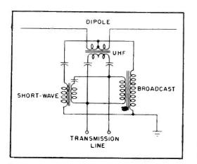
FIG. 3—Antenna coupling unit for nonamplifier system designed to abstract broadcast, shortwave and television signals from a single vhf dipole
