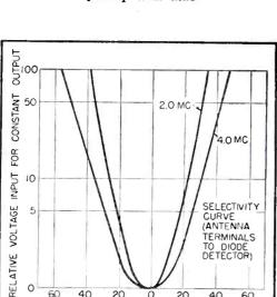
FIG. 2—Overall bandwidth of receiver
