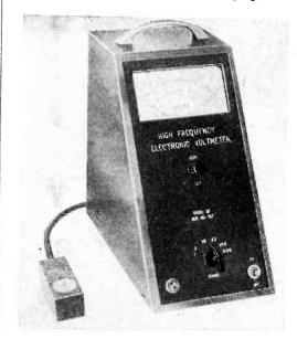
with an input capacitance of 0.75 micromicrofarad, making possible measurements up to 500 megacycles. It measures 0.3 to 300 volts r-f in five ranges. The instrument operates from 115 volts and weighs 8 pounds.
