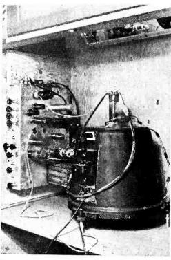
Housing of the optical elements of the Schmidt system and the projection tube in the receiver cabinet. Vertical and horizontal controls are on the chassis at left and additional power supplies are mounted on a shelf below
