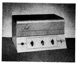
cycles and less than 3 percent harmonic distortion at maximum power. Hum is 60 db down. Two half-megohm inputs are provided. Output is tapped for 4, 8, 16, and 500 ohms impedance. Further information is given in Bulletin 134.
