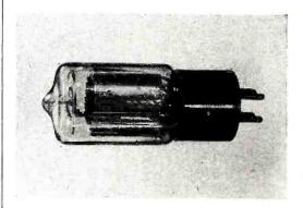
anode current, 1.0 amp; peak anode current, 8.0 amp; maximum peak inverse voltage 700 v; and filament voltage, 2.5 v. The tube has been designed for motor-control, servo-amplifier, high-speed counting and similar circuits.
