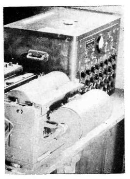
Amplifier bank alongside recording galvanometer
