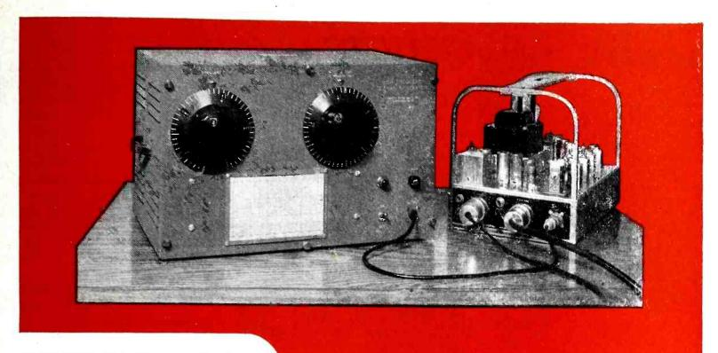
Model 196TS High Frequency Signal Generator being used to align a Harvey 152-162 Mc. Mobile Receiver.
