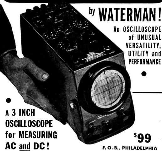
Amplifiers for vertical and horizontal deflection as well as intensity... Linear time sweep from 4-cycles to 50-kc with blanking of return trace... Sensitivity up to 100 mv/in... Fidelity up to 350-kc through amplifiers... Attenuators for AC and for DC... Push-pull amplifiers... Anti-astigmatic centering controls... Trace expansion for detail observations.
