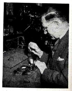
Principles of spectrophotometry are plied to fluorimetry in this instrument developed by Dr. T. E. Friedmann to identify vitamins by their emitted light
