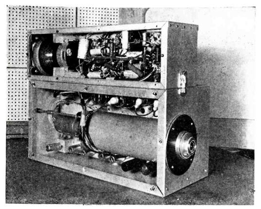
In the camera pickup unit, the image orthicon is shielded and mounted behind the lens. The five-inch electronic viewfinder faces the rear of the instrument and can be removed in its own cabinet if needed remote from the camera case
