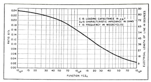
FIG. 2—Length of line relative to resonant wavelength is a function of the capacitance loading and characteristic impedance
