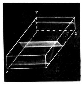
Three-dimensional cathode-ray tube portrayal of a sinusoidal wave traveling down a waveguide, with the lines simulating the waveguide formed by an auxiliary lantern-slide projector
