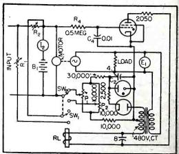
FIG. 3—Stabilized voltage source replaces the reference battery in the final circuit
