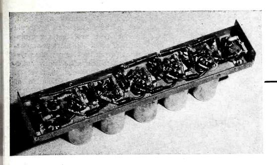
FIG. 2—Internal construction of channel amplifier shown in Fig. 1. Single-tuned staggered circuits are employed to secure flat response on each channel, high attenuation outside
