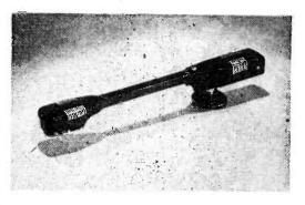
sional uses has a stylus pressure of 25 grams. Its overall design permits even the tracking of warped records with minimum distortion. The new instrument provides frequency response with distortion of only plus or minus 2 db from 30 to 10,000 cycles.
