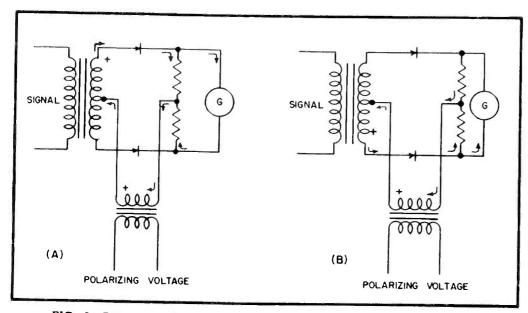
FIG. 2-Directions of current flow in bridge-type demodulating circuit
