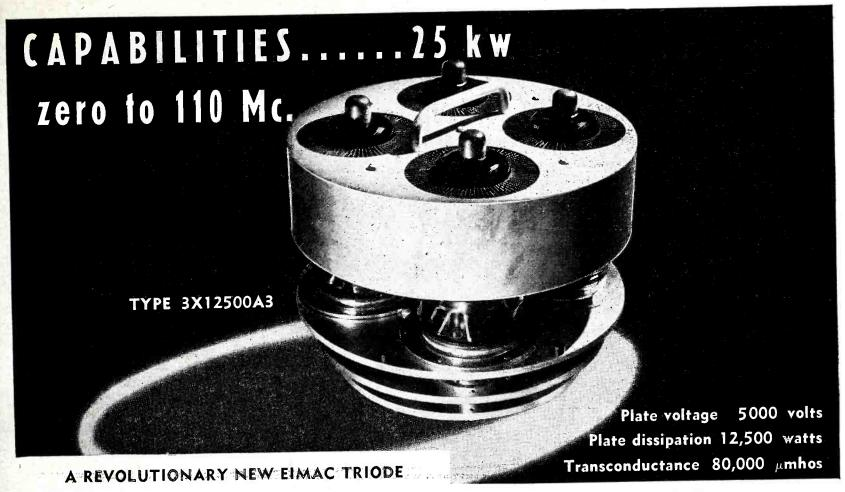
YES . . . The 3X12500A3 is truly revolutionary . . . packaged power . . . that will fill not several, but all applications for a power-amplifier or oscillator from zero to 110 Mc. It will do a low frequency job better than "special low frequency" tubes. It's performance at vhf has long been the aim of vacuum tube researchers. The 3X12500A3 is smaller (over-all 11"x9") and lighter (net 32 lbs.) than any comparable tube. . . Yes, it is truly a revolutionary tube.
