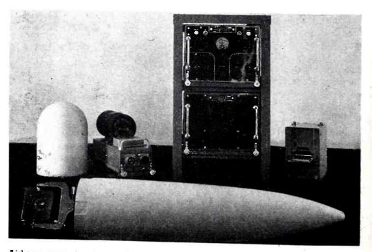
Airborne magnetometer used during the war to detect the presence of submarines beneath the surface of the sea, and now of wide interest to geologists (AIL)
