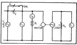
FIG. 1—Basic charging circuit in which a manually operated switch is used for illustration
