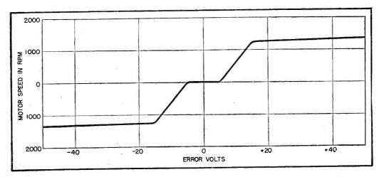
FIG. 6-Motor speed as a function of error voltage applied to d-c amplifier
