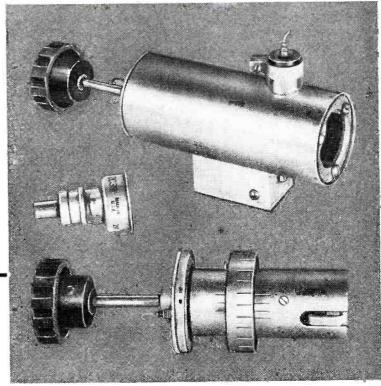
Complete 1,000-mc oscillator employing series-capacitance method of frequency stabilization (above), and view of cavity unit and 2C39 lighthouse tube used in it
