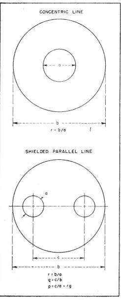
FIG. 1-(A) Size of concentric line is expressed by dimensionless ratio. (B) Size of shielded parallel line is expressed by two dimensionless ratios
