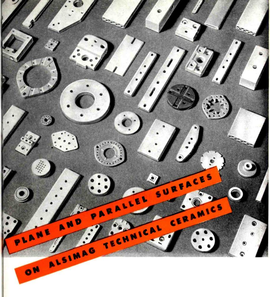
To obtain truly plane and parallel surfaces on AlSiMag ceramics, we at American Lava Corporation have equipped our grinding department with the latest grinding equipment, of the type used for the production of quartz crystals or optical flats. It is possible to supply ceramic plates ground flat and parallel within .0001".
