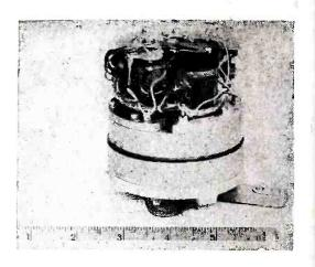
the torque arm. Back lash in the gear train is less than plus or minus a half of a degree. The servo unit can be made to traverse any angle less than 180 degrees, plus or minus two degrees. An automatic centering mechanism is also provided that centers the torque arm within the limits of plus or minus one degree. Length of the servo is four inches and the diameter is three and onefourth inches. It weighs 2.0 pounds.
