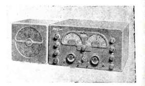
satisfy short-wave listeners, communications people including amateurs, as well as broadcast listeners who want versatile equipment. Voltage regulation stabilizes beatfrequency and crystal-filter operation. The receiver is equipped with noise limiter, signal-strength meter, low-and high-impedance audio output as well as a high-impedance input for phonograph pickup or other similar device. The price with speaker is \$189.50.
