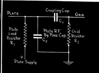
First commercial application of the "printed circuit", and now available for the first time, Centralab's new *Couplate* is a complete interstage coupling circuit which combines into one unit the plate load resistor, the grid resistor, the plate by-pass capacitor and the coupling capacitor.
