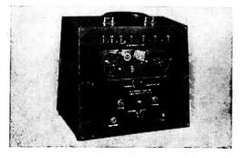
record continuously for one hour. Recordings may be edited by cutting out the unwanted wire with scissors, and tying the ends with a square knot. The knot will pass through the machine without perceptible noise.
