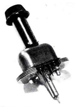
Magnetron suitable for use in high-power f-m and television transmitters (RCA)
