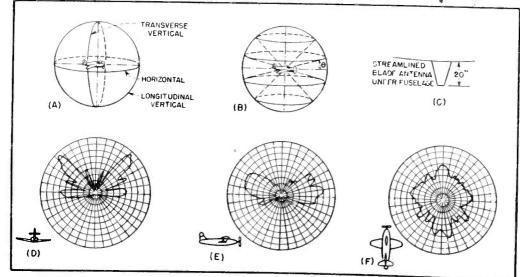
FIG. 2—Principal plane patterns are shown at (A), conical radiation pattern planes at (B), streamlined blade antenna used in tests at (C), and principal plane patterns for streamlined blade antenna at (D, E, and F)
