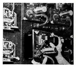
operation. Maintenance on the control unit can be effected after a spare unit has been inserted in its place.
