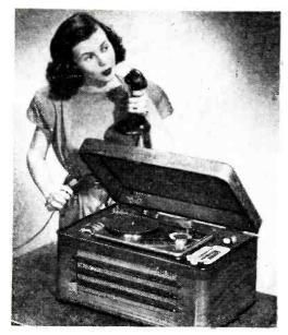
corder that uses a large drum driven by the turntable as a takeup reel. Recordings are stored on a  $3\frac{1}{2}$  inch spool of stainless steel wire capable of holding an hour's program. Selling price of the combination is \$169.50.
