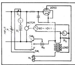
FIG. 2—Electronic charging control circuit with battery  $B_2$  supplying a reference voltage
