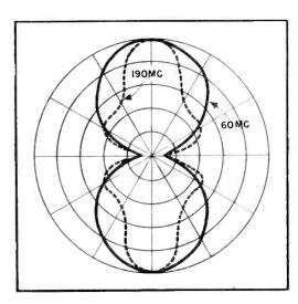
FIG. 6—Horizontal coverage diagrams of antenna shown in Fig. 5, taken at typical frequencies in the low and high frequency regions of the television band
