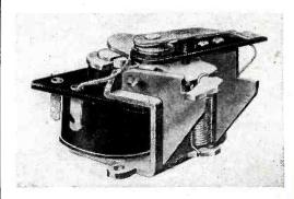
nated. External or remote mounting of the relay is permissible eliminating maintenance difficulties. Contacts are single-pole normallyclosed suitable for operation of a load as large as a 1 hp, 115 or 230 volt, 60 cycle capacitor motor.
