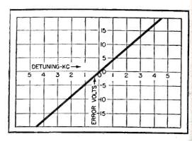
FIG. 4-Discriminator output characteristics with 100-microvolt signal at antenna
