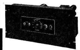
Calibrated self contained MARK-SPACE frequency measuring circuit.
