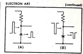
FIG. 1—Nonlinear compression circuits use crystal rectifiers
