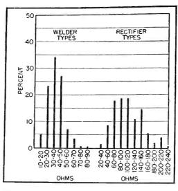
FIG. 7—Typical distribution of cold resistance of ignitors of ignitron tubes
