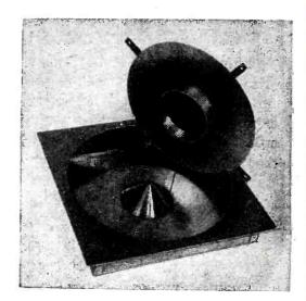
Annular-slot antenna designed to improve coverage from aircraft without introducing serious drag (AIL)
