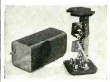
two bridges in cascade. Terminals are brought out so that either or both can be used. Only fixed mica capacitors and low temperature coefficient resistors are used, the whole assembly being sealed in polystyrene.
