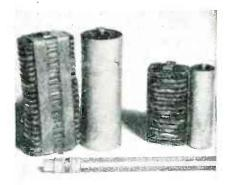
FIG. 6—Batteries for wearable equipment are available in a variety of types and sizes. Shown here are two pairs of A- and B-Batteries with their paper covers removed; both pairs give the same voltage
