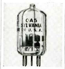
to fire the tube when the anode rests at 750 volts. The new tube has been designed for use in electronic photoflash and similar equipment.
