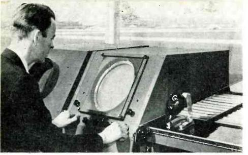
Experimental search radar installation at CAA control tower in Indianapolis. PICAO encourages further development, to solve such problems as obtaining a sufficiently bright ppi presentation for reliable observation in a brightly illuminated control tower
