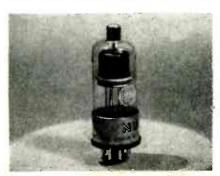
regulation of low-current power supply voltages up to 8 kilovolts, such as in pulse amplifiers, for high-impedance measurements, and in television equipment.
