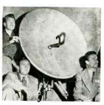
Waveguide and reflector of RCA microwave radio relay transmitter, set up near ring of Mexico City's 60,000-seat bullring for beaming first televised bullfights to a hotel six miles away
