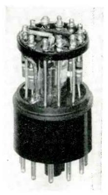
FIG. 5—Calibrated pre-assemblies are used to obtain stable circuits, by balancing drifts in the components against each other, in this multivibrator
