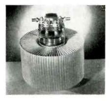
use in grounded-plate, grounded-grid, or grounded-cathode circuits. Design features include a thoriated tungsten filament, low-inductance and high-conductivity leads.
