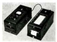
Brush Single-Channel Magnetic Oscillograph with amplifier. Especially suited for strain-gauge applications, counting, surface analysis and similar applications. Three-speed paper drive, 5, 25, 125 mm per second. Chart paper 23%" wide.
