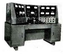
electronically regulated power channels, bridge signal source, amplifier, meters, and other accessories conveniently located for tube tests and maintenance. The console is 55 inches high, 70 inches long, and 34 inches deep. It weighs 1,500 pounds.
