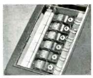
Brush Six-Channel Magnetic Oscillograph. Excellent for strain-gauge recordings. Dust-proof case. Interchangeable gear paper drive. Your choice of paper speeds from ½6" to 5" per second. Chart paper 12" wide. Compact design.
