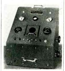
personnel. Tests at peak voltages between 1,000 and 21,000 volts can be rapidly determined. The instrument can be modified for testing high tension cable or for other resistance, corona and breakdown testing. The unit measures 20x20x22 inches.
