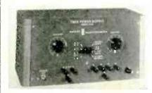
model 210 features two independent adjustable output voltages that remain constant regardless of variations in the power line and load connected to each output. A selector switch allows connection of the supplies in series or parallel. An unregulated output of 6.3 volts is also available.
