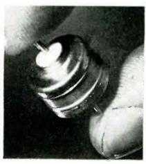
diameter and is less than 1½ inches long. Frequency coincides with that assigned by the FCC for this service and the unit is completely enclosed with soldering terminals provided for quick connection to the circuit.
