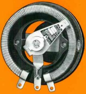
Rheostat windings are sometimes tapered—that is, wound in two or more sections of diminishing wire sizes. This can be done because only the first turn of a rheostat carries the maximum current. Succeeding turns carry only a fraction of the maximum current. Thus, they can be of smaller wire size, permitting the use of a smaller rheostat—or a winding of higher resistance for a given size rheostat. Ohmite will design special tapered windings to suit indi-
