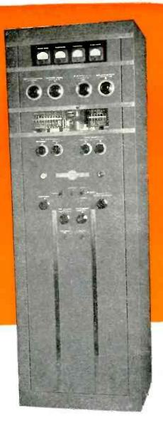
The new Collins 30K-2 embodies certain design features that are of ourstanding benefit to owners who employ radio communication from point to point, ground to plane, or shore to ship. This 250 watt radio transmitter can be pretuned to any two frequencies between 2.0 mc and 30.0 mc. Relay operation of all r-f circuits, including antenna tuning, provides instantaneous frequency shift.
