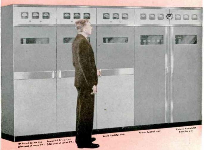
STRAIGHT-LINE Arrangement (pver-all width 208 inches). Unit-construction permits flexible station layout, advantageous use of available floor space.
