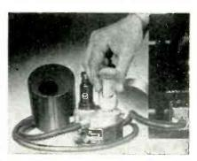
of radioactive materials and cosmic radiation. A loudspeaker is provided for the former and either a meter or an ink recorder can be used to count rates from 5 to 20,000 a minute.
