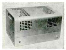
booster amplifiers, types G050 and G0125, capable of delivering 50 and 125 watts respectively use multistage inverse feedback to attain a flat response within 1 db from 20 to 20,000 cycles. Input impedance is 500,000 ohms with provision for balanced-line zero-level input for use on telephone lines. The self-contained power pack provides a regulated screen supply.
