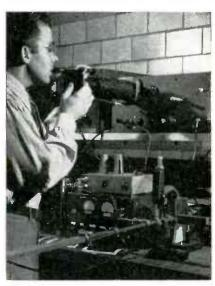
FIG. 2—Photographing microwave absorption bands as displayed on cathoderay tube
