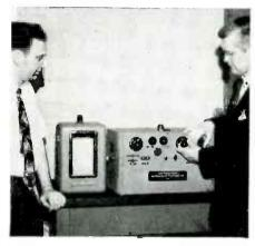
FIG. 2-Professor Klotz (left) and Professor Dole of Northwestern demonstrate the ultraviolet photometer developed by them for gas analysis
