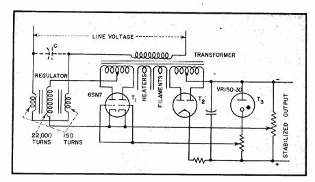
FIG. 8—Power-supply stabilizer, to regulate both filament and heater as well as high-voltage supply, uses controlled saturable reactor in power input circuit
