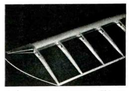
There are 15 P-K Self-tapping Type "Z" Screws in each wing structure, fastening spar, ribs, leading edge and tip securely together.
