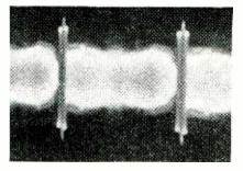
FIG. 5—One frame of a typical television signal as seen on the screen of the modified test oscilloscope
