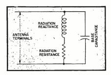
FIG. 4—Equivalent circuit of antenna as seen from its input
