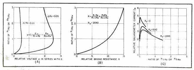
FIG. 2—Curves used in determining optimum values of circuit parameters for stable high-sensitivity vacuum-tube voltmeter
