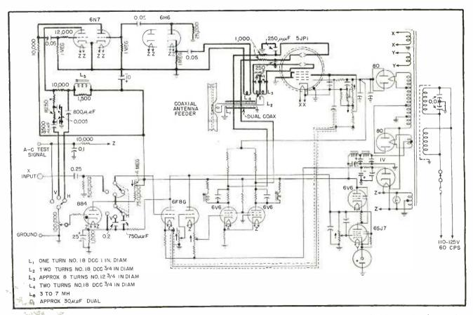
FIG. 1—Circuit modifications, shown in heavy lines, adapt standard oscilloscope for operation at television carrier frequencies
