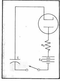
FIG. 6—An equivalent magnetron pulsing circuit containing a storage capacitor
