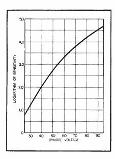
FIG. 2—(left) Were the transfer characteristic of the circuit of Fig. 1 ideally logarithmic, this response function would be a straight line
