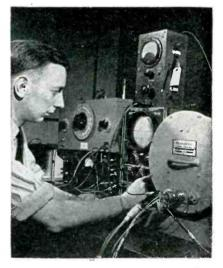
Signals from hydrophones on the hull of the target ship, increased by the Westinghouse preamplifier at the right, are transmitted by radio to a recorder miles away from Operation Crossroad. High-speed cameras in the recorder make a permanent record of pressure fluctuations
