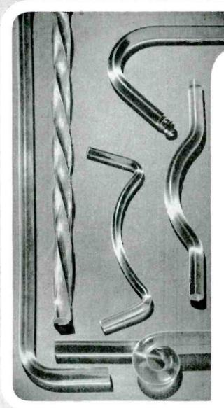
Plax crystal polished polystyrene rod can be heat formed without difficulty into many shapes and intricate bends. Correct forming techniques should be closely observed.
