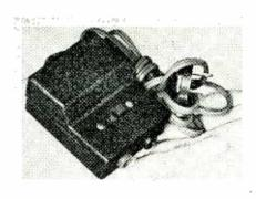
volt a-c or d-c line, a neon lamp, series resistor and switch, and a pair of leads. It is conveniently packaged for continuity testing and sells for about \$5.
