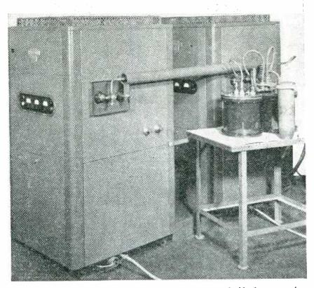
Side view of two heaters connected by a coaxial line to give double the power of a single unit in the common work coil. The two r-f transformers that feed the work coil rest on the table at the right
