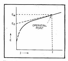
FIG. 5-Load characteristics of d-c anode circuit of magnetron can be simulated by battery and resistor
