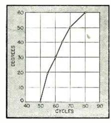
FIG. 6—Operation in the frequency range from 50 to 80 cycles provides 60 degrees of rotation of the inductance shaft
