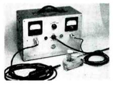
indicated by the thermocouple, whereas the tube is connected after diffusion pump has been started. A feature of this tube is its cold cathode. There is no filament to burn out with accidental increase of air pressure. The tube is also enclosed in an oval metal shell surrounded by a strong magnetic field. The anode consists of a rectangular loop of wire embracing the maximum position of the
