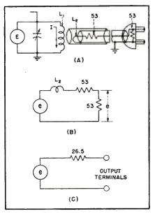
FIG. 10. Circuit (A) is the output system in which the D-shaped coil  $L_1$  is used. The equivalent circuit of the attenuator is shown at (B) and the equivalent circuit of the signal generator at (C)
