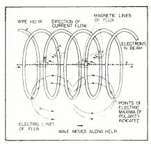
FIG. 3—Field diagram shows orientation of electric and magnetic lines of flux in relation to helix and electron beam. Coupling is only through electric field
