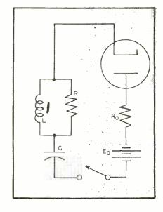
FIG. 2—Ä biased diode can be a part of the load through which constant current is passed
