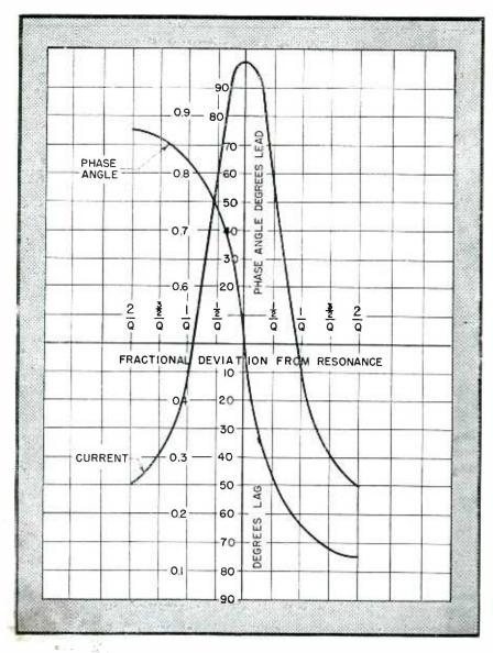
FIG. 1—Near resonance, the phase angle changes rapidly. Advantage of this characteristic is taken in design of the control system
