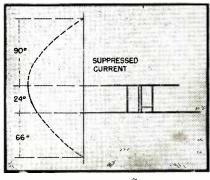
FIG. 3—Vertical distribution of antenna current
