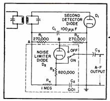
FIG. 1—Simple series limiter, requiring only the four additional components inside the dash-dash rectangle
