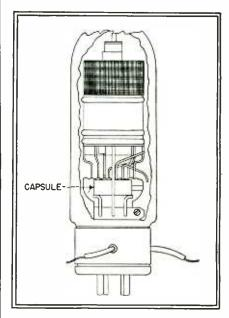
With a hydrogen generating capsule located inside 5C22 thyratrons, greater life and higher pulse rates were possible
