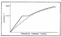
Drying curves for dielectric heating of foundry cores show that same ultimate temperature is reached by second pass through heating unit. Knee in solid curve is produced by moisture in initial core. Dashed curve is that of subsequent pass
