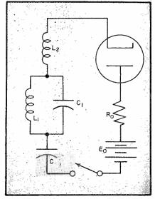
FIG. 8—A corrective network can be made entirely of reactive elements
