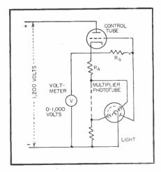
FIG. 1—Basic feedback circuit for producing logarithmic relation between light intensity and dynode voltage of multiplier phototube
