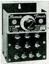
in pairs or combinations they can control a number of operations in a predetermined sequence with either self or manual recycling. Five timing periods, depending upon the value of fixed capacitor plugged into the circuit, are available from ½ to 60 seconds. The unit can also be modified for use as a sensitive control relay.
