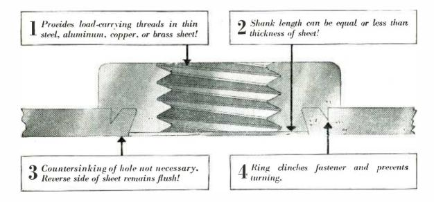
PEM Self-Clinching Fasteners solve assembly problems involving steel, aluminum, copper, or brass sheet. Because no special tools are required, PEM Self-Clinching
