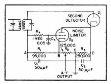
FIG. 10-Triode shunt-type noise limiter
