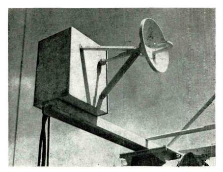
K-band (one centimeter) dish for monitoring APS-34 radar transmissions through blast cloud. Note curved waveguide feed
