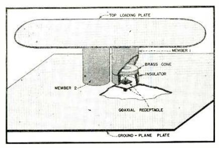
FIG. 1-Cutaway shows method of feeding antenna
