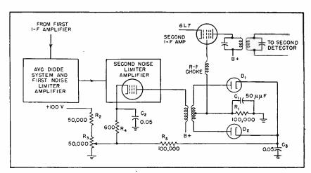
FIG. 13—Degenerative noise limiter, acting between first and second i-f stages
