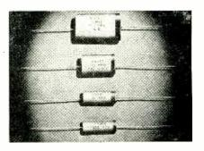
with Kraft paper and impregnated. Leads are securely anchored and the end-fill compound is not melted by a hot soldering iron. Capacitance values range from 0.001 to 0.1 microfarad in d-c rated voltages from 150 to 600 volts.
