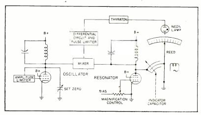
Fig. 1—Essential stages of the reactance comparator. Within its useful range, inductance can be checked against a standard with an accuracy better than one percent, and capacitance within 0.1 percent
