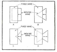
Fig. 2—Different vane shapes determine whether the scale of the special indicator capacitor is linear in frequency and capacitance or exponential
