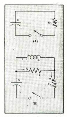
FIG. 1—(A) Exponential circuit, and (B) compensated circuit from which constant current can be obtained
