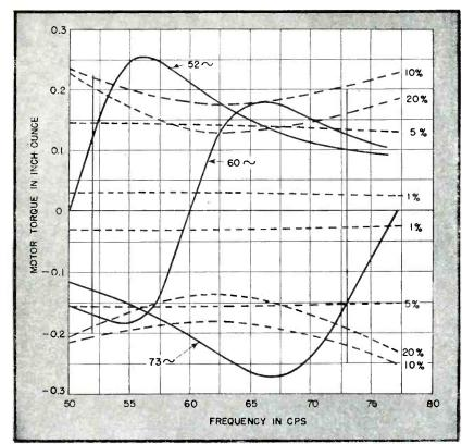
FIG. 8—Torque response curves of the control when set for resonance at frequencies of 52, 60, and 73 cycles. The solid lines indicate the resonant frequency constant; the dashed lines show the constant deviation in percent
