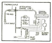
Complete circuit of the wattmeter for use from 20 to 1.500 megacycles
