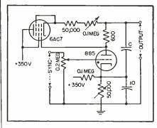
FIG. 3-Complete circuit of laboratory sweep generator whose output is linear
