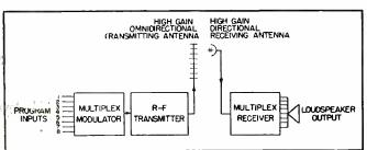
FIG. 1—Basic portions of Federal's pulse time modulation system. Use of the omnidirectional transmitting antenna permits broadcasting services
