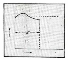
FIG. 7—Percent deviation from a constant level over a given time can be reduced by adjusting the corrective network
