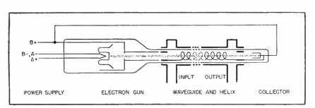
FIG. 2—Pictorial circuit shows how helix is coupled to waveguide at input and output ends. Guide extension along helix serves only as electrostatic shield
