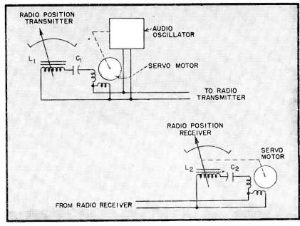
FIG. 9—Essential units of the receiver and transmitter of the radio control system
