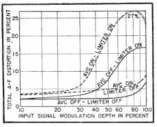
FIG. 3—Modulation distortion curves as measured at output of typical communications receiver using simple series limiter. The avc-off curves are substantially the same as for weak-signal avc-on operation. Signal input frequency is 4,000 kc, a-f output frequency is 1,000 cycles, and signal input level is 1,000 microvolis
