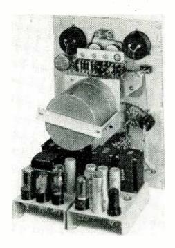
Front and rear views of the signal generator. Frequency deviation and percent of amplitude modulation are controlled by two potentioneters below the modulation meter switch. On the tuning dial, the vernier scale changes the frequency by about 26 kc on the low-frequency range and 52 kc on the high range. Choice of modulating frequency is provided by the dial at lower left and output from 0.0000001 to 0.2 volt is controlled by the attenuator dial at lower right
