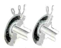
During manufacture, the resistance may be varied over its length to provide any resistance-rotation curve. After molding, heat, cold, moisture, or hard use cannot affect it.
