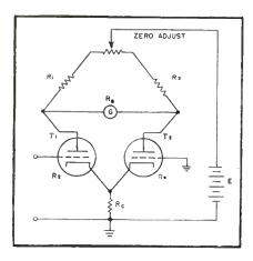
FIG. 1—Basic bridge-type vacuum-tube voltmeter circuit used with radiation pyrometer for flame radiation measurements
