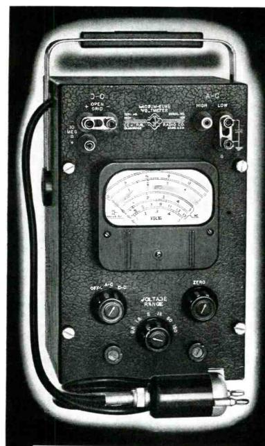
THE Type 1800-A vacuum-Tube Voltmeter is a new instrument based on the fundamental designs of the Type 726-A, introduced by G-R in 1927. With greater sensitivity, increased ranges improved probe construction, both dec and a-c voltage calibrations, and housed in a much more compact and convenient-tz-use cabinet, the useful upper-frequency limit of this meter is extended just about as far as present-day vacuum-tube construction will permit.
