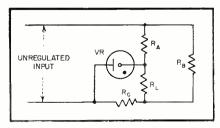
FIG. 6—Improved gaseous tube stabilizer circuit makes voltage across load resistance independent of input over α wide voltage range
