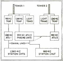
Fig. 1—Two transmitters on different frequencies feed one antenna system
