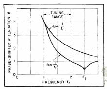
FIG. 7. Attenuation  $B \ a \ 1/t_r$  produced by conventional two-element inductive reactance-tube phase shifter and arrenuation  $B \ a \ 1/t_r^2$  required by an inductive reactance tube for constant deviation of a capacitance-tuned circuit
