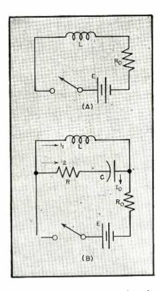
FIG. 4—(A) An inductor can replace the capacitor of Fig. 3. Corrective network (B) contains inductance
