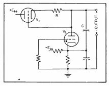
FIG. 1—Basic circuit of relaxation sweep generator to which current feedback has been added to improve the linearity
