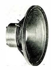
other in the line of dual speakers designed for good fidelity in home reception and reproduction. This model has a power rating of 18 watts and a 3-inch voice coil with an impedance of 10 ohms. Weight of the unit is 12 pounds.
