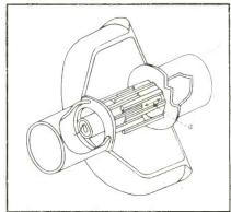
FIG. 1—Squirrel-cage magnetron is tuned by varying the distance by which the two sets of interleaved bars overlap each other
