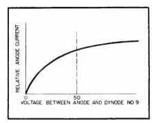
FIG. 5—Voltage versus current relationship of anode of multiplier phototube for constant dynode voltage and constant incident illumination
