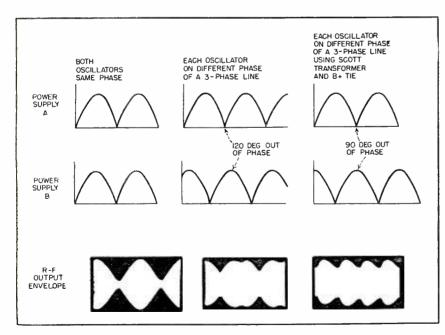
FIG. 3—Waveforms encountered in the output envelope when the heating units are connected in various ways to power lines. Double power can not be obtained from the two units unless the power input phasing is correct
