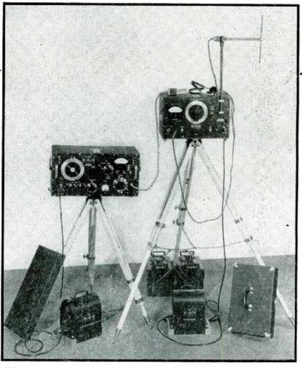
FIG. 1—Field-strength meter and standard-signal generator developed for National Defense Research Committee by General Radio Co. to be used for measurements between 300 and 1.000 mc
