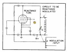
FIG. 2. Constant deviation is obtained by ganging a modulation input potentiometer with the tuning capacitor
