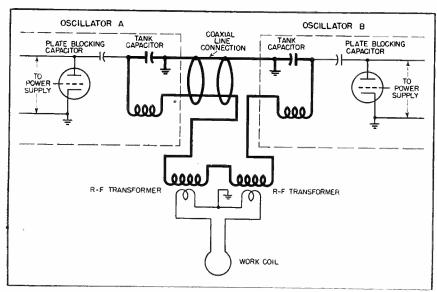
FIG. 2—Two oscillator r-f transformers and work coils can be wired in series for double power. A coaxial connection is necessary, besides other ground bonds, to maintain a low reactance between units and ground
