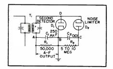
FIG. 9-Balancing-type noise limiter
