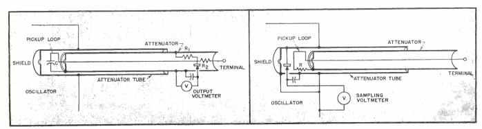
FIG. 6—Output meter of standard-signal generator can be located at output of attenuator
