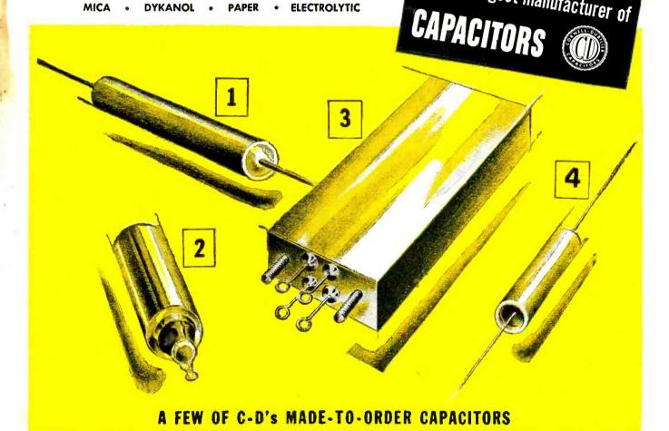
CAPACITOR #1. Here is a capacitor designed specifically for automobile horn spark suppression. Fits into horn housing with minimum of assembly operations. Leads firmly, mechanically anchored to stand extreme vibration.
