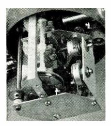
FIG. 9. Mechanical details of the r-f assembly. The arrow indicates the slotted stator of C1
