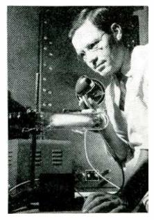
Norman C. Beese, research engineer at Westinghouse Lamp Division, demonstrates the caesium vapor lamp he designed for talking over an invisible infrared light beam
