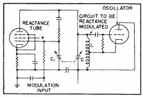
FIG. 3. Method of obtaining constant deviation by ganging an element of the phase shifter with the tuning capacitor
