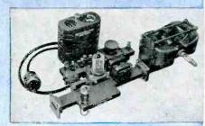
RF Radar Assembly DB-412
