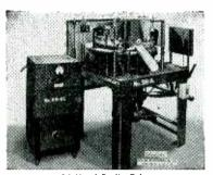
24 Head Radio Tube Exhausting Machine.
