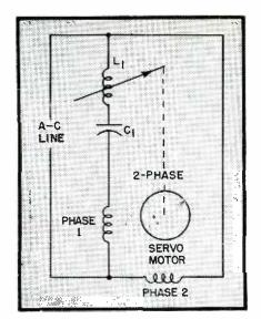
FIG. 3—Coupling the serve motor to  $L_1$  provides automatic tuning of the motor circuit to the line frequency
