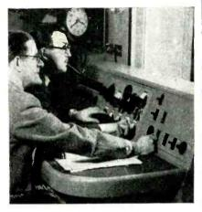
A program engineer and a producer at a new B.B.C. control console. The panel at the right is for use by the producer, the center and left-hand panels contain more technical controls
