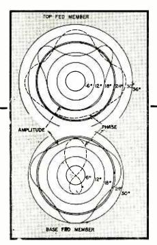
FIG. 2—Current distribution at base of antenna radiators
