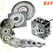
Featuring extremely low and uniform contact resistance and low noise level. Daven switches are supplied in varied combinations of decks, poles per deck and contacts per deck. Heavy duty, laminated, self-wiping arms need no lubrication; switch contacts and arms are of a special silver alloy lother metals to your specifications); bakelite or ceramic panels; breakbefore-make or make-before-break witring.
