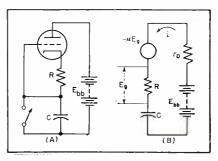
FIG. 2—(A) Simplified circuit of linear sweep generator (B) equivalent circuit of generator
