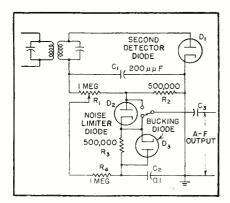
FIG. 4—Series-type noise limiter with threshold adjustment so that limiter operation can be set to start anywhere in range from 0 to 65 percent modulation
