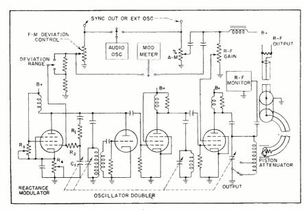
FIG. 8. Simplified diagram of the f-m signal generator
