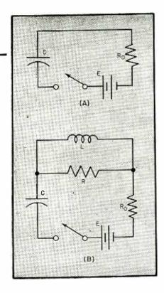
FIG. 3—Instead of discharging a capacitor, as in Fig. 1, the capacitor can be charged in the manner shown here
