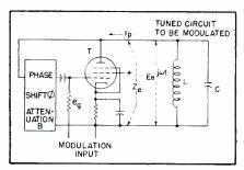
FIG. 4. Fundamental reactance-tube circuit
