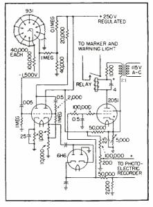
A multiplier phototube replaces the usual film for high-speed automatic inspection of parts for internal defects. The thyratron operates a marker and warning light
