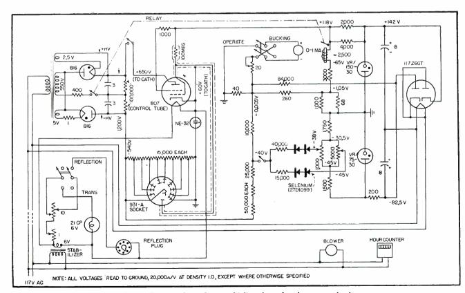
FIG. 4—Complete logarithmic multiplier phototube photometer circuit
