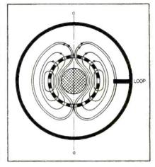
FIG. 2—Because the magnetic field links the squirrel cage, the size of the tube shell cavity does not appreciably affect the resonant frequency
