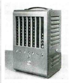
Neon-lit figures on the panel of the time interval counter can show b velocities and accelerations for intervals up to one second in steps of one millionth of a second
