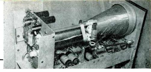
FIG. 2—High-frequency line terminating loop can be seen coupled to tuning coil of vertical deflection circuit in the converted oscilloscope
