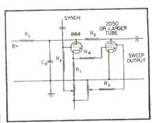
Sawtooth oscillator circuit combining advantages of 884 and 2050 to obtain rapid return trace of beam in c-r tube
