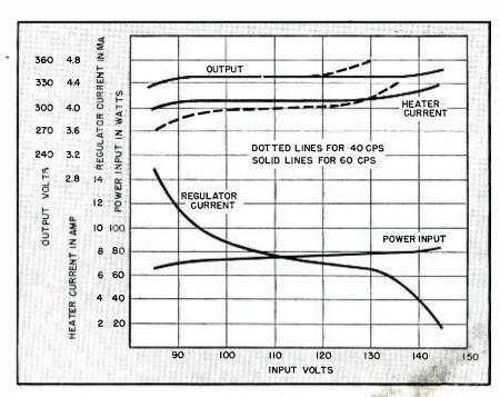
FIG. 10—Measured characteristics of power supply show the wide range over which the stabilizer operates
