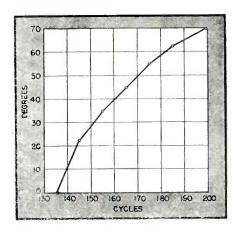
FIG. 7—Seventy degrees of rotary motion were obtained by using frequencies between 135 and 198 cycles
