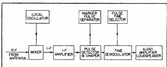
FIG. 2—In the receiver, pulses are separated and sorted to provide eight 9,000-cycle audio channels and/or audio, facsimile, and telegraph services
