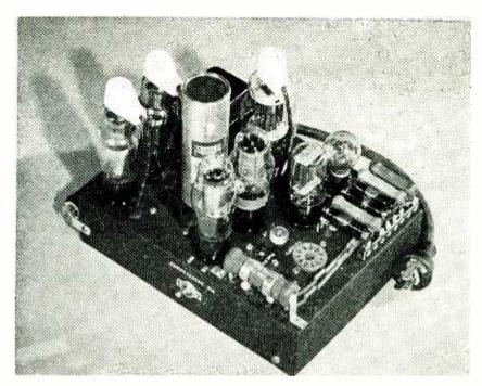
FIG. 7—Assembled power supply and control circuit of photometer
