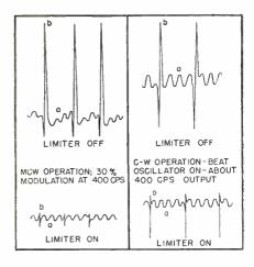
FIG. 2—Oscilloscope tracings of audio output of receiver, illustrating noise suppression of simple series limiter. Signal input to receiver is 80 microvolts, and avc is off
