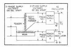
FIG. 4—Single-phase type units can be connected to a three-phase line through a Scott transformer. When the outputs of the power supplies are paralleled, the heating units give optimum power and the power line is also balanced
