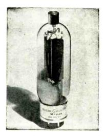
tube as a class A amplifier are: d-c plate, 1,500 volts; peak a-f grid, 150 volts; power output, 55 watts.
