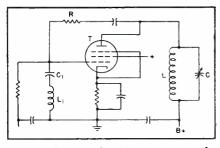
FIG. 5. Constant-deviation reactance-tube circuit. Phase shifter R,  $C_1$ , and  $L_1$  produces an attenuation inversely proportional to the square of the frequency over the tuning range
