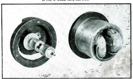
quently no brushes or slip rings to wear and deteriorate. The inductance variation is linear for a little more than sixty degrees rotation of the shaft.
