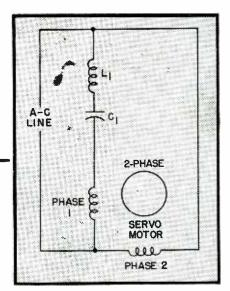
FIG. 2—The reasonant circuit formed by  $L_1$  and  $C_1$  controls the current flowing through the motor winding of phase 1
