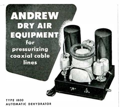
A compact, completely automatic unit that pressurizes coaxial transmission lines with clean, dry air. Starts and stops itself. Maintains steady pressure of 15 pounds. A motor driven air compressor feeds air through one of two cylinders containing a chemical drying agent where it gives up all moisture and emerges absolutely clean and dry. Weighs 40 pounds; 14 inches wide, 14 inches high, 11 inches deep. Power consumption, 210 watts, 320 watts during reactivation.
