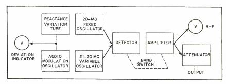
FIG. 1. Essential stages of f-m signal generator employing the heterodyne system
