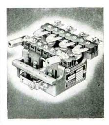
feature of the contact mechanism eliminates pigtail connections. Coils can be supplied to operate at voltages up to 230 volts, a-c or d-c. Typical power consumption of the coils is less than 3.5 watts on d-c, 8 watts on a-c.
