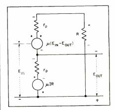
FIG. 2—Equivalent circuit of the low output impedance cathode follower
