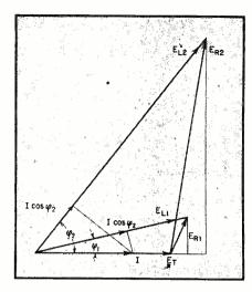
FIG. 9—Vector diagram shows that reactor absorbs the change in input voltage
