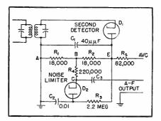
FIG. 12-Modified shunt noise limiter
