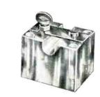
Measuring 13/4" x 21/2" x 17/8", this acrylic stand-off insulator holds vertical whip antennas erect in marine radio installations. A brass strip with wing nut swings open to permit easy removal for lowbridge underpassing. This is another typical example of Printloid's ingenuity with plastics.
