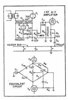
FIG. 6—Hum-reduction version of simple series limiter, with equivalent circuit arranged to show bridge configuration
