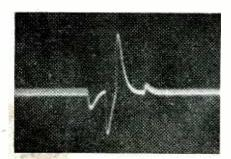
FIG. 4—Horizontal synchronizing pulse taken from L<sub>5</sub> through the H position of selector switch
