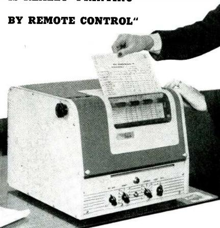
Finch Telefax equipment transmits and records—by radio or telephone—exact facsimiles of written or printed messages, as well as drawings, photographs, signatures, typewriting, etc. Finch Telefax is really "printing by remote control." It is the fastest known and most accurate system of communication.
