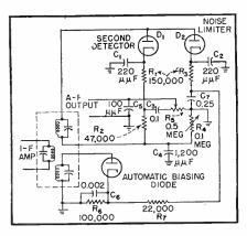
FIG. 8—Automatic balanced-detector noise limiter
