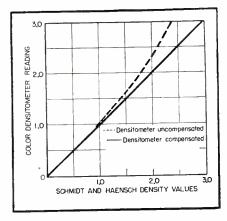
FIG. 9—Measured accuracy of color densitometer indicates improvement made by meter compensating circuit
