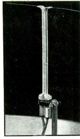
FIG. 5—Doublet antenna can be quickly tuned by sliding flexible tapes in two-wire transmission-line track
