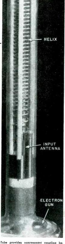
Tube provides nonresonant coupling between electron beam and traveling wave
