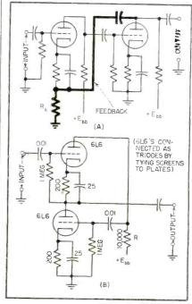
FIG. 1—By rearranging a two stage feedback amplifier (A) the plate resistance of the second tube can serve as the cathode resistor in the stage of the first tube (B)
