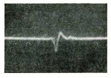
FIG. 3—Integrated vertical synchronizing pulse fed to the type 884 tube
