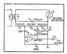
FIG. 5—Low-loss series limiter, requiring three more components than the simplest version in Fig. 1
