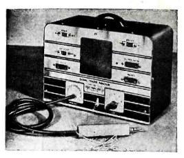
with a Bakelite probe which picks up the signal, the main unit converts the resultant signal into an audible tone or a vacuum-tube meter reading. Loudspeaker or phones can be employed. Complete with batteries the unit weighs  $10\frac{1}{2}$  x 6 inches.
