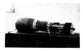
display of four separate signal indications on a five-inch screen. Deflection plates are brought out to sixteen separate terminals. A twenty-seven-pin special base is used. The screen can be supplied in various types of phosphors. Overall length of the tube is 181 inches.
