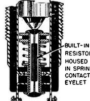
RESISTOR HOUSED IN SPRING CONTACT EYELET
