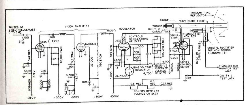
FIG. 6—After additional amplification, the multiplex position-modulated pulses amplitude modulate the reflex Klystron
