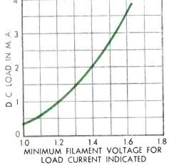
Note: Curves indicate that in a television receiver rectifier circuit supplying 250 microampetes D. C. load current, the filament voltage may fluctuate from 1.0 to 1.65 volts.
