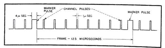
FIG. 4—Pulse multiplex signal that modulates microwave transmitter
