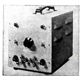
use. Output is continuously variable from 180 to 360 volts, and will remain constant to within 1 percent for loads from 0 to 75 milliamperes, and for line-voltage variations of plus or minus 10 percent. Either the positive or negative out-
