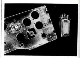
Fig. 6—Portion of chassis showing bridged cutout and a mounted i-f trans-
