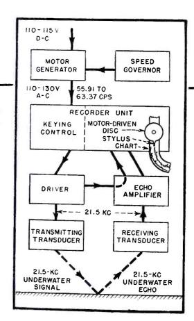
FIG. 1—Block diagram of precision depth recorder employing echo-ranging principle
