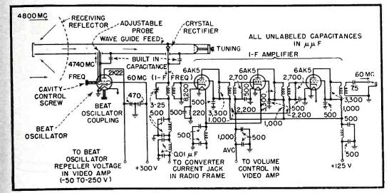
FIG. 8—Using a reflex Klystron as a local oscillator, the receiver converts the microwave carrier to the intermediate frequency in a crystal
