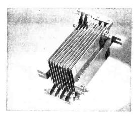
designed to withstand an rms voltage of 26 volts. The method of mounting improves air circulation, so that the stack can be mounted vertically or horizontally.
