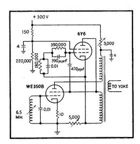
FIG. 11—To stabilize the saw-tooth oscillator, a resonant circuit is introduced into the grid circuit
