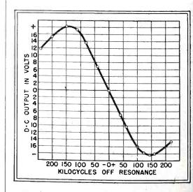
Fig. 2—Discriminator response of a production receiver
