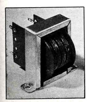
The assembled oscillator transformer has four ple windings. Construction details are given under Specifications
