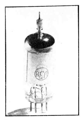
FIG. 5-New high-voltage rectifier tube. type 1654
