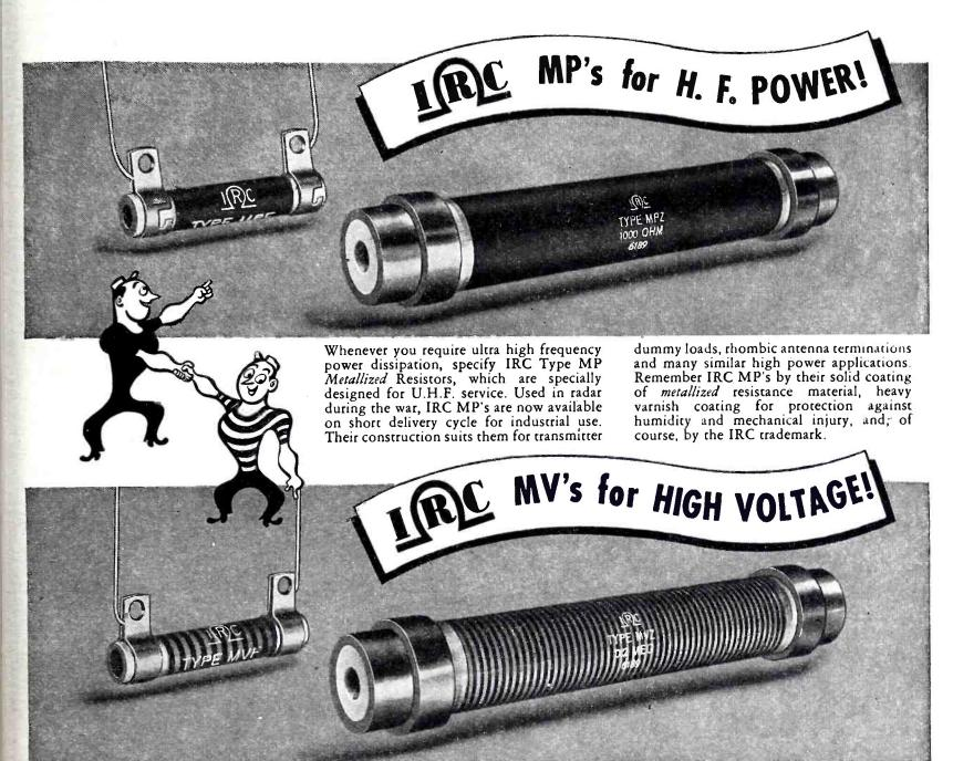
In high voltage applications where requirements are for high resistance and power, IRC MV High Voltage Metallized Resistors are designed and constructed to do the job. They are manufactured with the famous metallized coating applied spirally on ceramic forms. This provides a conducting path of extensive effective length. Turns are
