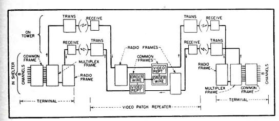
FIG. 9—Two sets connected back to back through their radio frames act as relays for links longer than line of sight
