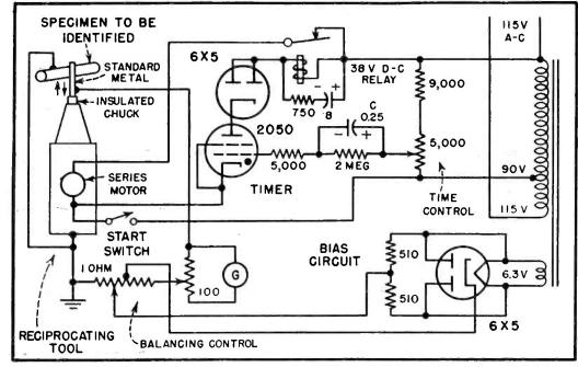
FIG. 2—Electronic circuit used in connection with reciprocating tool for nondestructive identification of alloys
