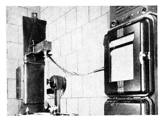
FIG. 7—High-speed dilatometer (left) and recorder
