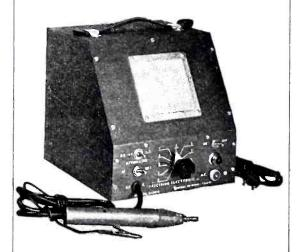
with associated detector and loudspeaker used in tracing modulated r-f signals through receivers and allied electronic equipment. The equipment operates from a 110- to 120-volt 60-cycle line. It lists at \$29.95.
