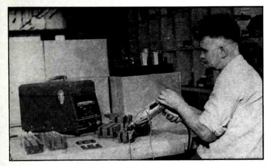
Commercial version of triboelectric instrument, used here for sorting transformer laminations accidentally punched from two different grades of steel
