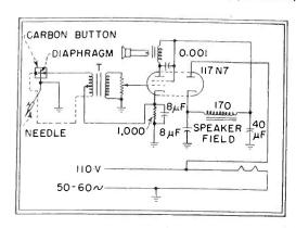
One-tube amplifier and rectifier circuit used in testing the carbon pickup. A double-button unit could be connected as shown by the dashed line
