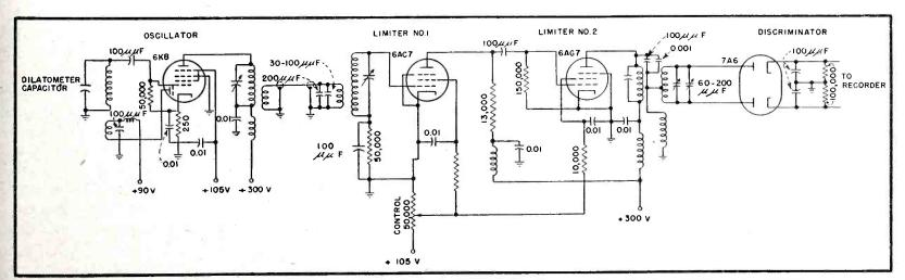
FIG. 8—Single-channel dilatometer circuit diagram. The recorder input and switching details are omitted
