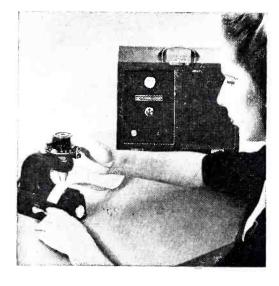
measure the instant of contact between a calibrated lead screw and the material being gaged without exerting pressure. The units are operated from any a-c outlet.
