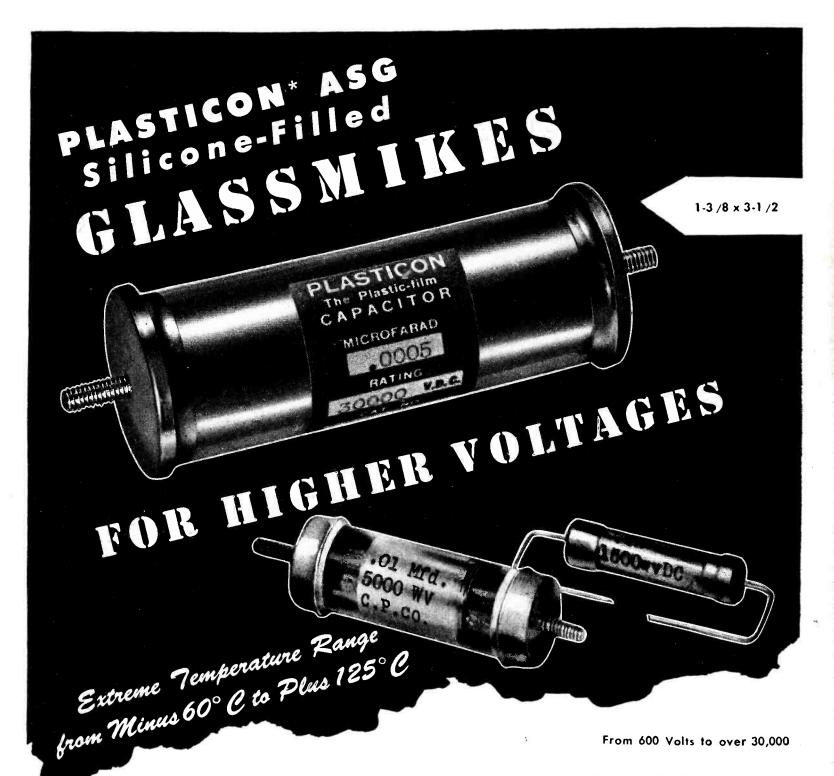
Modern functionally designed capacitors. Metal ferrules are soldered to silver bands fused to each end of heavy-walled glass tubes. This vacuum tight assembly is fungusproof and passes Signal Corp, Air Corp, and Navy thermal cycle and immersion tests. Ample flashover spacing is provided between silver bands for sea level operation. Submit specifications for high altitude applications.
