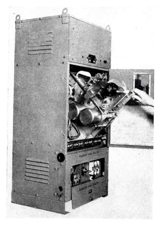
Central station recorder with the tape printer tilted forward for access
