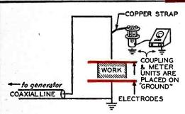
Quickly and directly measures r-f voltage between applicator electrodes. Enables you to vary load voltage during heat cycle in accordance with any pattern you select, or regulate the voltage on one load after another to assure uniform results.
