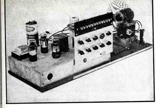
Front view showing tone generator out of its cabinet. Pushbuttons turn individual lamps on and off, while rheostats below permit changing brilliancy of any lamp to vary the amplitude of the corresponding harmonic
