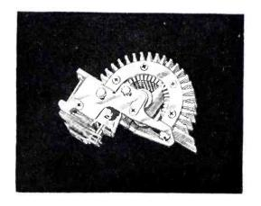
making a maximum of 8 or 4 contacts, respectively. Operated from a telephone-type dial pulser the maximum operating speed is 30 steps a second, or double that speed with self-cycling operation.
