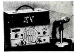
with a 5-inch permanent magnet speaker, a desk stand microphone, and is priced at \$595, less tax. The unit operates from 115-volt alternating current.
