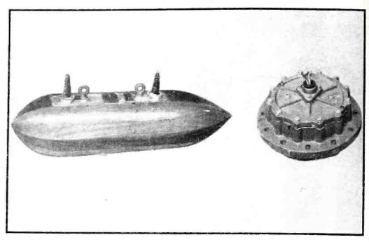
Streamlined outboard "fish" used to support portable magnetostriction units for hydrographic survey work, and one of the magnetostriction units
