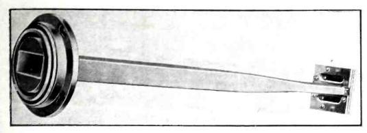
FIG. 5—Waveguide from transmitter is terminated in slot dipoles, at extreme right, which radiate back toward the parabolic reflector
