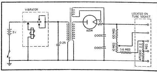
FIG. 4—Circuit of 5,000-volt pocket-size power supply
