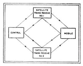
Fig. 1—Multicarrier diversity transmission system provides wide coverage at uniform signal strength
