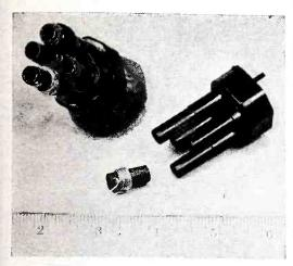
Fig. 3—The i-f coils are slipped over the posts on the molded piece at right to form the complete assembly at left
