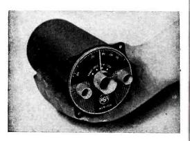
units can be mounted in out-of-theway places. The receiver tunes from 200 to 415 kilocycles, but can be switched to the traffic control channel on 278 kilocycles without disturbing the position of the variable tuning dial. A range filter for 1,020 cycles is also available.
