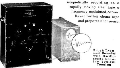
Brush Tran-sient Recorder with Oscillo-scope Show-ing Typical Transient
