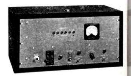
has an input sensitivity of 0.25 volt and a resolving time of better than 5 microseconds. It is little affected by changes in line voltage. Input line voltage can vary between 95 and 130 volts.
