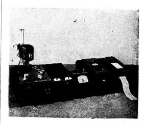
ishes from 1 to 5,000 microinches. Visual and graphic indications are given of surface finishes of metals, glass, plastics, plated and painted materials.
