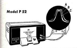
For rapid alignment of I.F. coils of frequencies from 85 kc to 11 mc. Operator adjusts test trace (B) to fall between traces of limit coils (A and C), set up to production specifications. Defective coils immediately detected. All error is eliminated as circuit changes or line voltage
