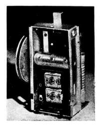
plished by moving the carriage along a rack by means of brass ribbons terminated on a brass cylinder of about \{\mathbf{g}\-inch\ diameter\ as\ illustrated.\ The movement is positive and claimed to be noiseless.
