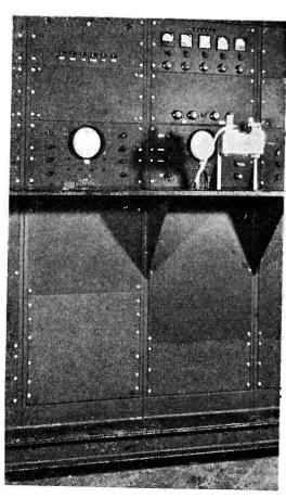
Fig. 1—Two sections of the five-channel oscillograph used to record forces in milling cutter
