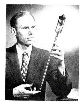
megacycles is typical of the device. The tube is a foot long and a few inches in diameter. Its amplifying property results from the transfer of energy from an electron stream to a wave moving on a helix surrounding the stream.
