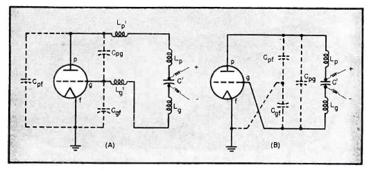
FIG. 1—The combination of interelectrode capacitances and tube lead inductances. plus—if necessary—externally added inductance, gives a high-frequency oscillator (A) which is basically a Colpitts circuit (B)
