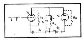
FIG. 4—Elements of basic damping circuit that acts like the switch of Fig. 2
