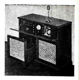
switch and broadcast receiver, making possible the automatic recording of programs in the absence of the set owner. In addition, a disc record album can be continuously embossed on the film from the turntable and pickup with which the console is equipped. Other recorders suitable for office and home use are also available.
