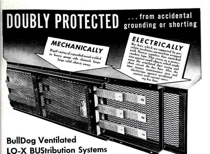
VENTILATED "Lo-X" BUStribution Duct, manufactured by BullDog Electric Products Company, Detroit, makes plant layout flexible because it gives access to adequate power supply up to 4000 amp., wherever it is needed. Wide, flat bus bars supported by porcelain insulators are arranged in closely spaced, paired phase design to assure low voltage drop by reducing reactance lose.
