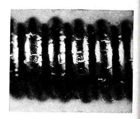
This enlarged photograph shows enameled magnet wire stretched 10 per cent—half as much as the Formex wire in the top illustration—and wound upon twice its own diameter. Note the cracks in the insulation, the absence of cracks in the Formex wire.
