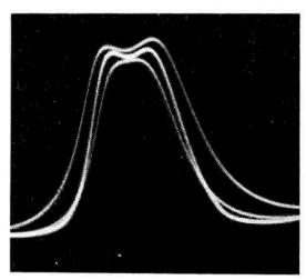
The production coil is adjusted so that its curve falls within the limit traces that have been previously standardized
