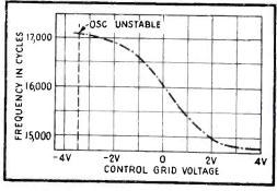
FIG. 6—Saw-tooth frequency and grid voltage for one value of screen voltage
