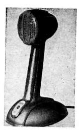
phone has a substantially flat response from 70 to 7,000 cps. Voltage developed by normal speech (10 dynes per square centimeter) is 0.0394 volt. The unit works into a high-impedance input amplifier. The model 902 microphone lists at \$13.25.
