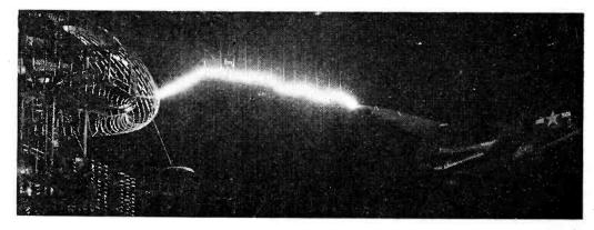
Artificial lightning leaps from electrostatic generator to Ventura twin-engine bomber suspended from roof of special laboratory at Wold-Chamberlain Airport, Minneapolis during research on causes and cures for precipitation static
