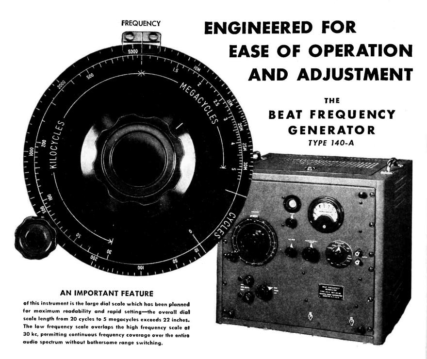
One of the most valuable instruments in the laboratory is a generator of signal voltage. Boonton Radio Engineers in designing the Type 140-A Beat Frequency Generator have provided an instrument of wide frequency coverage, capable of supplying accurate output voltages ranging from several microvolts to 30 volts and having a variety of output impedances from 20 ohms to 1000 ohms.
