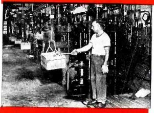
One of several batteries of precision presses for molding Mykroy. Here are produced a large percentage of all molded mica ceramic parts now being used in many industries.
