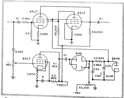
Fig. 1—Circuit of single-ended volume expander that requires no pushpull transformer for canceling out the d-c surge in each expander tube
