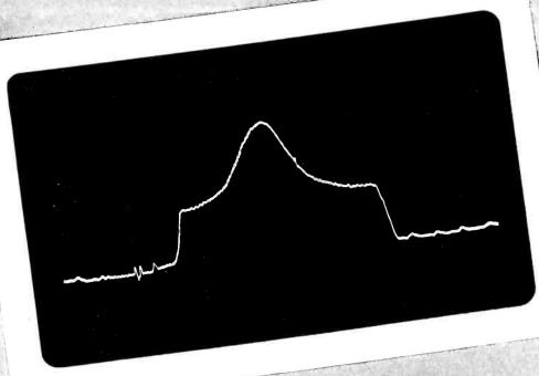
Brush Transient Recorder caught this photoflash bulb exposure in recent tests on camera shutter synchronization. A transient of 40 milliseconds duration—automatically recorded and reproduced for study! This wave trace indicates peak light intensity at exactly the right moment—an excellent start toward a perfect picture! Such transient phenomena recording by the Brush Transient Recorder bares production defects never before so easily measured.
