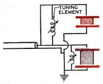
Simplifies the adjustment of a setup consisting of two or more pairs of electrodes connected in parallel. The heating rate of each can be adjusted as desired.
