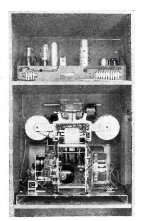
Rear of the central station. Below the electronic equipment chassis is the electromechanical printer and averaging device. The sequence switch is shown at the right. Power supply below is omitted
