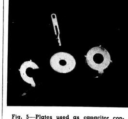
Fig. 5—Plates used as capacitor contacts and terminals
