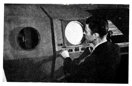
These two radar scopes give the air traffic controller a picture of all planes in the air within a radius of 30 miles from the control tower. Scope at left indicates altitudes of planes in thousands of feet, while that at right gives ppi presentation for azimuth
