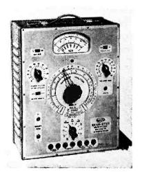
and comprises a d-c bridge to measure capacitance from 10 micromicrofarads to 2,000 microfarads and resistance from 100 ohms to 7.5 megohms. A supplementary circuit allows measurement of resistance up to 10,000 megohms.
