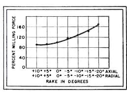
Fig. 3-Effect of rake on milling forces is plotted from many oscillograms
