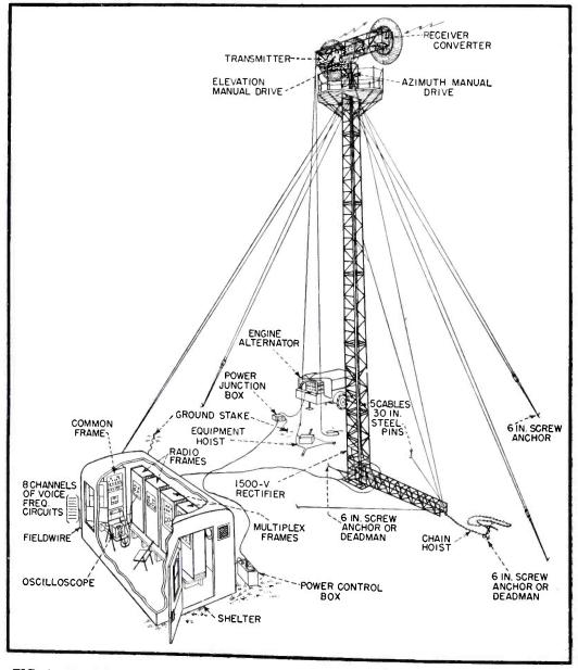
FIG. 1—Field layout of pulse modulation voice multiplex microwave communication terminal
