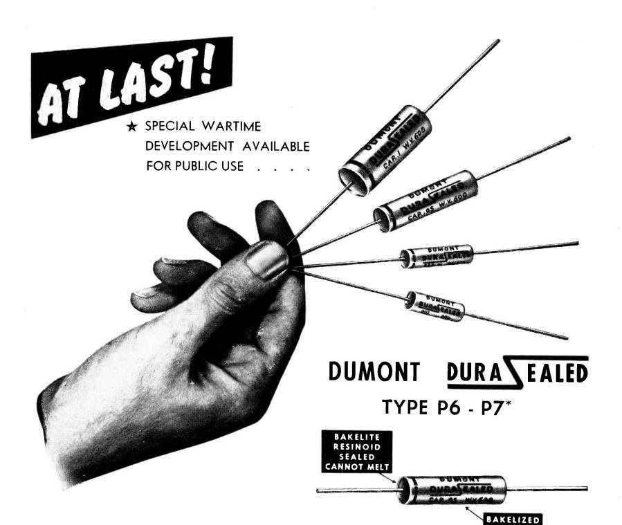
★ Dumont engineers scored in the greatest single achievement in paper tubular capacitors . . . meeting the most exacting requirements. This type P6 has the ends sealed in BAKELITE RESINOID. Leads cannot PULL OUT or MELT OUT. Bakelite treated tubes sealed in vacuum.
