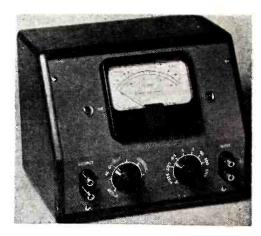
static voltmeters represents improvements over existing equipment, particularly in the reduction of leakage. For a-c measurements, a true rms value is very little dependent upon frequency. Accuracy of 1 percent or better is possible. Instruments with ranges from 300 up to 35,000 volts are available.
