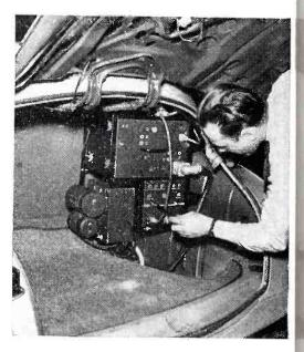
In the baggage trunk of the cab are mounted the 40-watt f-m transmitter at top, receiver at lower right, and dynamotors at lower left
