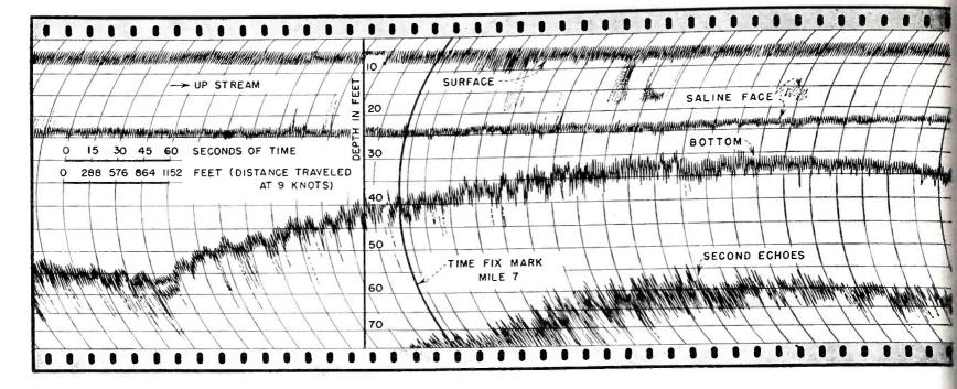
Profile of river bottom along 1.75-mile stretch of Southwest Pass, near mouth of Mississippi River, as made with precision shallow-water depth recorder. In addition to bottom depth, an experienced operator can accurately interpret such additional information as
