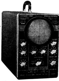
testing and radio servicing. Vertical and horizontal amplifiers have a range from 20 to 50,000 cycles. Deflection sensitivity at full gain is 0.65 rms volt per inch. List price is \$99.50.
