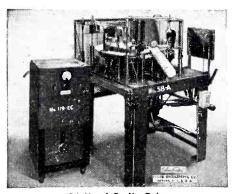
24 Head Radio Tube Exhausting Machine.
