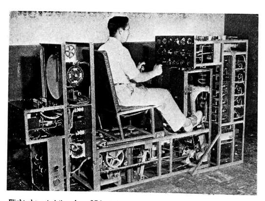
Flight characteristics of an AT-6 airplane in the air are simulated by the prototype version shown above stripped of its aluminum fuselage. Produced for the Army Air Forces by Curtiss-Wright, it uses serves to feed an electronic computer
