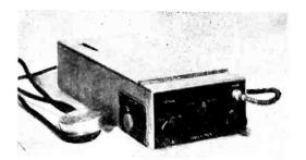
playback. Four subminiature tubes are used with small batteries having a life well in excess of the maximum time for a continuous recording. The unit measures  $9\frac{1}{2} \times 4\frac{1}{4} \times 2\frac{1}{4}$  inches and weighs  $4\frac{1}{2}$  pounds.
