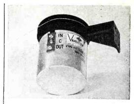
adjusted automatically as the cutting head of a recording lathe progresses across the disc, equalizing from 8 db at 5 inches to 0 db at 12 inches at 10,000 cycles. Impedance of the device is 500 ohms and the insertion loss is 10 decibels.
