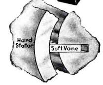
Internal Vane is softer than the stator. Wears indefinitely and improves with use.
