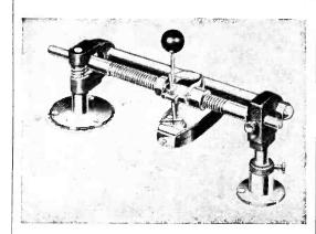
low cost for 12- or 16-inch discs. Cutting pitch is 110 lines per inch, outside-in. Four types of Astatic cutting heads are presently available. The 16-inch model sells for \$55.
