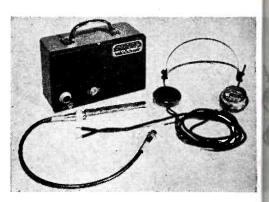
headphones. An internal oscillator converts 135 volts from the B battery to a counter operating potential of over 1,000 volts. The unit measures  $7 \times 5 \times 3$  and weighs  $4\frac{3}{4}$  pounds without batteries. It costs \$150 complete, f.o.b. Arlington.
