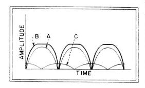
Fig. 2—Comparison of the wave shapes produced by conventional and wave-form controlled rectifiers shows closer approach to d-c in the output of the latter
