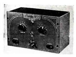
millivolts from the former. The high voltage is variable from 180 to 300 volts and the bias continuously from 0 to 75 volts. A 6.3-volt unregulated winding furnishes 2 amperes.
