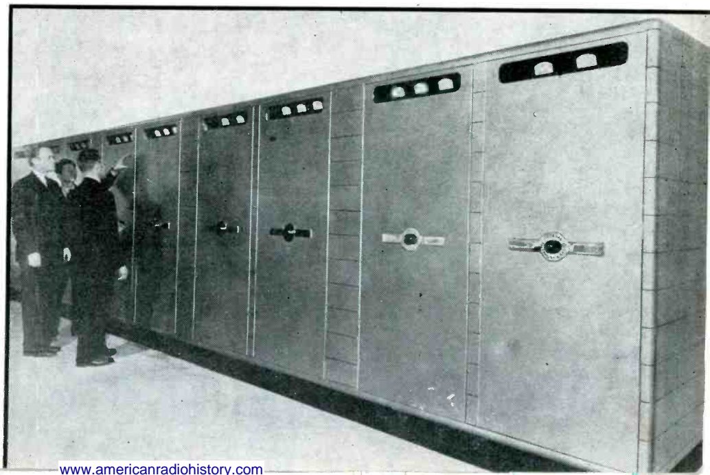
Front view of transmitter. The large size is required to provide sufficient r-f and video stages to reach 1-kw peak output modulated over 10-mc band
