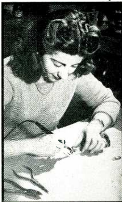
Soldering of subminiature tube leads to a printed ceramic chassis. Ceramic capacitor discs in foreground are also soldered to the steatite
