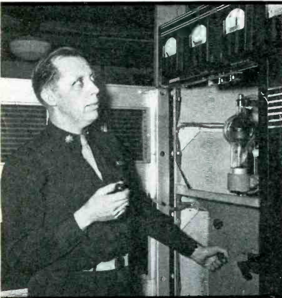
Lt. Colonel John H. DeWitt, Jr., in charge of the project, at the power supply controls of the transmitter, a modified version of the SCR-271 early-warning radar used at Pearl Harbor. DeWitt is former chief engineer of WSM
