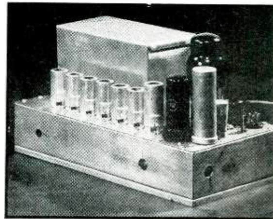
FIG. 4—R-f and video signal components of the receiver. A crystal mixer and six i-f stages (at left of center) are used, and 8-microvolt sensitivity is achieved
