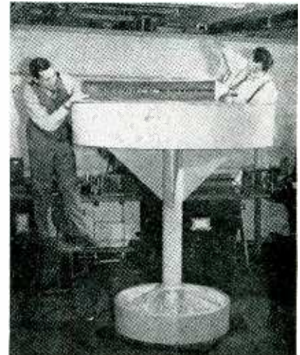
Westinghouse engineers mount the antenna for laboratory tests of marine radar equipment for the Old Bay Line's Baltimore-Norfolk night boat, City of Richmond . The antenna will rotate under a mushroom-like protective cover atop pedestal to be located on the wheelhouse roof
