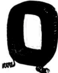
GENERATOR FIELD COIL
