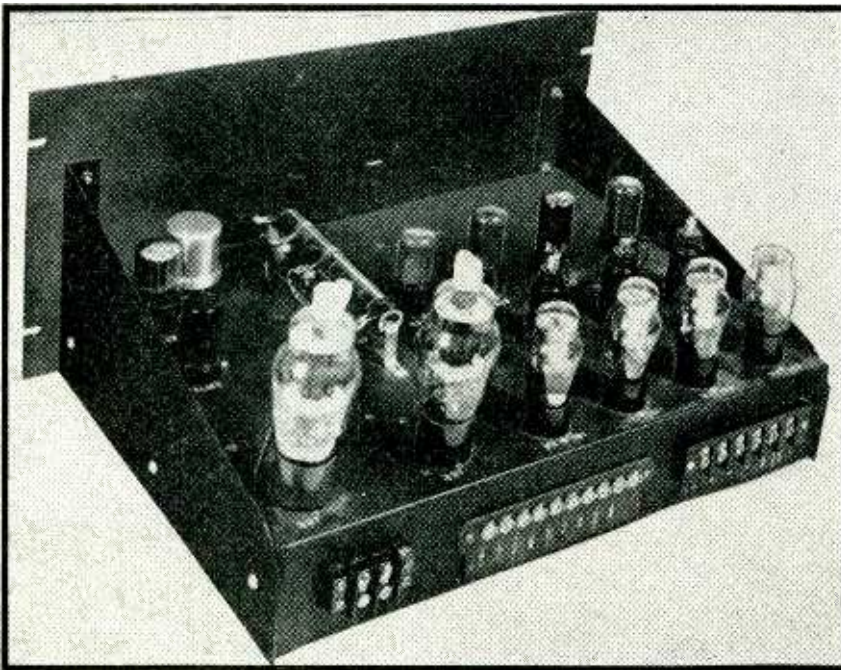
Top chassis view of the four-channel electronic switch, showing the ring-counter and gate-amplifier tubes at the right and the crystal-oscillator trigger circuit tubes near the front panel. The wide-band amplifier tubes are type 807
