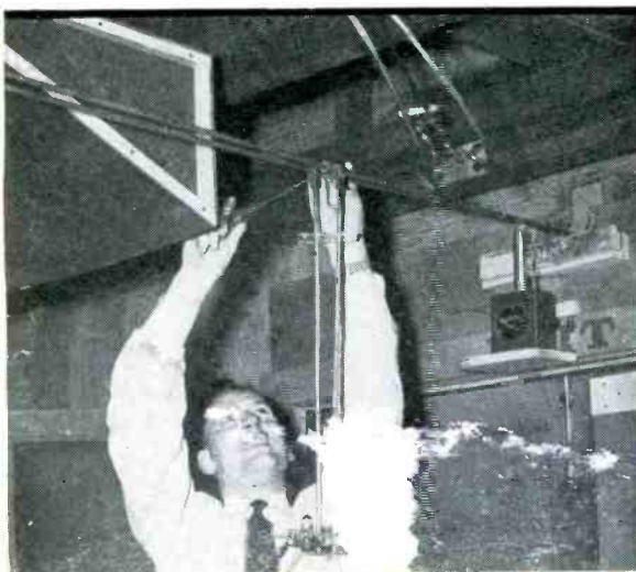
The author, Jack Mofenson, adjusts the position of the waveform-monitoring stub. Over this transmission line traveled the 3-kw transmitted pulse and the millionth of a billionth of a watt echo
