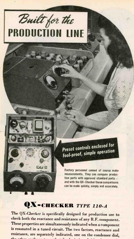
the other on the meter so that the deviation of either from established tolerances is immediately shown. Insures uniform parts held within close tolerances. Frequency range 100 kc. to 25 mc.
