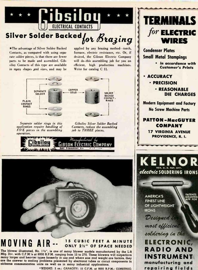
WEIGHT: 2 oz.; CAPACITY: 15 C.F.M. at 8000 R.P.M.; CONSTRUCTION: Housing of high impact phenolic plastic. Wheel is turbo-type cadmium-plated steel; SIZE: 25%" long x 61/64" wide x 2½" high.
