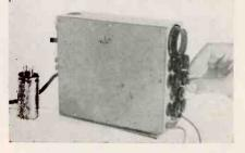
Midget controls and a 1½-in. c-r tube permit the Miniscope panel to be only two inches wide
