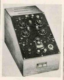
high and low limit dials covering a range of plus or minus 11 percent in 0.1 percent steps, and uses a sensitive built-in galvanometer to provide for the high and low indication, respectively. This bridge can be used to check resistors between 1 ohm and 3 megohms.
