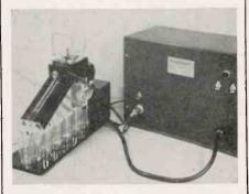
Complete equipment of the ball-sorting gage developed by Jack and Heintz engineers
