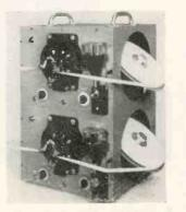
quired to provide a new roll of tape for the first recorder. The Model MA-126 can also be furnished for relay rackmounting. It operates on either 110-220 volts, 60 cycles, or 220-230 volts, 25-50-60 cycles. Designed for efficiency at a rate of 1200 words per minute, the unit handles low and average speeds with ease.
