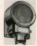
road-type cast aluminum case. The unit can be mounted in any position. It is rugged and is capable of withstanding shock and vibration, as well as prolonged exposure to smoke, dust and other elements. Voice coil impedance is rated at 12 ohms nominal value. Power handling capacity for speech is rated 10 W. Jensen Radio Mfg. Co., 6601 S. Laramie Ave., Chicago 39, Ill.
