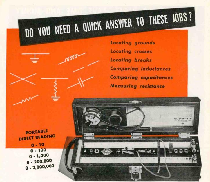
• The type GOM ohmmeter is a handy, all around measuring instrument of the bridge type, particularly well suited for work on wire circuits.
