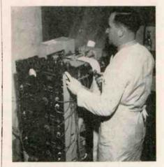
The only electro-encephalograph in Australia is shown in operation at an RAAF center near Sydney. The instrument detects microscopic brain waves, amplifies them, and records them on a paper strip to help doctors diagnose brain conditions in military patients. The recording shown below indicates a near-normal condition which develops into an abnormality that may be due to an unseen brain injury
