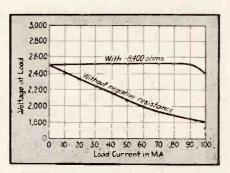
FIG. 27—Improved regulation obtained with negative resistance in Klystron power supply
