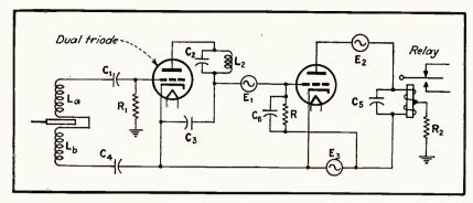
FIG. 5—Oscillator relay circuit arranged for operation from a power transformer energized by the a-c power line and having three separate secondary windings providing a-c voltages  $E_1$ ,  $E_2$ , and  $E_3$
