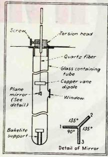
Construction of induced dipole for u-h-i field strength measurements. The insert shows the minor details: reflecting surfaces are represented by heavy lines
