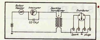
FIG. 4—Addition of a ballast resistor in the primary excitation line gives a constant break-current which permits better highspeed operation
