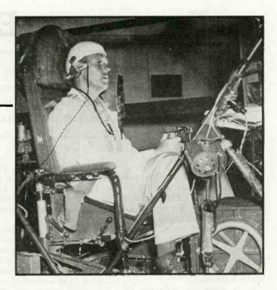
SEATED in an aircraft pilot's position, a volunteer, above, is whirled in a human centrifuge at speeds calculated to reproduce the effect of pulling out of a dive at various values of g.
