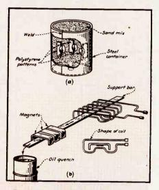
Fig. 2—A mold for centrifugal casting of steel parts is shown at (α) and α method of heat-treating and quenching magnets at (b)
