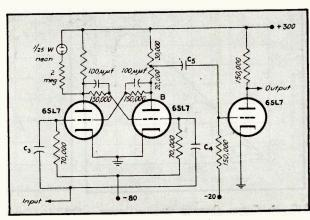
FIG. 9—Basic scale-of-two trigger circuit and rectifier output stage employed in the scale-of-64 counting arrangement
