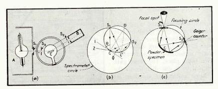
FIG. 3—Bragg ionization spectrometer for single crystal analysis (a), focusing crystal arrangement of Bragg spectrometer (b), and focusing spectrometer arrangement for powder diffraction (c)
