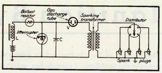
FIG. 5—Further addition of a charging inductor and gasfilled discharge tube in primary circuit gives freedom from effects of secondary loading
