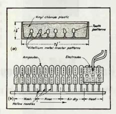
Fig. 3.—A resilient mold for manufacturing false teeth is shown at (a). A conveyor-belt operation for sterilizing ampoules is illustrated at (b).
