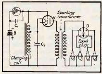
FIG. 11—Breakdown of gas-filled tube in this arrangement generates a high-voltage pulse in the secondary
