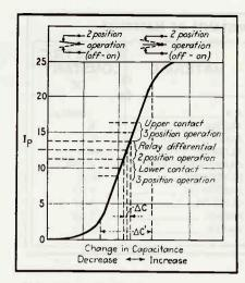
FIG. 10—Typical tuning curve for oscillator relay
