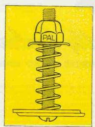
**Adjusting Nut on Relay**
