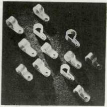
sulated materials from wearing off. Clips are non-corrosive, non-conductive, light in weight, strong and resistant to acids, alkalies and oils. They are fabricated with LT Ethocel, a thermoplastic developed by Dow to provide toughness, shock resistance at low temperatures, and low dimensional change over a wide range of atmospheric conditions.
