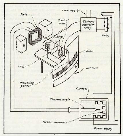
FIG. 7—Schematic diagram showing arrangement of basic elements of an oscillator relay system, with connections to a pyromatic control system shown as a typical application
