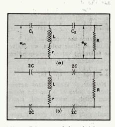
FIG. 1—Either an unbalanced (a) or a balanced (b) high-pass filter can be used to introduce a leading phase shift
