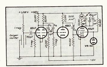
FIG. 8—Pulse producer and pulse averaging circuit of counting rate meter used in Geiger counter focusing spectrometer
