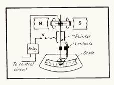
FIG. 1—Basic arrangement of a moving-coil contacting instrument, wherein the meter pointer carries a contact
