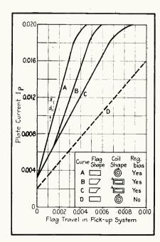
FIG. 6—Effect of flag travel, flag shape and use of regeneration on plate current of an oscillator relay system
