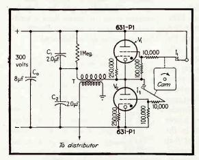
FIG. 13—Cold-cathode tubes serve this system in conjunction with α single ignition coil and one distributor. A high-voltage source is required
