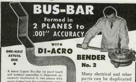
angles formed both flat and edgewise, across the material horizontally and vertically.
