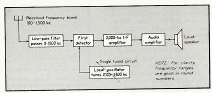
FIG. 2—Block diagram showing essential features of a broadcast and longwave receiver having a 2-megacycle i-f amplifier
