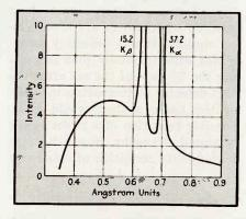
FIG. 1—X-ray spectrum of molybdenum bombarded with 35-kilovolt electrons. showing characteristic lines
