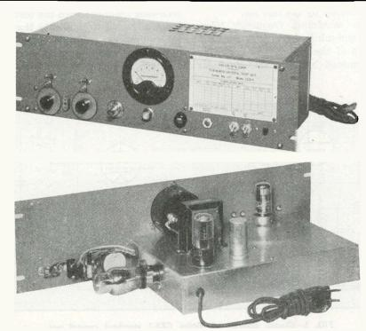
Front and rear views of quartz crystal test set show simplicity of design.
