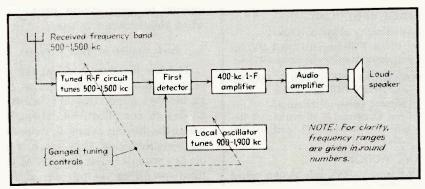
FIG. 1—Block diagram of conventional broadcast receiver, which requires ganged controls for tuning the r-f input circuit and the local oscillator
