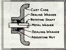
Fig. 2—Method of sealing α shaft hole in α cast panel
