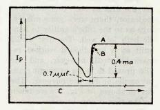
FIG. 3—Plate current of a crystal oscillator changes as the tuning capacitor is tuned through resonance. Data for this curve was taken from an oscillator using the triode section of a 6E5 tube, and an X-cut 7-Mc crystal
