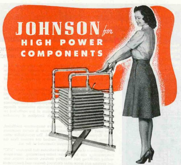
To meet the need for a light-weight, high-capacity, high-voltage tank condenser for transmitter applications, Johnson engineers developed a new type of condenser. The unit illustrated has a capacity of 1200 mmf. at a peak voltage of 40,000 volts at 2 megacycles. Nearly any combination of capacity and voltage ratings may be had. The capacity may be varied in the field by removing plates or altering spacing.
