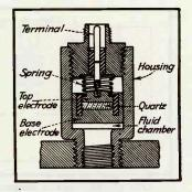
FIG. 15-Ignition can be directly related to the pressure-time curve by a system utilizing a crystal as shown
