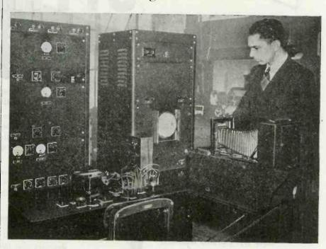
The measurement of tube characteristics in regions where previous test methods were inapplicable has been made possible through the development, by Sylvania Electric, of a new procedure, based on photographing an oscillographic trace.
