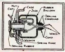
Fig. 7-A rubber balloon behind the panel and an auxiliary rubber cover seals a phone jack
