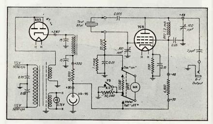
FIG. 1—Circuit diagram of Model CES-1 standard crystal test set. Note reduced heater voltage to insure long tube life
