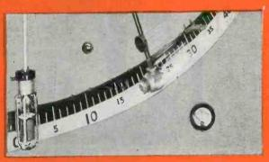
QST-3—United tubes designed for very rough service have extro, built-in shock resistance proved by the severe Bump Test each tube must poss.
