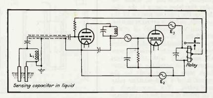
FIG. 11—Oscillator relay circuit adapted for liquid-level sensing operation
