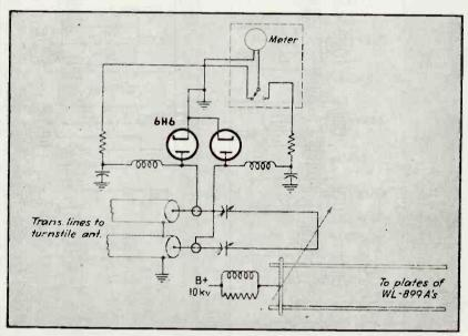
FIG. 5—This vacuum-tube voltmeter is used in place of thermo-ammeters at the input to the transmission lines feeding the antenna system
