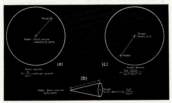
FIG. 1—Geometric relations underlying the radar equation
