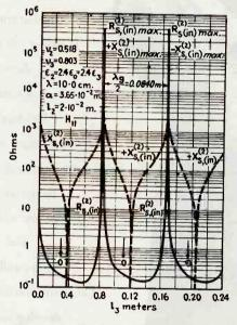
Fig. 2—Terminal impedance of guide of Fig. 1 for which the attenuation in guide is 2.11 × 10<sup>-3</sup> nepers/m; in the dielectric is 2.93 × 10<sup>-3</sup> nepers/m; phase shift in guide is 37.5 rad/m; in dielectric is 83.4 rad/m
