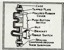
Fig. 5—A molded rubber cover seals pushbuttons and toggle-switch handles
