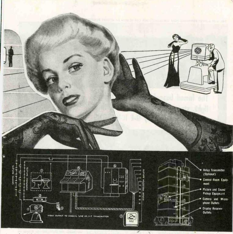
A typical G-E intra-Tel system. With the Intra-Tel system, portable television cameras and sound microphones can be operated from any place in store or plant. Pictures and sound picked up by cameras (1) and
