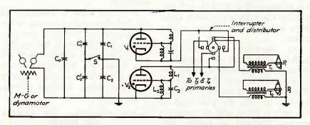
FIG. 9—Aircraft ignition systems encounter problem of high-altitude loss in insulating properties of the atmosphere. This circuit gets away from arc-over, leakage, and cross-firing by using special spark plugs and two gas-filled triodes
