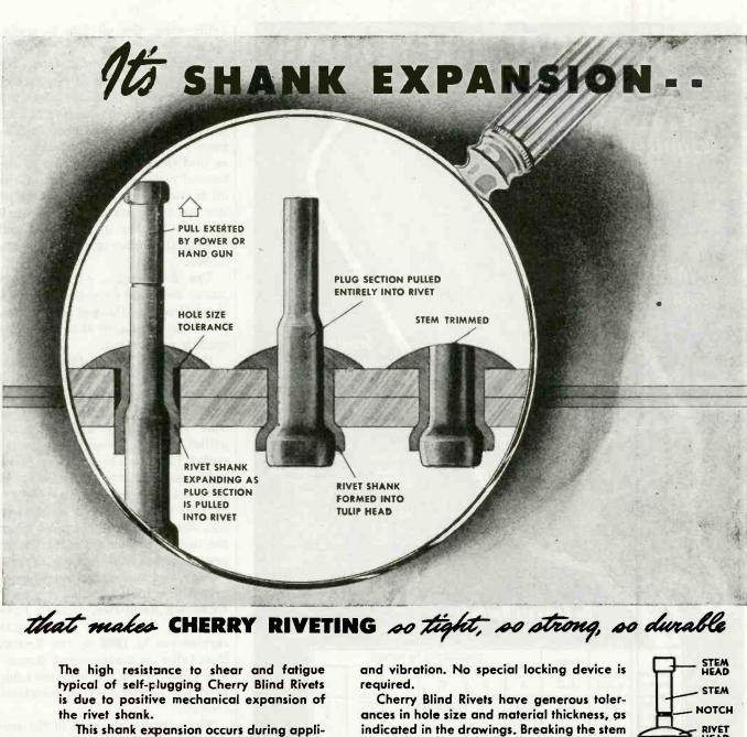
cation when the enlarged plug section of the stem is pulled into the rivet (drawings to right and above). The sides of the rivet are forced against the material being fastened, filling any irregularities in the drilled hole. The installed Cherry Rivet has shear and fatigue values comparable with those of a solid rivet—stays firm, even under excessive strain
