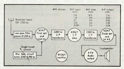
FIG. 3—Block diagram of the test receiver for which constructional details are given in this article. Use of a 2000-kc i-f value permits high-quality local reception with only five tubes
