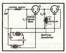
FIG. 7—Availability of a high-voltage source makes possible the application of a circuit which provides powerful sparks at a rate of speed higher than can be attained in a make-and-break arrangement
