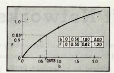
FIG. 3—Graphical interpolation is used to determine the attenuation factor F from the value of b obtained from the charts
