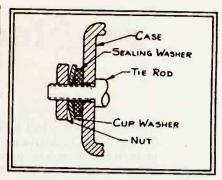
Fig. 6—Simple seal for tie rods
