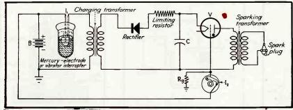
FIG. 12—High-speed acceleration is improved by this circuit which combines power-supply interrupter with timed breaker and gas-filled triode
