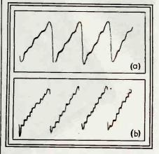
FIG. 2—Synthesis of a saw-tooth wave using (a) the first four terms in the Fourier series and (b) using the first eight terms
