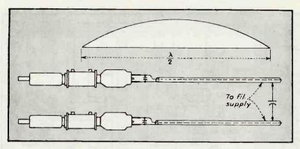
FIG. 4—The addition of half-wavelength lines in the WL-899A filament circuits overcame difficulties caused by reactance in these circuits of the 50-kw 1-m station final r-f amplifier
