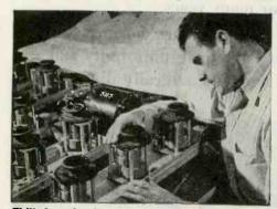
Skilled mechanics assemble and synchronize the heavy duty Autotunes used on the output network of the 3000 watt Collins 231D ground station transmitter.
