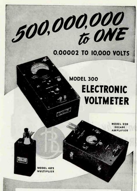
This enormous range of voltages—five hundred million to one—is accurately covered by our Model 300 Electronic Voltmeter and some of the accessories shown above. Frequency range 10 to 150,000 cycles. Accuracy 2% over most of the range. AC operation. Five decade ranges with logarithmic scale make readings especially easy. Uniform decibel scale also provided. May also be used as a highly stable amplifier, 70 DB gain, flat to 150,000 cycles.
