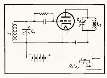
FIG. 2—Tuned grid, tuned plate oscillator circuit used in all types of oscillator relay systems
