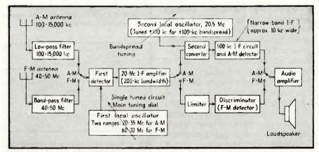
FIG. 5—Block diagram of proposed combination a·m/1·m communication receiver employing a 20-Mc i-t value. Both local oscillators are tuned, but the second is used only for bandspread purposes
