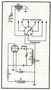
FIG. 8—Triode in circuit as shown attacks problem of cross-firing between high-impedance spark-plug leads. This circuit is particularly useful in fuel-injection-type engines using a continuous discharge
