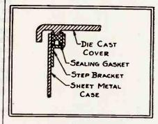
Fig. 1—Detail of end of a metal cabinet showing use of a step bracket
