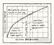
Typical activity correlation curve relates CES-1 test set indication to average radio equipment requirement. These curves are the means by which determinations of specification values are made for crystals
