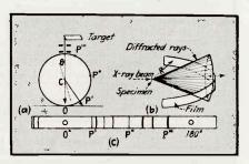
FIG. 2—Basic arrangement for analysis by powder diffraction (a), use of cylindrical film to intercept a cone of diffracted radiation (b), and example of pattern obtained on film (c)
