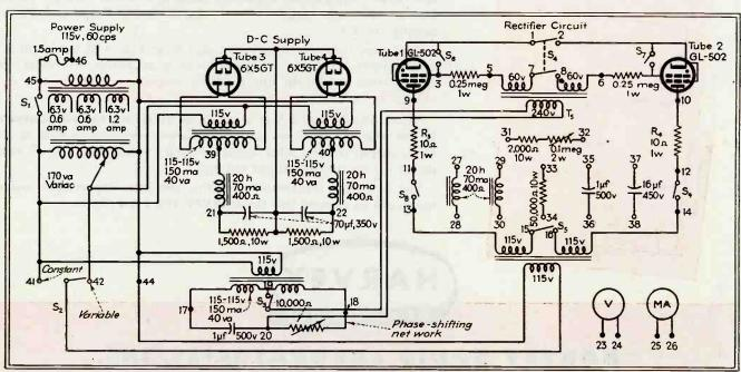
Circuit of wave-form demonstrator for controlled rectifier circuits. All terminals numbered from 1 through 38 go to jacks on the front panel, for use with patch cords in setting up various circuit combinations for connecting these terminals to the two meters
