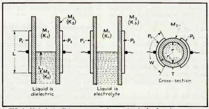
FIG. 8—Method of utilizing a manometric capacitor for level-sensing purposes
