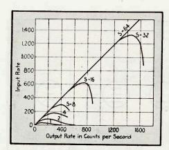
FIG. 10—Curves showing counting losses as a function of the scaling ratio
