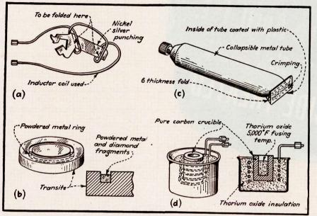
Fig. 1—Shape of coil used to heat two spots on a metal strap for later bending.
