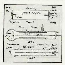
FIG. 7—Three types of Geiger counter tubes suitable for detecting soft x-rays
