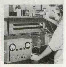
Instantaneous detection of mercury vapor in the air of industrial plants is made with this G-E instrument. It measures concentrations as small as one part in 200,000,000
