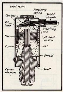
FIG. 10—All high-frequency currents in the spark-produced transient are confined to the spark plug itself in this design which serves with the circuit shown in Fig. 9
