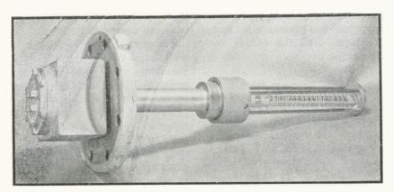
Immersion capacitor designed for use with oscillator relay to sense liquid levels in a high-pressure system. Note the heavy construction and the film-destroying corrugations on the protecting tube
