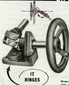
The type "H" hinged Universal Link Joint with solid shafting has three distinct advantages for remote controls. (1) Simplicity of installation (the Universal Link Joint hinges from 0 to 90°). (2) A minimum of backlash. (3) Output shaft turns in exact angular rotation with the input shaft.
