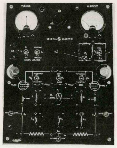
Front panel of wave-form demonstrator, developed for use as a teaching aid in industrial electronics classes
