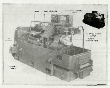
A combination of electronic and hydraulic controls on this one Sundstrand cylinderhead fin miller permits cutting the same number of fins as formerly required four machines. During the milling operation, the work is totally enclosed as shown in the insert
