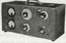
This instrument retains the same general operating principles and characteristics of the 160-A Q Meter but with such structural modifications and design refinements as are required for accurate performance at higher frequencies. Has a continuously variable frequency range of 30 mc to 200 mc.
