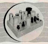
7. HIGH-QUALITY AMPLIFIERS—The several types of standard, RCA studio amplifiers are well-suited for FM use. All amplifiers have a flat frequency response, which may be compensated, when desired, for particular installations.
