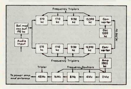
FIG. 2—Block diagram of the phase-shift modulator system. A complete schematic is shown in Fig. 3
