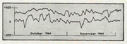
FIG. 1—Graph showing maximum frequency deviations of the modulator unit over a period of two months
