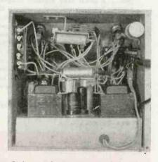
Lights on the front panel of the plug tester are controlled by the relays shown in this rear view of the instrument
