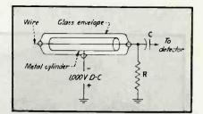
FIG. 4--Fundamental circuit of Geiger counter
