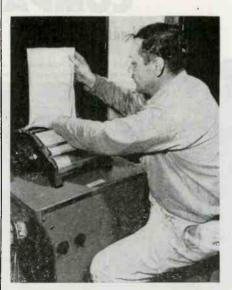
The conductor of a Rock Island freight train removes a facsimile message sent to him by radio from a wayside station. A complete message form is turned out in three minutes
