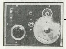
This photograph shows the dials of the meter capacitors, terminals for connection to the test cell, and the 6E5 which serves as oscillator and resonance indicator
