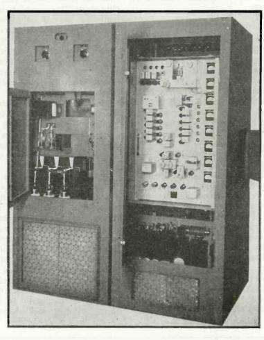
grids of the balanced modulator, in the second unit. In the grid circuit of the modulator is another network, sometimes called the corrector, which produces the inverse audio-frequency effect necessary with a phase modulation system.
