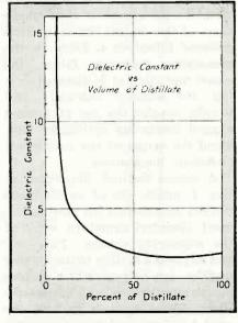
FIG. 6-One industrial application of the dielectric-constant meter is to determine the condition of the charge in a still pot. This curve is for the separation of acetone, toluol, and benzene
