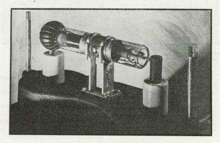
X-ray tube used in the Geiger-counter focusing spectrometer (housing has been removed)
