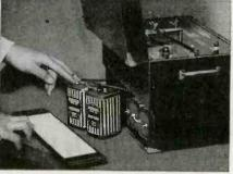
carbanalyzer, powered by Burgess Industrial Batteries, operates over a range of .05% to 1.50% carbon content and is sensitive to a change of ± .005%. The power requirements of modern control and test instruments are fully met by Burgess Industrial Batteries—the standard of quality for all commercial uses. The types you require may not be immediately available today since industrial battery production is greatly reduced by urgent war needs.
