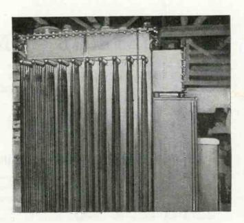
The socket is also made of copper, with an insert of Elkonite at the contact point. In the actual installation, the socket is cut into several segments, each mounted on a spring.
