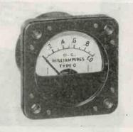
bration and shock in aircraft service. The manufacturer states immersion tests show the units will withstand hydrostatic pressures up to 14.7 psi without case leakage. Accuracy is rated at 2 percent. They are available in all practical ranges above 50 millovolts as d-c voltmeters, and in all practical ranges above 500 microamps as d-c ammeters. Lower ranges can be supplied for other applications.
