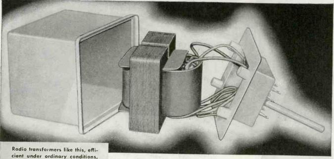
cient under ordinary conditions, had been going bad in airplanes. The trouble was traced to moisture, condensation being accelerated by changes in altitude and temperature. Fedelco-Sealing solved the problem. A metal case was designed to fit the original mounting-one requirement; leads were brought through sealed terminals in the base, and the cover was sealed on. Then the case was exhausted, refilled with dry air, and sealed permanently, ending moisture troubles.
