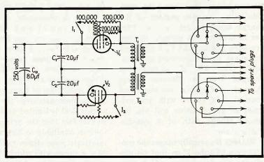
FIG. 14—This circuit uses cold-cathode tubes with two coils and two distributors. Ability of these tubes to carry high surge currents makes them ideal for this service
