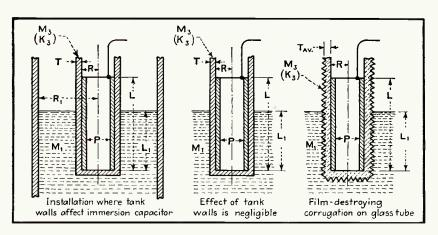
FIG. 9—Use of immersion capacitor for level-sensing applications
