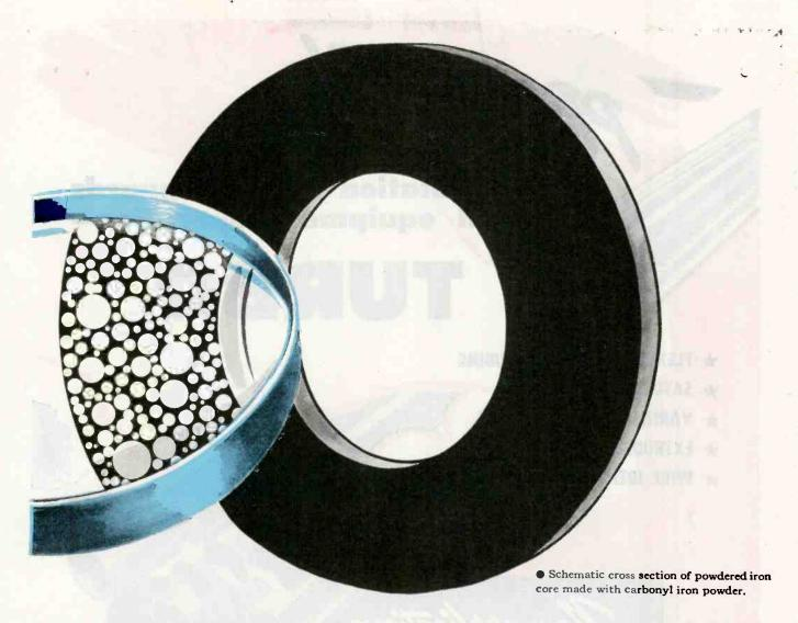
Table 2 below gives relative Q values (quality factors) and effective permeabilities for the different grades of carbonyl iron powder. The values given in the table are derived from measurements on straight cylindrical cores placed in simple solenoidal coils. Although the
