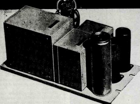
TYPE 201A RECTIFIER. Designed to furnish filament and plate current to line amplifiers such as the Langevin 102 Series. Delivers 275 V. at 75 M.A., 6.3 V. at 8 A. Length  $10\frac{2}{3}$ ." Width  $5\frac{2}{3}$ ." Maximum height  $6\frac{1}{2}$ " (5½" above, 1" below mounting chassis). Occupies one third Langevin Type 3A mounting frame:
