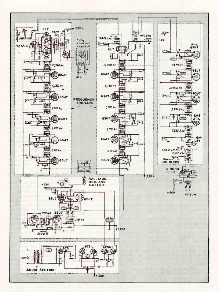
FIG. 3—Schematic of the WMFM phase-shift modulator shown in block-diagram form in Fig. 2
