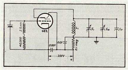
FIG. 4—This type of dielectric-constant meter uses few parts. The 6E5 tube serves both as oscillator and balance indicator. The power supply can have no direct-current path to ground
