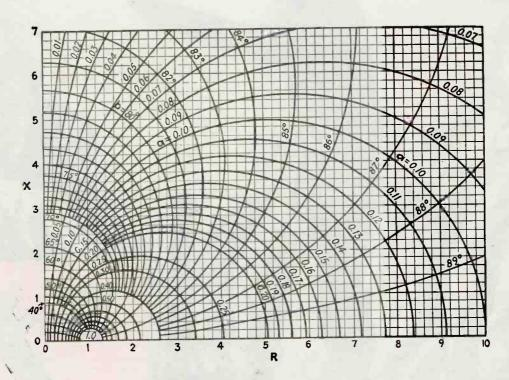
Chart for obtaining transmission-line impedance R+jX from hyperbolic function of propagation constant
