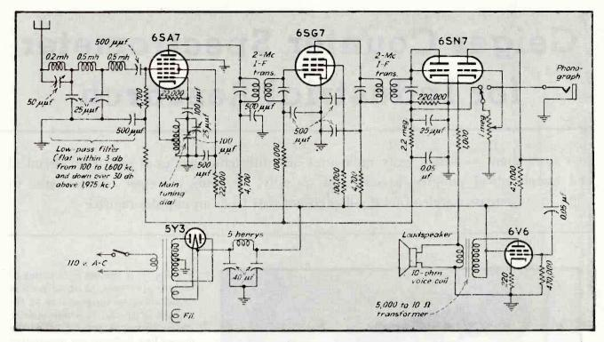
FIG. 4—Schematic circuit diagram of test receiver using 2000-ke intermediate frequency amplifier, with values of all component parts
