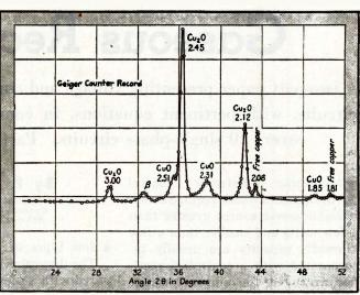
FIG. 13—Plot of focusing spectrometer data for the sample of Fig. 12, showing clearer delineation of peaks, Sample contains both cuprous and cupric oxide and some free copper
