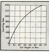
FIG. 11—Calibration curve of complete counting system for focusing spectrometer
