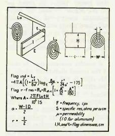
FIG. 4—Two views of the control mass and colls used in the oscillator relay system, with basic equations for inductance and r-f resistance of the moving flag attached to the meter pointer
