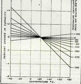
TEMPERATURE COMPENSATION OBTAINED WITH VARIOUS TEMPERATURE COEFFICIENTS
