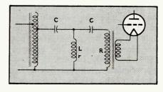
FIG. 2—Application of phase shifting to filament supply
