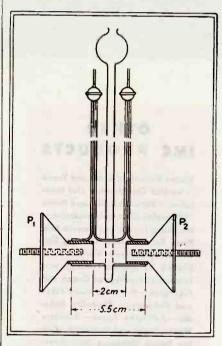
FIG. 1—Voltameter with tin-plated electro-magnetic pole pieces from which gas was expected to be liberated if there is a magnetic current
