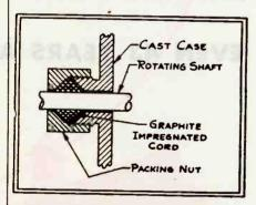
Fig. 4—Shaft hole can also be sealed with impregnated cord and a packing nut
