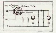
FIG. 3—The use of a mixer tube to combine two light impulses from the phototube Fourier analyzer accomplishes electrically the required mathematical integration of a product
