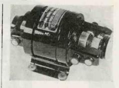
ferent voltages, also, one of the outputs can be ac. A typical unit (perhaps for mobile transmitterreceiver) would be one with a 350v, 50-milliamp output, a 250-v, 25milliamp output, and a 6.3-v ac (100 cps), 2-amp output. The 6.3volt a-c and the 250-volt d-c outputs can be used continuously while the 250-v output is for intermittent duty. Units are compact and light in weight.
