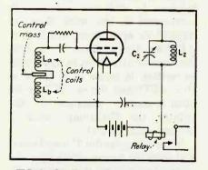
FIG. 3—Oscillator relay circuit in which movement of a non-ferrous metal flag into or out of a pair of coils affects oscillator operation sufficiently to actuate a relay
