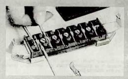
AMP connector block assembled. Connections insulated and locked when cover is in place.
