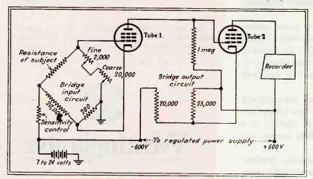
Basic Pathometer circuit, illustrating the electronic principles involved in amplifying changes in skin resistance. The actual circuit now being used employs more conventional balanced stages for d-c amplification, along with feedback for greater stability accompanying increased sensitivity. The sensitivity level is changed by varying the amount of resistance in series with the subject or by changing the d-c voltage source
