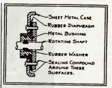
Fig. 3—Gland construction for sealing a sheet-metal panel
