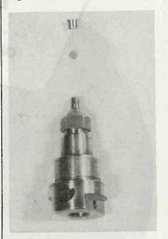
Adjustable high-magnification specimen holder. Above it are the specimen screen and screen holder cap
