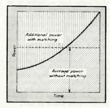
FIG. 3—In dielectric heating of thermosetting materials, power absorption increases with time because power factor increases with temperature. Continuous rematching would permit using peak power output throughout the heating cycle
