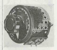
up to 135 v are obtainable with 115-v input. A new type of brush and radiator construction is used so that brushes can be changed in a few seconds. Type 60 Variac is available with or without a case. Overall height is  $4\frac{1}{6}$  in., overall diameter is  $5\frac{1}{2}$  in. Cased, the unit weighs  $3\frac{1}{2}$  lbs, and uncased 3 lbs, 2 oz.
