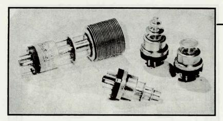
FIG. 1—Commercial disk-seal and lighthouse tubes
