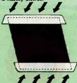
HORIZONTAL DEFLECTION — Because the blocks are free to deflect laterally, vibration and impact loads are easily absorbed. The conventional method of bonding a rubber disc to a metal ring does not provide this herizontal freedom.
