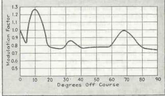
FIG. 6 (above)—Phase control unit serving the antenna system FIG. 7—Variation of modulation factor of runway localizer
