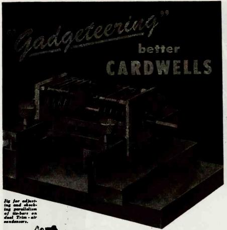
Special tools, jigs and fixtures are, in the final analysis, the key to improved quality for even the simplest devices.
