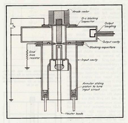
FIG. 11—Mechanical layout of a disk-seal tube circuit shows unity of the tube proper with the wave circuit
