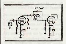
Fig. 3—This high-pass filter circuit satisfactorily attenuates frequencies below 350 cycles
