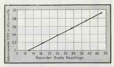
FIG. 3—Comparison of calibration over a period of four days illustrates instrument stability
