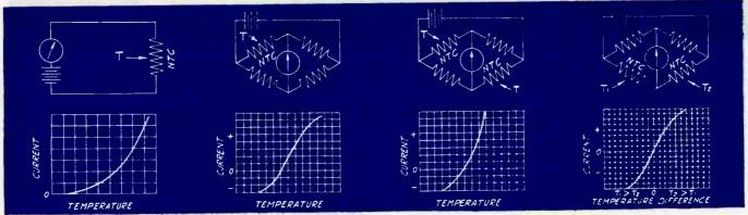
This simple series circuit of voltage source, instrument and NTC unit has been utilized to indicate engine coolant temperature, etc. It provides sufficient accuracy for many applications despite scale crowding at the bottom.
