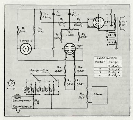
FIG. 2—Complete circuit showing component values for a four-range amplifier
