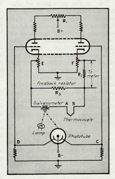
FIG. 1—Basic phototube amplifier circuit
