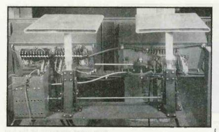
Details of rematching mechanism for 20-kw plastic preheating unit. A thyratroncontrolled motor moves the two capacitor plates towards or away from the electrodes supporting the plastic preforms
