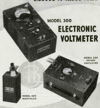
This enormous range of voltages—five hundred million to one—is accurately covered by our Model 300 Electronic Voltmeter and some of the accessories shown above. Frequency range 10 to 150,000 cycles. Accuracy 2% over most of the range. AC operation. Five decade ranges with logarithmic scale make readings especially easy. Uniform decibel scale also provided. May also be used as a highly stable amplifier, 70 DB gain, flat to 150,000 cycles.
