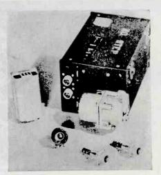
Units of the temperature control system. The electronic amplifier and infinite position motor which connects to the dampers of the plane's heaters are in the large cabinet. At left is the cabinstat, and at lower right are the outside air compensators which sense temperature changes and signal the amplifier that controls the motor delivering heat into the cabin
