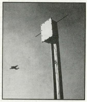
Localizer field monitor used to detect failure of on-course pattern
