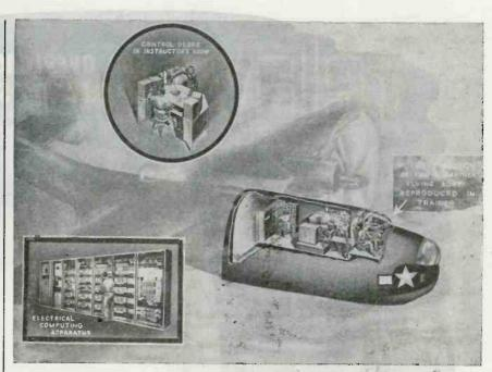
Important sections of the operational flight crew trainer used for instructing Navy airmen under operating conditions without leaving the ground. More than 200 electronic tubes and 60 electric motors are in the equipment
