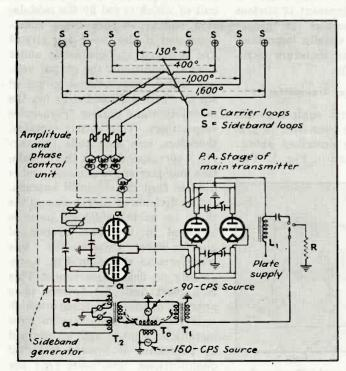
FIG. 5—Output and antenna circuits of runway localizer. Main transmitter feeds only carrier loop, with other loops being fed by the sideband generator
