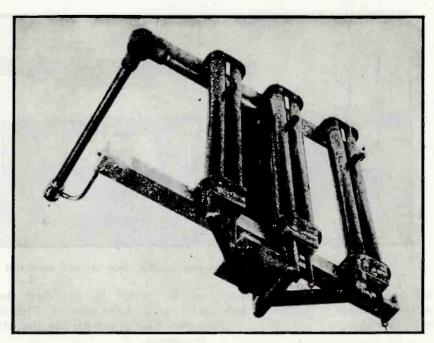
Quarter-wave transmission line transformers used as phasing controls to place all sideband antenna pairs in phase with each other and in quadrature with the carrier antenna pair of the runway localizer system
