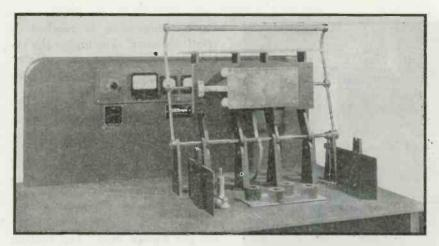
Details of working table of 5-kw unit, with four preforms in position and top electrode raised
