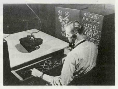
Flight problems for the crew in the electronically-equipped trainer are set up by the instructor. Values of wind velocity, direction, rough air, wing ice, etc., are determined by the knobs. Monitoring of the crew's actions is done with the aid of the indicator panel at the right and the flight recorder (called the "crab") on the desk that automatically follows the course flown
