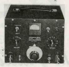
calibrated dial indicates the percentage difference between the unknown and the standard. The comparison bridge is supplied with three frequencies of 60, 1,000 and 10,000 cycles. Components being compared to a similar standard range are: capacitors 25  $\mu\mu$ f to 20  $\mu$ f; inductors 5 microhenries to 500 henries, resistors from 10 ohms to 5 megohms. The instrument measures  $10 \times 7\frac{1}{2} \times 8\frac{1}{4}$  in.
