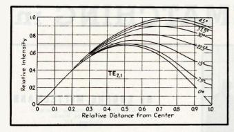
FIG. 5—This intermediate graph gives relative intensity, but not direction, of the transverse field
