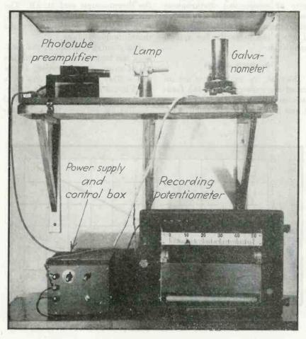
The phototube amplifier is the connecting link between a sensitive galvanometer and an electronic recorder. The optical system comprising the lamp, galvanometer mirror and phototube of the amplifier is best enclosed to eliminate stray light and temperature variations
