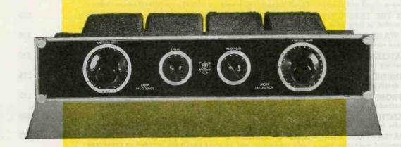
3AX ... THE UNIVERSAL EQUALIZER FOR BROADCAST AND RECORDING SERVICE. PRO-VIDES ADJUSTABLE EQUALIZATION AT 25, 50, OR 100 CYCLES FOR LOW END, AND AT 4000, 600C. 8000, OR 10,000 CYCLES AT HIGH END. CALL BRATED CONTROLS READ DIRECTLY IN DB EQUAL-IZATION AND FREQUENCY SETTING. THE INSERTION LOSS EFFECTED BY THE EQUALIZER IS COMPENSATED THROUGH SPECIAL COMPENSATING PADS, SO THAT IT IS CONSTANT REGARDLESS OF SETTING. RAPID CHANGE IN TONE COLOR CAN BE OBTAINED WITH NEGLIGIBLE CHANGE IN VOLUME
