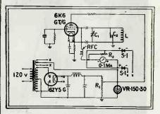
Circuit of electronic gage for measuring width of a continuous strip such as movie film
