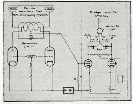
FIG. 8—Simplified schematic diagram of dielectric heating generator provided with automatic and continuous readjustment of matching between the load and the generator tank circuit
