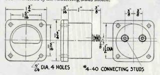
Design and development of this line of 1½" instruments were based on rigid U.S. Army Air Force specifications. They are built to withstand extreme conditions of temperature, humidity, vibration and shock, and immersion tests have demonstrated their ability to withstand a hydrostatic pressure of 14.7 psi.
