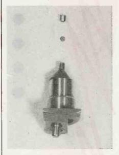
Stereo specimen holder tilted to one side for making one of a pair of stereo negatives
