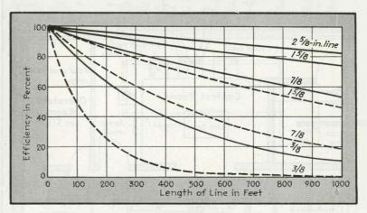
FIG. 5—Graph illustrating the percent efficiency of various sizes of coaxial transmission line using Isolantite insulation. Solid lines show efficiency at 50 Mc. Dashed lines show efficiency at 300 Mc (General Electric)
