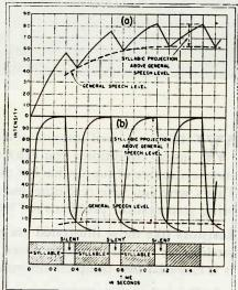
Fig. 2—Growth and decay of sound in a room (a) of 5 sec reverberation time, and (b) of 0.5 sec reverberation time show the general speech level and the syllabic projection above that level
