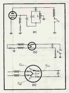
FIG. 4—At low frequencies, the lumpedconstant oscillator circuit shown at (a) can be used. At higher frequencies the line oscillator shown at (b) replaces the lumped constant oscillator. At still higher frequencies the important circuit elements lie within the tube as illustrated at (c)
