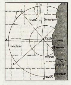
FIG. 3—Map showing predicted 1000 and 50-microvolt contours around WMFM. Radials on which signal-strength measurements were later taken are numbered
