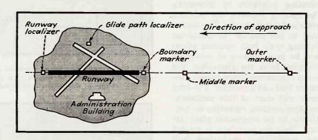
FIG. 1—Arrangement of components of CAA instrument landing system on and near a typical airport
