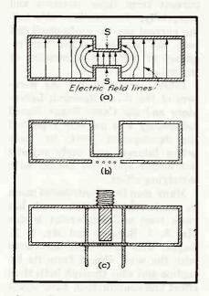
FIG. 8—The evolution of the disk-seal tube from a cavity resonator
