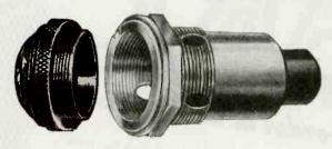
Every design detail of this Gothard Light counteracts troublesome vibration. Jewel holder is threaded into body of light and is unscrewed to permit lamp change from front of panel. Bayonet type lamps are used—accommodating a range from 6 to 24 volt ratings. The No. 1203 requires only a 1" mounting hole and mounts on panels up to 3/6" thick. Metal parts are all brass, except hex nut. Heavy plated. Available with plain, faceted or frosted jewels—in colors: red, green, amber, blue, opal
