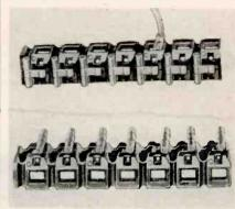
fastening device is necessary. The block may be used in place of disconnect plugs. A quick self-locking feature provides for snap-in contacts, holds the contacts firmly in position, and requires manual release by means of levers. Identification markers are clearly visible when the lever is in the locked position.
