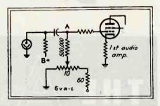
Fig. 2—Balancing arrangement for overcoming the effect of 60-cycle modulation of a light beam
