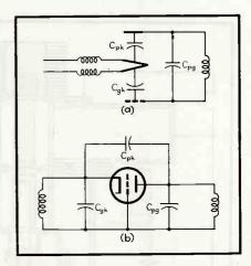
FIG. 9—The circuits used with the diskseal tube take advantage of the interelectrode capacitances shown in drawing (a) by placing them in the resonant circuits as at (b)
