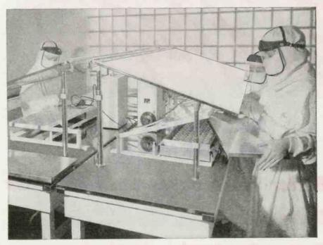
LIFE-SAVING PENICILLIN salt solution is carefully tested by battery-powered pH meters before it is placed in vials by white-clad technicians at the modern Commercial Solvents Corporation plant. Throughout the entire manufacturing process, rigid pH checks against excess acidity and alkalinity must be maintained while the penicillin is in solution.
