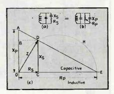
FIG. 4—Vector diagram for transformation of a series load circuit into an equivalent parallel circuit having identical power dissipation. Peak power output is delivered to the load Z as long as the loci of this vector is the circle indicated here
