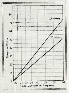
Power-current chart drawn on parabolic graph paper to provide straight lines
