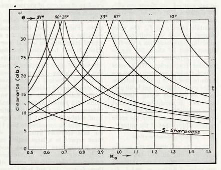
FIG. 9—Variation of clearance with sideband current in carrier loops
