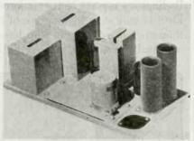
db. It employs input stage mixing, and is intended for public address installations. Type 102-C consists of a three-stage amplifier, fixed gain, adjustable, 75/85/95 db. Type 102-D is a two-stage amplifier with fixed gain of 61 db with 600 ohms input impedance, and 45 db bridging also with 600 ohms input impedance.
