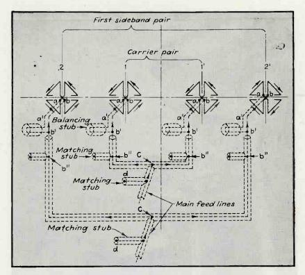
FIG. 3—Schematic diagram showing general arrangement of the first two pairs of antenna circuits associated with the runway localizer
