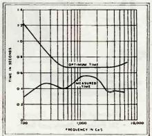
Fig. 5—Optimum and measured reverberation times for the room of Fig. 1 as a function of frequency
