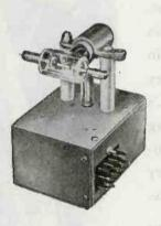
pole which handles high-voltage r-f currents by means of a vacuum switch. All high-voltage parts are rounded to reduce corona.
