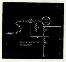
Cathode-follower circuit for use in vtvm to eliminate the tube in the test probe
