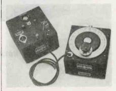
than the older type, covers a frequency range of 100 to 500 Mc, and is designed for use as a power source for laboratory measurements. Maximum output is ½ w or better over the entire frequency range. The frequency-determining element is a new type butterfly h-f tuned circuit in which the inductance and capacitance are varied simultaneously, with a single control and no electrical contact to the
