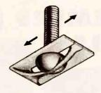
Detail shows the simple arrangement that prevents stud from turning while it permits centering in two directions. Clip is stamped from heavy gauge, cadmium plated steel.
