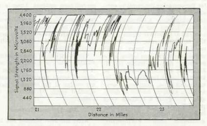
FIG. 2—Shadows such as those shown in Fig. 1 produce marked variations in signal strength, as shown on this graph obtained by continuous recording while driving through a hilly area
