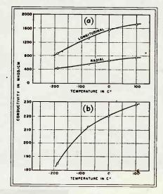
(a) Electrical conductivity of graphite vs temperature. (b) Electrical conductivity of carbon vs temperature
