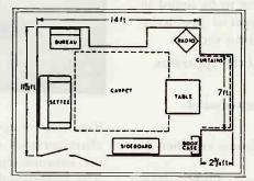
Fig. 1—Walls of this room used for acoustic measurements were distempered and the floor was covered with linoleum
