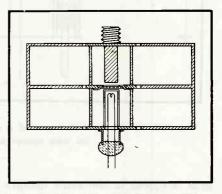
FIG. 10—The disk-seal tube and resonator equivalent of the lumped-constant circuit shown at Fig. 9 (b)
