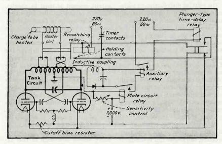
FIG. 5—Simplified schematic diagram of induction heating unit providing one step automatic rematching of tank circuit to load. The timer contacts open momentarily at the end of the heating cycle to release the rematching relay in preparation for a new cycle
