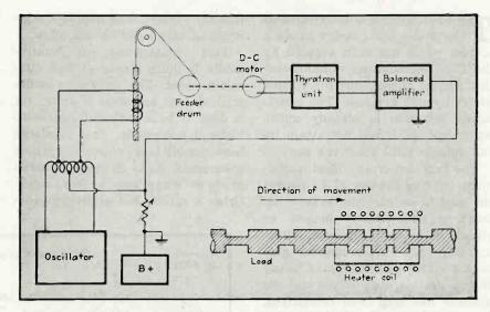
FIG. 7—Schematic diagram of electronic heating unit provided with continuous rematching equipment for heating to a constant surface temperature a moving charge of non-uniform cross-section as shown at the lower right
