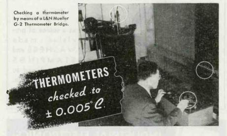
Here you see but one of the tests used in the H-B laboratories. There are many others, all made with one thought in mind—to produce precisely accurate thermometers. Typical uses of H-B precision instruments include: checking TNT setting point temperatures, the measurement of surface temperatures of gun breeches, checking hydraulic brake oils at minus 40, 50, 60 and 70° F., with mercury-thallium thermometers accurate to 0.1° F. at all points, etc. If high precision, mercury-
