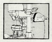
Set up to punch 3 holes simultaneously
