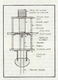
FIG. 2—Basic construction of disk-seal tube
