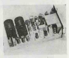
Complete chassis, including dynamotors, of the f-m transmitter and receiver designed for operation on frequencies between 70 and 200 kc
