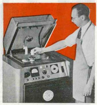
Here's the new RCA 2000-watt electronic generator designed especially for the plastics industry. One pound of molding material can be thoroughly preheated to 275°F. in about 40 seconds. Note convenience of operation: preform is placed on electrode and cover closed. Timing and cover opening are automatic.
