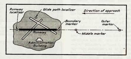
FIG. 1—Arrangement of components of CAA instrument landing system on and near α typical airport
