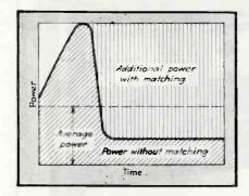
FIG. 2—Without continuous rematching of generator to load in induction heating, the total Btu of heat delivered to the charge during the heating cycle (diagonally shaded area) is only a fraction of that obtainable with the load matched at all times
