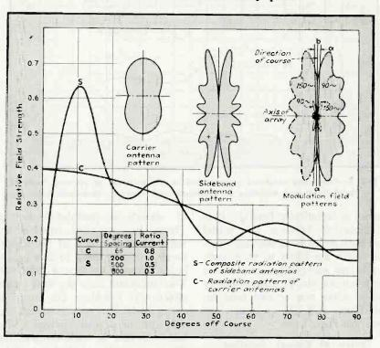
FIG. 2—Radiation patterns of the sideband and carrier antennas, plotted in both rectangular and polar coordinates
