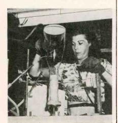
Metallic buttons are sealed-in on cathode-ray tubes at the Dobbs Ferry plant of North American Philips. The operator controls the air pressure in the tube with her mouth while the gas burner is rotated around the button
