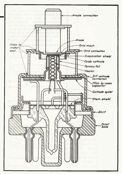
FIG. 3-Mechanical details of the 2C40 lighthouse tube
