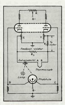
FIG. 1-Basic phototube amplifier circuit
