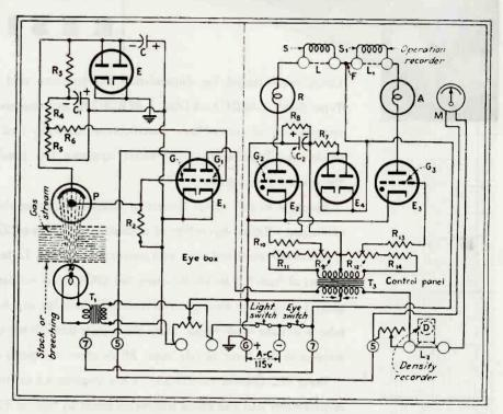
FIG. 1—Complete electronic circuit of a smoke density indicator. Recording equipment may be used with the unit to show the length of time the smoke is off-color or the density of the gases
