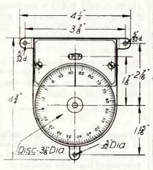
Front and side dimensions of Techrad Interpolating Counterdial
