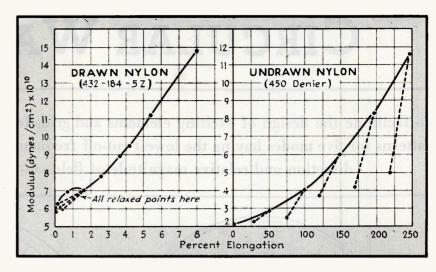
FIG. 3—Graphs showing characteristic behavior of a Nylon polymer yarn, depicting the change in modulus introduced by a drawing operation which orients the yarn and forms it into a tough resilient material
