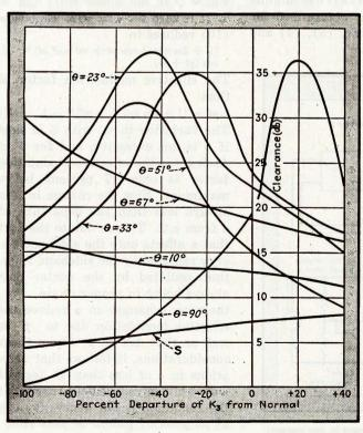
FIG. 11-Variation of clearance with current in outer pair
