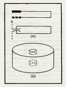
FIG. 6—Choosing a different axis of revolution from that of Fig. 5 for the equivalent circuit at (a) gives the mechanical arrangement at (b) which readily lends itself to use as the electromagnetic basis of the disk-seal tube; the electrodes for the electronic system go at the center
