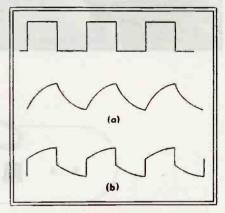
Square-wave modulation signal is reproduced by an a-m system involving a resonant circuit as at (a), and by an f-m system containing the same resonant circuit as at (b)
