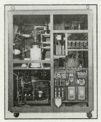
Rear view of generator. Oscillator compartment, with two air-cooled transmitting tubes, is at upper left, with blower just below. Motor-driven Variac transformer for adjusting filament voltage is in approximate center of unit. Peak output of this unit is 20 kw
