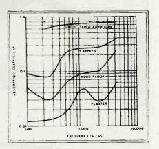
Fig. 4-Absorption coefficients of typical domestic surface materials
