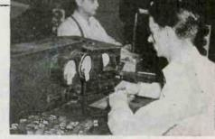
Each Mallery Vibrator is tested on the oscilloscope for wave form under all operating conditions to insure precise performance.
