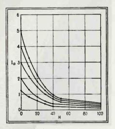
Four curves plotted at different anode voltages for anode current versus H. the magnetic intensity
