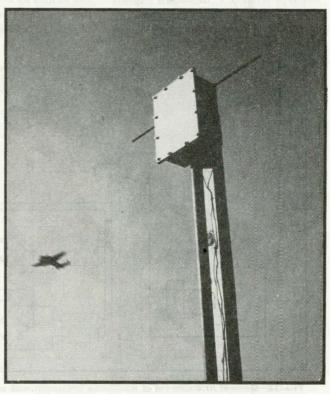
Localizer field monitor used to detect failure of on-course pattern
