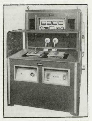
Electronic generator with continuous rematching equipment, developed for dielectric heating of large plastic preforms involving a load weighing from 3 to 12 pounds and varying in both power factor and dielectric constant during the heating cycle
