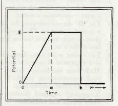
Applied voltage versus time for third illustrative example of Laplace transform
