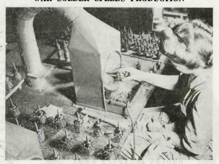
Wire loops on small armatures having their Formex insulation burned off at the same time they are tinned in one Fairchild plant. This is accomplished by heating 60-40 solder to 1,000 deg. F in an electrically-heated pot. The operation formerly required burning off the insulation in an alcohol-lamp flame and wire-brushing before soldering. This took three times as long as the present technique using the war solder
