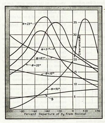
FIG. 11-Variation of clearance with current in outer pair
