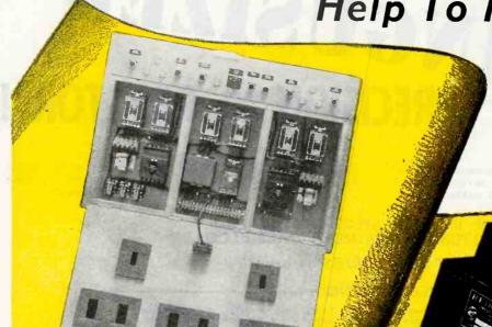
Open view of ATC Automatic Time Control Panel Showing HEINEMANN Circuit Breakers in Place
