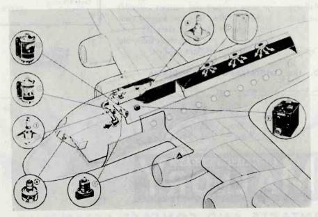
Hiustrating the location of units of the Minneapolis-Honeywell electronic cabin temperature control system for planes, as installed on a C-54
