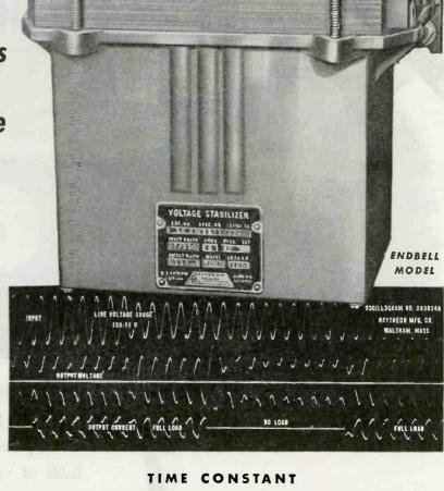
Transient changes in output voltage result from variations in line voltage. These transients disappear entirely in 6 cycles. The major effect of the transient recovery is practically complete in 2 cycles. These changes are not evidenced on a volt meter of normal characteristics
