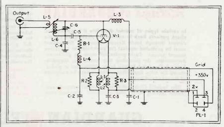
Schematic of v-h-f oscillator that contains the butterfly circuit for tuning from 100 to 500 Mc without sliding contacts
