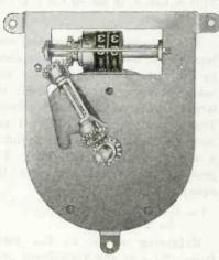
Rear view construction of Techrad Interpolating Counterdial
