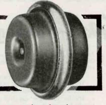
G-E Safety Spark Gaps are used for protection of condensers and other equipment against high-voltage surges. These spark gaps are of the metal-to-glass sealed gas-filled type. They are designed to perform satisfactorily over a wide range of temperatures. G-E Spark Gap ratings are 1200- and 2200-volts  $\pm 10\%$ . They're available with or without mounting brackets.
