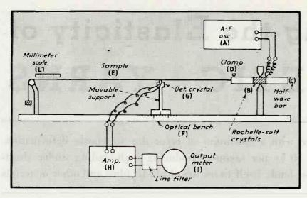
FIG. 1—Schematic of the setup used to measure the elasticity of synthetic yarns and plastic films by a method described in the text. A photograph of the equipment appears on the preceding page
