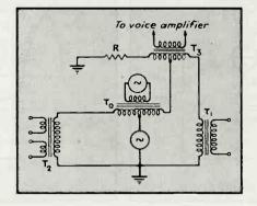
FIG. 8—Hybrid unit used with voice channel to give verbal instructions to incoming pilots over runway localizer radio system
