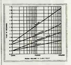
Fig. 3—Subjectively determined optimum reverberation times for different types of sound in various sizes of rooms
