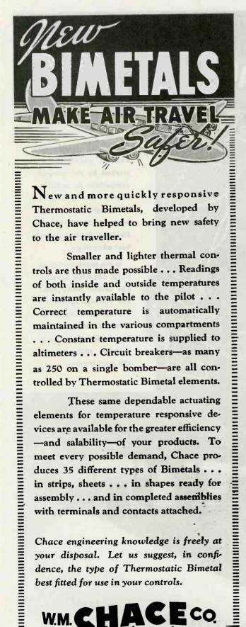
New and more quickly responsive Thermostatic Bimetals, developed by Chace, have helped to bring new safety to the air traveller.
