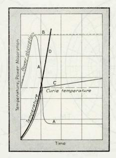
FIG. 1—Variation of power absorption and temperature of a ferromagnetic charge with time during the heating cycle, assuming constant current through heater coil
