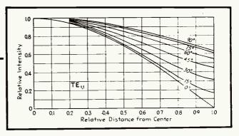
FIG. 3—As an aid to plotting relative transverse field intensity. this intermediate graph is used
