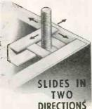
In position for mounting, the stud can be moved (NOT BENT) in FOUR directions to align with poorly spaced holes. Strains applied to stud through excessive tightening are absorbed by mount.
