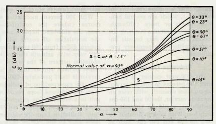
FIG. 10-Variation of clearance with phase of carrier loop current
