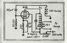
Fig. 1—Circuit of self-excited oscillator for supplying current to a 6-watt exciter lamp
