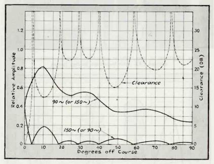
FIG. 4—Composite sideband pattern due to all radiators of runway localizer (solid lines) and variation of clearance with azimuth (dash-dash lines)
