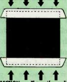
VERTICAL DEFLECTION — The uniform distribution of leading over the entire surface of the rubber block eliminates concentrated tensile or shearing stresses. Long service life is thereby assured.
