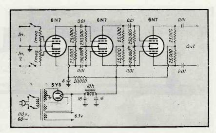
FIG. 2—Circuit of the audio amplifier employed. Only one channel was used in the experiments described. The second channel was provided to facilitate a proposed direct-reading scheme utilizing a phase-meter
