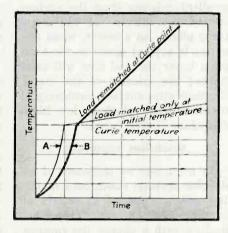
FIG. 6—Time-temperature curves for two high-frequency generators used for induction heating. The smaller unit with rematching (B) reaches temperatures above the Curie point much faster than generator A which has twice the output rating of B
