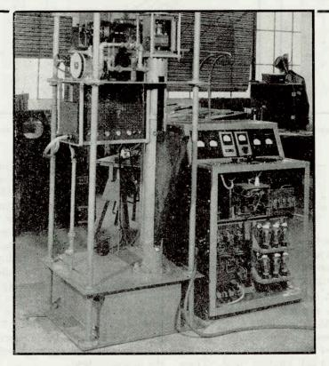
Continuous rematching equipment developed for heating a moving charge having a non-uniform cross-section, such as rifling broaches
