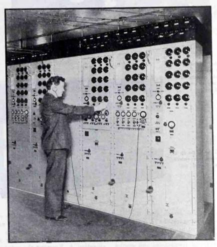
Racks of receivers used for diversity reception at high frequencies in the RCA receiving station at Riverhead, N.Y.
