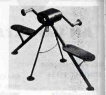
hand-generator which requires at outside electricity to operate. The cranks have been improved to prevent breakage due to operational leakage. A shatterproof unit enclosed with the meter, tells the operators when the output is being held to the correct value.
