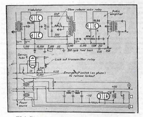
FIG. 8-Ship transmitter modulator circuit and audio amplifier circuits
