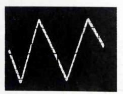
FIG. 4—Output wave form of the 400cps pyramid oscillator used to modulate the f-m signal generator
