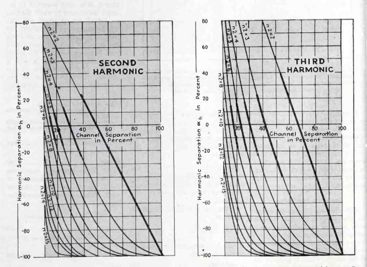
FIG. 2—General design work sheets showing the separation between a harmonic and the channels as a function of the separation of the channels themselves. Curves are plotted for systems up to fifteen channels; thus, the curve n2 = 6 is for a six-channel system. The heavy-line portion of each curve indicates the cyclic variation of the optimum channel separation
