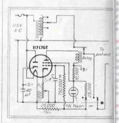
Circuit of electronic timer for control of therapeutic electric shocks. The neon bulb is used as a voltage stabilizer in the screen-grid circuit
