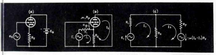
FIG. 1—(a) The actual circuit in which the impedance across  $R_2$  is sought. In (b) a fictitious generator,  $E_1$ , of internal impedance  $R_1$ , is introduced. The equivalent circuit from which the derivation begins is shown at (c)
