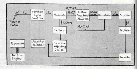
FIG. 2-Block diagram of the analyzer circuit
