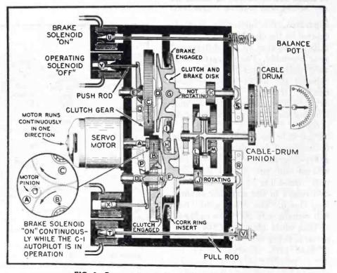
FIG. 6—Power transmission system of a servo unit
