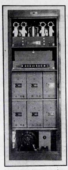
FIG. 4—Ship radio equipment, shown with the front door removed. The sixfrequency crystal-controlled transmitter is at the top. Immediately below is the modulator and relay assembly. Occupying most of the space in the cabinet are six receivers. The transmitter voltage is supplied by the dynamotor at the bottom. The selective ringer is mounted on the inside of the cabinet door. Meter jacks, fuse clips and adjusting screws are at the front of each unit to facilitate
