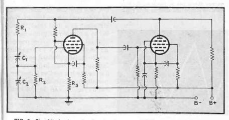
FIG. 2—Simplified schematic showing the type of *R*-C oscillator circuit used to obtain 400-cps modulation of the 455-kc amplitude-modulated signal generator. A similar R-C circuit is used as the frequency-modulated signal generator
