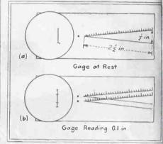
Gage for reading displacement of vibrating equipment and components. Made of fiber or plastic, it measures displacements from 0.005 to 0.3 in.
