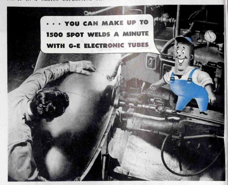
HIGH-SPEED PRECISION WELDING IS MADE POSSIBLE BY THE G-E IGNITRON AND THE G-E THYRATRON
