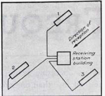
FIG. 4—A space diversity antenna layout. Three directive antennas (shown as rectangles) are placed a number of wavelengths apart, at the corners of an isoeceles triangle
