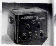
100-kc and 10-kc intervals. It operates from 60 cps, 115 v line. The unit is housed in a sturdy metal cabinet.
