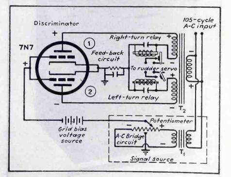
FIG. 2—Simplified schematic diagram of the discriminator circuit used in a single channel of the autoplifot amplifier. Two signals, differing in phase by 180 degrees, may enter this stage from the a-c bridge circuit: one makes the right-turn relay operate, and the other makes the left-turn relay operate
