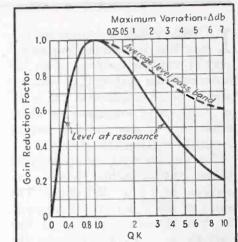
Find k and gain at resonance to give a compromise between gain and selectivity. Determine the gain at bandwidths of 10, 25, 50 and 75 kc.
