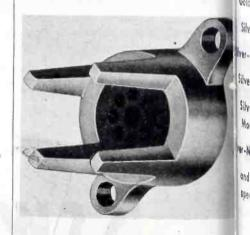
The tube pin straighteners for miniature tubes also have a zinc base alloy. The inserts are made of either hardened tool steel or of stainless steel.
