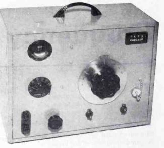
$\begin{array}{l} \operatorname{Coil} Q = \binom{F_r}{F_r - F_0} \binom{F_0}{F_r + F_0} \left( \sqrt{\frac{E_r^2 - E_0^2}{E_0^2}} \right) \\ \text{where } F_r \text{ and } E_r \text{ are the resonant} \\ \text{frequency and voltage respectively} \\ \text{and } F_0 \text{ and } E_0 \text{ are the off-resonant} \\ \text{frequency and voltage respectively.} \end{array}$
