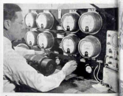
Test panel for Westinghouse dynamotors having four separate output voltages from 14 to 300 volts. Output voltages are held constant for normal input-voltage variations by a regulator field which weakens when the input voltage rises and strengthene when the voltage drops
