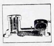
An air operated collet holding fixture for precision chucking or machine tools
