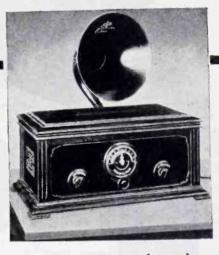
Another important step forward was achieved with this first single-dial radio produced by Magnavox in 1923. Its importance at the time is appreciated when we remember that all previous radio sets required the use of three dials for tuning in a station.
