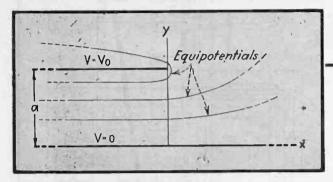
FIG. 1—Situation adjacent to one infinite and one semiinfinite capacitor plate in space. Note that equipotential contours tend toward a curved-edge plate, above
