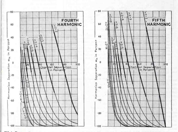
FIG. 3—These are the same type curves as in Fig. 2, but for higher harmonics. Over the heavy portion of each curve, harmonic to channel separation is small. Beyond the heavy-line regions, channel separation is either dangerously small or unnecessarily large. The end points of the heavy lines locate the optimum channel separations, a compromise between channel and harmonic interference
