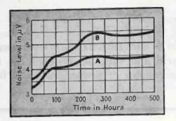
FIG. 4—Noise level vs. number of hours of continuous operation for a triodeconnected 6SJ7 tube. Curve A—40 μμf in grid circuit; curve B—40 μμf in parallel with 35 meg in grid circuit
