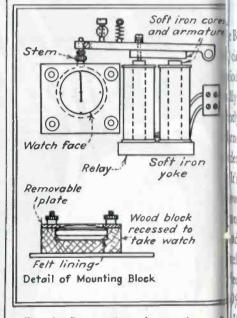
Fig. 3-Construction of mounting unit for adapting a standard stop-watch to an electronic starter
