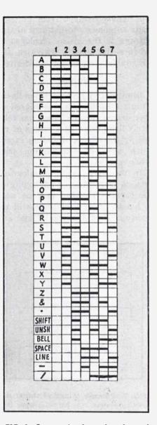
FIG. 8-Seven-unit telegraph code used to prevent printing of wrong letters due signal malformation
