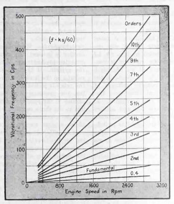
FIG. 1—Curves showing vibration frequency for various "orders" discussed in the text as engine speed varies
