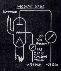
Circuit shows operation of the VG-54 which is essentially a triode vacuum tube. Emmission current from cathode ionizes gas molecules in tube by electron bombardment. Number of ions flowing to negative electrode is a measure of gas present, and hence of vacuum pressure.
