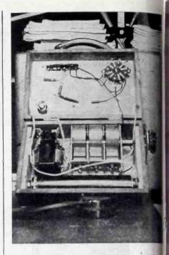
With components mounted in a wooden box, the capacitance bridge can be carried to the car to check the antenna and back to the bench for substitution of the correct capacitance
