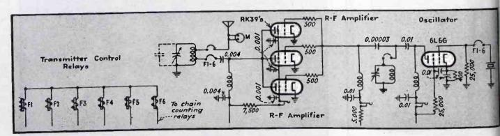
FIG. 5-Six-frequency ship transmitter circuit. Capacitance coupling between oscillator and final reduces the number of tuned circuits which must be switched. The frequencyselector relays are actuated from the chain-counting relays on the modulator chassis
