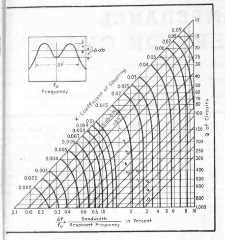
asilable Q, the required Qk is demined from Fig. 1, and thus the ue of k is found. If attenuation a specific point has been the dem criterion, the resulting  $\Delta db$ be determined from Fig. 2.
