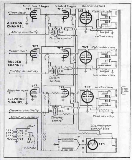
FIG. 5-Schematic diagram of 7-tube amplifier serving all three channels
