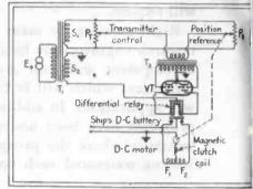
Fig. 2—Circuit of vacuum-tube system using an a-c bridge and relay for positioning control
