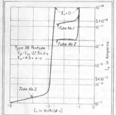
Fig. 6—Curves of grid current obtained from three tubes of the same type
