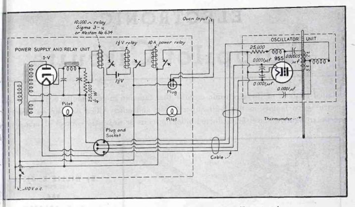
FIG. 1—Circuit diagram of the electronic control device. It is readily constructed from parts available in most laboratories and is relatively simple to adjust
