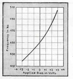
FIG. 3—Variation in f-m oscillator frequency around the 455-kc mean-frequency obtainable by changing the bias on a resistance-tube used as  $R_2$  in Fig. 2
