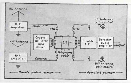
FIG. 9-Block diagram of shore station remote-control receiver.
