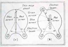
FIG. 1 (a)—Arrangement of phosphor coatings in the new television tube for a two-color system. (b) A ridged back on the screen provides two surfaces on one side of the screen for a three-color system
