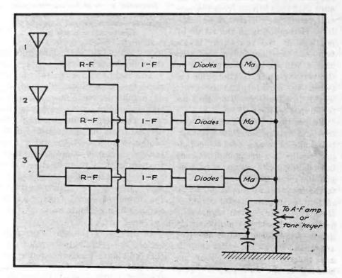
FIG. 5—In this space diversity reception system the rectified output of three receivers is combined, operating the keyer and also supplying blue for automatic gain control
