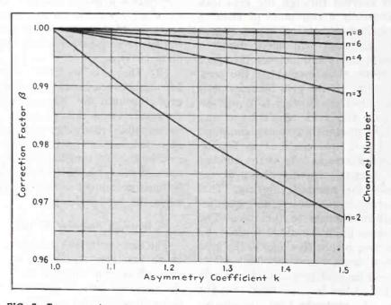
FIG. 7—To correct for selector response dissymmetry the factors given above for asymmetry coefficients through 1.5 and channels up to eight are applied to the optimum channel multipliers given in Table 1
