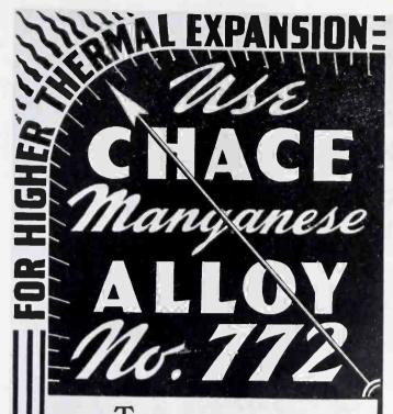
THE temperature coefficient of expansion of Chace Manganese Alloy No. 772 is twice as great as that of ordinary steel ... considerably higher than aluminum, particularly at elevated temperatures ... and far beyond that of any other strong alloy. Its expansion rate is independent of thermal treatment, and is not altered by cooling to .100° F. Thus it makes possible unusual differential expansion designs.
