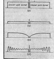
FIG. 1—A typical interference pattern, showing areas or bands of maximum and minimum field intensity. Antennas arranged for space diversity reception are shown as boxes FIG, 2—General types of fading: (a) normal signal; (b) distortionless and non-selective fade; (c) selective fading of a carrier; (d) selective fading of sidebands
