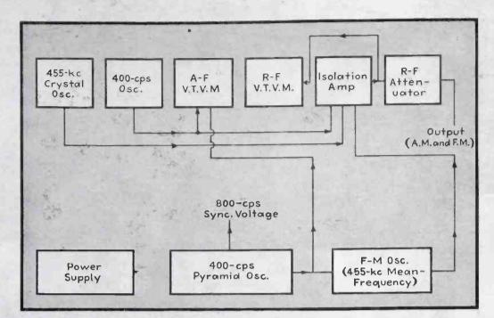
FIG. 1-Block diagram of the test unit, shown without switching. A complete schematic is given in Fig. 5
