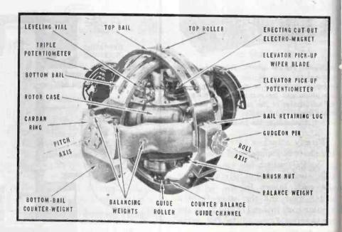
Vertical gyro of autopilot, with housing removed to show the erecting mechanism that keeps the gyro lined up with the pull of gravity despite rotation of the earth. The gyro rotor is a cup-shaped mass surrounding and driven by an electric motor in the center of the assembly
