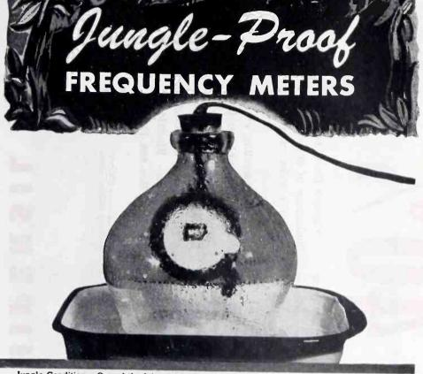
Jungle Conditions—One of the laboratory tests simulating field use is a minimum run of 120 hours at 120° F, 95 RH. Component parts have previously been tested at 180° F.
