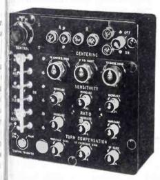
utopilot control panel, mounted within onvenient reach of the pilot. With the utopilot in control at any given altitude, he plane can be maneuvered by fingerp adjustment of the turn-control and eleator knobs or by similar remotely located knobs near the bombgrdier
