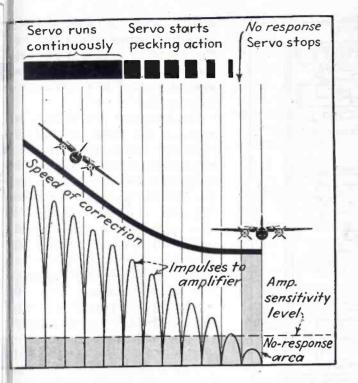
13. 4—Curve showing how speed-ofrection decreases as plane returns to right-and-level flight after an extreme deviation
