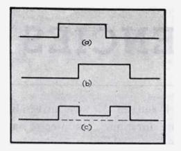
FIG. 3—A "split", showing the effect of multi-path propagation on the formation of a high-speed telegraph dot. (a) The first signal received; (b) the delayed ray signal; (c) the resultant
