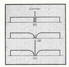
FIG. 7—Principle of exalted carrier receiving system. (a) normal signal; (b) selective fade of carrier; (c) carrier exalted or reinforced at the receiver
