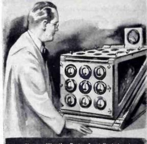
Simpson Vibration Test — Specially designed equipment provides rapid movement of instruments in three different planes. Variable speed regulator permits vibration of any desired intensity.
