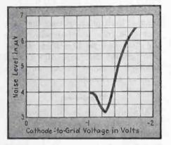
FIG. 1—Noise level vs. cathode-to-grid voltage for a 6SJ7 tube connected as a triode, with 40  $\mu\mu$ f in the grid circuit to simulate a high-impedance crystal pickup having no shunt resistance
