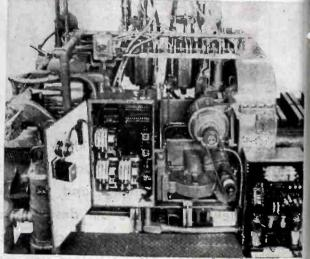
Close-up of G-E Thy-mo-trol panel and a-c magnetic controller (at left, door open) on the milling machine. The control panel at right without cover is for the 2-hp motor (center) which drives the carriage feed
