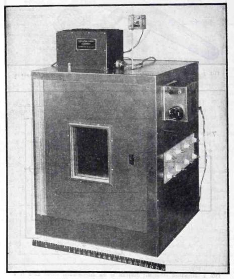
FIG. 3—A typical laboratory oven, showing the two-unit electronic control in position on the top, operating in this instance as a safety control supplementing standard controls
