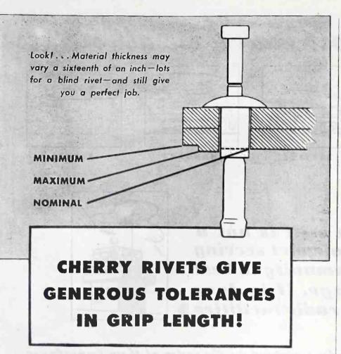
Don't hesitate to use blind rivets just because the materials used may vary slightly in thickness in different areas. Use Cherry Rivets. As long as you stay within the generous tolerances specified, you'll get a good finished job.
