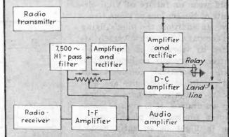
FIG. 10—Frequency-controlled heterodyne oscillator produces two signals, equal in the presence of noise, unequal in the presence of a modulated carrier in this noise-discriminating volce-controlled terminal-relay used in shore stations
