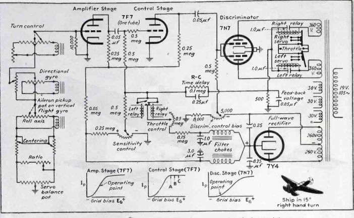
FIG. 3—Complete schematic circuit for the aileron control channel, with characteristic curves showing operating points of the tubes. The complete a-c bridge network for this channel, at the left, provides the required interlocking with other channels for properly co-ordinated turns
