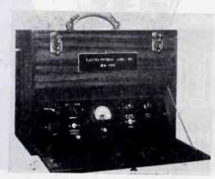
comes supplied with an amplifier and recorder which will give a graphic record between 0.1 and 80 cps at a sensitivity of 1 millivolt and 2 cm total deflection or a range from zero to 80 cycles for 60 millivolts and 2 cm deflection. A high speed writer can be supplied which will extend the frequency range to approximately 200 cycles. The phase correction is such that perfect square-wave response from 0.5 to 80 cycles is realized with the one-millivolt sensitivity connection.
