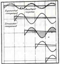
FIG. 11 (above)-Responses to component voltage waves of a controlled gaseous rectifier, for an inductive load
