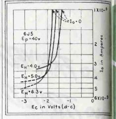
Fig. 2—Grid-current curves of a 615 tube with 40 volts applied to the plate
