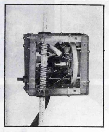
FIG. 2-Close-up of the oscillator unit, shown with the front cover removed. It is light in weight and readily supported by the thermometer which passes through it
