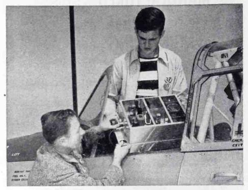
THE RADIO FLIGHT REPORTER accurately supplements test-pilot observations on performances of new planes. From a 70-point system of gauges, vibration, strain and engine performance readings are flashed to the ground receiver. When this amazing device was developed by Consolidated Vultee, the *portable* power was supplied by Burgess Batteries, used in all laboratory testing and development work at Vultee Field.
