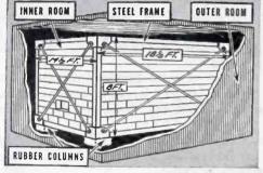
**SOUND-PROOF ROOM**—Floor and ceiling are of reinforced concrete, with walls a double layer of concrete blocks laid with no coincident joints. Special U.S. engineered rubber was selected to support this structure after comparative tests.
