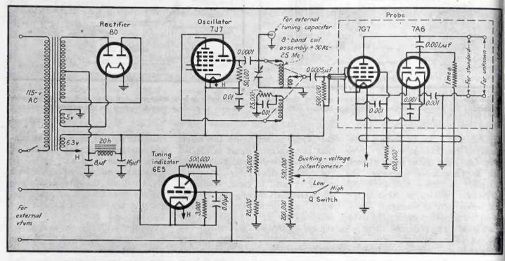
FIG. 1—Wiring diagram of the circuit-constant checker. Resonant tank for capacitance measurements and capaci-
