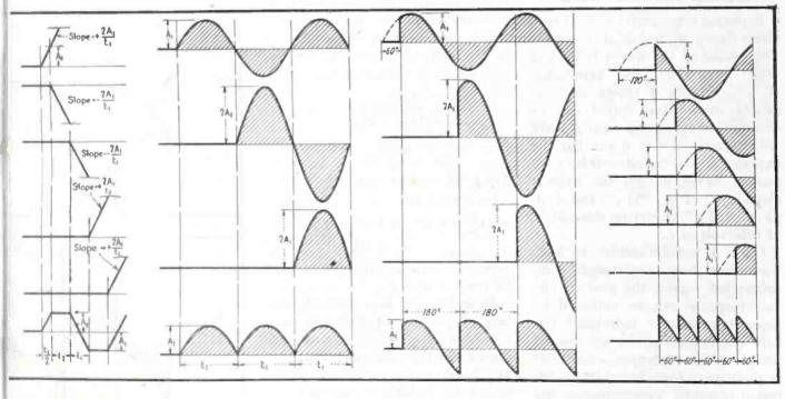
FIG. 5-Decomposition of trapezoidal waves. Components are cut off here to conserve space FIG. 6—Decomposition of output voltage of biphase uncontrolled rectifier; no phase retard FIG. 7—Decomposition of output voltage of biphase rectifier, phase retarded 60 degrees FIG. 8—Decomposition of output voltage of sixphase rectifier, phase retarded 60 degrees
