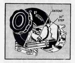
Construction of the turn control, showing the on-course detent in the cam and the 30-degree step in the cam to caution the pilot making turns requiring steeper banks
