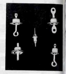
welded to a unit enclosure. Anoth feature claimed for these leads that the use of Pyrex and Kow form an absolutely gas and moi ture-tight chemical bond, so the internal gas pressure may be main tained in units using them. The bond also minimizes the stress an strain of severe temperatur changes.
