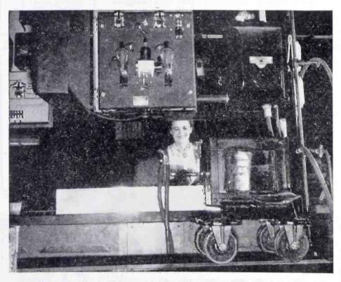
The tubes on the panel control a current impulse of 40,000 amperes for magnetizing bolts and castings. The transformer is mounted on trucks to permit short lead lengths to the test positions
