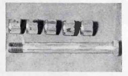
Cracks and flaws in nuts and bolts made visible by the action of heavy current from vacuum-tube rectifiers through the part under test. Iron oxide collects at the crack
