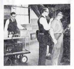
Engineers in the Du Pont plant check on the efficiency of a large suction hose used to draw off fumes during a production process. The intake hose of the analyzer is held at the operator's nose level
