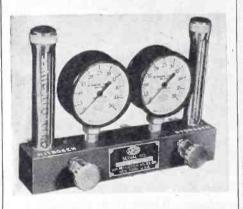
porating accurately sized orifices and on which are mounted flowmeters, pressure gauges and needle valves as well as inlet and outlet nipples. It can be furnished with any two of six available flowmeters. Flowmeters for hydrogen service cover a range of from approximately 2 to 200 cu ft per hour. For itrogen, the range is from approximately 6 to 140 cu ft per hour.
