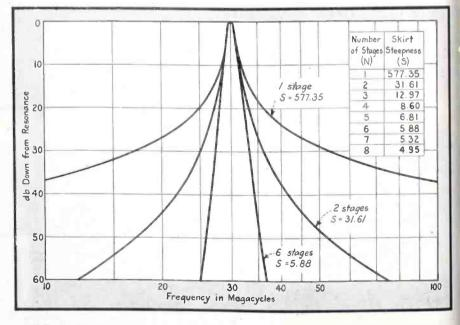
FIG. 5—Skirt steepness ratio values and response characteristics for amplifiers having different numbers of identical stages using single-Inductor coupling
