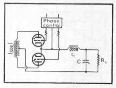
FIG. 4—Grid-controlled rectifier circuit with inductive-input filter
