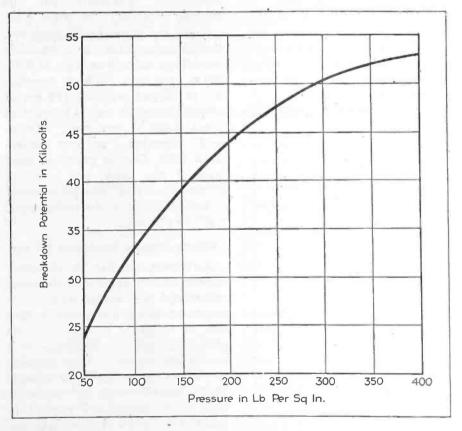
FIG. 3. Rise in breakdown potential with pressure increase in this curve results from greater opportunities for collision between a travelling electron and nitrogen molecules as more of them occupy a given space. This inhibits ionization
