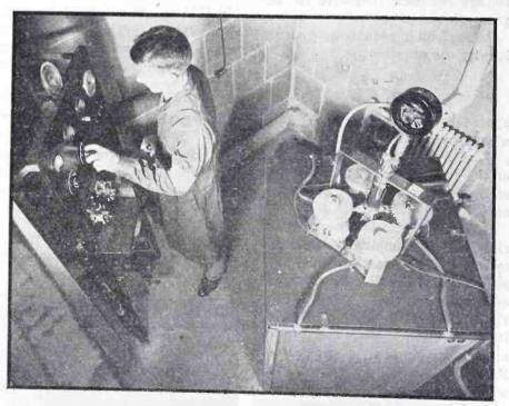
At the right are four evacuable powder cameras in position around the x-ray tube of an x-ray diffraction unit. High-voltage equipment is under the table, enclosed by metal screening. The operator is adjusting the intensity of the x-ray beam. This unit was built in Socony-Vacuum Laboratories about six years ago, but complete and versatile commercial equipment is now available
