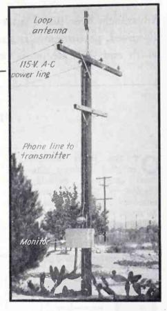
Mounted on a pole, the remote monitoring unit receives a signal from the antenna array to the right of the pole in the background and 1½ miles away. Receiver diode current goes back to the transmitter by phone line
