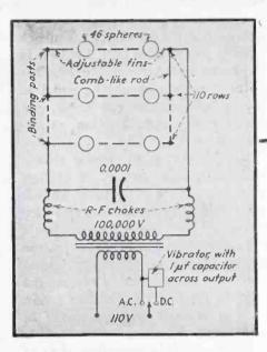
FIG. 1-Schematic of the generator
