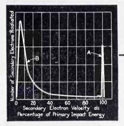
FIG. 1—Energy distribution of secondary electrons produced by the impact of primary electrons having a kinetic energy of 155 volts. The general shape of this curve holds between 20 to 10,000 volts
