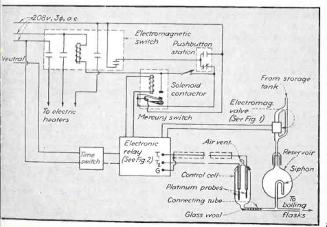
FIG. 3—Schematic of the complete still-control scheme, showing how platinum probes immersed in distilled water within the system provide the necessary conductivity path for operation of the electronic relay
