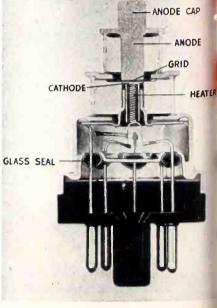
Cross-section of the new uhf tube used in military equipment
