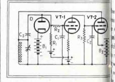
Fig. 3—Output voltage of the diode is amplified by VT-2 and applied to VToperating as an amplitude limiter
