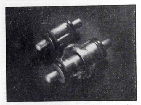
Vacuum capacitors for 7500 peak voltage in 25 and 50  $\mu\mu t$  sizes are supplied by General Electric Co. in the style at the left. Applications for the same capacitances at 16,000 peak volts are filled by the type at the right. Size comparisons with air capacitors give these units ten-to-one advantage for the same voltage rating
