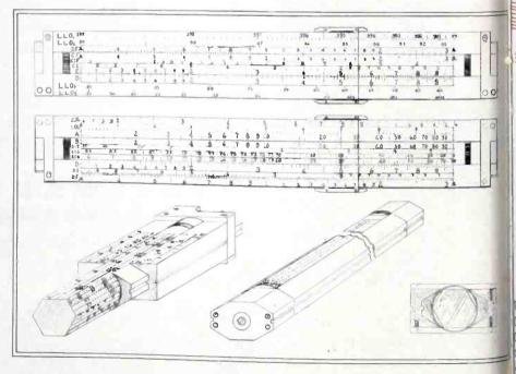
Several views of the new slide rule and its assemblies. At lower left is a section of the body of the rule, rotatable slide and housing. A cross-section is at lower right
