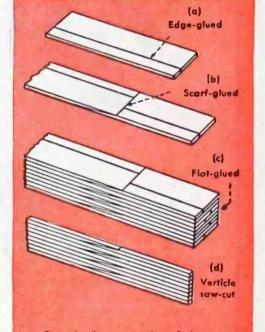
Steps in the construction of the spars: (a) edge-gluing to obtain 6-inch width, (b) scarf-gluing to obtain 16½-foot length, (c) laminating to obtain 6-inch by 6-inch by 16½-foot beam, (d) beam cut to obtain edge-grain laminated spars 3/4 inch by 6 inches by 16½ feet.
