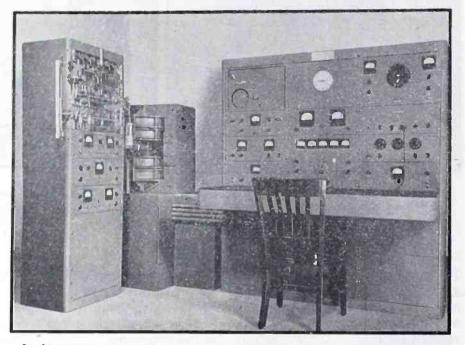
In this mass spectrometer made by Consolidated Engineering Corp., several cabinets full of electronic equipment are needed to provide an automatic record showing how many ions of each mass are present in a gas. From left to right, the cabinets contain gas introduction systems and vacuum gages; the magnet, with the mass spectrometer tube between the pole pieces; and the power supplies, ion current amplifier, recording oscillograph and automatic mass scanning device
