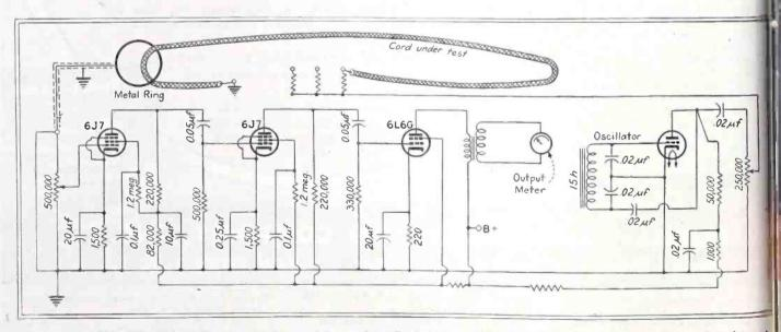
Cords and cables are tested for breaks by the amplifier and oscillator connected in the circuit shown above. The cord under test and the metal ring act as the coupling medium between the two units
