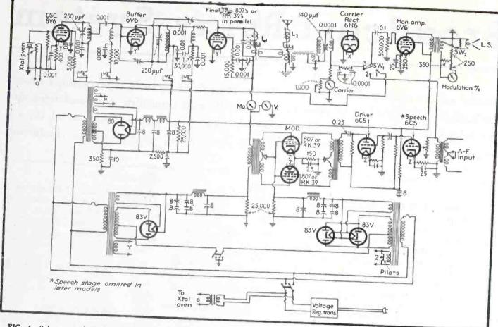
FIG. 4—Schematic of the low-power relay transmitter finally developed for use at a number of locations in British Columbia. The r-f portion of the unit may be seen at the upper left; the
