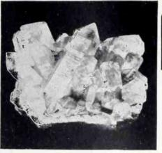
To insure constant frequency and high activity, Crystals must be cut at the correct angles to the crystallographic axes. That's why C.T.C. Crystals are X-RAY ORIENTED. This process predetermines the axes of the Crystals, making it possible to cut each slice with extreme accuracy.
