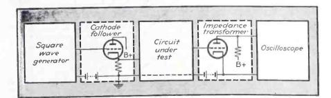
FIG. 1 (left)—Cathode follower decreases output impedance of generator while impedance transformer increases input impedance of oscilloscope in the general set-up of equipment used for square-wave testing
