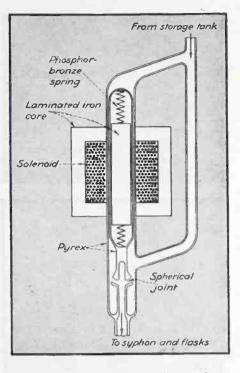
FIG. 1—Electromagnetic valve used to control the flow of water to the boiling flasks
