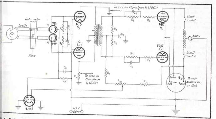
5—Basic circuit of electronic relay includes a pair of thyratrons which can be replaced with FG57 type where ige motor is required for valve operation. Light source,
