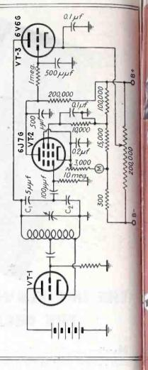
Fig. 4—Practical circuit used to hold output voltage constant on a multirange oscillator covering frequencies from 30 kc to 9 Mc. One grid and the cathode of VT-2 form the detector
