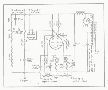
FIG. 2—Complete beam-blanking circuit, with power supply and provisions for applying a dotted "Z" timing voltage to the cathode-ray tube
