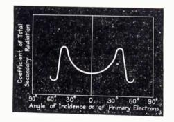
FIG. 11—Coefficient of total secondary radiation from an insulator as a function of the angle of incidence of the primary electrons. A critical angle of incidence will be observed
