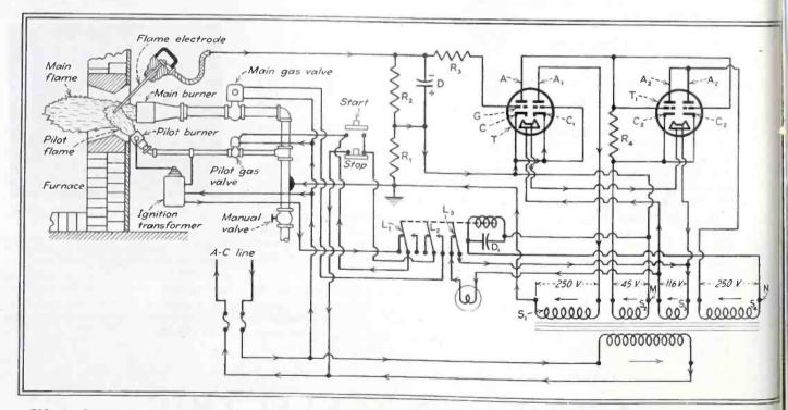
FIG. 2—Circuit of a flame protection system for a gas-fired furnace. Actuated by a flame electrode and electronic amplifier are a solenoid-operated pilot valve, main gas valve, and automatic ignition. The electronic amplifier controls the working units of both the fuel and ignition systems
