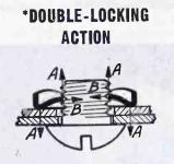
When the PALNUT is tightened, its arched, slotted jaws grip the bolt like a chuck (B-B), while spring tension is exerted upward on the bolt thread and downward on the part (A-A), securely locking both.
