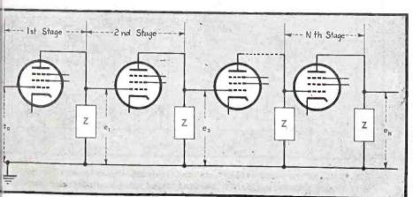
FIG. 3----Use of single-inductor coupling networks (represented by equivalent impedance Z) in N identical stages
