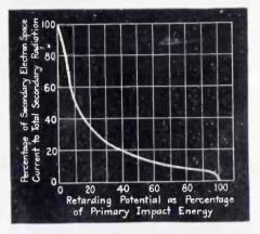
FIG. 6—Ratio of secondary electron current travelling to a collector and the total secondary radiation, plotted as a function of the retarding potential between the radiator and the collector
