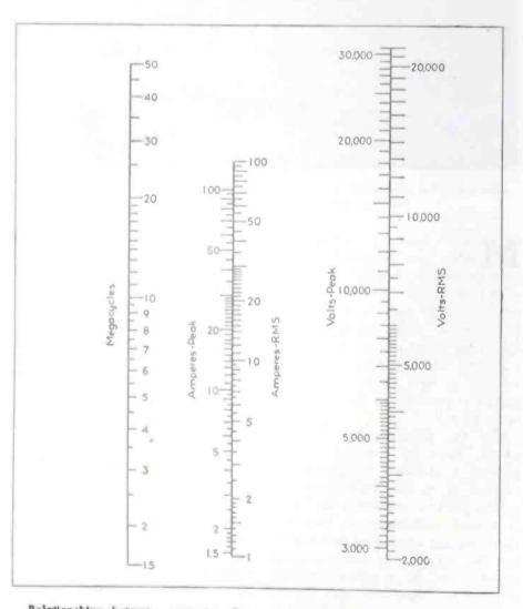
Relationships between current, voltage, and frequency for  $50\mu\mu i$  vacuum capacitors of the types in an accompanying illustration are established for reference on this nonograph. Straight line passing through any two factors reveals the third
