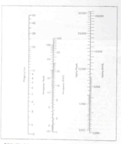
Relationships between current, voltage, and frequency for Mani vacuum capacitors of the types in an eccumpanying illustration are established for relevance on this somegraph. Scribble line passing through any two factors reveals the third
