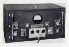
strument provides fast, easy calibration up to 2000 Mc. It may be used for calibrating wavemeters, signal generators, oscillators and receivers. The unit is equipped with transmission line output and a built-in detector unit.
