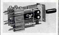
non-corrosive. The positive positioning-cam has roller detents which eliminates friction and contact bounce. Coil springs are used on both sides of the cam, so that equalized pressure is assured regardless of the number or arrange-
