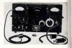
20,000 cycles may be used, adjustable from zero to 60 percent, indicated by a direct-reading modulation meter.
