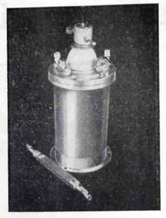
Pressurized, gas-filled capacitors made by E. F. Johnson Co. follow a basic design. Fixed and variable units both have copper-plated, drawn-steel shells in 6-in. diam. Miter-gear drive serves on variable version shown here
