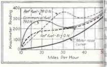
Typical knockmeter curves of unkno and reference fuels during accelerat of a 1939 Oldsmobile automobile
