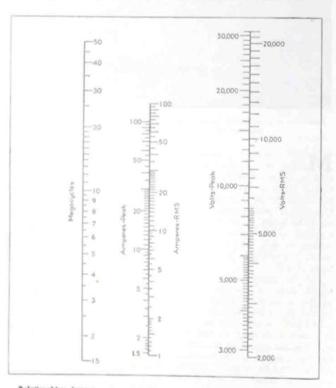
Relationships between current, voltage, and frequency for 50µµf vacuum capacitors of the types in an accompanying illustration are established for reference on this nonegraph. Straight line passing through any two factors reveals the third
