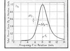
FIG. 6—Example of power response characteristic, the area of which is utilized in determining the effective bandwidth of a stage using a singleinductor coupling network
