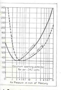
1. Curves show that sparking in air er various pressures, about parallelstates, always takes place at 342 v
