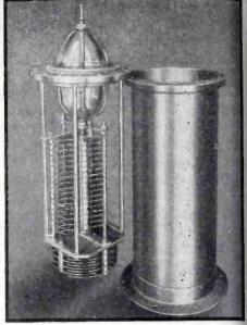
Disposition of internal elements is here illustrated for an early Johnson pressure capacitor. This type is described as partially variable. Diameter is 10 in. and the shell is thick-walled, seamless, and heavily copper plated
