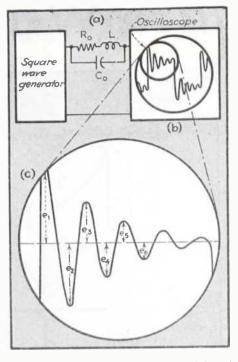
FIG. 4—Equivalent inductor circuit (a) and square-wave response (b) enlarged in (c) from which come values for determining: Natural frequency  $f_0 = nF$ , where n is the number of cycles per cycle of square wave and F is the square-wave frequency:  $R_0 = 2Lf_0 \log((e_0/e_0); C_0 = 1/[(2\pi f_0)^3L); and$
