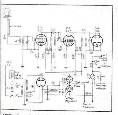
Circuit of the remote monitor. The 30-ohm rheostat in the power-transformer primary circuit reduces the line voltage to extend service life
