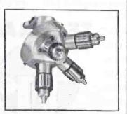
Quadrill assembly complete ready for attachment to drill press
