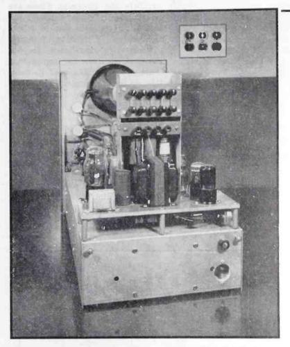
Rear view of a commercial cathode-ray oscilloscope in which the beamblanking circuit has been incorporated
