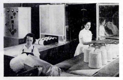
Factory layout of dielectric heating equipment used for setting the twist of rayon tire cord. The 18-lb spools of cord are wrapped in moistureproof paper for control of moisture. The operator at the right is removing plywood covers that were placed over the spools during passage through the heating chambers
