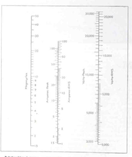
Relationships between current, voltage, and frequency for 50,441 vacuum capecitors of the types in an accompanying illustration are established for reference on this noncograph. Straight line passing through any two factors reveals the third aircraft capacitor. Absence of internal corona and stability of voltage ratings make vacuum capacitors well suited to aircraft applications.
