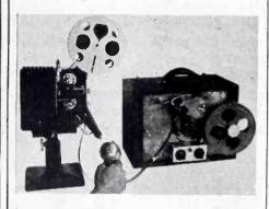
accessories. Recordings can be made on Filmgraph M-5 special film, on which a number of sound tracks (up to 40) may be recorded, or a recording may be made directly on 16 mm film. Recordings cannot be made directly on 8 mm film because the speed of 8-mm projectors is too slow for good results on this recorder. Where it is desirable to use 8-mm film, it is necessary to use Filmgraph M-5 film as an auxiliary.
