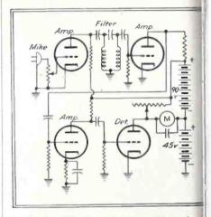
Circuit of the knockmeter used to show the relative intensity of two fuels
