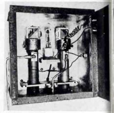
The carbon disulfide analyzer contains a mercury lamp with glass envelope removed and mounted so that its radiation is reflected down absorption tubes to photocells. The contaminated air is also supplied to one tube, then passed through activated charcoal and fed to the second tube for comparison
