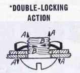
When the PALNUT is tightened, its arched, slotted jaws grip the bolt like a chuck (B-B), while spring tension is exerted upward on the bolt thread and downward on the part (A-A), securely lock, ing both.
