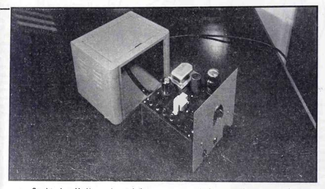
Complete beam-blanking equipment built as a separate unit for use with any oscilloscope
