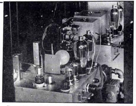
Close-up of electronic control unit. Covers have been removed from chassis in the foreground to reveal plastic bars which transmit light from the source to the rotameter glass and back to the phototubes
