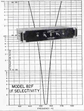
THE radio telephone receivers illustrated above are of the fixed tuned, crystal controlled, superheterodyne type, for aeronautical ground stations, airport control towers, police radio stations or point-to-point service.
