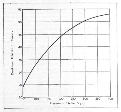
FIG. 3. Rise in breakdown potential with pressure increase in this curve results from greater opportunities for collision between a travelling electron and nitrogen molecules as more of them occupy a given space. This inhibits ionization
