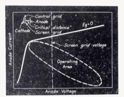
FIG. 17 — A critical - distance beamtetrode characteristic
