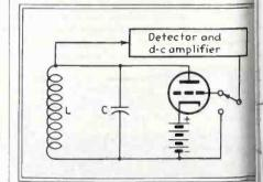
Fig. 2—Addition of an amplifier to a triode permits variations of the oscillator voltage to be detected, amplified and transmitted to the grid of the triode
