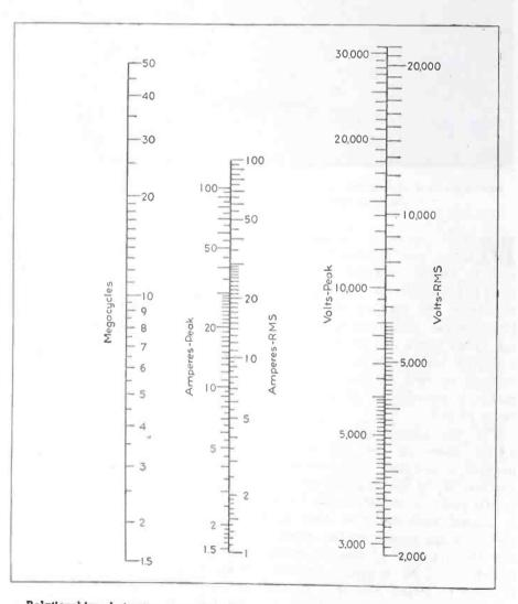
Relationships between current, voltage, and frequency for  $50\mu\mu i$  vacuum capacitors of the types in an accompanying illustration are established for reference on this nomograph. Straight line passing through any two factors reveals the third
