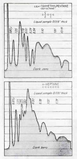
FIG. 2—Infrared absorption spectra obtained automatically with an infrared spectrograph covering the wavelength region from 7 to 10 microns, for two hydrocarbons that are difficult to separate by distillation. Characteristic absorption peaks provide positive identification of gas or liquid samples
