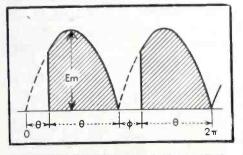
FIG. 2—Wave form for grid-controlled rectifier with no filter
