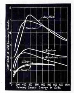
FIG. 9B—Coefficient of total secondary radiation as a function of primary impact energy for various substances
