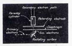
FIG, 4—The retarding potential method of arriving at the velocity distribution of secondary electrons radiated in a specific direction
