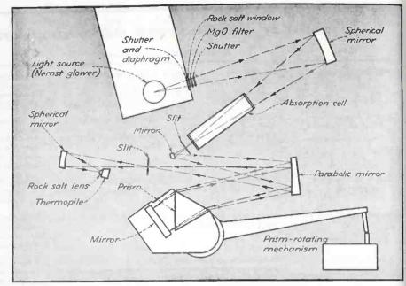
FIG. 3—Optical arrangement of infrared spectrophotometer made by National Technical Laboratories. The gaseous sample to be analyzed is placed in the absorption cell. The thermopile (or thermocouple) output is read on a sensitive galvanometer mounted in a draft and vibration-proof housing
