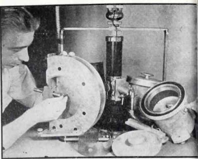
This Leeds and Northrup recording microphotometer can be used to measure the optional density of each spectral line on a photographic plate produced by an emission spectrograph
