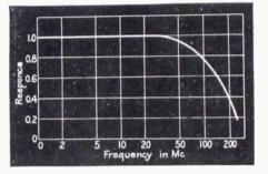
FIG. 14—Frequency response of an electron multiplier, showing fall-off at very high frequencies due to the transit angle effect illustrated in Fig. 13
