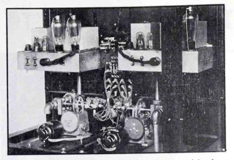
FIG. 4—In a rear view, motor drives and control valves appear below the electronic relays. Mercoid units mounted on the valve shafts include limit switches and extras which can be used to operate relays on terminal panel for automatic shut-down feature
