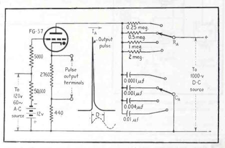
FIG. 1—Circuit used to generate pulses at high repetition rates (up to 400 per sec.), with waveform of output pulse. Performance data is in Table I
