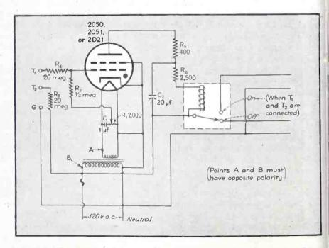
FIG. 2—Circuit of the electronic relay which operates the valve illustrated in Fig. 1 and an electromagnetic switch controlling current-flow to electric heaters beneath the boiling flasks
