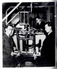
Two Chinese engineers remove the anode coil from a high-power broadcast transmitter made in England for China, while the third examines a band-change unit mounted on a turntable. Young Chinese are being trained in Britain for postwar reconstruction in their own country
