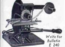
An ideal machine for hot stamping letters and figures on plastic nameplates, and other small parts, with the use of colored roll leaf. Furnished with an electric heating element, and rheostat for regulating heat. All figures and entire alphabet are on one dial.
