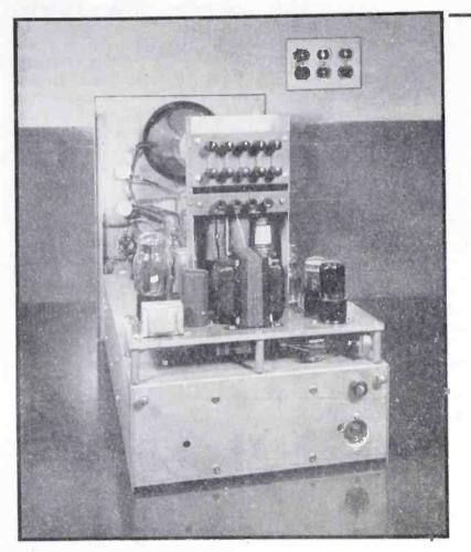
Rear view of a commercial cathode-ray oscilloscope in which the beamblanking circuit has been incorporated
