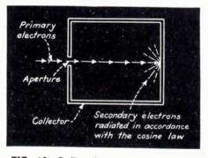
FIG. 16—A Faraday cylinder or electron trap
