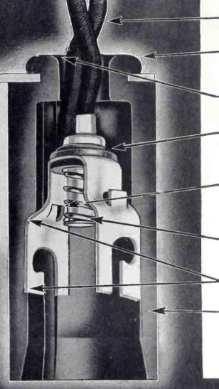
Tensile strength of leads and cannections far in excess of requirements.
