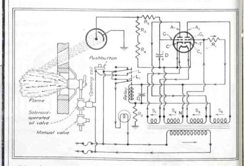
FIG, 1—Simple flame-failure system for an oll-fired furnace. A pushbutton opens a solenoid-operated fuel valve and the flame is lit manually with a torch
