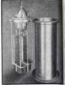
Disposition of internal elements is here illustrated for an early Johnson pressure capacitor. This type is described as partially variable. Diameter is 10 in. and the shell is thick-walled, seamless, and heavily copper plated
