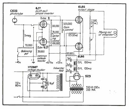
FIG. 3—Push-pull amplifier circuit used with the plethysmograph to actuate one pen of a six-channel Grass electroencephalograph
