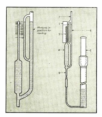
FIG. 2-The barometer vacuum or McLeod gage
