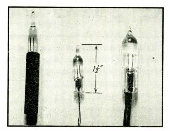
Description of a new temperature measurement and control system utilizing a resistance thermometer consisting of a small glass bulb filled with an organic material having a high temperature coefficient of resistance. Sensitivity can be adjusted for a  $\pm 0.01$  deg F control range
