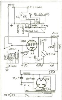
Fig. 1—Complete circuit of the electronic voltmeter using α 0.5 ma milliammeter. Voltages ranges from 1.5 to 500 volts are covered with an input resistance of one megohm per volt
