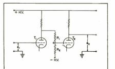
FIG. 1—Hypothetical circuit for direct coupling between two tubes
