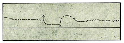
FIG. 4—Inkwriter record obtained by a Valsalva experiment with the photoelectric plethysmograph. The dip between points  $\overline{A}$  and B indicates increased congestion and corresponding higher ear density
