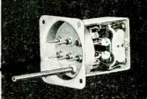
3. Relay is mounted an the base assembly and wired to the sealed terminals.
