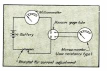
FIG. 4—Circuit for thermocouple vacuum gage
