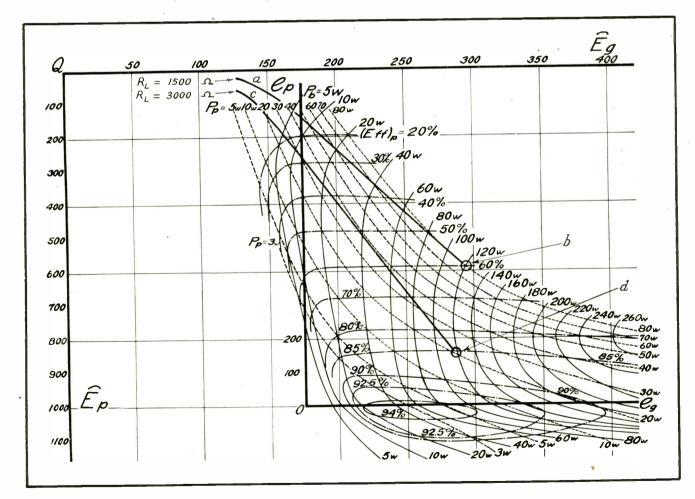
FIG. 2—Chaffee contour diagram for accurate determination of the operating characteristics of a UV211 tube when  $\overline{E}_{B}$  is 1000v and  $\overline{E}_{c}$  is — 175v
