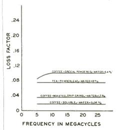
Loss factor curves for tea and three forms of coffee, ground, drip and pulverized, show that the loss factor is substantially independent of frequency
