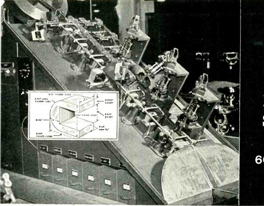
HAMILTON STANDARD PROPELLERS Rely on 14 MICRO SWITCHES to Check 602 DIMENSIONS PER MINUTE
