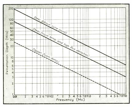
FIG. 1—Penetration depth vs. frequency for steel in the process of being hardened. A curve for copper is shown for reference
