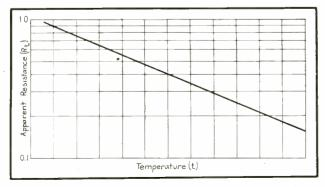
FIG. 1—Typical thermometer bulb characteristic plotted on rectangular coordinates
