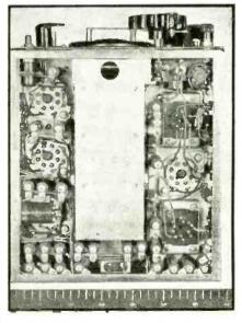
Bottom view of modern Japanese aircraft radio receiver, used with Model 99, Type 3 radio set. Note mounting of resistors in vertical positions
