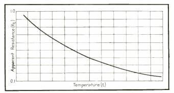
FIG. 2—Same data as in Fig. 1, plotted on semi-log paper to show linear relationship
