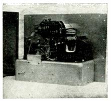
Internal view of the components and their mountings in the strain gage test set. The gain of the amplifier is adjusted by the shaft at the rear of the chassis
