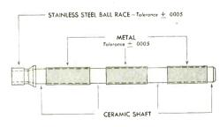
**I**LLUSTRATED is a "precision condenser" equipped with Stapakoff insulators and metallized ceramic sub-assembly. This metallized ceramic rotor shaft is only one of many extremely accurate sub-assemblies produced by Stupakoff.
