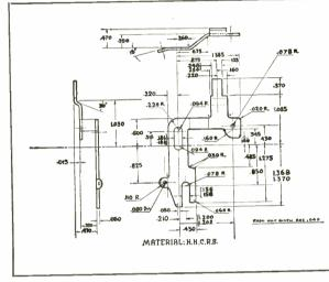
**D**<sup>IE</sup> cut metal stampings in small lots in quantities as low as 25 or 50 pieces can be produced as accurately as with permanent dies at a cost of 15% to 20% of conventional type permanent tools.
