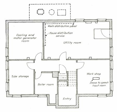
Basement floor plan of the f-m transmitter at Richfield. A work shop, boiler room, and tube storage racks are provided. Cooling equipment for the water-cooled tubes and motor generators are also housed in the basement
