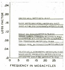
The relation between electrical loss factor and frequency is shown by the curves above for a representative selection of foods
