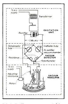
FIG. 6—Hot-filament gage connected in a bridge circuit of a vacuum regulator
