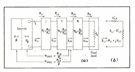
FIG. 1—Power transfer in a transmission chain connected to a nonlinear source
