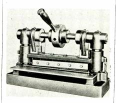
slitting and notching operations to close tolerances. Tolerance accuracy is 0.001 inches in all duplicated work. The maximum shearing width is 12 inches, and the maximum shearing capacity, for instance, on 18 gauge steel plate is
