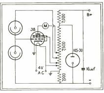
The circuit of the microdensitometer contains a 0-200 microammeter to register the unbalance of the bridge circuit formed by the phototubes. Not shown in the diagram, a 150,000-ohm resistor is in series with the meter to limit the current to slightly less than full-scale deflection of the pointer
