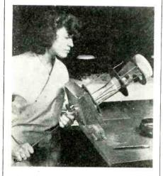
Glass bulbs for cathode-ray tubes are rotated in this jig at a constant speed while the operator moves a brush containing Aquadag up and down the vertical axis of the tube. The unit is in use at the Dobbs Ferry, N. Y. plant of North American Philips Co., Inc.
