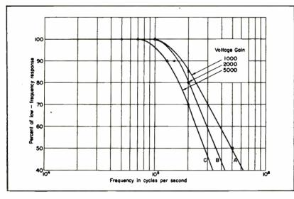
Fig. 6—High-frequency response characteristic of the amplifier
