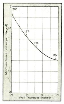
FIG. 4-Scanning speed required for hardening various wall thicknesses by self-quenching, down to 1/8-in. Numbers on curve refer to power requirement relaative to lowest
