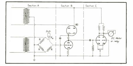
inator element which receives the a-c signal and produces a pulsating direct current flow between the plates of the two triodes to actuate either an indicating meter or a sensitive relay. This section is essentially an a-c Wheatstone bridge with one triode section serving as the variable resistance element.
