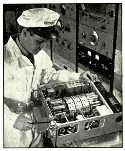
Aircraft radio mechanic adjusting a 10-frequency combination transmitter and receiver at United Air Lines' maintenance base at Cheyenne, Wyoming
