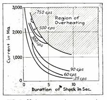
FIG. 7—Minimum currents necessary to cause death from shocks of different duration at several frequencies
