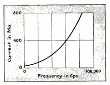
FIG. 6—Effect of frequency on tolerance current
