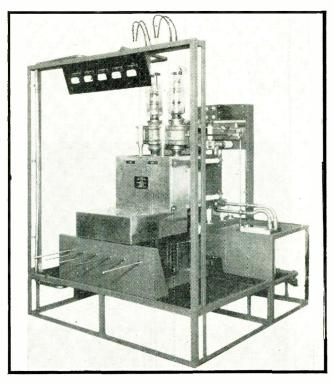
Final f-m amplifier of WMFM in Richfield. Plates are watercooled, and jets of cool air are forced around grid and filament leads. Shafts in foreground are for tuning and neutralizing
