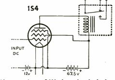
The book says a 1S4 should operate into a 5,000 ohms plate load when used with a 67.5 volt plate supply. Bear in mind that we wish to put as much power as possible into the relay under conditions of minimum signal.
