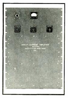
Front elevation of the oscilloscopedeflection amplifier having a voltage amplification of 5000
