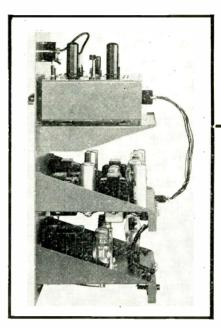
Right profile showing the arrangement of component parts and tubes in rackand-panel instrument
