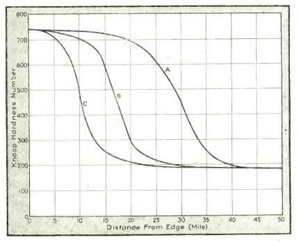
FIG. 6—Hardness traverses taken across samples of hardened 1095 steel. The sample shown by curve A required 50 kw per square inch power input, that of curve B, 30 kw and that of curve C, 15 kw per square inch of area treated at one time
