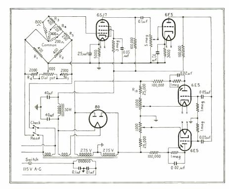
Endge circuit and electronic amplifier used to feed the grids of the 6E5 indicator tubes. The plates of these tubes are supplied with a.c. by the high-voltage winding of the power transformer
