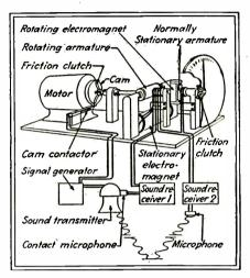
Fig. 1—Mechanical arrangement of an electronic instrument for indicating distance or depth directly on a dial. It operates by permitting impulses of reflected sound waves to determine the pointer position
