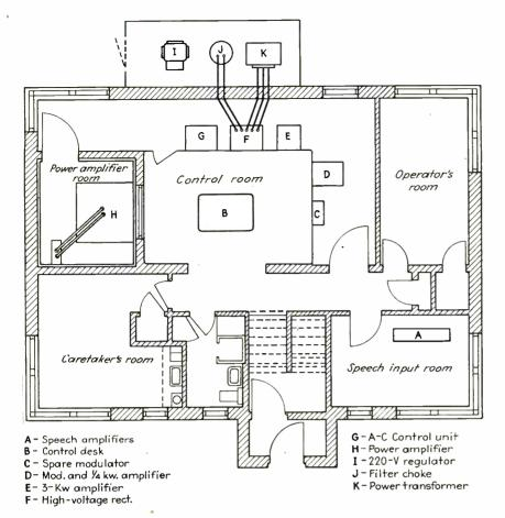
First floor plan of the f-m transmitter building at Richfield, about 12 miles from Radio City. All operating units can be seen from the control desk
