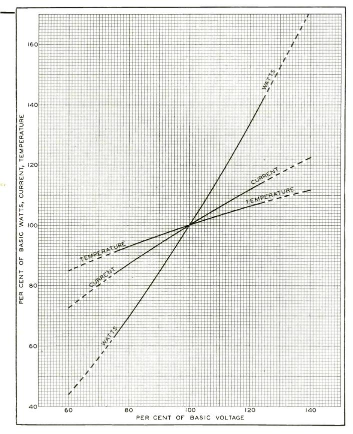
FIG. 1—Chart giving wattage, current and temperature of a filament or heater at operating voltages up to 25 percent
