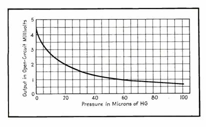
FIG. 5—Characteristic curve for a thermocouple vacuum gage
