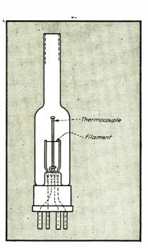
FIG. 3-Thermocouple vacuum gage tube
