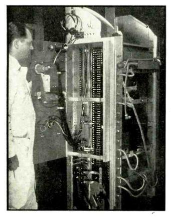
Radio rack mock-up of a Mainliner, wired so sets can be operated as in flight, to study the effects of proposed changes without holding an airplane out of service
