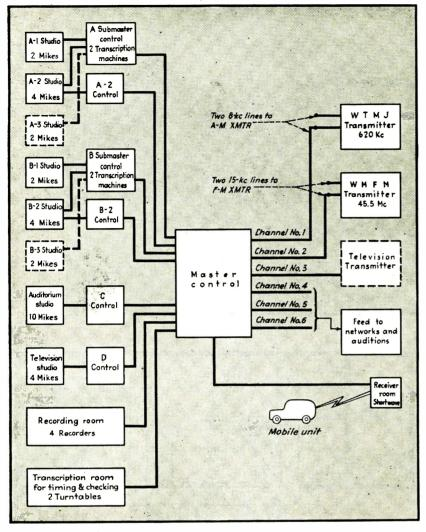
Block diagram showing arrangement of radio and audio facilities of the Milwaukee Journal, including Radio City and the various remote transmitters. Units shown dotted will provide for future expansion
