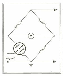
Fig. 2—Stripped to essentials, the electronic voltmeter consists of a bridge circuit in which the current flow in the milliammeter is proportional to the unbalance of the bridge
