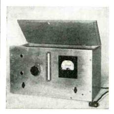
The turbidity of small amounts of solutions in chemical test tubes can be measured with this electronic microdensitometer
