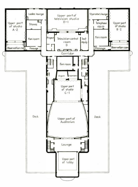
Second floor plan of Radio City. Studios and observation rooms occupy most of this space. All television operating facilities are located on the second floor
