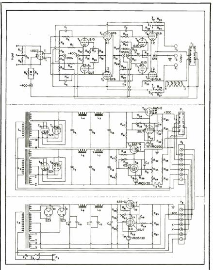
FIG. 5—Schematic of complete stabilized direct-coupled amplifier. Parts list is given in the accompanying text
