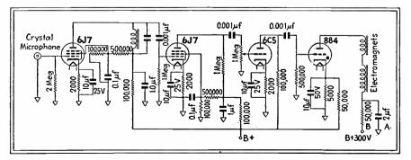
Fig. 2—Circuit of electronic amplifier for energizing the electromagnets that position the indicating pointer of the depth measuring instrument
