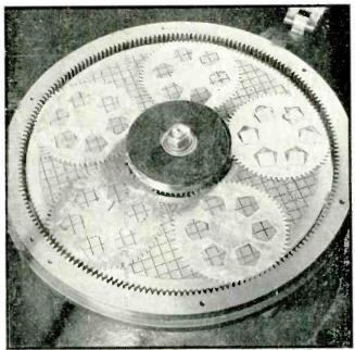
ABOVE: In one step of the grinding process, the quartz wafers are placed in pentagonal holes in planetary gears that revolve and rotate with abrasive between two cross-grocved plates
