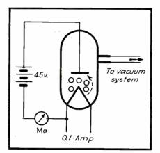
FIG. 8---An emission gage using a diode tube
