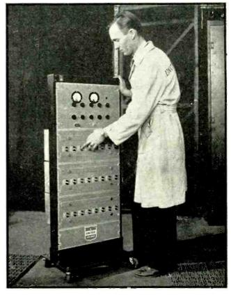
Signal generator used for measuring frequencies and aligning all aircraft radio receivers carried aboard Mainliners. Pushbuttons select any of 24 crystal-controlled frequencies
