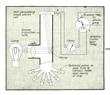
**A**DDITION of photoelectric smokedetecting apparatus to the Rich system for detecting smoke by sight and smell provides for ships at sea an automatic fire alarm system comparable in speed and effectiveness to the finest modern installations in buildings.
