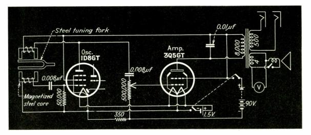
Circuit diagram of the oscillator-amplifier. Coupling between the plate and grid of the 1D8GT oscillator is dependent upon mechanical movement of the tuning-fork tines
