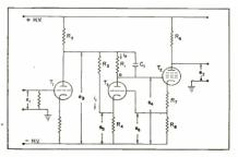
FIG. 2—Basic circuit in which a tube,  $T_{3}$ , stabilizes the amplifier
