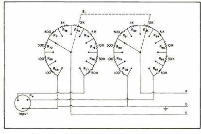
FIG. 7—Input attenuator detail. Each resistor is a ½-watt unit
