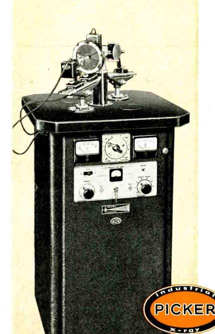
In X-Ray Diffraction, Industry has at hand an indispensable means for quick, accurate, chemical and physical determinations, by graphic demonstration of the actual microscopic structure of materials.
