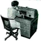
NEW, COMPACT, G.E. ELECTRON MICROSCOPE distinguishes objects as small as 1.000,000th of an inch...magnifies them directly to 5,000 or 10,000 times actual size. If photographic enlargements are wanted, blow-ups can be made to show objects at 100.000 times their true size. Can be plugged into a regular 110-volt A.C. line,
