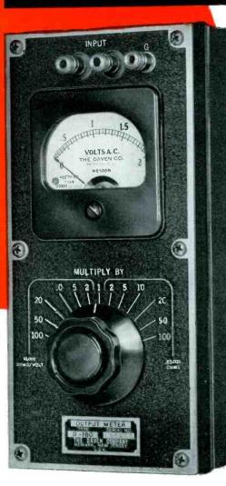
The DAVEN D-180 Output Meter is a combination of a high impedance voltmeter and a constant impedance output meter. The high impedance voltmeter range is particularly convenient when measuring transformer secondary voltages and as a bridging indicator where a high impedance is required. The constant impedance range serves as a null detector and as a beat indicator in the comparison of two frequencies.
