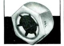
\*DOUBLE LOCKING ACTION When the Palnut is wrench - tightened, its arched, slotted jaws grip the bolt like a chuck (B-B), while spring tension is exerted upward on the bolt thread and downward on the part (A-A), securely locking both.
