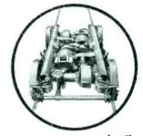
INSUROK brake beam bearings, four in a series, are used on each truck.
