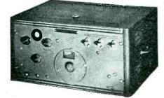
**D**ESIGNED for precision measurements of small capacitance and inductance, the G-E radio frequency capaci-tometer has found acceptance in colleges and industrial laboratories due to its simplicity and compactness.
