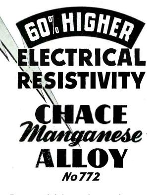
Recommended for use by manufacturers seeking an alloy with exceptionally high electrical resistivity ... Chace Alloy No. 772 has an electrical resistivity of 1050 ohms per circular mil foot or 175 microhms per cm<sup>3</sup> —about 60% higher than most resistance alloys in common use . . . its temperature coefficient of resistance is .00014 per degree centigrade... resistivity value is not affected by annealing procedure, cold working or by cooling to — 100 F. . . this alloy is nonmagnetic.
