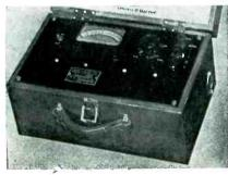
mental samples of insulating material. The instrument consists of an electronic rectifier, a Thyrite bridge circuit, and an electronictube voltmeter. It is available in two types. One type has a scale calibrated from 1 to 50 megohms and measures resistance at 500
