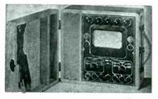
to 1500 volts, 7 direct current ranges up to 30 amp, 1 alternating current range up to 3 amp and 5 resistance ranges up to 10 megohms. Sensitivity of the meter is rated 1,000 ohms per volt on both a.c. and d.c.
