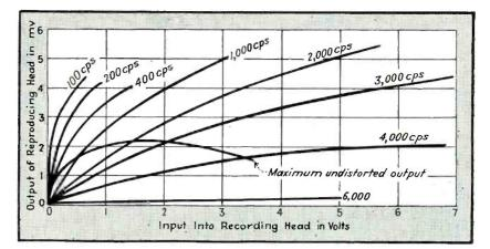
FIG. 2—Input-output curves of a magnetic tape recorder for various frequencies
