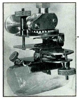
Quartz crystal mounted on intermediate swivel fixture in preparation for rodometric examination
