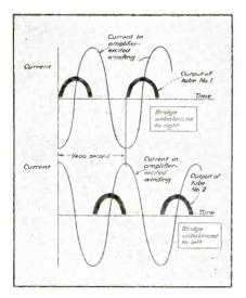
FIG. 5—Curves showing output currents of 7C5 tubes and corresponding currents in amplifier phase of waste-gate motor for both types of bridge unbalance
