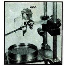
FIG. 5—Upper part of rodometer
