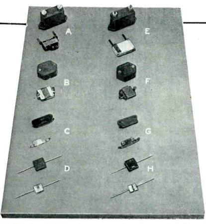
Typical mica capacitors and their unit assemblies are shown at A, B, C and D (left). Alternative types that are mechanically interchangeable are (right): E, glass capacitor; F, molded Lectrofilm capacitor; G and H, molded paper capacitor
