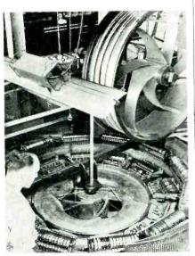
This basket-weaving machine braids wire sheathing on a cable for naval use. The machine weaves 360 wires at one time and was shown in U. S. Steel's annual report for 1943
