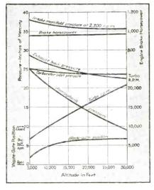
FIG. 6—Curves showing operation of turbo control equipment during a climb from 5000 ft to 30,000 ft
