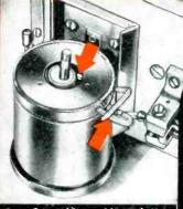
Transflex tubing withstands repeated deformation by the cam used to start, reverse, or completely stop the flow of ink from reservoir to pen. It also is resistant to the cam and recess lubricant. (Partially assembled, underside view.)
