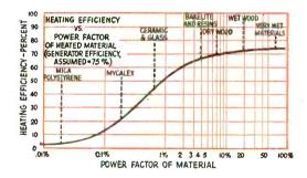
• CURVE B—Assuming a 75% efficiency for the electronic generator, the overall efficiency of an electronic heating installation depends on power factor of the heated material, as shown.
