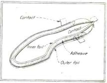
Two metal foils, mounted along the edges of a layer of adhesive, provide electrodes for the application of r-i energy in glueing shoe soles
