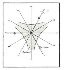
FIG. 3—Relationship between axes and light pattern for left quartz, in which the spot pattern appears to be rotated counterclockwise from the star points
