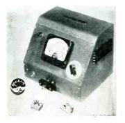
meter magnets, this new device can . be used for comparing various types of magnet steel. Different sizes and shapes of search coils may be used and may be made small enough to insert in the air gap of assembled meters.
