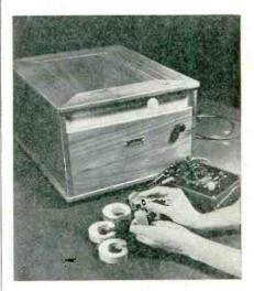
This G-E fluxmeter uses a lightbeam to show the deflection of a galvanometer coil caused by current induced in a search coll surrounding a magnet
