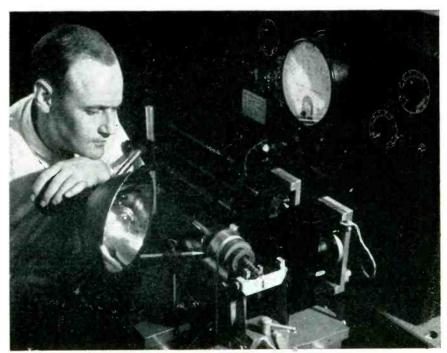
Electronic Dynetric balancing machines show the degree of unbalance of a rotor, while running at normal speed, directly on a meter. The operator sees the spot on the revolving rotor that is out of balance with a stroboscope. The electronic method, developed by Westinghouse research engineers, determines the exact location and amount of corrective mass necessary to eliminate unbalanced vibrations as small as 25-millionths of an inch
