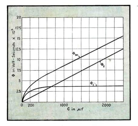
FIG. 5—Curves for maximum flux in the welding transformer as a function of capacitor size, with a constant turns ratio value n of 150. Circuit constants for these curves are those of the example in the article. The two lower curves are for the components that make up the maximum flux at each instant
