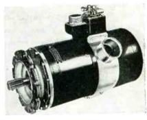
a-c and d-c outputs are available simultaneously over the entire rated speed range. The generator is designed to mount on the main engine generator of aircraft.
