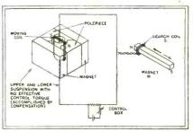
The circuit of a simple fluxmeter illustrates the principle of operation
