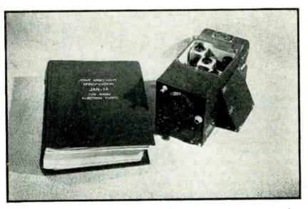
Electronic units for field use, like this BC454B radio receiver for radio command sets in airplanes, must be designed to take into account the normal tolerance variations in electron tubes. These standard tolerances are set forth in Joint Army-Navy Specification JAN-1A for Radio Electron Tubes
