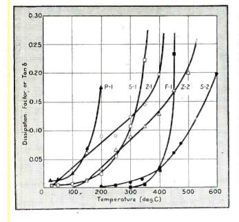
FIG. 3—Dissipation factor at 100 kc of various bodies versus temperature
