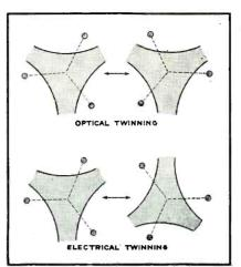
FIG. 4—Effect of the two types of twinning on the refraction pattern as the etched surface is moved in a plane perpendicular to the light beam
