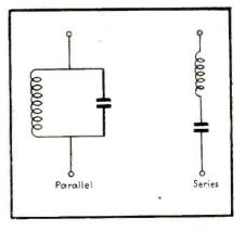
FIG. 1—Fixed-tuned resonant circuits generally require capacitors having high Q
