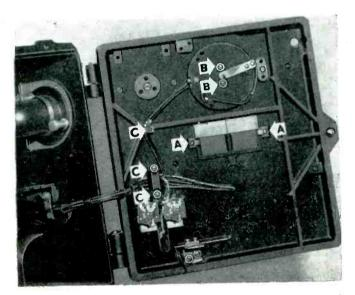
**DEPENDABLE STRENGTH** is another advantage of the simpler P-K fastening method. Above, P-K Type "Z" Screws are used (A) to attach steel clips fastening window to plastic door; (B) to fasten plastic rheostat disc to door; (C) to attach steel clamps holding wire to door. The screws form their own strong threads as they are turned into plain, untapped holes. One easy operation makes a fastening.
