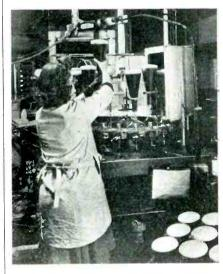
After the sealing-in operation, cathoderay tubes are baked, bombarded, evacuated and sealed on this machine. A complete tube leaves the machine every two minutes at the North American Philips plant
