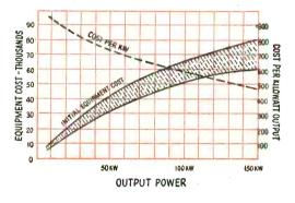
• CURVE A—Initial cost of electronic generators and cost per rated kw based on a number of installations made by different manufacturers.
