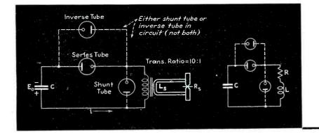
FIG. 1—Basic capacitor-discharge welding circuit (left). and simplified equivalent circuit (right)
