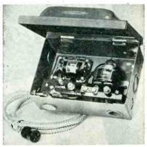
which will handle a load up to 30 amps at 110 volts a.c., or 20 amps at 220 volts.) These two relays are mounted side by side on a hingecovered housing which measures  $5\frac{3}{4} \times 5\frac{1}{4} \times 3\frac{1}{2}$  inches. A convenient terminal block is furnished below the two relays with marked terminals for line connection. A 4-foot armored cable, equipped with a plug, is attached to the side of the housing and is all ready for connection to the instrument.
