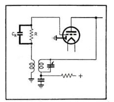
FIG. 6—Detector and oscillator circuits with grid-leak bias arrangements are not materially affected by low-Q capacitors when the leak resistance is small compared to the effective shunt resistance of the capacitor
