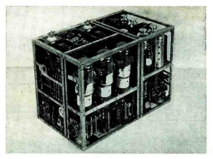
Rear view of Jap Model 13 transmitter-receiver
