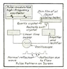
FIG. 3—Flaw detection by observation of reflected supersonic waves
