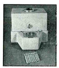
Supersonic instrument for inspecting steel punches. Punches are tapped on the anvil just under the grille protecting the crystal microphone. If the supersonic vibration frequency of a punch is outside the predetermined pass band, the indicator lamp at the top of the instrument is automatically turned on
