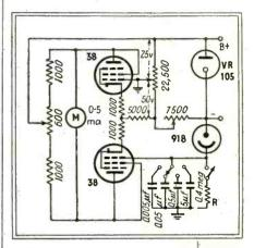
Circuit of electronic components in the shutter speed meter. The phototube is actuated by light from a small spotlight passing through the camera shutter and lens. A conventional power supply is used to provide the B voltage
