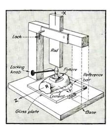
FIG, 7—Final mounting of crystal in scaffold
