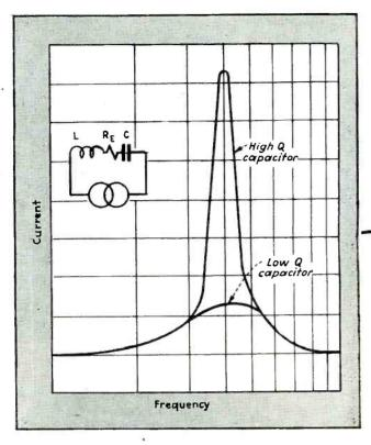
FIG. 2—Curve showing the reduction of current in a resonant circuit due to the additional resistance of a low-Q capacitor
