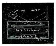
FIG. 4—Flaw detection by immersing specimen in oil and sending a supersonic beam through it. Amount of light reflected from surface of oil is proportional to amount of supersonic energy passed by piece to be tested
