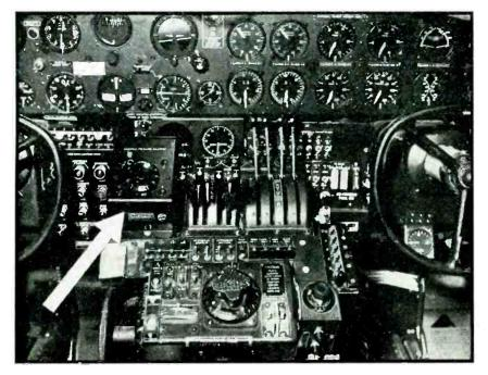
Location of turbo boost selector at right of pilot on a B-24 airplane
