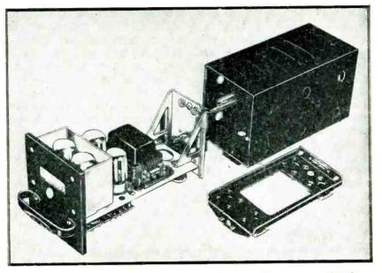
Turbo amplifier removed from its cabinet. The two 7C5 tubes are directly behind the front panel in a chimney-type enclosure, since they handle all current for one phase of the waste-gate motor
