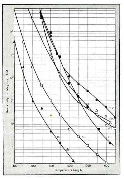
FIG. 5-Resistivity of various bodies versus temperature
