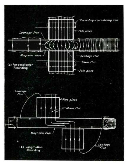
FIG. I—Positions of pole pieces and approximate flux distribution in magnetic tape for two types of magnetic tape recording
