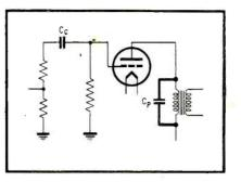
FIG. 4—In audio-frequency amplifiers, both the coupling capacitor  $C_{\sigma}$  and the capacitor  $C_{\sigma}$  across the transformer primary may be low-Q types
