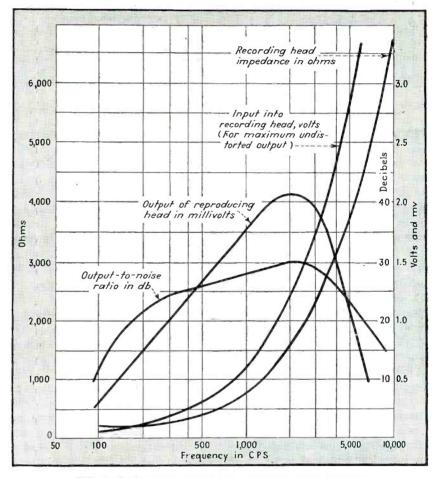
FIG. 3-Performance curves for a magnetic tape recorder
