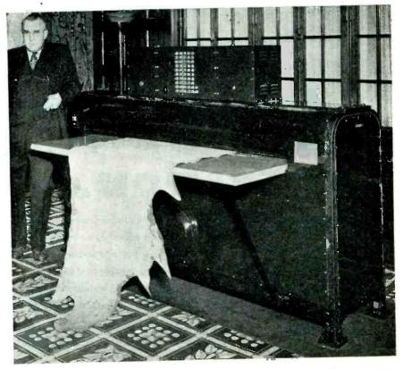
Complete assembly of the Stockton area calculator. The bottom cabinet contains photoelectric equipment that scans thin pieces of hide traveling over a slot. The top cabinet houses an electronic calculator that counts unit areas of the hide
