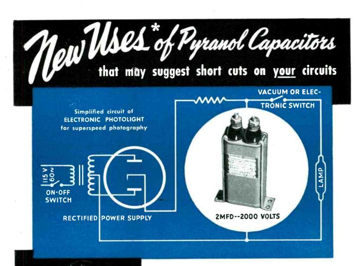
**IN THREE SECONDS** this small Pyranol capacitor accumulates enough energy to discharge 4,000,000 watts in four millionths of a second through a mercury lamp, producing a flash one-fifth as bright as the sun's surface.
