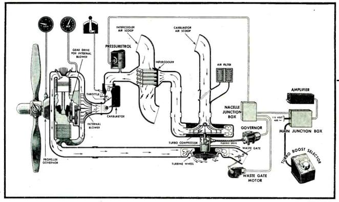
FIG. 1—Schematic diagram of electronic control system and associated mechanical parts of a turbosupercharged engine. The pilot controls the entire system with the single knob on the turbo boost selector box at the lower right
