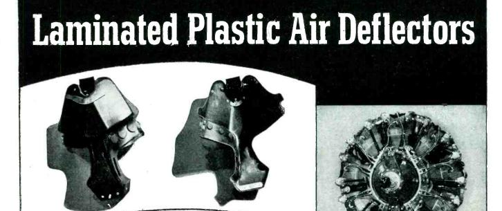
Intricacy of design and contour of typical PANELYTE air deflector is shown in photo above. Right: Wright Cyclone 9, showing deflectors and push-rod housings in place.
