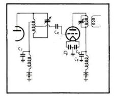
FIG. 5—Capacitors used across low impedance circuits, such as  $C_p$ , may have a fairly large dielectric loss without affecting operation of the circuit. Capacitors  $C_c$  and  $C_f$  are often low-Q types in current production
