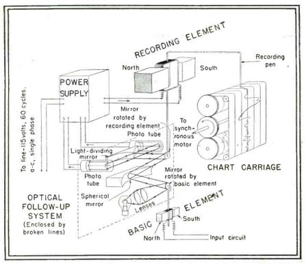
Mechanical arrangement of the mirrors and phototubes used in the recorder. Light reflected from the mirror of the basic measuring element controls the current supplied to the recording element
