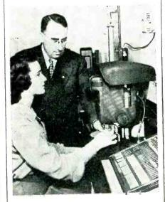
Dimensions of less than two-millionths of an inch are measured by this gage made by Sheffield Corp. It will reveal the degree of expansion of a piece of metal when warmed by a human hand
