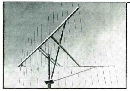
FIG. 1a—One of the two unidirectional 118-Mc arrays used at Sacramento for receiving signals relayed by the Mt. Diablo and Blue Canyon repeater stations. Use of a coaxial antenna permits the entire assembly to be built around a single support-point, facilitating orientation
