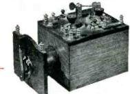
Crystal wireless receiver as built for the Signal Corps in 1917
