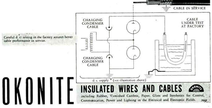
Okonite high voltage cables must pass super-voltage tests made with this d. c. kenotron set.
