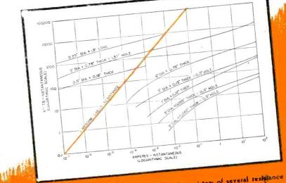
Typical volt-ampere characteristics of Thyrite resistors of several resistance levels and power ratings. Note that the nonlinear voltage-current characteristic extends over an extremely wide current range. Compare it with the characteristic (orange line) of a 1-megohm linear resistor.
