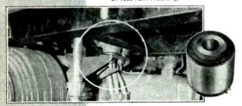
acf Moto-Railer Engine Installation on V. S. Tube Form Mountings
