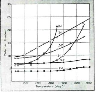
FIG. 4—Dielectric constant at 100 kc of various bodies versus temperature
