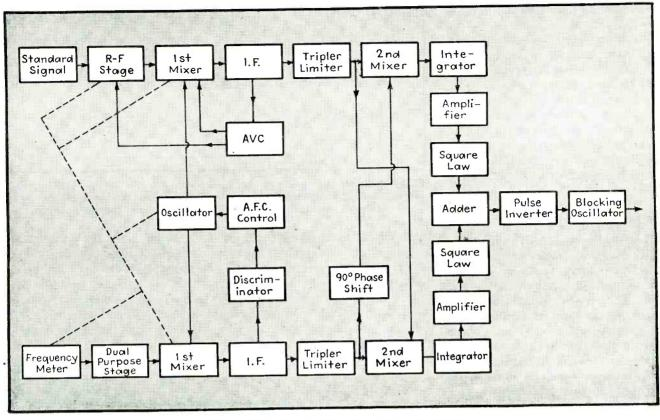
FIG. 6-Block diagram of complete zero beat detector
