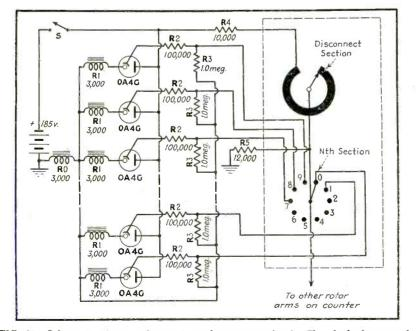
FIG. 15—Schematic of one column of number storage bank. The dashed rectangle at the right encloses a representative section of the revolution-counting switch
