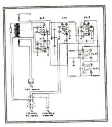
Circuit of the electronic amplifier section of the photoelectric recorder
