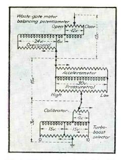
FIG. 2—Complete bridge circuit of the Minmeapolis-Honeywell type B control system for turbosuperchargers. All three windings are on a core having a 115-v. 400-cps primary
