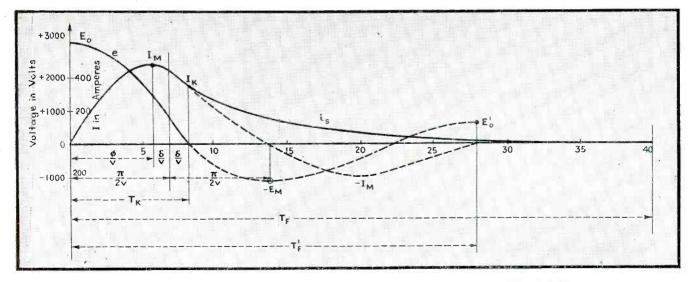
FIG. 3—Welding current and voltage as calculated for the two circuit versions of Fig. 1. Solid lines are for system with shunt tube; dash dash line for system with inverse tube
