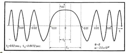
FIG. 3—Zero beat wave form for which  $\theta = 0^{\circ}$ , and for which a calibrating time of six minutes is assumed. Here  $t_i$  represents the maximum permissible limits for triggering
