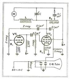
Novel circuit for determining the inductance of an iron-core reactor while carrying the normal amount of direct current
