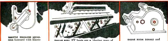
NISM fastened with Elastic Stop Nuts keeps throttle settings the same, even when the hull is distorted by heavy seas.
