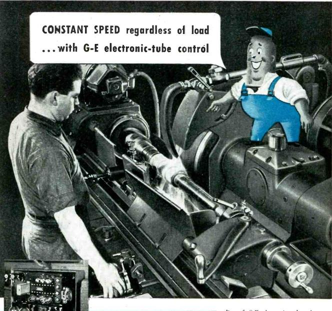
The G-E thyratron tube is the "heart" of the G-E Thy-mo-trol unit which keeps the grinder going at uniform speed.
