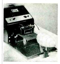
Shutter speed meter used to check timing of a miniature camera. The intensity control, meter-range switch and calibration pushbutton are on the panel. Exposure time is read directly on the meter scale
