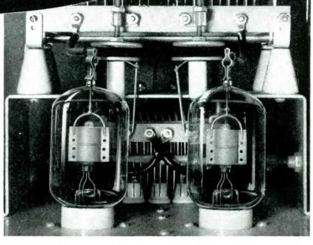
FINAL AMPLIFIER of the main station (WRAQ) at the Barnstable County Jail and House of Correction, showing the pair of Gammatrons still on the job after approximately 38,000 hours of operation.
