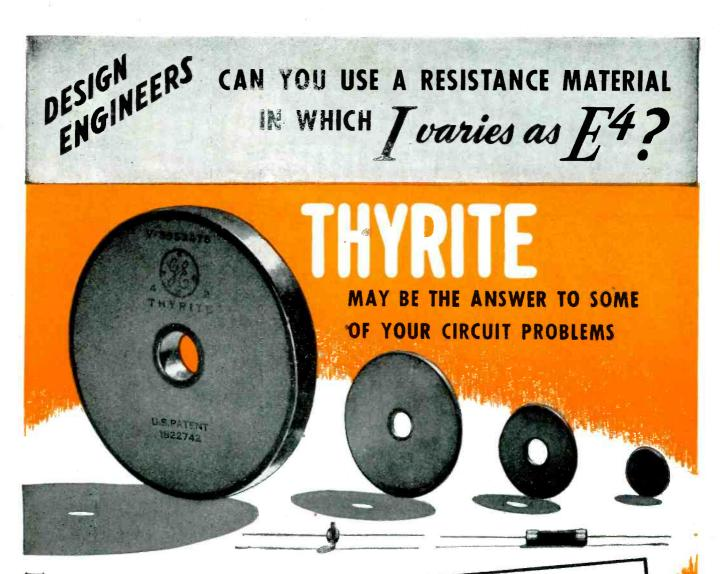
THYRITE\* is a silicon-carbide ceramic material, dense and mechanically strong, having nonlinear resistance characteristics—the resistance varying as a power of the applied voltage. Its resistance characteristic is stable, and substantially independent of polarity or frequency. Thyrite has been used for many years in many important applications, including electronic. Thyrite can be produced in various shapes and sizes (those which can be successfully molded).
