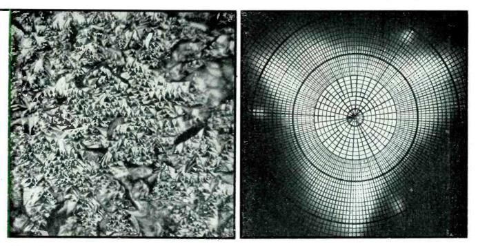
FIG. 1—Appearance of etched ground surface of quartz after three hours of etching, as seen through a microscope. The cracks between the triangular etch pits and pyramids are due to grinding
