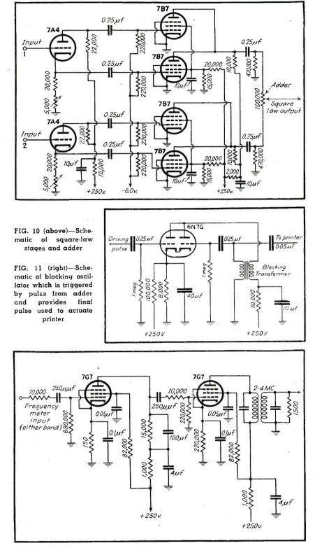
FIG. 12—Schematic of dual-purpose input stage for channel 2. This stage accepts a signal from either band of the frequency meter without switching, and supplies a 2 to 4-Mc signal to channel 2. The latter signal is the fundamental of the high band or the sixteenth harmonic of the low band
