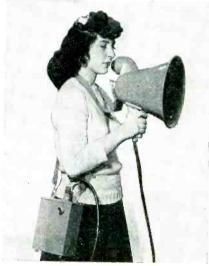
Operation anywhere is provided by this portable electronic megaphone. Mounting of the microphone above the horizontal axis of the loudspeaker permits viewing the place being addressed
