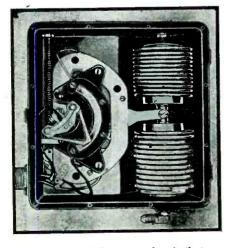
Interior view of Pressuretrol unit that responds to changes in carburetor pressure
