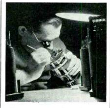
This worker is making final adjustments on a 150-kw polyphase circular scale instrument. The scale covers a 250 deg arc as required on U. S. Navy switchboard installations
