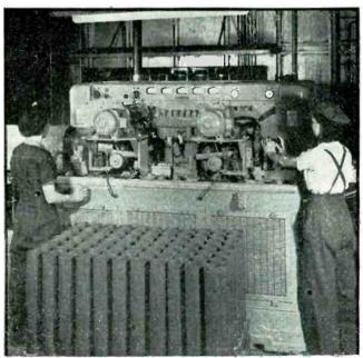
Two jigs support 3-in. steel cartridge cases while they are mouth-annealed at 1300 deg F for four seconds. This inductionheating machine has two stations and an output of 1,000 cases per hour. Hardness before treatment, 98 R.B.; after, 70 R.B.
