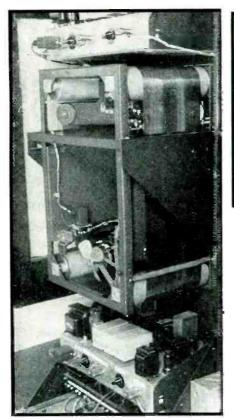
Rear view of a magnetic tape recorder and associated chassis, showing aircooled motor used to drive the endless magnetic tape
