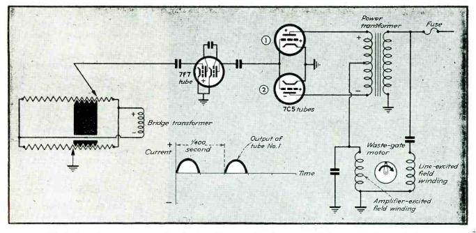
FIG. 4—Simplified version of amplifier circuit in Fig. 3, showing instantaneous polarities for the instant
