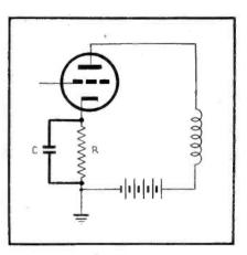
FIG. 3—When used for by-passing, a capacitor may have a low Q without materially affecting the by-pass action
