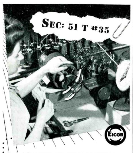
**This armature,** when completed, is destined for an important mission. It is being wound for one of hundreds of Eicor dynamotor designs—and may be used in one of scores of varied applications. One factor alone remains constant—the requirement for complete reliability.
