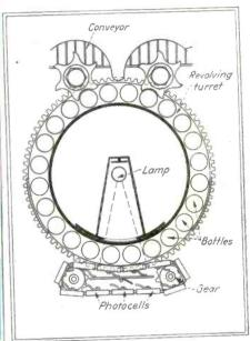
Continuous inspection of beverage bottles is obtained by having the bottles travel through a lightbeam in step with moving photocells
