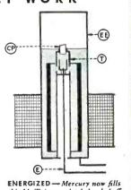
ENERGIZED-Coil C pulls plunger P down into mercury. Mercury thus displaced enters thimble T through orifice O. Inert gas in thimble gradually escapes through ceramic plug CP—thus producing time delay.
