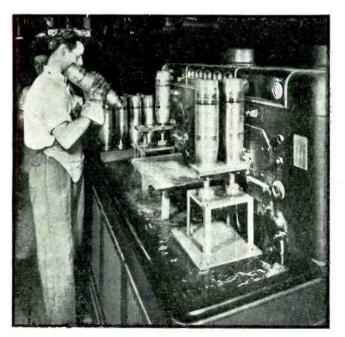
An induction-heating unit brazes adaptors on 105-mm chemical shells in one large Detroit plant without heating the sidewalls of the shell. The machine, made by Tocco Division of Ohio Crankshaft Co., has an output of 140 shells per hour
