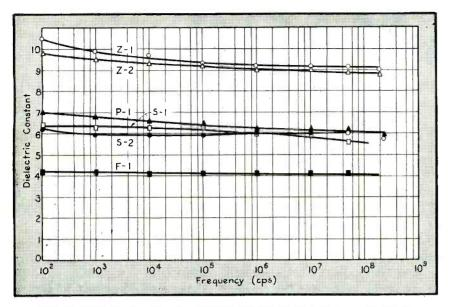
FIG. 2—Dielectric constant of various bodies versus frequency at 25 deg C
