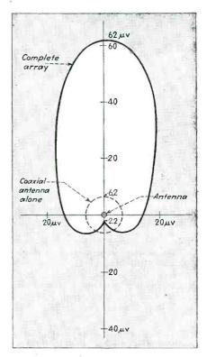
FIG. 3—Field-strength pattern of the 60-deg corner reflector array and, for comparison, the pattern of the coaxial antenna alone
