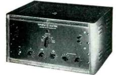
**D**ESIGNED for testing over-all performance of radio systems and networks, this self-contained instrument generates its own frequency with remark-able stability. Can be synchronized from an external source.
