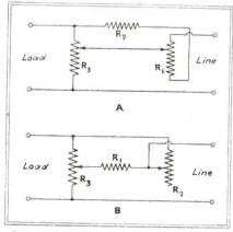
Suggested circuits for maintaining practically constant impedance with a minimum of resistance components
