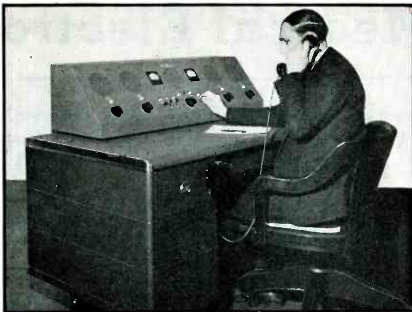
This central control unit, employed in ordnance plant radiotelephone service, is located at the yardmaster's or dispatcher's office and permits radio-equipped locomotives, motor vehicles and secondary-stations within the service area to be instantly contacted
