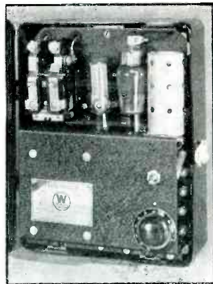
Fig. 4—In this unit the phototube feeds into a single-stage amplifier which, in turn, controls the thyatron under the shield at the right
