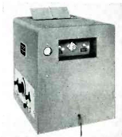
Heater and ventilator controls are recessed in the side of the cabinet on the a-f standard oscillator. The thermometer shows the operating temperature
