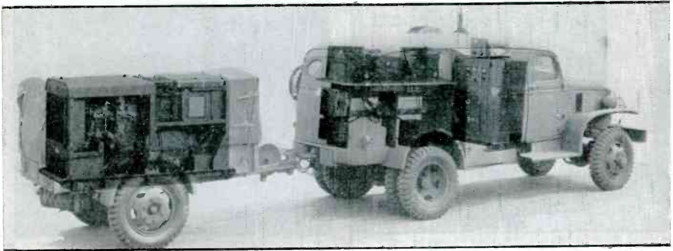
Phantom view of the SCR-299 communications truck and trailer. The transmitter seen in forward part of truck is the BC-610-E
