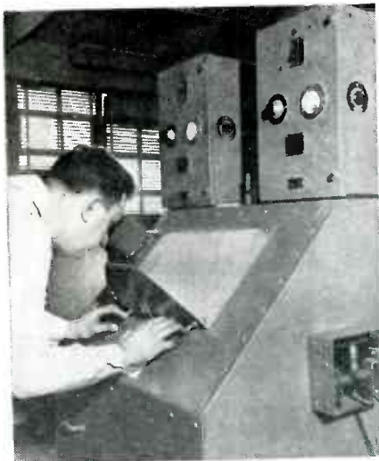
Rubber insulation of wire for high-voltage use is given an x-ray examination at the research laboratories of General Cable Co.
