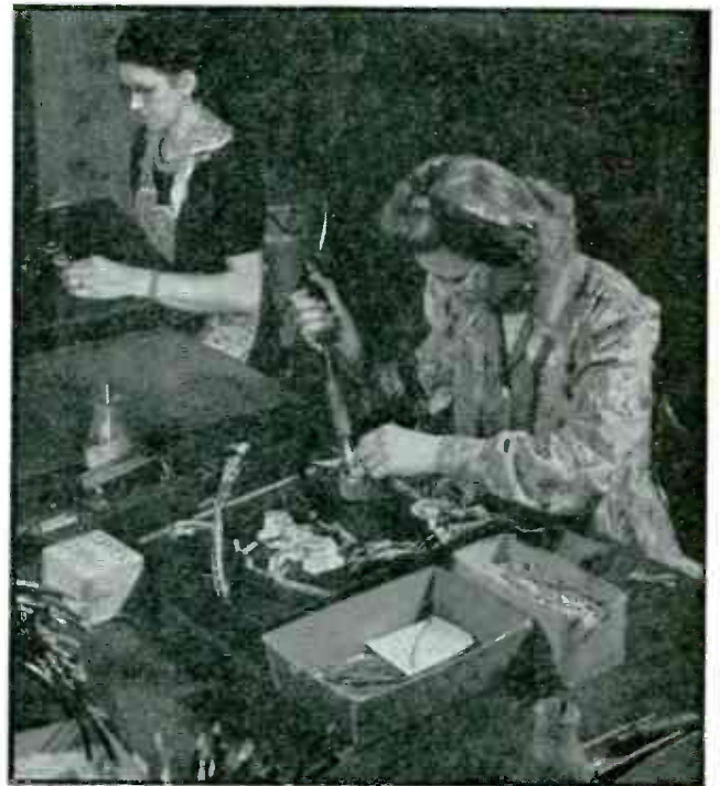
2 Power-control panel assembly starts here, on an auxiliary production line. Parts are mounted on the panel and wiring is completed
