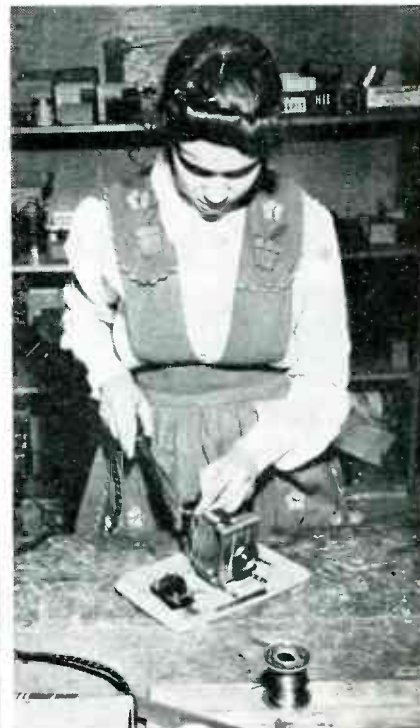
Mary Maderas, 19, solders leads of a one-tube receiver she is building in a beginner class at the New York Institute for the Education of the Blind
