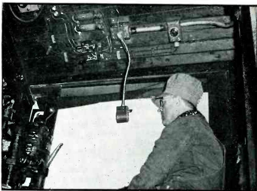
Locomotive radiotelephone installation employed in the Proviso yard of the Chicago and North Western Railway
