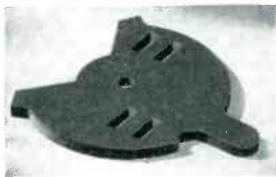
"Cat's head," they call it. The core is Phenol Fibre—to eliminate moisture absorption and to increase dielectric strength. But because an electric arc will not carbonize Vulcanized Fibre, the front and back of the Cat's head are made of Vulcanized Fibre.
