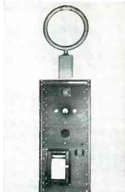
This radio range monitor constantly receives radio range signals and flashes the ground crew if changes occur in the signal. A warning signal is also sent out over the defective beacon to warn pilots
