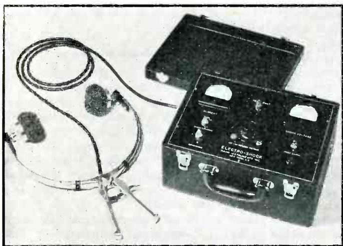
ABOVE—Electro-shock therapy unit made by Rahm Instruments Inc., New York. Balls of steel wool held by locking tongs serve as electrodes
