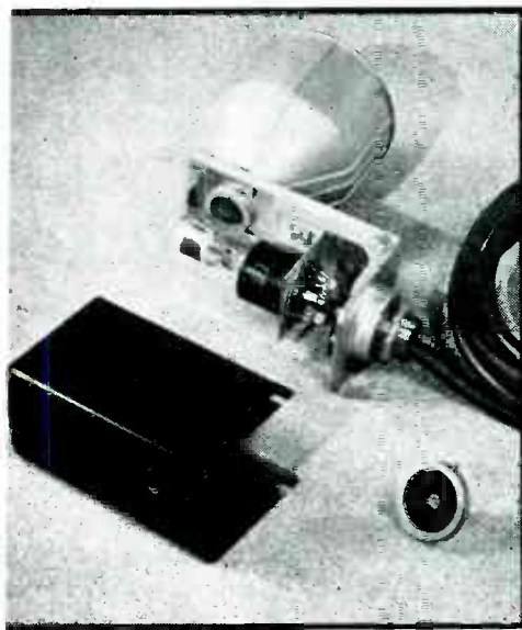
5—This phototube housing contains a large lens and infrared filter
