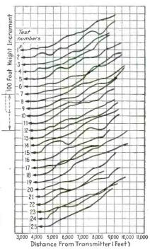
Fig. 1—Flight paths of 25 blind landings. Each curve represents a separate approach and all curves extend through contact
