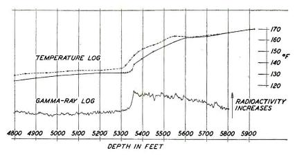
FIG. 4—Comparison of temperature log and gamma-ray curve in a well containing activated cement
