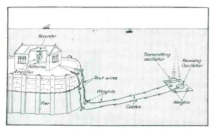
This schematic diagram of a harbor tide-recorder is an interesting practical supersonic application. (From "Precision Echo Sounding and Surveying", by Lt. Commander D. H. Macmillan, Henry Hughes & Son, Ltd, 59, Fenchurch St., E.C. 3, London). Both oscillators are on ocean bottom
