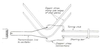
Fig. 10—Schematic illustration of the r-f connections used to feed the forms shown in Fig. 8 and Fig. 9. A tuning stub is used to parallel tune the load
