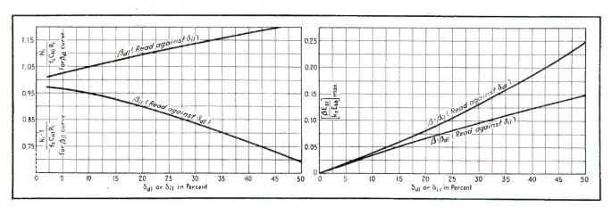
Fig. 4.1—Value of  $N_1/f_sC_{h1}R_1$  that maximizes  $\beta_{d1}$  or  $\beta_{i1}$  as a function of  $\delta_{i1}$  and  $\delta_{d1}$ . Multiply the ordinate by  $N_1/(N_1-1)$  to obtain  $N_1/f_sC_{h1}R_1$  for the  $\beta_{i1}$  curve
