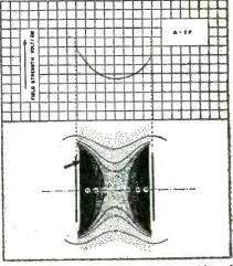
Fig. 2—Field distribution in a meridional plane between two parallel circular plates
