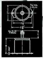
Type 1860 (see photo and above drawing has suitably plated brass terminal mounted in mica insulating plate. Dimension A is from 2
