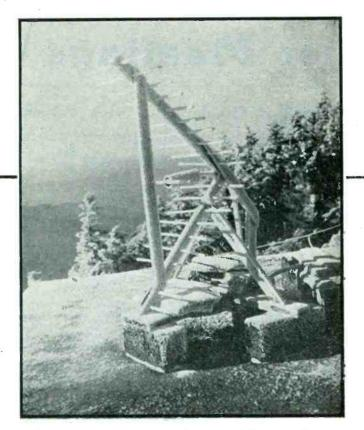
Square-corner antenna originally used at Clingman's Peak to receive 337-Mc signals from the 25-watt Winston-Salem relay transmitter W4XGG
