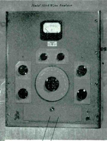
There are only three standard -hp- instruments included in this laboratory set-up yet the two units include the following seven: an -hp- Resistance-Tuned Audio Oscillator, an attenuator, a vacuum tube voltmeter, a set of fundamental elimination filters, an input meter, an output meter, and a wave analyzer. The uses for this combination of instruments are too extensive to list here but some idea of its scope is shown by the following:
