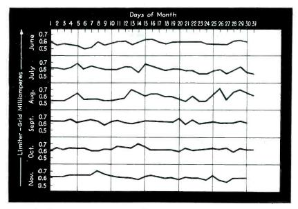
Graphs showing signal received at Clingman's Peak from the 25-watt, 337-Mc f·m relay transmitter W4XGG at the Winston-Salem studios. Readings were all taken in 1943. Limiter-grid current of 0.5 ma indicates 100  $\mu$ v input
