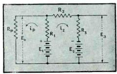
Fig. 1—Basic bridge circuit. and bridge version used for interstage coupling
