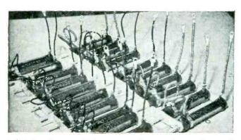
Indent cannectors are widely used an resistors and other small electrical companents since they eliminate all troubles due to loose connections, and provide better circuit performance.
