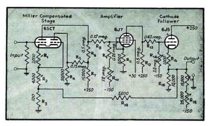
FIG. 9—A two-stage d-c amplifier using a Miller compensated stage, a cathode follower, and stabilized negative feedback
