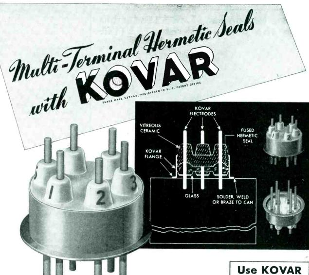
ERMETIC transformer or capacitor seals of Kovar and glass may be made in a wide size range and with single or multiple electrodes. Electrodes may be solid or tubular.
