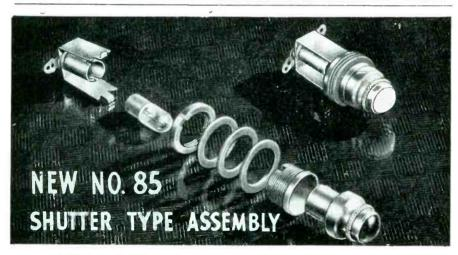
A LOCKING SLIP-FIT BEZEL is one of the big features of this new and better DRAKE Shutter Type Assembly. It permits instant lamp replacement from front of panel, without tools! Other improvements are complete, uniform illumination over entire surface of Jewel, and complete blackout with a quarter (90°) turn to right. Three fibre washers compensate for varying panel thick-
