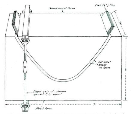
FIG. 7—Arrangement of male and female forms for making the laminated section shown in Fig. 5. Pressure is applied by means of a large number of hand-clamps. Radio-frequency heating is applied by utilizing the steel face plates of the forms as electrodes
