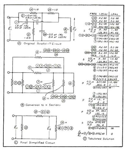
FIG. 4—Original circuit and steps in simplifying it for Example III in text, with complete tabulated solution for two different frequencies. An orderly compilation of data minimizes changes of mistakes and permits checking any part of the work quickly. Impedances are numbered for the same reason
