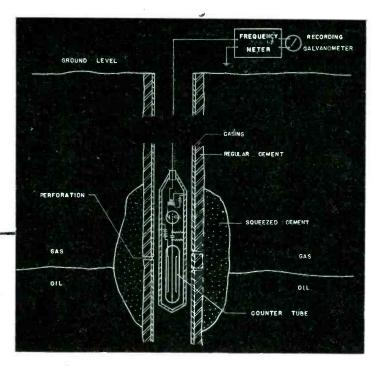
Gamma-ray counter used to detect squeezed cement
