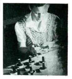
Checking dimensions of Prestite insulator used for terminal posts on capacitors for aircraft equipment to prevent flashover as high altitudes. The insulator, a Westinghouse product, holds up at altitudes of 60,000 feet and resists temperature changes from 234 deg. above zero to 15 deg. below. The insulating material is a mixture of clay, feldspar, and flint and can be solder-
