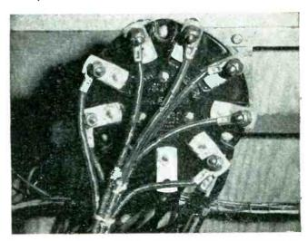
Indent connections are used on rotary switches of all sizes; Burndy Indent connectors being available for all wire sizes from #29 up through the larger cable sizes.
