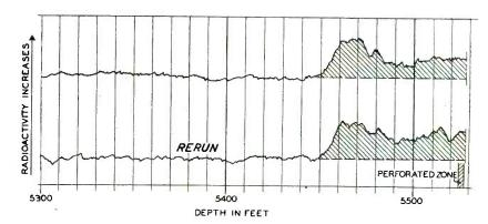
FIG. 5—Gamma-ray curves obtained when using radioactive "squeezed cement."
