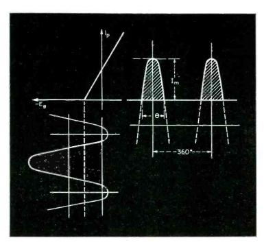
FIG. 1—Diagram illustrating the idealized linear amplifier characteristics on which the main graph in Fig. 2 is based
