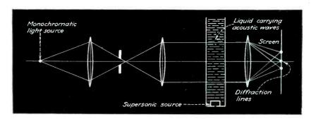
FIG. 5—Arrangement for obtaining diffraction patterns from light that has passed through a liquid carrying supersonic waves
