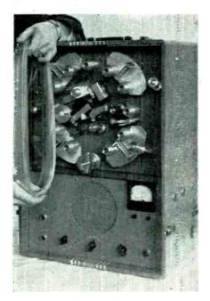
Loading the inch-wide cellophane tape on the feed mechanism of the recorder. The cellophane passes between the recording stylus and a felt bed. Both recording and playback are made with permanent jewels
