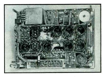
FIG. 4-Intercom amplifier, shown with tubes removed
