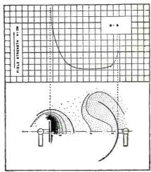
Fig. 5—A cylindrically curved electrode produces this field form
