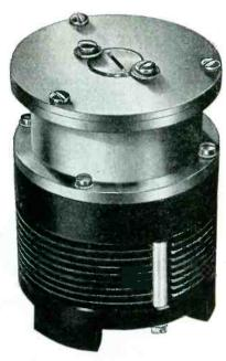
ulator varies the field excitation of an inverter, alternator or special dynamoter in such a manner as to produce constant output voltage across the load. Where the machine is delivering a.c., a rectifier may be provided to supply the regulator solenoid circuit.
