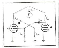
Fig. 4.5—Ripple voltage in the plate power supply is coupled directly into the grid circuit of each tube in the MV
