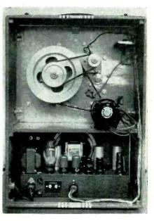
Rear view of the cellophane tape recorder shows the electronic equipment and speaker, at the bottom of the case, and the motor drive mechanism that feeds the tape through the machine
