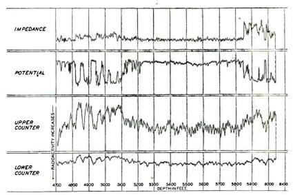
FIG. 1—Comparison of gamma-ray (two lower curves) and electrical logs made in an uncased well
