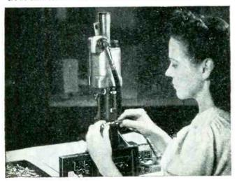
This automatic Burndy HYPRESS indents connectors as fast as the operator can press the trigger. Used extensively by aircraft and electrical manufacturers producing harnesses or leads in large quantities.
