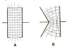
Fig. 1—Homogenous and nonhomogeneous fields. Force lines are shown solid. equipotential lines dashed, and iso-field strength lines dotted
