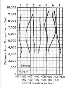
Fig. 2—Several curves of approach paths, showing lateral deviation from the runway centerline. Points marked X indicate contact of the plane to ground and dotted portions of the curves represent taxiing paths after contact
