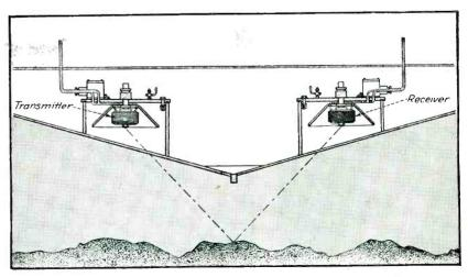
Echo sounding is one important application of supersonic waves. A typical arrangement in a boat is shown here; the transmitter mounted against the hull inside the ship sends supersonic waves down to the ocean bottom, and the receiver picks up the reflected waves. Electronic equipment plots depth on moving tape as ship moves. (From "Precision Echo Sounding and Surveying")
