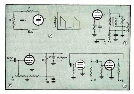
A—Direct voltage produces ionization in *T*, charging *C* through *r*. Voltage across *C* builds up, with an accompanying decrease across *T*, until ionization can no longer be sustained and *C* is discharged through *R*, after which the circuit conditions are returned to their initial state, and the sequence repeats
