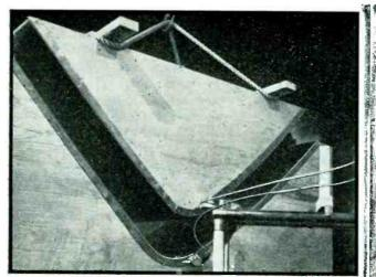
FIG. 8—Photograph of the male and female forms used to make fuselage ring section, with r.f connections in place
