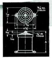
Type 1865 (no photo, but see drawing above) differs in the use of cast-aluminum case and steatite insulator to support terminal and withstand higher voltages. Dimension A is from 2-11/16 to 6-11/16".
