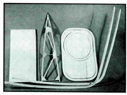
FIG. 4—Some aircraft parts made by the use of r-f heating. Left to right: curved-laminated stock for fuselage reinforcing; wing rib web; bomber door; sections of fuselage ring
