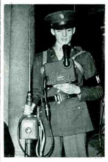
Originally designed for cavalrymen, with the bottom of the antenna fitting into a saddle boot, this guidon radio is also used by other troops on the ground or on the bumper of an army vehicle
