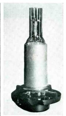
Mercury vapor lamp assembly as used in a typical motion picture printer at Paramount Pictures, Inc. for making release prints
