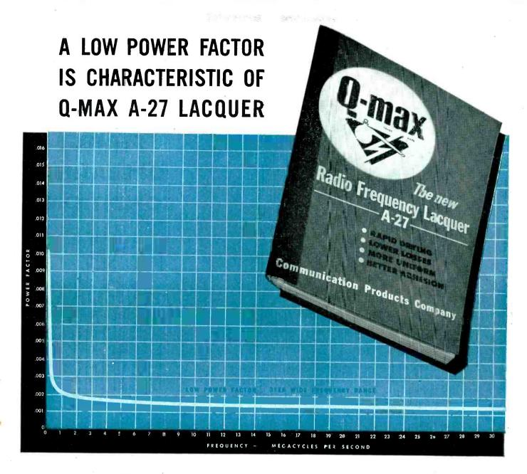
Comparison of the curves published in the new Q-Max A-27 Booklet indicates that the power factor of Q-Max, along with its dielectric constant, decreases as the frequency increases. This is a correlation to be expected, for it is known that the power factor curve reaches a maximum whenever the material undergoes any form of polariza-
