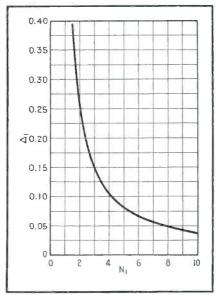
Fig. 4.6—Curve of  $\Delta_1$ —exp  $[-(N_1-1)/f_s$   $C_{h1}R_1]$ —exp  $[-N_1/f_sC_{h1}R_1]$  vs.  $N_1$  using the maximizing values of  $N_1/f_sC_{h1}R_1$  as given in Fig. 4.7
