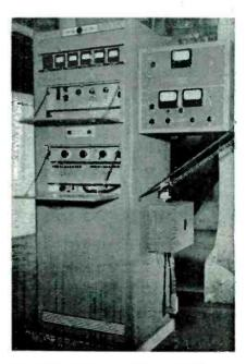
The 25-watt General Electric 337-Mc f-m relay transmitter. Equipment extending from the right side includes frequency and modulation monitors and remote control apparatus
