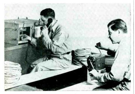
A combination radio-telegraph-telephone set for use in life boats is demonstrated by employees of Radiomarine Corp. of America. While one man cranks the generator, the other operates the equipment to contact nearby ships
