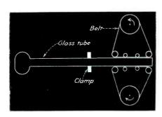
FIG. 4—Holtzmann's ultrasonic generator using two moving belts
