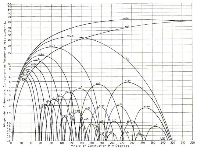
FIG. 2—Graph illustrating the magnitude and phase of the first ten harmonics of an overbiased amplifier. The harmonic amplitudes are expressed in percentages of the peak current, for various conducting angles in degrees
