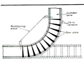
FIG. 2—Corner of a table model radio set made by the process of slotting, steaming and bending as now used
