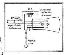
Amplitude-modulated frequencies above 50 Mc can be observed satisfactorily on a commercial oscilloscope when this circuit is used to correct for capacitive coupling between the plates of the tube
