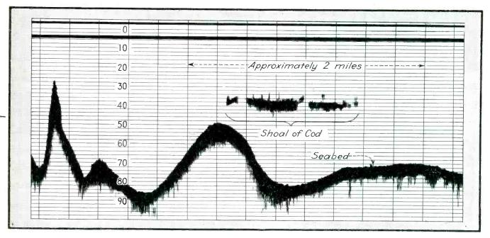
Example of supersonic depth record obtained on a ship. Such objects as fish above the ocean bottom give indications also, making the equipment of great value to deep-sea fishing boats
