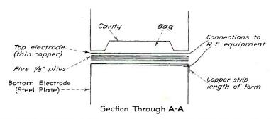
Fig. 11—Sketch of the arrangement used to obtain "flexible" pressure on one side of the laminated assembly. A rubber bag which occupies a cavity in the upper form is inflated to 75 psi after the clamps are applied. Using a thin copper sheet for the upper electrode gives an approximation of "fluid" pressure
