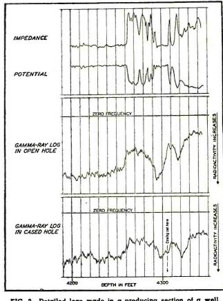
FIG. 3—Detailed logs made in a producing section of a well. electrically, and electronically in open and cased holes
