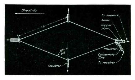
Rhombic receiving antenna. Theoretical signal gain is 11.5 db, theoretical directivity gain 15.8 db
