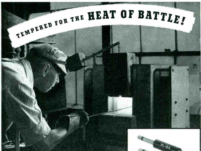
Remler craftsman heat treats welding and cutting dies and tools for automatic screw machines.
