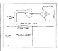
Circuit for maintaining constant illumination by blowing more air around a mercury vapor lamp when the line voltage rises and less air when it decreases
