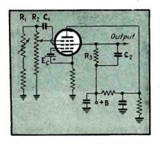
FIG. 2—Basic transitron oscillator circuit.  $R_1$  is the frequency adjustment,  $R_2$  the feedback adjustment, and  $C_1$  the feedback capacitor:  $R_3$  and  $C_2$  are screen grid resonant circuit components.  $E_c$  is the grid bias used to produce sine waves
