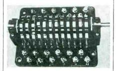
The all-molded construction provides easily accessible terminals, silver to silver wiping and self cleaning double break contacts, and needle bearing shaft suspension.
