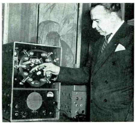
Jay Fonda adjusts the embossing stylus of the cellophane tape recorder he developed.
