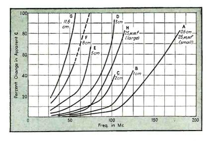
FIG. 2—Percent changes in apparent capacitance with frequency for a midget 25.\(\mu\mu\mu\) f capacitor (A) and a 25.\(\mu\mu\mu\) f unit with physical dimensions twice as large (B). These curves are based on data in Table III. Curves A to G show percent changes in apparent capacitance with frequency for a 25.\(\mu\mu\mu\) f midge capacitor used with leads from 0.6 to 11.6 cm long, as given in Table IV
