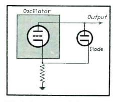
FIG. 6—Automatic amplitude control of this transitron oscillator is used to compensate for a falling off in output voltage
