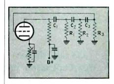
FIG. 7—Usual method of operation of this phase shift oscillator over a frequency range is to make  $C_1$ ,  $C_2$ , and  $C_3$  variable and ganged, while  $R_1$ ,  $R_2$ , and  $R_3$  are switched in steps to change ranges
