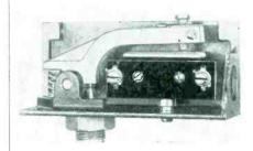
Locking-screw locks temperature setting. Terminal plate has large screw terminals. Snap-action micro-switch eliminates contact troubles. Range 0-1400 deg F. Adjustable range 200-300 deg F. Dimensions are 5½ by 1¾ by 3 in.
