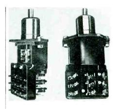
struction providing easily accessible terminals. Contacts are double break, self cleaning due to wiping action, and of silver. Rated for voltage up to 550 ac or dc.
