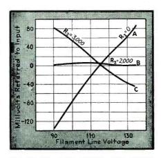
FIG. 10—The effect of Miller compensation on the stability of the amplifier shown in Fig. 9, in respect to filament voltage changes
