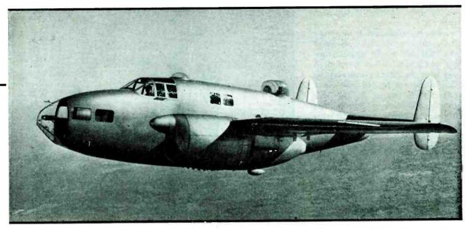
The Fairchild AT-21 Gunnery Crew Trainer, a "plastic plywood" plane of the type referred to in this article. The only metal used in its construction is in the engines, the engine supports, instruments and certain other equipment, supports and controls
