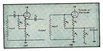
Fig. 5—The conventional R-C coupled cathode follower (a) and the Brubaker equivalent of the conventional cathode follower (b)
