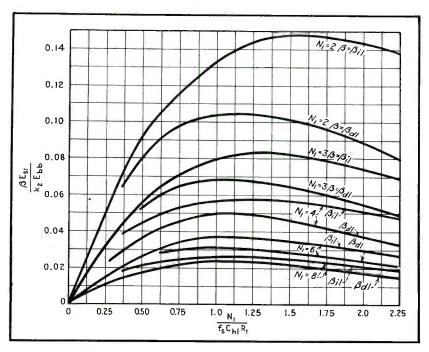
Fig. 4.3—Increase and decrease permissible in the amplitude of the synchronizing pulse for various orders of division as a function of  $N_i t_c C_{kl} R_i$ . These curves are applicable only in the special case of  $\delta_{di} = \delta_{ij} = 1/(2N-1)$
