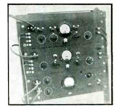
Electronic surface equipment used in conjunction with gamma-ray detector employing two counter tubes
