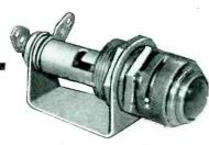
Gothard #431 Pilot Light is used in aircraft, ships, tanks, signal and similar applications where vibration is an important factor. Precision, snug fitting jewel and lens holder maintains set position. 90° rotation of shutter provides gradation of light from
