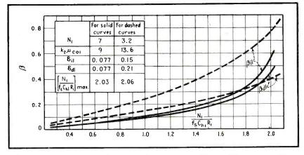
Fig. 4.4—Percentage variation permissible in the amplitude of the synchronizing pulse as a function of  $N_1/I_3C_kR_1$  for the MV's designed in Examples III and IV
