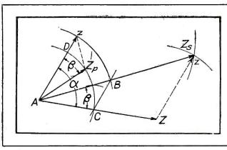
FIG. 2 — Geometric method of combining two impedances in series or parallel
