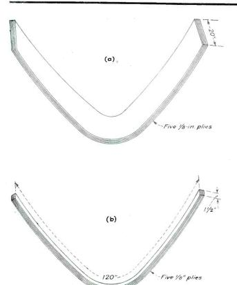
FIG. 5 (left)—Sketch showing makeup of the fuselage ring section shown in Fig. 4. A wide piece of curved-laminated board (a) is formed, and sections (b) are then sawed to required width
