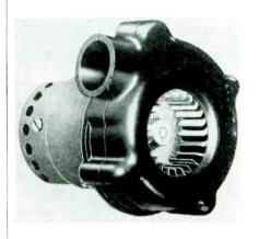
Running at 7200 rpm, the blower circulates 22 cu ft per min continuously. The motor is designed for use in ambient temperatures up to 80 deg C. Overall length of the unit is  $4\sqrt[3]{2}$  in.; weight  $19\frac{1}{2}$  oz.
