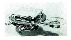
Adjustments are provided to compensate automatically for all wear, a feature which is extremely important in this type of equipment due to the abrasive action of quartz dust. Spring-loaded gears in the gear-train eliminate backlash, thereby assuring setting to minute precision. The gears on the sectorarm and the gear-train are meshed under constantly maintained tension to eliminate any inaccuracies due to tooth wear.
