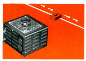
VARIABLE-VOLTAGE AUTOTRANSFORMER used for smooth control of uninterrupted voltage and small amounts of power. Mechanically strong, compact, and light in weight, designed for panel or bench mounting. Operates on low input power and low exciting current, with high efficiency and excellent regulation throughout entire range from zero to full load. Made in three capacities. Bulletin GEA-3635A.
