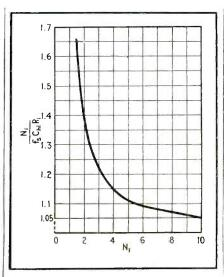
Fig. 4.7—The value of  $N_1/I_*C_{h1}R_1$  given by this curve maximizes the increase in the exponential grid voltage between the  $(N_1-1)$ th and the  $N_1$ th synchronizing pulses
