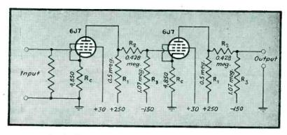
Fig. 3—A two-stage d-c amplifier using pentode tubes
