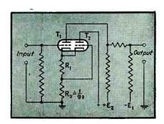
FIG. 8—The basic Miller circuit which improves the drift problem of the input stage of the d-c amplifier. If  $g_2$  is the transconductance of  $T_{\perp}$  then  $R_2$  is nearly equal to  $1/g_2$
