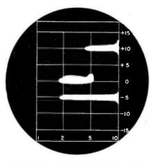
This vertical separation indicator shows a pilot the vertical distance between his plane and others within a fixed radius. A rough indication of the horizontal separation is also provided by the scale
