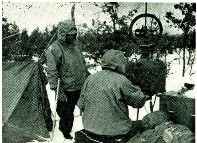
At least two radio direction finder stations like this are set up by the Signal Corps as soon as possible after capture of a beach-head during invasion, to determine positions of enemy radio stations by triangulation.—Signal Corps photo
