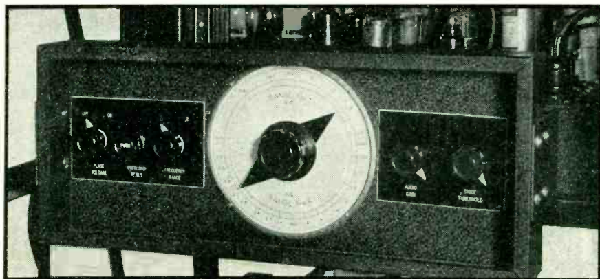
Close-up of variable-frequency electronic generator control panel
