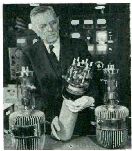
I. E. Mourmtseff, Westinghouse electronics engineer, holds one of the high-power oscillator tubes used in the recently-developed high-frequency process of reflowing tin after electroplating. Alongside are broadcast transmitter tubes that may also play important roles in industrial electronics
