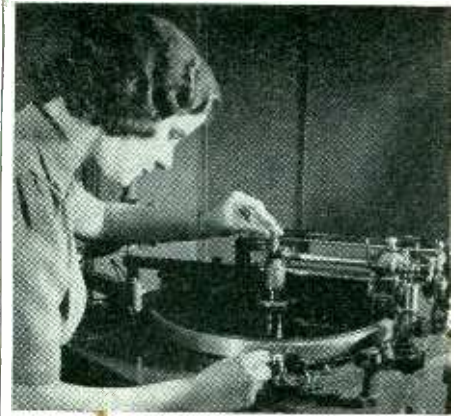
Starting up a Presto disc recording machine in the BBC Engineering Division in preparation for cutting one of the 4000 discs per week used by the British Broadcasting Corp. for radio programs. These photos are unposed, and represent fair samples of what women are doing in England
