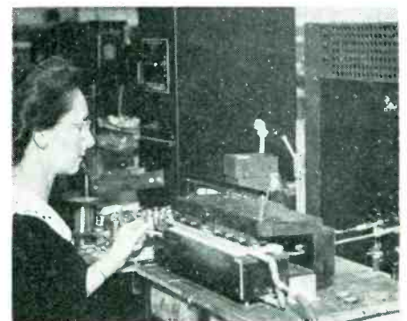
G-E high-frequency heating unit being used to provide heat for simultaneous soldering of six crystal units at a time
